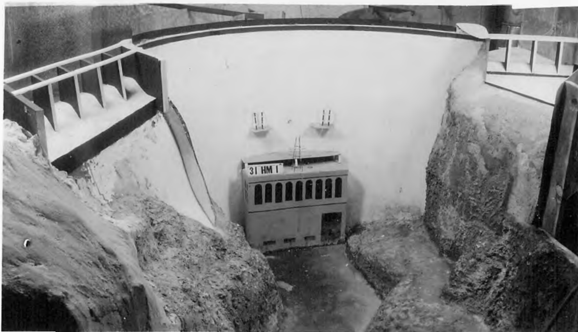
A. No Flow Crest Elevation 1889.0
