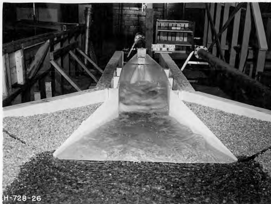
A. Modified gate with flat leaf discharging 200 cfs into stilling basin at a head of 80 feet.
