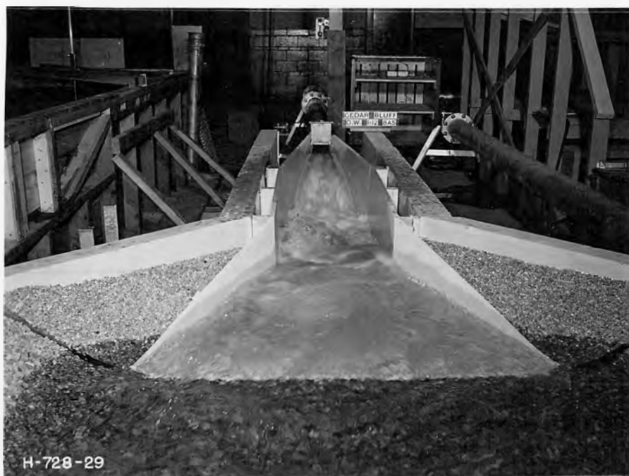
B. Modified gate with flat leaf discharging 760 cfs into stilling basin at a head of 80 feet.
