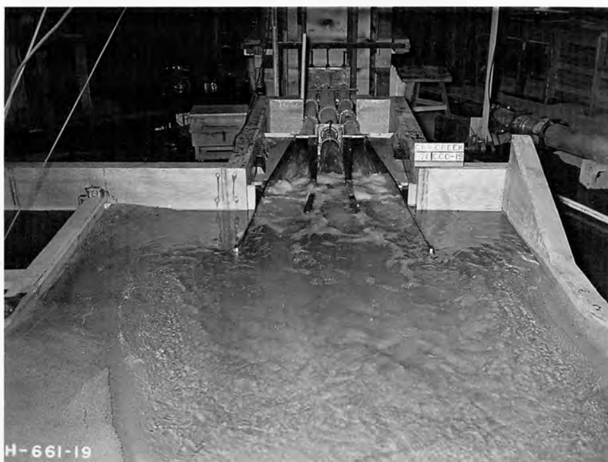
B. All conduits operating - 6,000 second-feet
