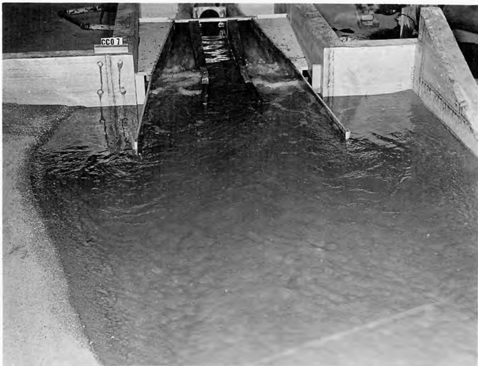
B. Both outside conduits operating - 4,550 second-feet
