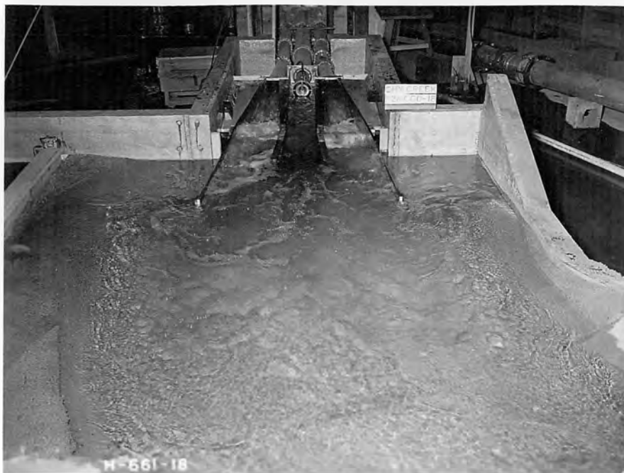
A. Both outside conduits operating - 6,000 second-feet
