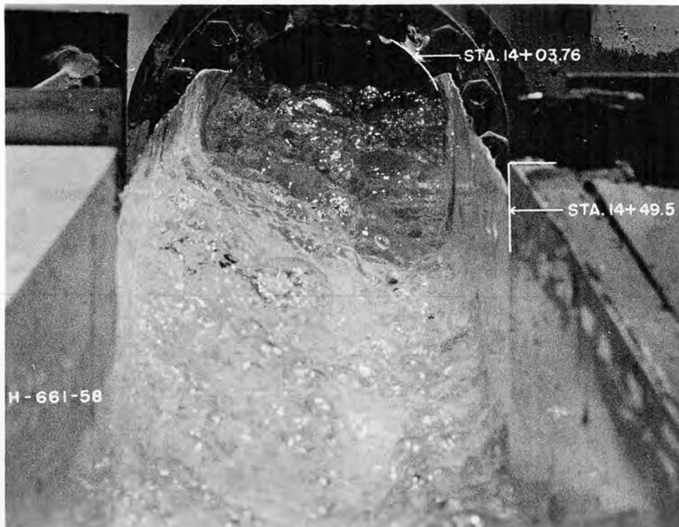
B. Flow in downstream section of left conduit with roof removed, discharge 2,275 second-feet. 1/20,000 sec. exposure.
