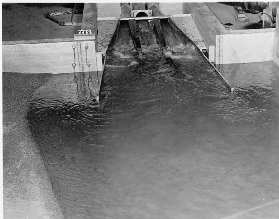
B. All conduits operating - 6,000 second-feet
