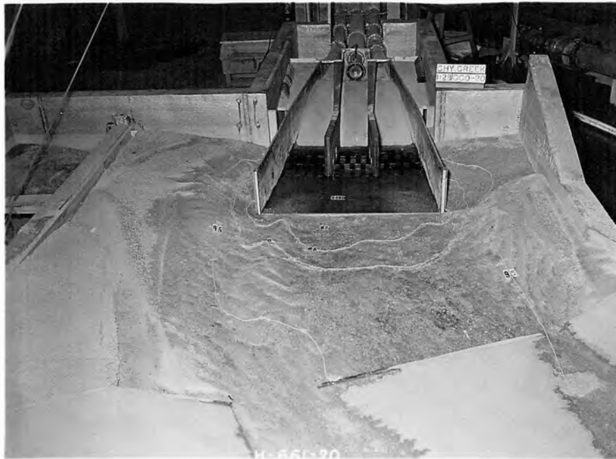
Scour after one hour operation, 3 conduits discharging 6,000 second-feet, tailwater elevation 5502.8
