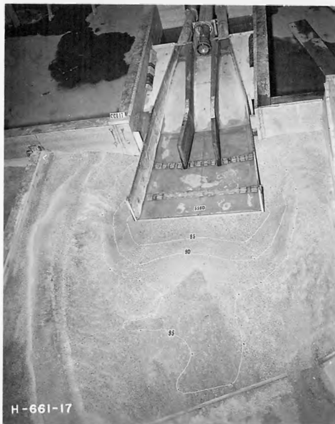
Scour after one hour operation, 3 conduits discharging 6,000 second-feet, tailwater elevation 5502.8.
