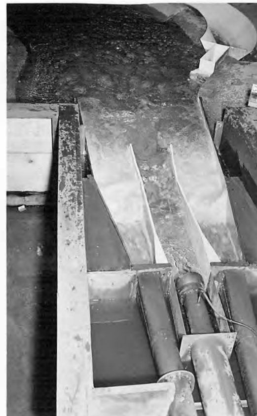
B. Both outside conduits operating - 6,000 second-feet
