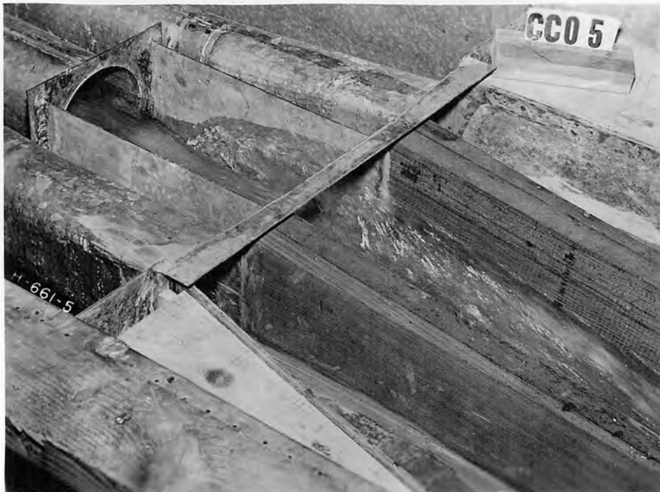
A. Flow near portal of center conduit - Initial phase, discharge 1,500 second-feet
