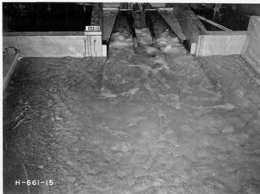
B. All conduits operating - 9,400 second-feet
