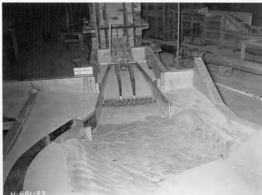
B. Scour after 1 hour operation, 3 conduits discharging 6,000 second-feet. Tailwater elevation 5502.8.
