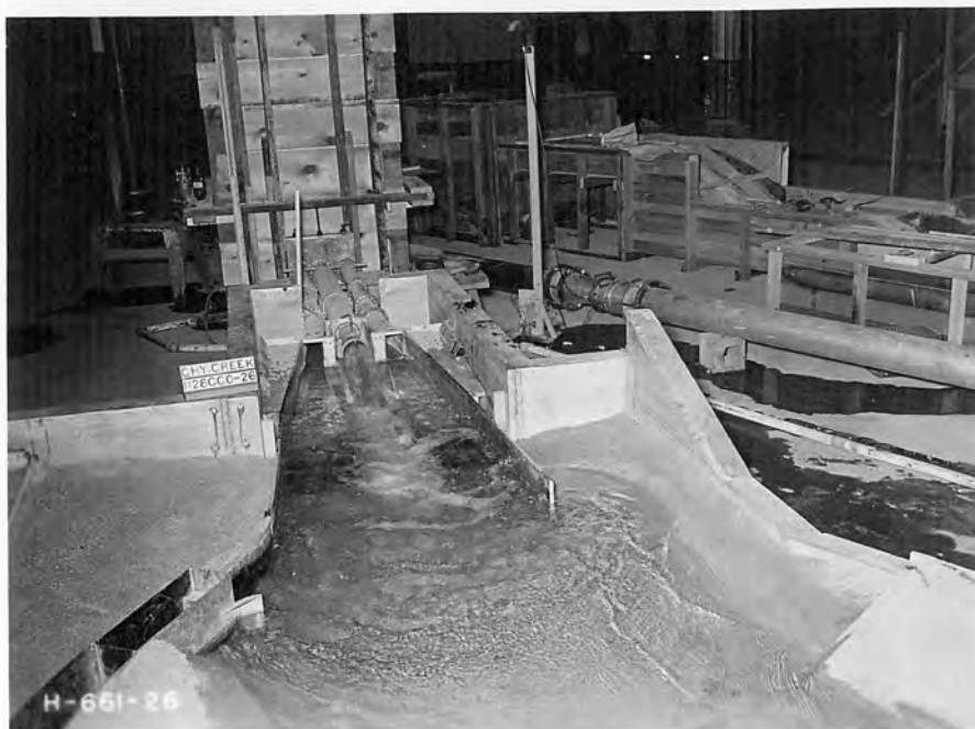
A. Hollow-jet valve discharging 1,500 second-feet. Flow is along centerline of basin.
