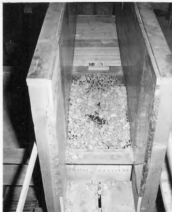
B. Case II - Gravel distribution on grating after discharge of 12 cfs/ft of width and velocity of 12.5 ft/sec
