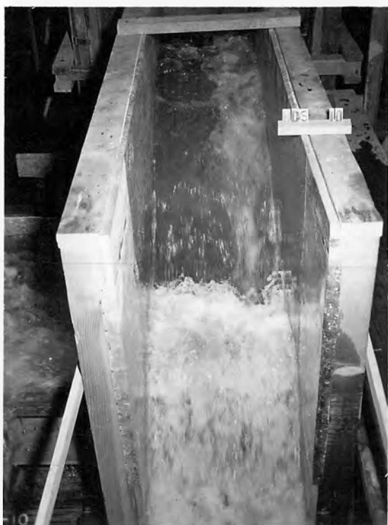
C. Case I - Flow conditions at grating No gravel. Discharge = 65 cfs/ft of width. Velocity = 7.9 ft per sec.
