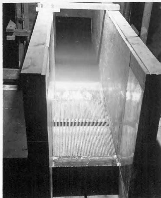
B. Case I - Flow conditions at grating Discharge = 12 cfs per ft of width Velocity = 1.62 ft per sec
