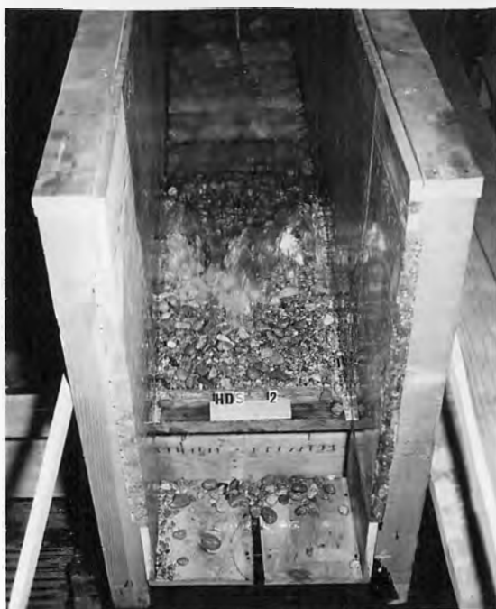
A. Case II - Flow conditions with gravel deposit on grating. Discharge = 12 cfs/ft of width. Velocity = 12.5 ft/sec
