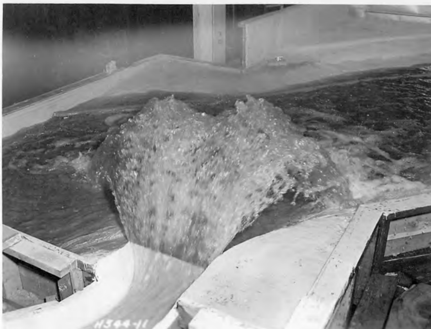
A. Diffuser Bucket Discharging 7,500 Second-feet.
