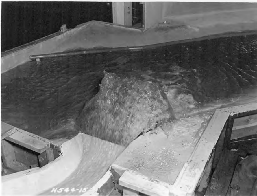
A. Diffuser Bucket Discharging 2,500 Second-feet.
