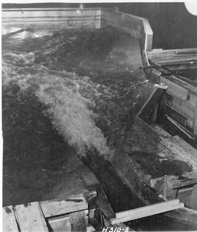
A. Straight Chute Outlet in Operation
