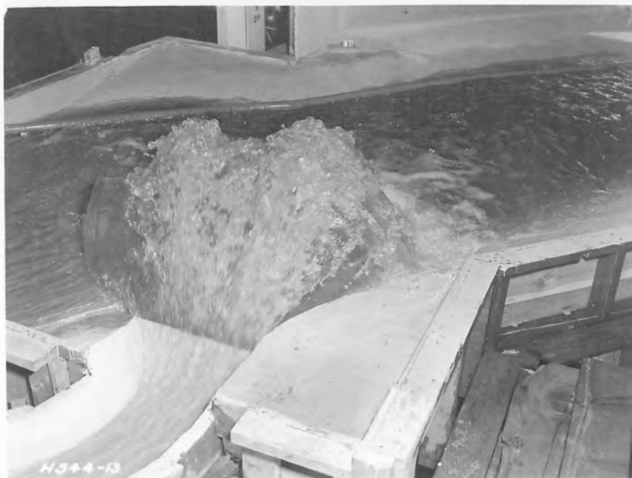
A. Diffuser Bucket Discharging 5,000 Second-feet.
