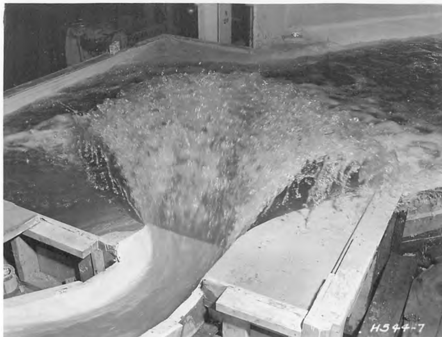
Diffuser Bucket Discharging 12,500 Second-feet.
