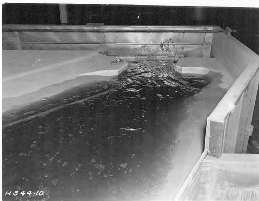
B. Resulting Flow Conditions at the R.R. Bridge.
