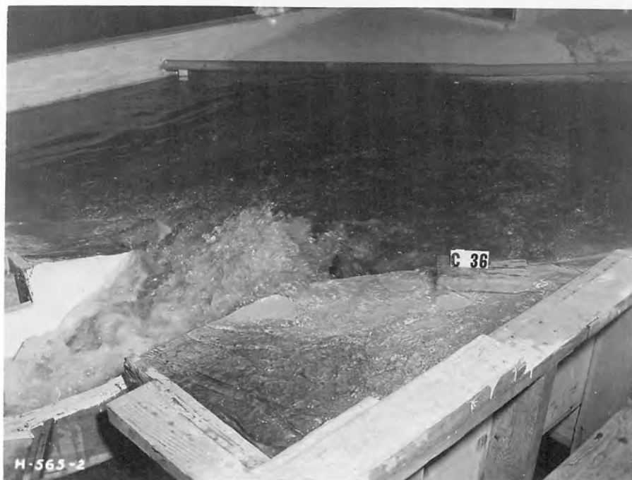
A. Diffuser Bucket Discharging Approx. 2,500 Second-feet. The Jet is approaching the washout stage.
