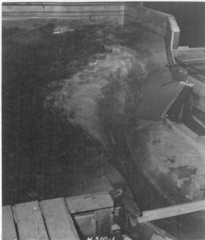
A. Curved Chute Outlet in Operation
