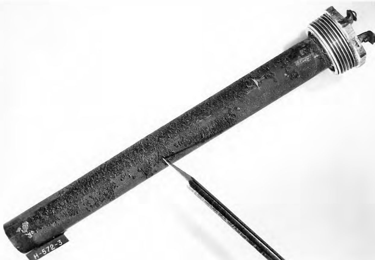
Corrosion of heating element jacket.
