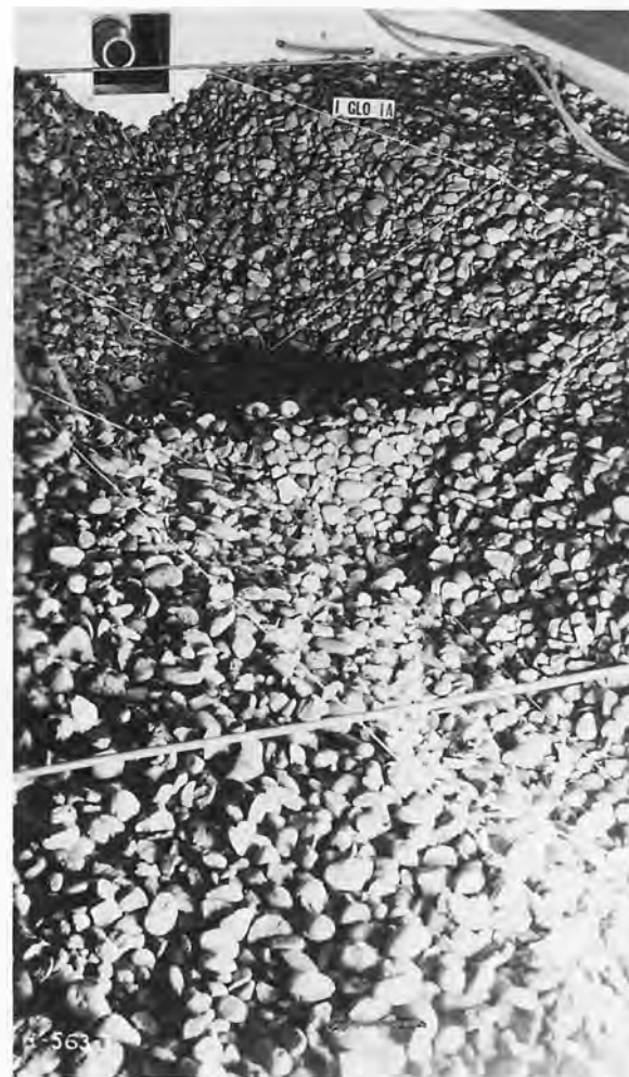
C. Riprap scour after 1 hour. (model)
