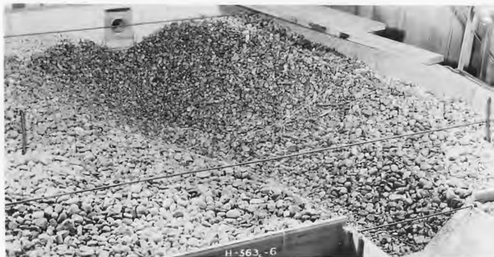
C. Riprap scour after 1 hour run. (model)
