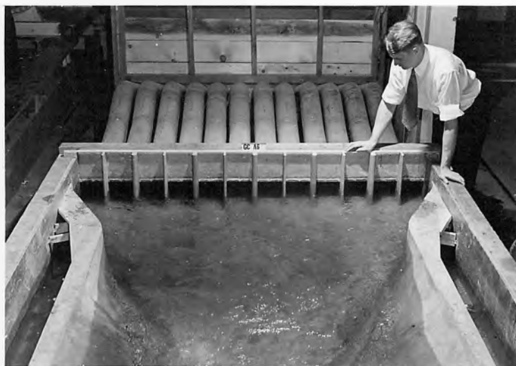
C. Six center units discharging 1,600 cfs. each.
