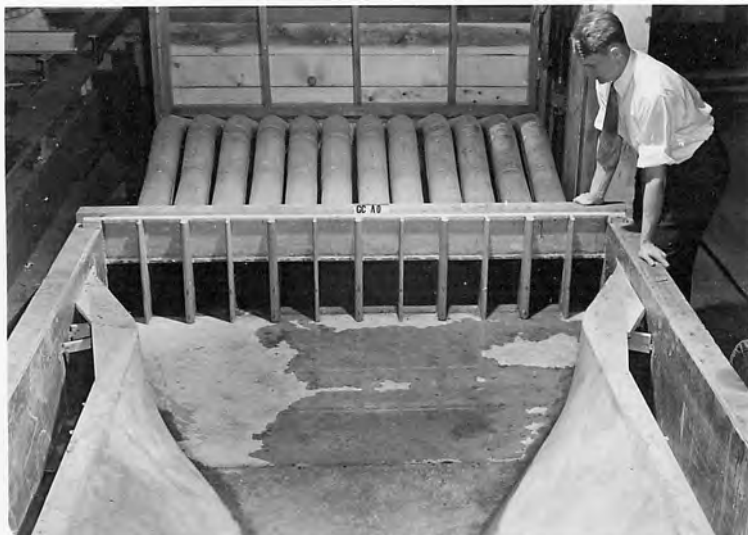
A. Model arrangement showing discharge pipe exists and transition to canal.
