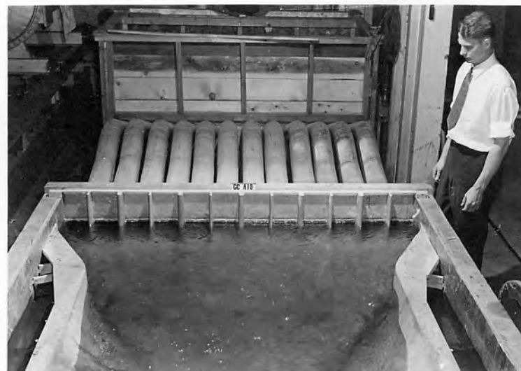
D. Ten center units discharging 1,600 cfs. each
