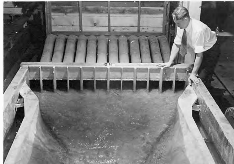
B. Four center units discharging 1,600 cfs. each.
