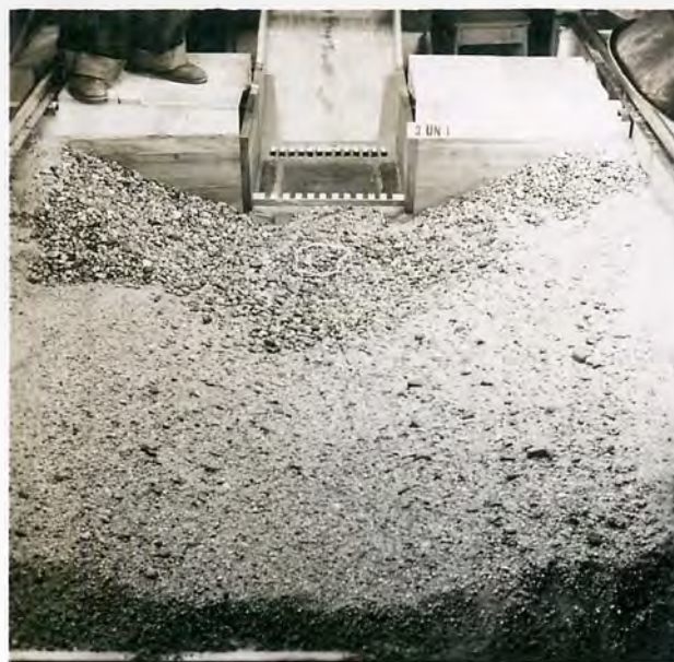
B. Scour caused by flow of 10,000 second-feet (Tail-water El. 3771.0) for 90 minutes-model time.
