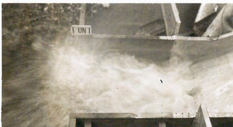
B. Position of hydraulic jump for maximum discharge of 10,000 second-feet. Tailwater El. 3771.0.
