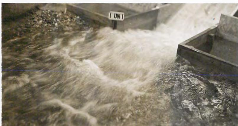
C. Position of secondary wave. Maximum discharge of 10,000 second-feet. Tailwater El. 3771.0.
