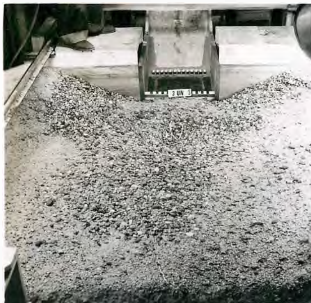
D. Scour caused by flow of 10,000 second-feet (Tail-water El. 3771.0 for 90 minutes, 3769.0 for 90 minutes, 3768.0 for 90 minutes) for 270 minutes-model time.
