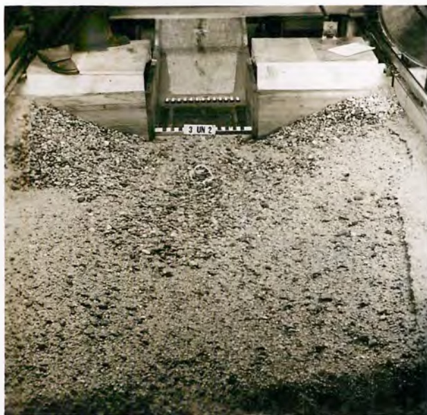
C. Scour caused by flow of 10,000 second-feet (Tail-water El. 3771.0 for 90 minutes, 3769.0 for 90 minutes) for 180 minutes-model time.
