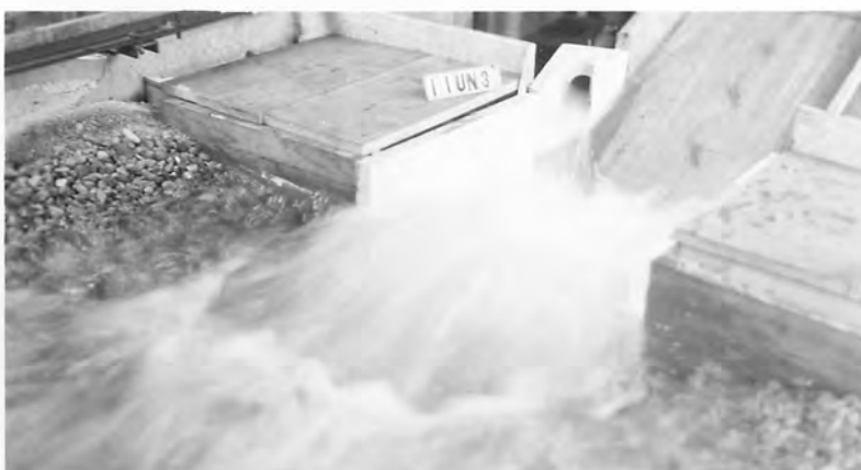
C. Maximum flow through outlet and spillway.
