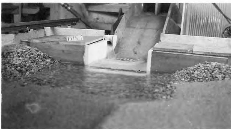
B. Maximum flow through outlet; 625 second-feet.
