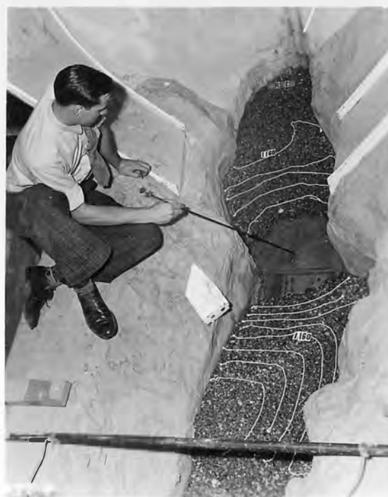
B. Resulting erosion pattern after 60,000 second-feet.
