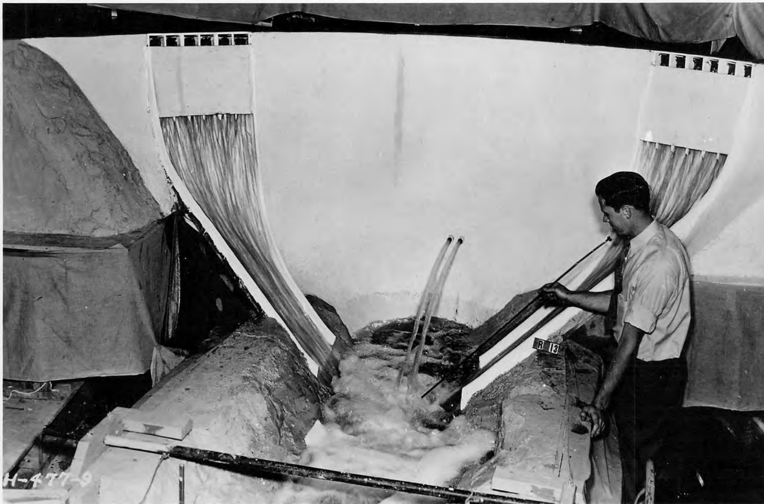
ROSS DAM 1:80 SCALE MODEL--SPILLWAYS DISCHARGING 127,000 SECOND-FEET
