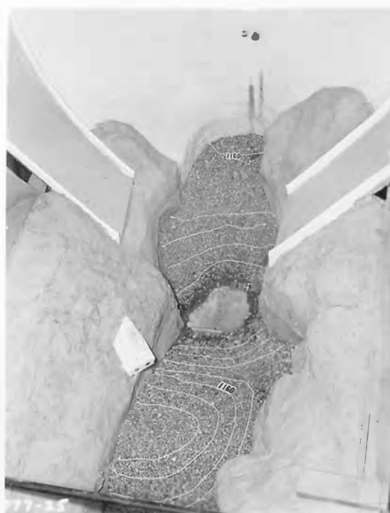
D. Resulting erosion pattern after 60,000 second-feet.
