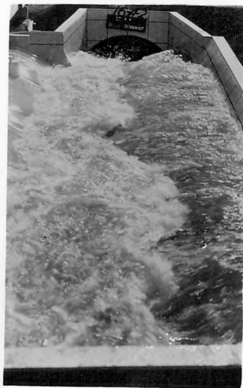
D-DISCHARGE 200,000 SEC. FT MODEL M-3
