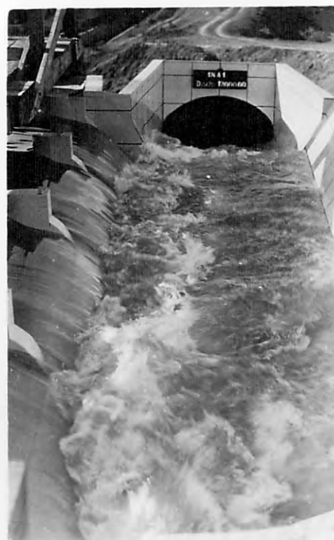
D-DISCHARGE 120,000 SEC. FT. MODEL M-3
