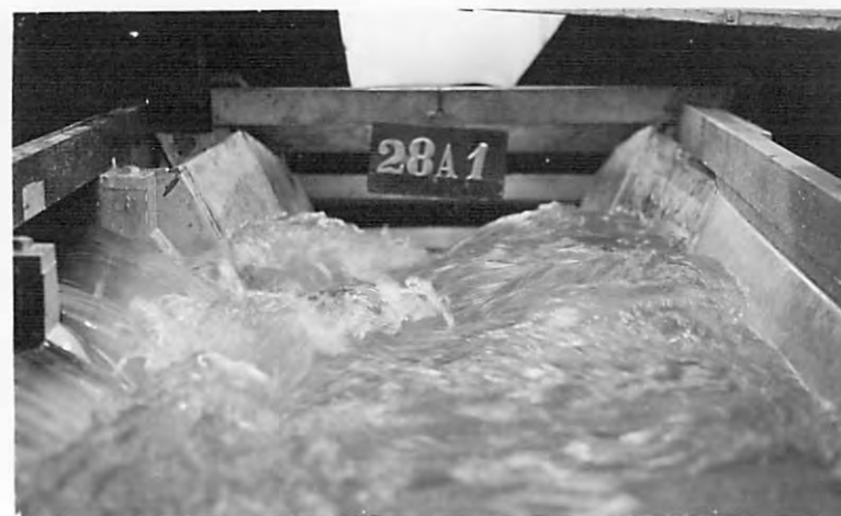
C-DISCHARGE 200,000 SEC. FT. WITH TRANSITION NO 1A AND CROSS WEIR
