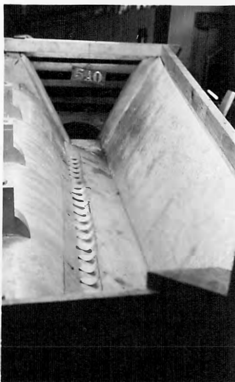
C-MODEL WITH DENTATED BUCKETS ON CREST SIDE OF SLOPING FLOOR
