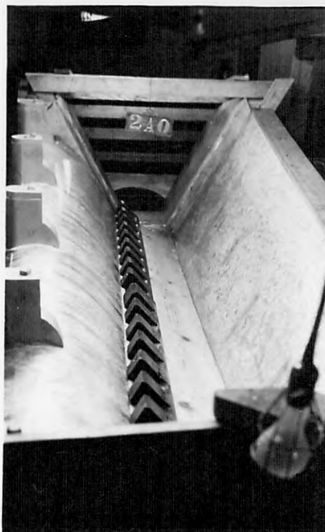
A-MODEL WITH DENTATED DEFLECTORS ON CREST SIDE OF SLOPING FLOOR
