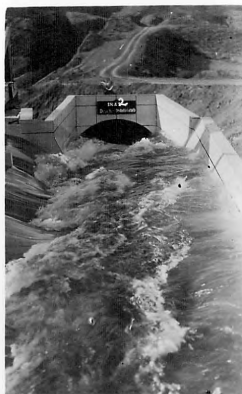
D-DISCHARGE 200,000 SEC FT MODEL M-3
