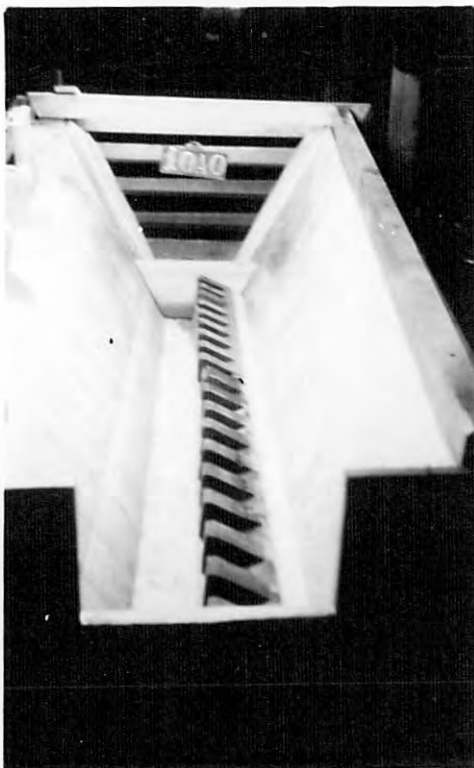
C-MODEL WITH TROUGH IN FRONT HALF OF CHANNEL AND DENTATED SILL
