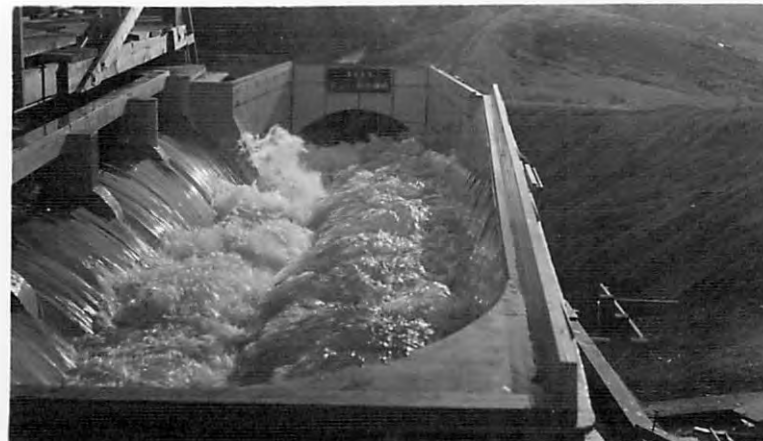
DISCHARGE 200,000 SEC. FT. DISCHARGE 160,000 SEC. FT. CONDITIONS WITH CROSS WEIR AT FINAL DESIGN HEIGHT
