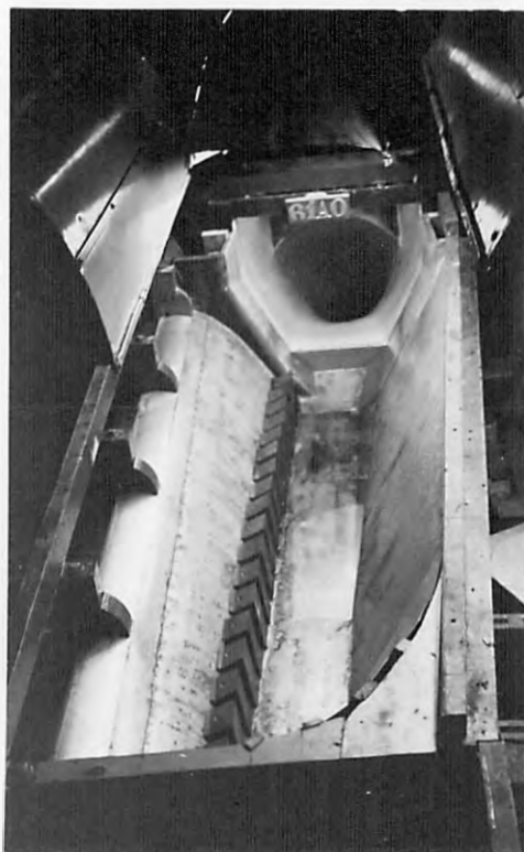
C-MODEL WITH DENTATED BLOCKS DENTATED BLOCKS ON CREST FACE AND CURVED WALL IN UPPER CHANNEL
