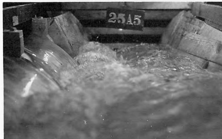
B-DISCHARGE 200,000 SEC. FT 15 FT. CROSS WEIR AT STA. 5+17
