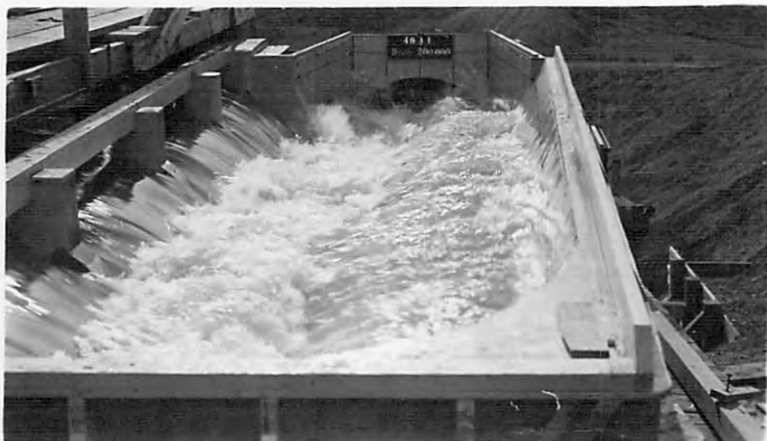
DISCHARGE 200,000 SEC. FT. DISCHARGE 160,000 SEC. FT. CONDITIONS WITH CROSS WEIR AT FINAL DESIGN HEIGHT
