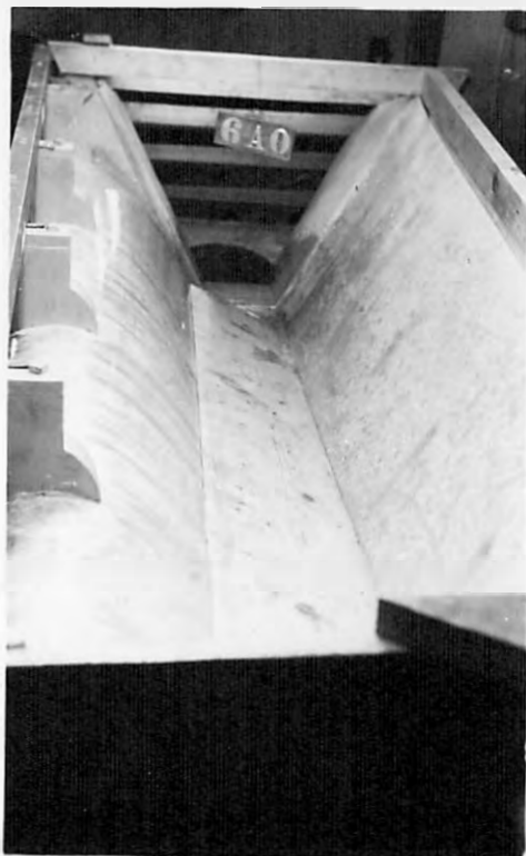
A-MODEL WITH FLOOR SLOPING ACROSS CHANNEL, 96° TO REAR WALL
