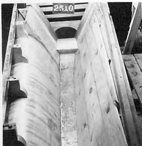
A-MODEL WITH FALSE BACK IN CHANNEL
