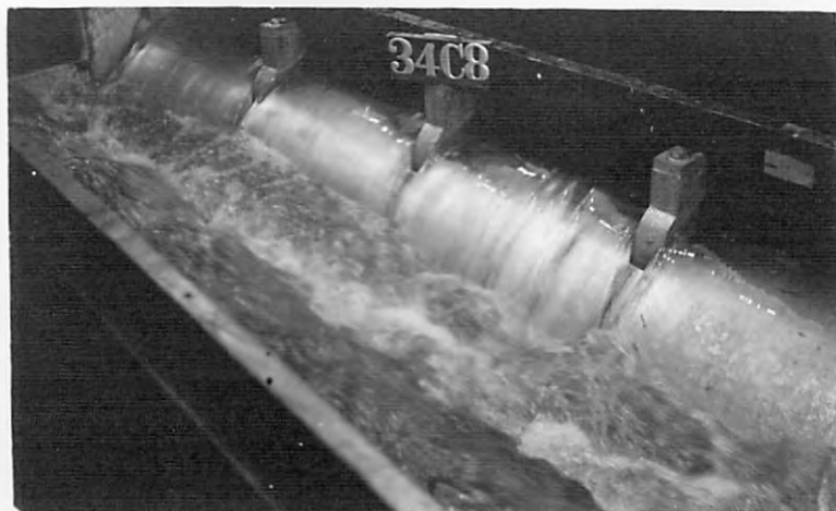
A-DISCHARGE 120,000 SEC FT WITH TRANSITION NO 2
