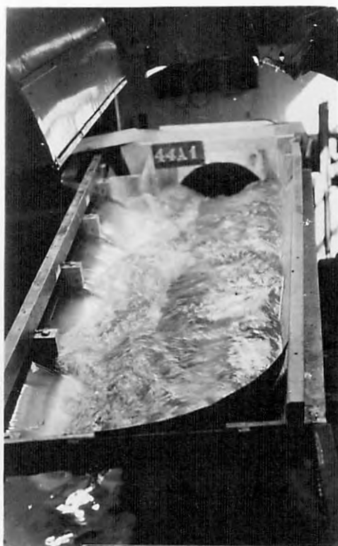
C-DISCHARGE 200,000 SEC FT MODEL C-4
