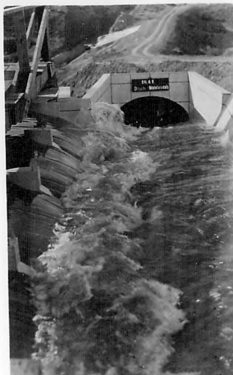
B-DISCHARGE 160,000 SEC. FT. MODEL M-3
