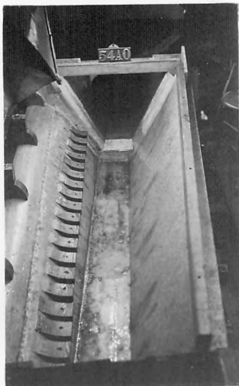
C-MODEL WITH DENTATED DEFLECTORS
