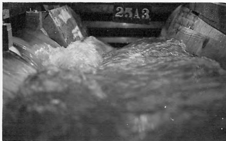
C-DISCHARGE 200,000 SEC. FT 20 FT. CROSS WEIR AT STA. 4+57
