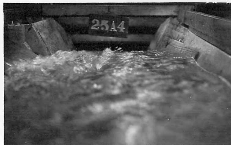
D-DISCHARGE 200,000 SEC. FT 35 FT. CROSS WEIR AT STA. 4+57
