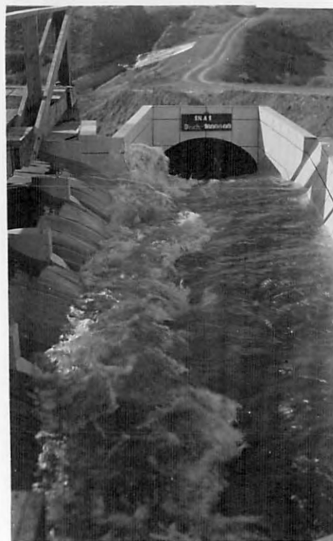
B-DISCHARGE 160,000 SEC. FT. MODEL M-3
