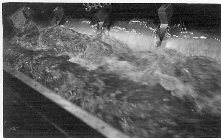
C-DISCHARGE 200,000 SEC FT WITH TRANSITION NO 2
