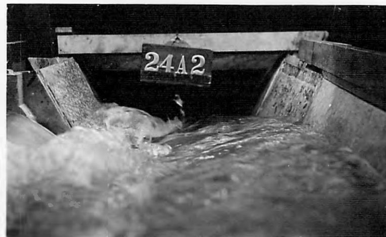
B-20 FT. WEIR AT END OF CHANNEL
