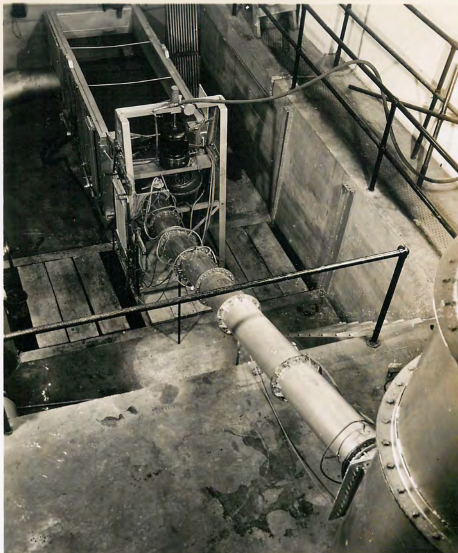
A. View of complete penstock and head tank
