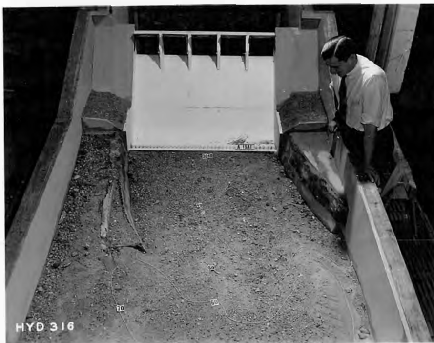
B - Erosion after flow of 50,000 second-feet.
