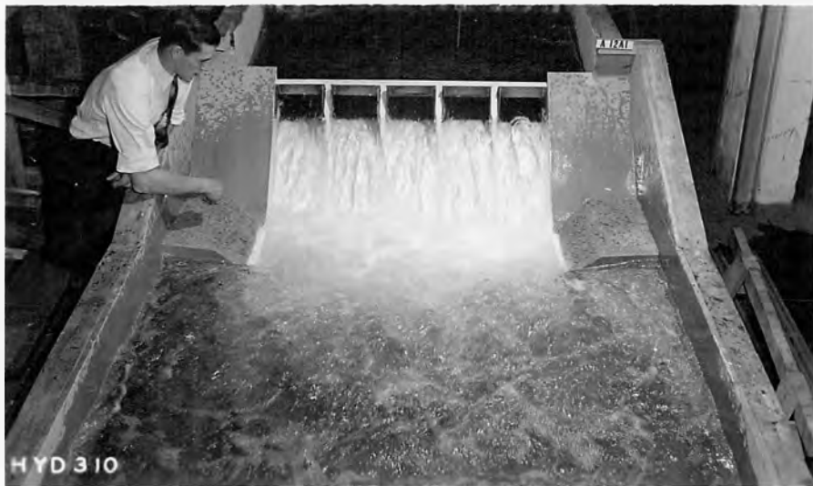
A - Flow of 277,000 second-feet over spillway.
