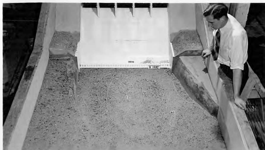
C - Erosion after flow of 277,000 second-feet for 1.5 hours.
