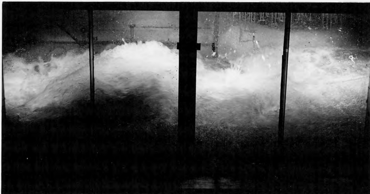
A - Flow of 277,000 second-feet 42 foot radius bucket.
