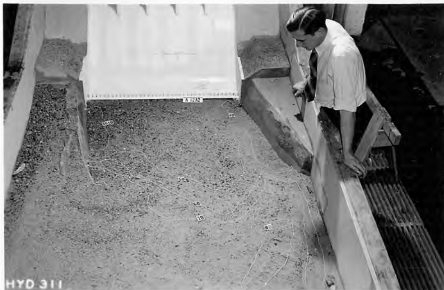
B - Erosion after flow of 277,000 second-feet for 20 minutes.
