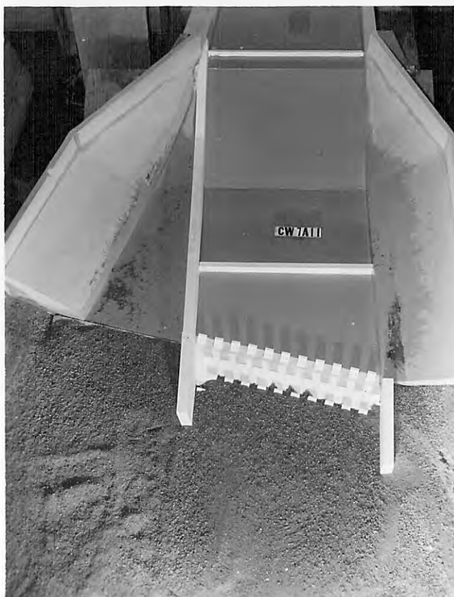
A. Looking upstream. Erosion after 1\frac{1}{2} hours 2000 second-feet flowing.
