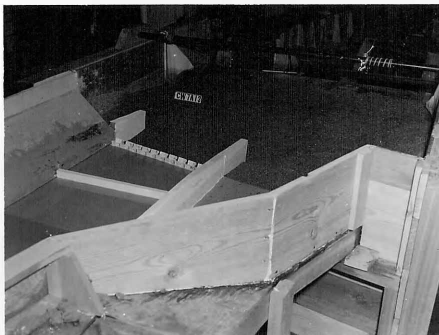
B. Looking downstream. Erosion after 1\frac{1}{2} hours 2000 second-feet flowing.
