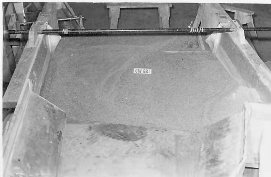
C. Erosion of left side after flow of 1000 second-feet.
