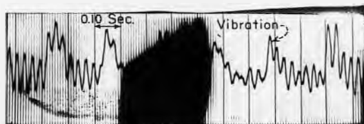
E. VIBRATION DUE TO TAPPING ON GATE
