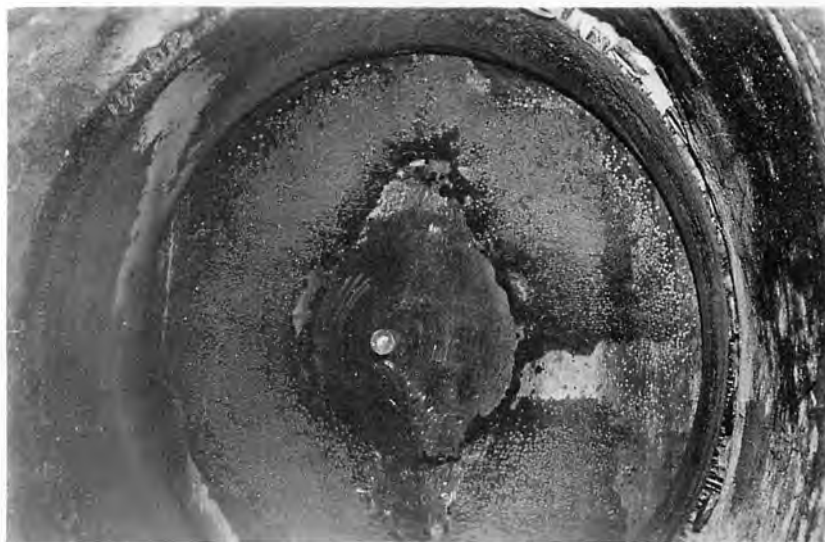
D. Face of needle in west 58-inch valve, showing extensive welding and exposure of air vent pipes downstream from metal liner.
