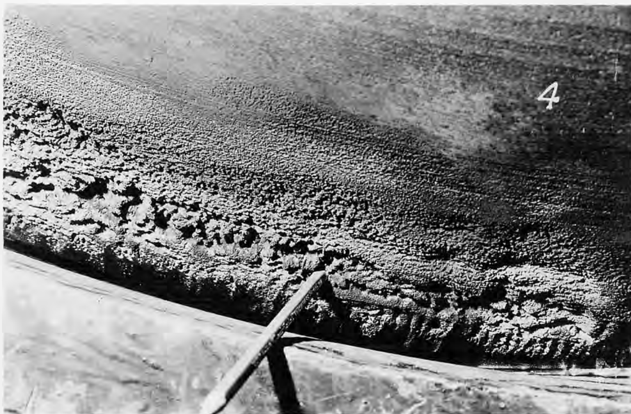
Close-up of Pitted Area 84-INCH CASPER ALCOVA VALVE
