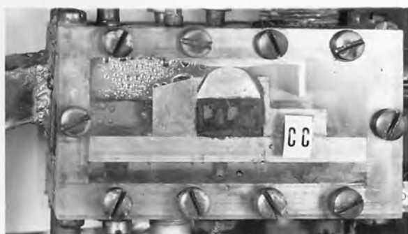
E-Plunger connected and 75 lb. per sq.in. pressure in chambers B and C showing cramped position of rubber.
