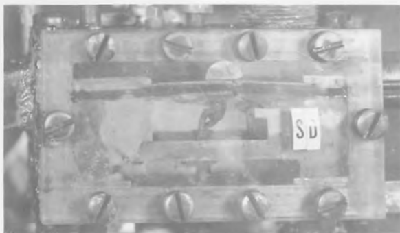
A-Initial test arrangement with 5/16-inch clearance. Sealed at 75 lb. per sq.in. penstock pressure with 45 lb. in chamber B, showing bending of stays with 75 lb. in chamber B.
