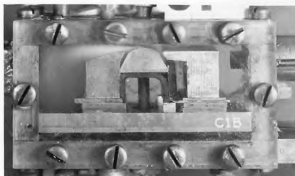
C-Maximum retraction 7/64 inch with 70 lb. pressure in chamber C and vacuum of 10 ft. at A and 13 ft. at D.
