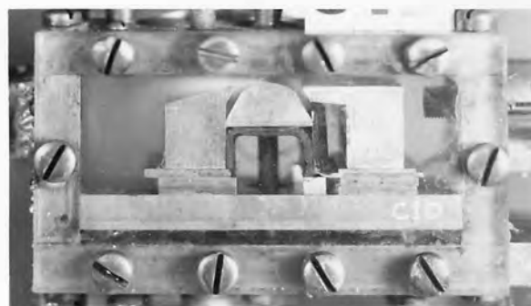
E-Maximum retraction 5/32 inch with 100 lb. pressure in chamber C and zero pressure in chamber B, showing cramped position of rubber.
