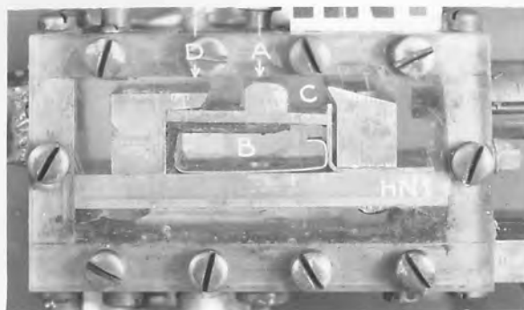
A-Assembled with 1/8-inch shaped rubber vulcanized to the stay but not to the downstream stop bar. Thin metal strip inserted holds rubber against stop bar.
