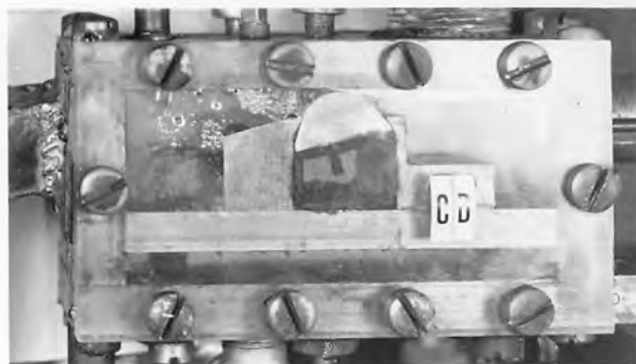
F-Plunger disconnected and seat retracted while penstock pressure was maintained showing rotation of seal bar in direction of flow.
