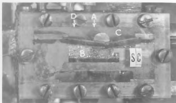
C-Maximum retraction 5/16 inch to the stop with pressure in chambers C 58 lb., in A 45 lb., and in D 42 lb. Maximum vacuum occurred at a gap of 5/32 inch and was 14 ft. and 12 ft. of water at A and at D, respectively.
