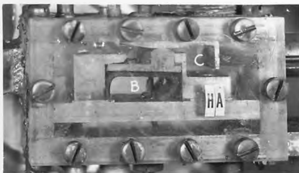
C-Seal bar mounted on 1/8-inch flat rubber strip showing looseness of rubber at hinge with no pressure.
