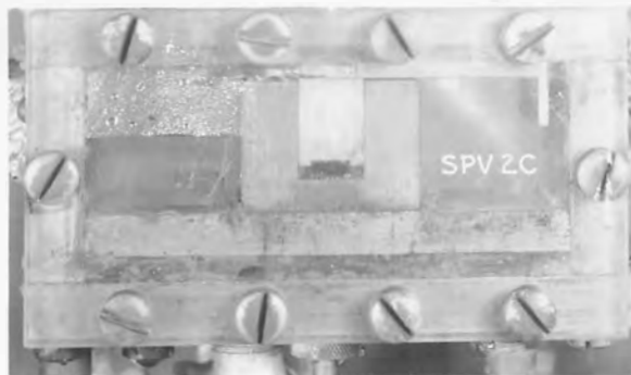
B-Flat of seal bar to the seat. Sliding seat retracted while penstock pressure was maintained at 75 lb. With 1/16 inch in contact, and sealing force reduced to zero the seal was unbroken; to unseal required a downward force on the bar.
