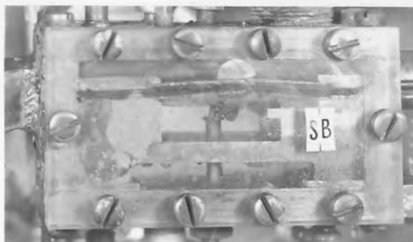
B-Sealed at 19 lb. per sq.in. in chamber C with 12 lb. in chamber B, showing stays nearly returned to flat condition and with 19 lb. in chamber B.
