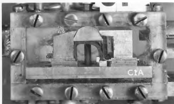
B-Sealed at 75 lb. per sq.in. penstock pressure with 46 lb. in chamber B, showing rubber sealing downstream corner at stop bar.
