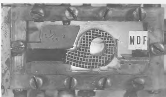
F-Seal bar collapsed to the bottom stop when penstock pressure of 75 lb. flowed wide open; pressure in chamber C was reduced to 44 lb., and pressures in chambers A and D were 42 and 38 lb., respectively.
