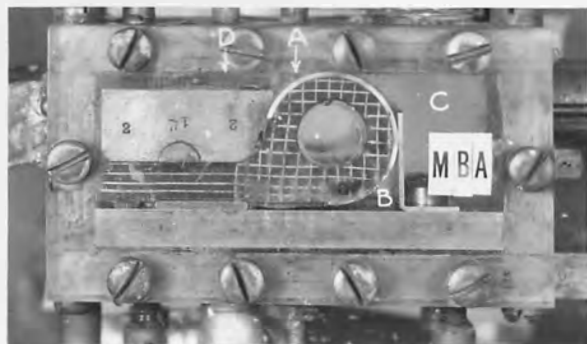
A-Initial assembly with nose of seal bar just touching seat and retraction spring. Brass sheath around rubber not vulcanized.
