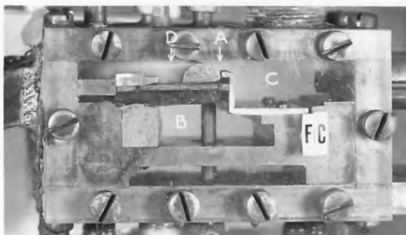
E-Maximum retraction 3/32 inch with 66 lb. per sq.in. in chamber C and 12 ft. of water vacuum in chamber D. Clamp bar is supported in rear by narrow blocks. Upstream stop bar is used as retraction spring in initial tests - plunger is used only as a lower stop. Seal bar collapsed at a penstock pressure of 110 lb.
