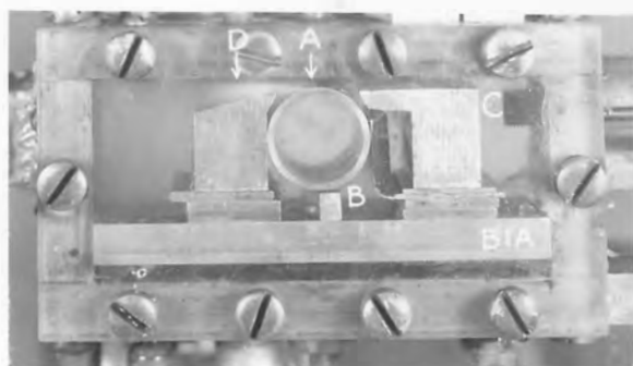
F-Maximum retraction only 5/32 inch with roller seal bar very free. Negative pressure at A was 10 ft. of water.
