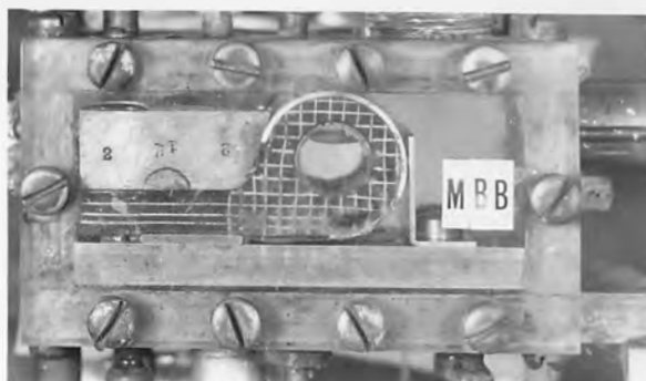
B-Sealed at 75 lb. per sq.in. in chambers C and B, showing the note of the rubber pushed away from the retraction spring. Sealing and breaking pressures were 45 and 39 lb., respectively.
