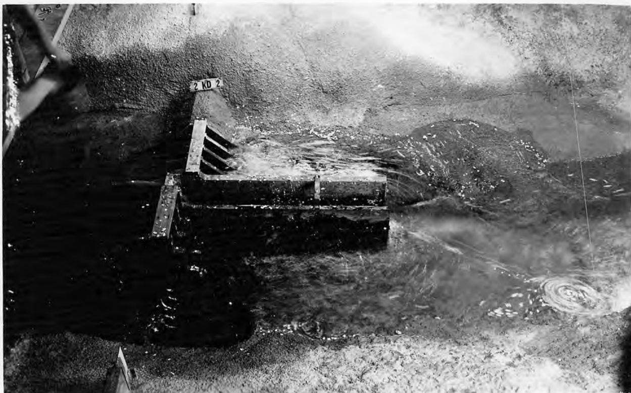
A. Original design - Spillway discharge, 25,000 second-feet; fishway discharge, 300 second-feet; and tailwater elevation 504.20.
