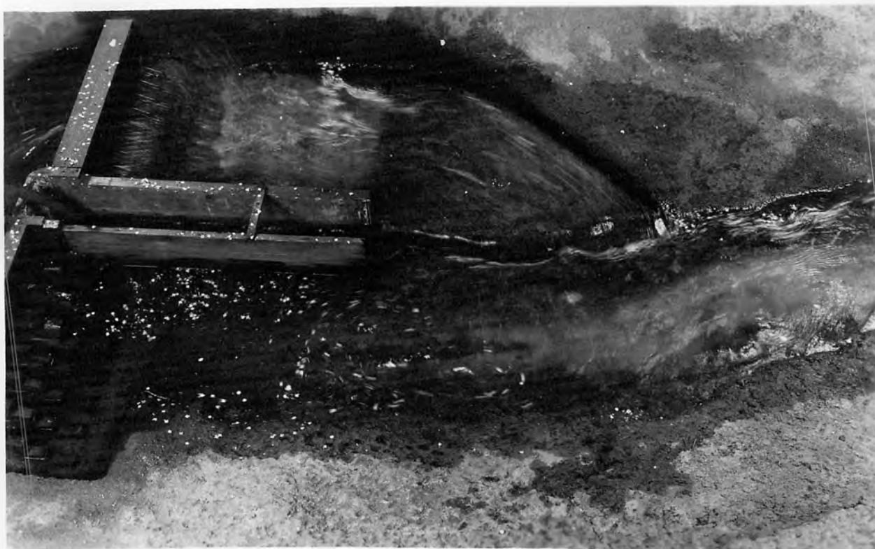
B. Modified design - Spillway discharge, 15,000 second-feet; fishway discharge, 300 second-feet; and tailwater elevation 498.75.
