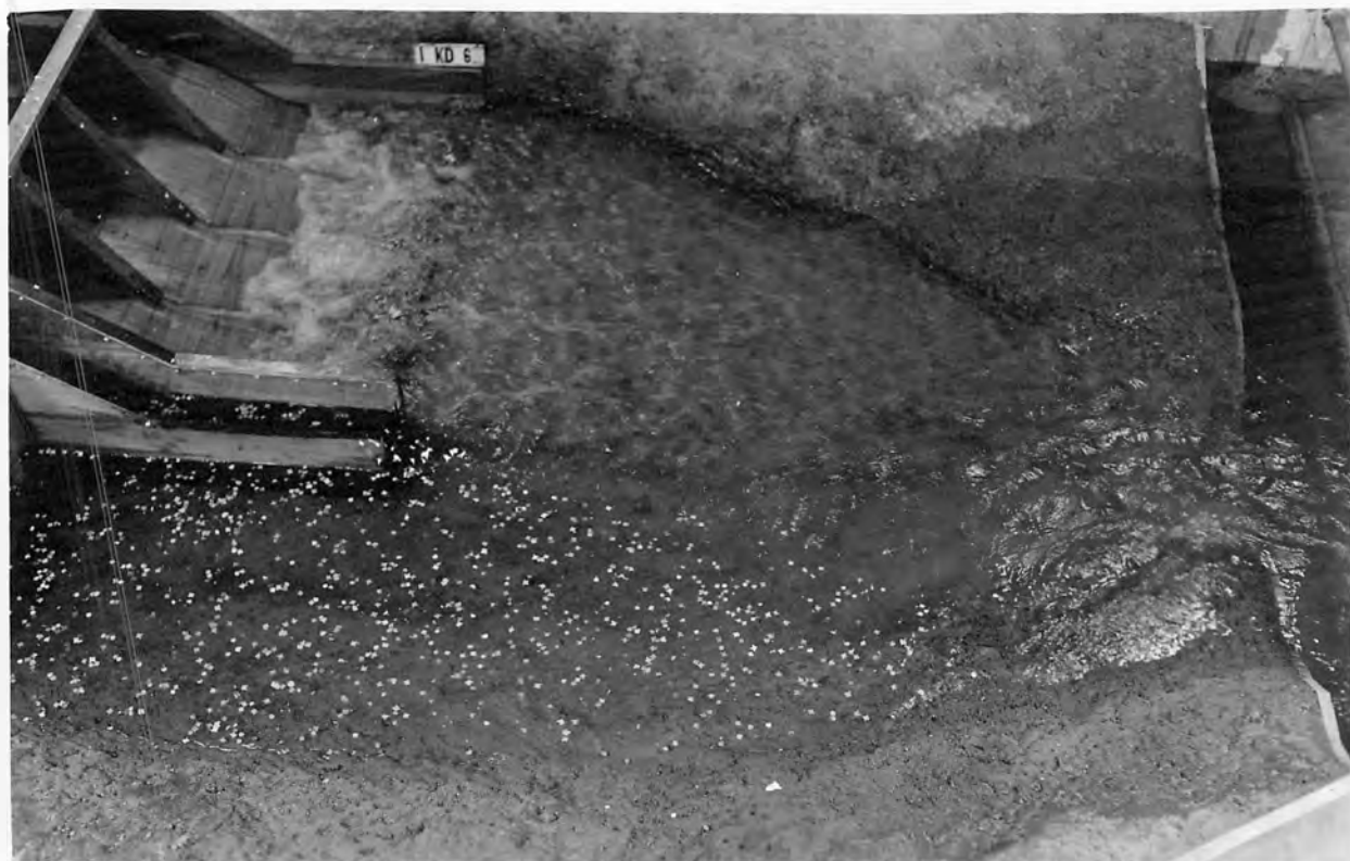
B. Spillway discharge, 50,000 second-feet; no fishway or powerhouse discharge; and tailwater elevation 513.75.
