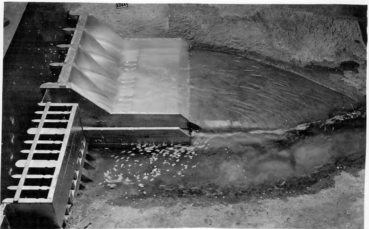
B. Spillway discharge, 15,000 second-feet; fishway discharge, 300 second-feet; no powerhouse discharge; and tailwater elevation 498.75.
