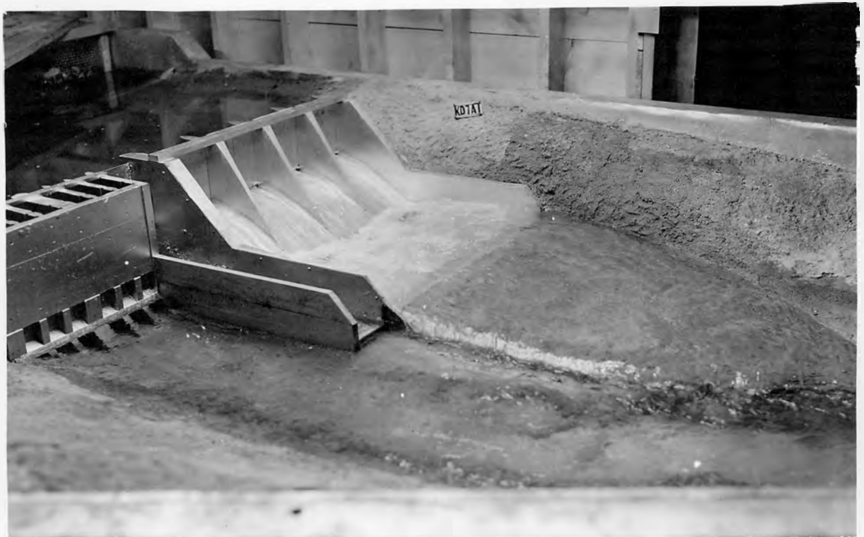
B. Spillway discharge, 50,000 second-feet; fishway discharge, 300 second-feet; no powerhouse discharge; and tailwater elevation 513.60.
