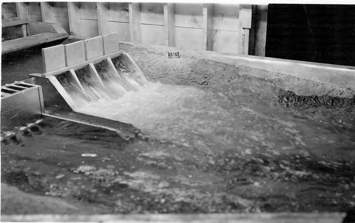
B. Spillway discharge, 250,000 second-feet; no fishway or powerhouse discharge; and tailwater elevation 541.00.
