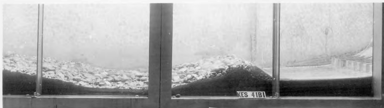
D. Erosion of sand-gravel bed.
