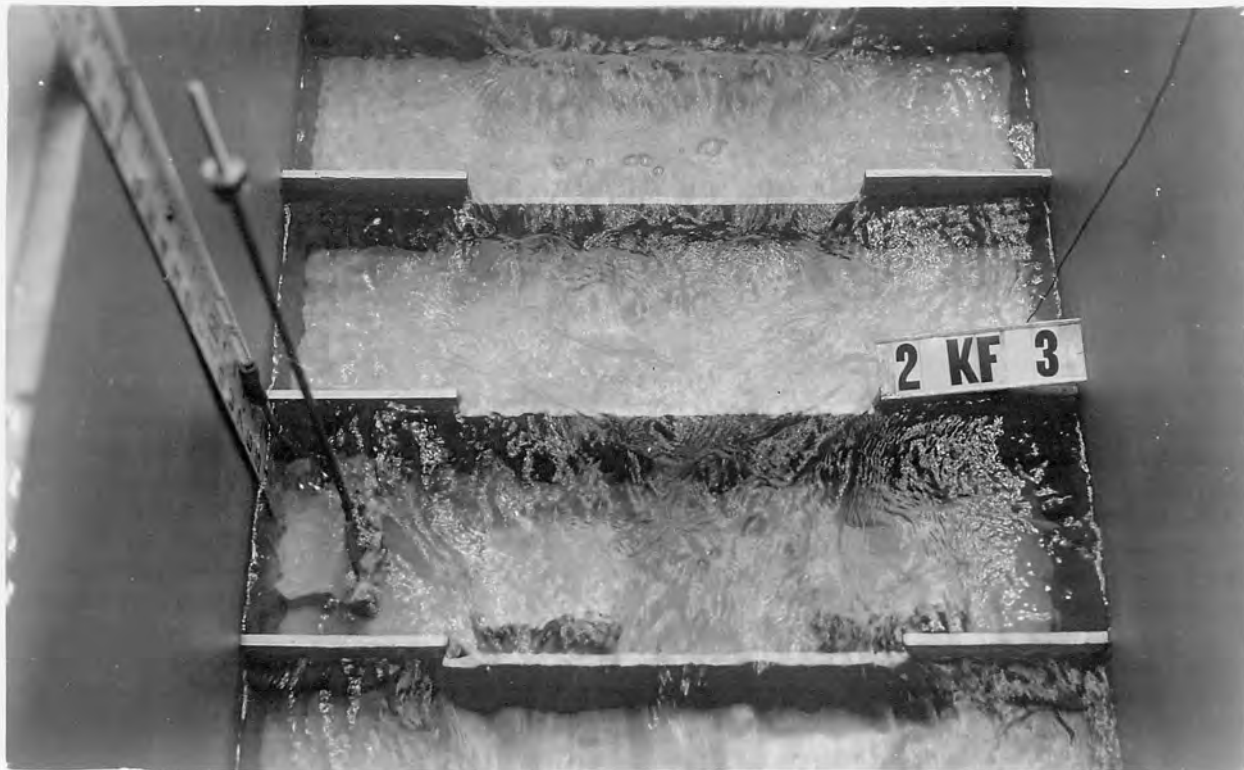
B. Action with flow of 120 second-feet through pools of ladder and 180 second-feet from auxiliary outlet in floor of pool in foreground.
