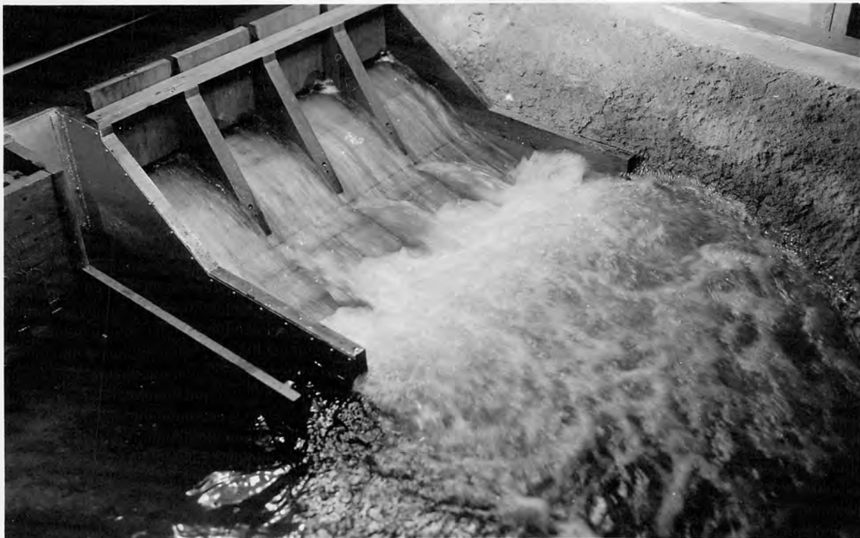
A. Fin downstream from original design of spillway piers.
