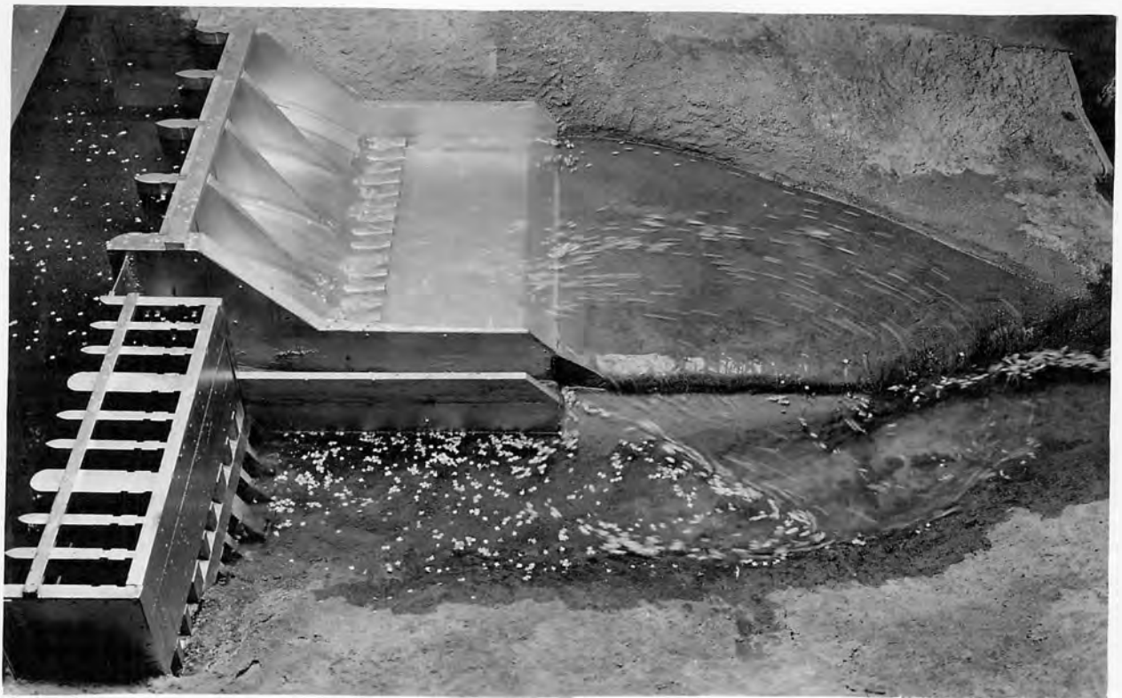
A. Spillway discharge, 3,000 second-feet; fishway discharge, 300 second-feet; no powerhouse discharge; and tailwater elevation 488.00.
