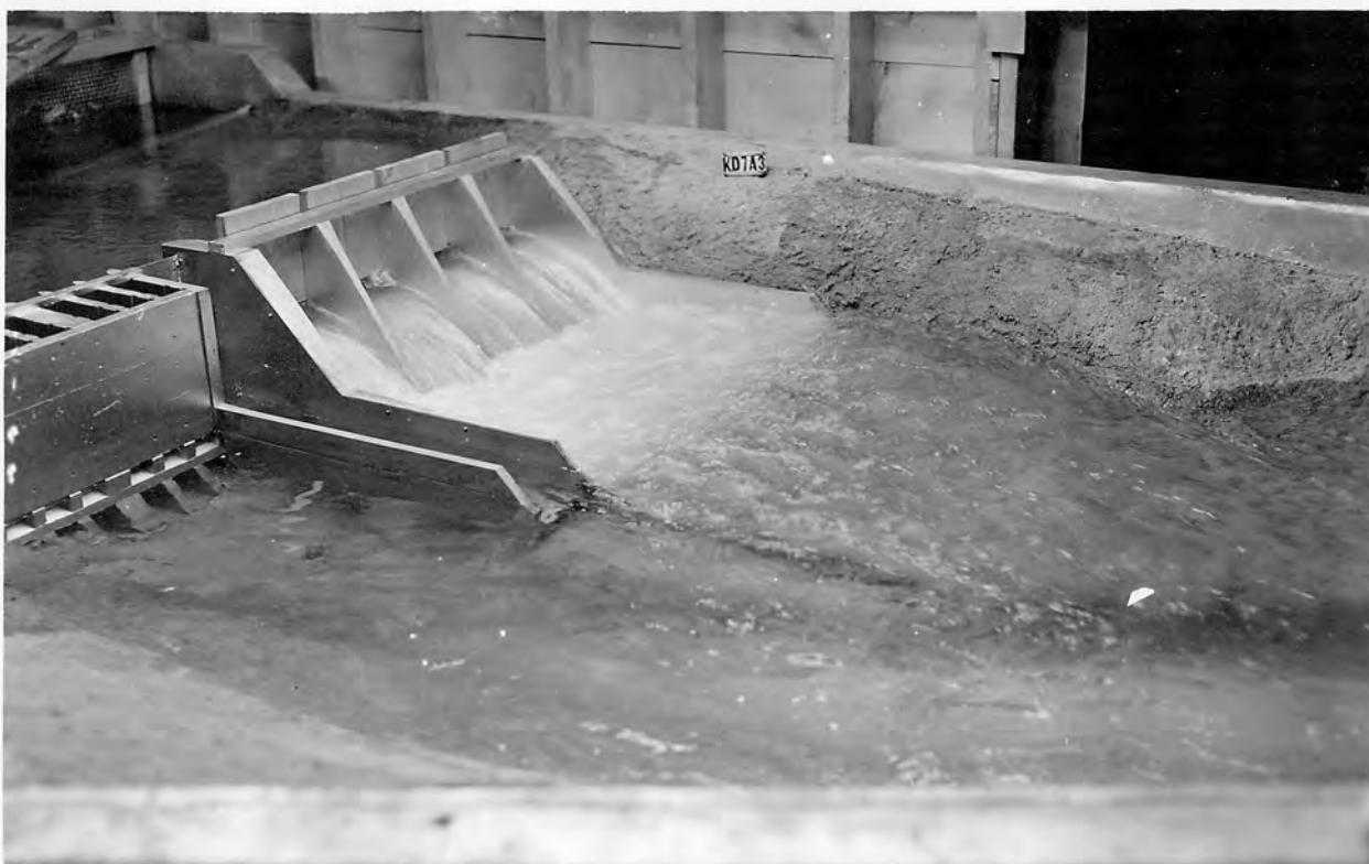
A. Spillway discharge, 100,000 second-feet; no fishway or powerhouse discharge; and tailwater elevation 524.20.
