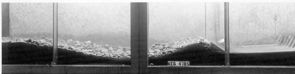
D. Erosion of sand-gravel bed.
