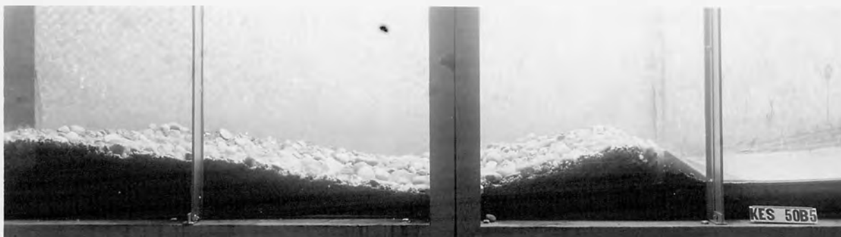
B. Erosion of sand-gravel bed.
