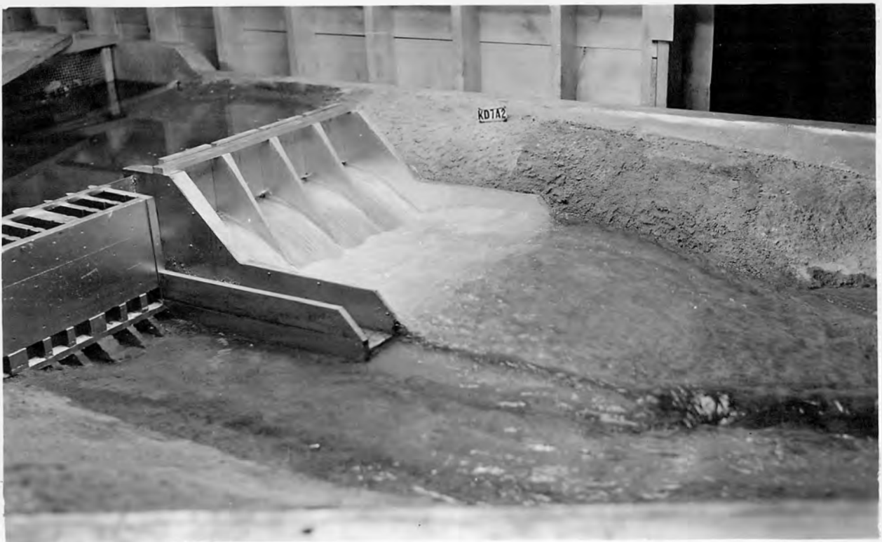
A. Spillway discharge, 25,000 second-feet; fishway discharge, 300 second-feet; no powerhouse discharge; and tailwater elevation 504.20.
