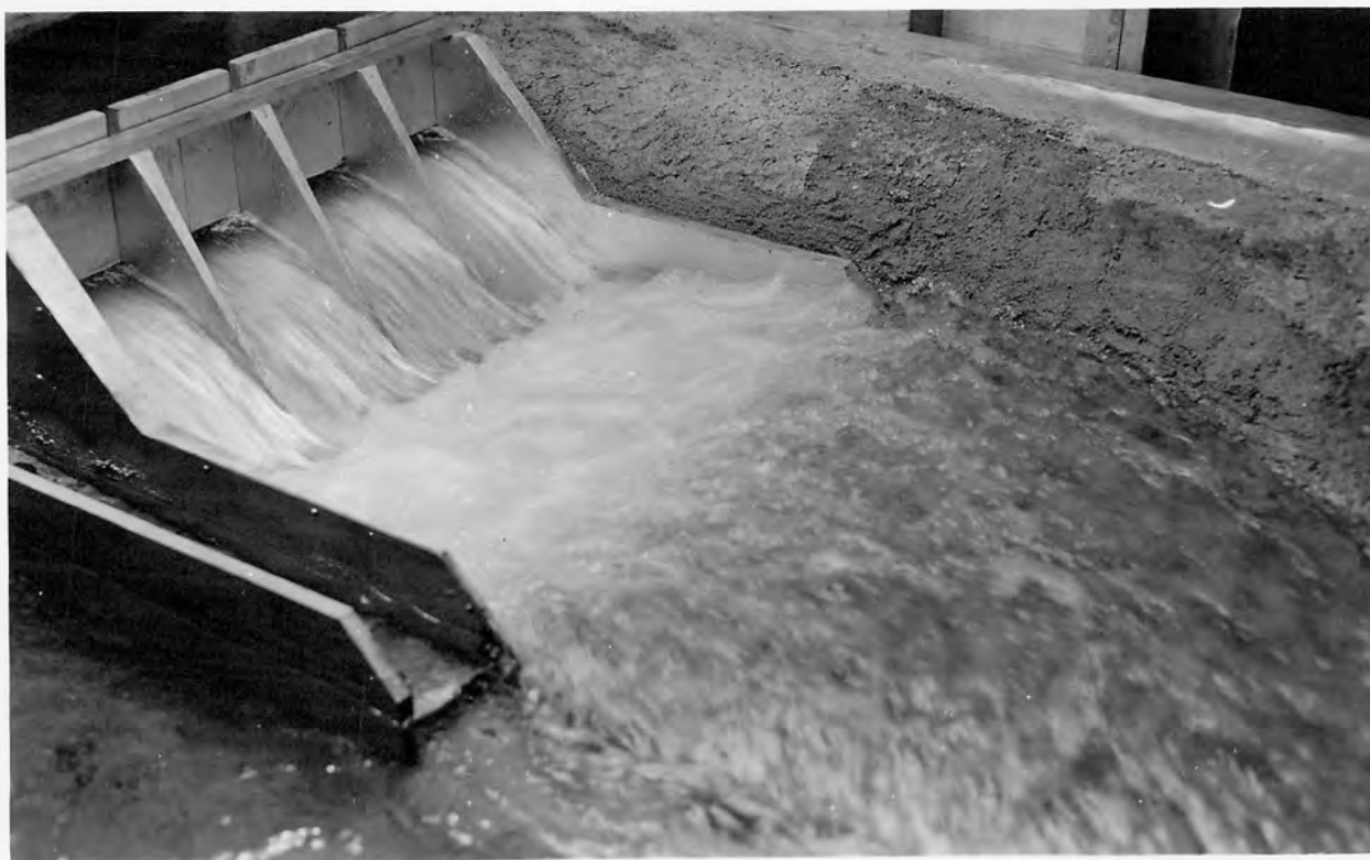
B. Elimination of fin by streamlining of piers.
