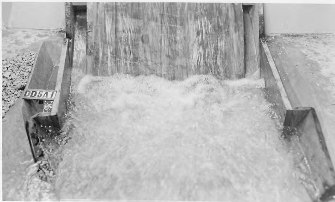
A. FLOW CONDITIONS WITH VERTICAL RETAINING WALLS AT SIDES OF SPILLWAY BUCKET (RECOMMENDED DESIGN).
