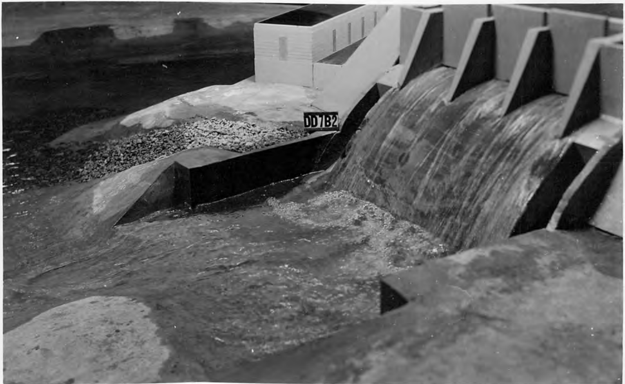
B. POWERHOUSE DISCHARGE 25,000 SECOND-FEET, SPILLWAY DISCHARGE 10,000 SECOND-FEET, ULTIMATE TAILWATER ELEVATION, OUTLET GATES CLOSED.
