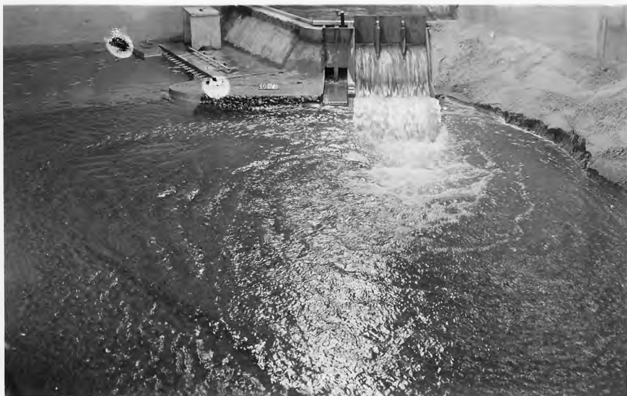
B. FLOW CONDITIONS WITH POWERHOUSE DISCHARGE 25,000 SECOND-FEET, SPILLWAY DISCHARGE 75,000 SECOND-FEET.
