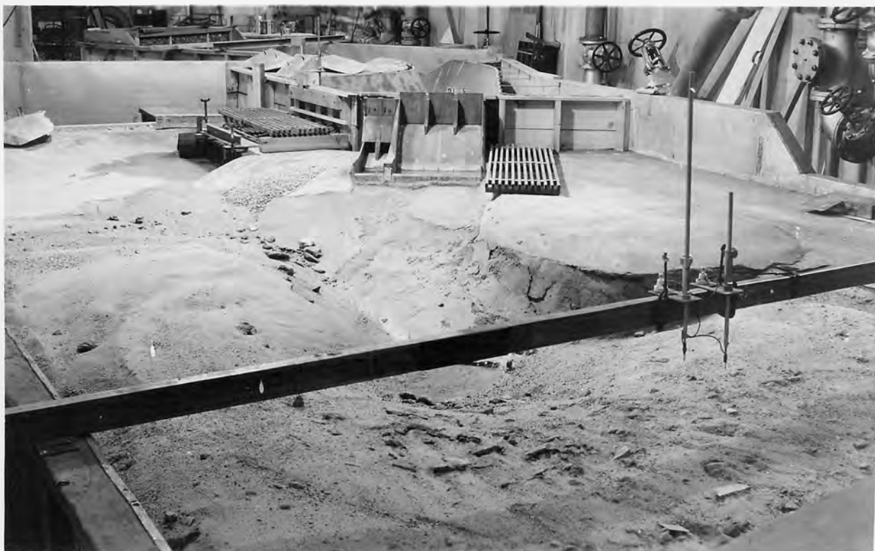
B. SCOUR OF RIVERBED AFTER 10 HOURS OF 250,000 SECOND-FOOT DISCHARGE (POTOTYPE VALUES).
