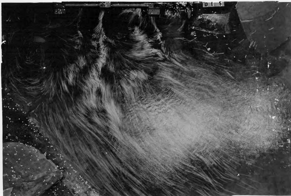
B. FLOW LINES FOR THE RECOMMENDED DESIGN - A SHORT WALL ON THE RIGHT AND RIP-RAP ON THE LEFT BANK.
