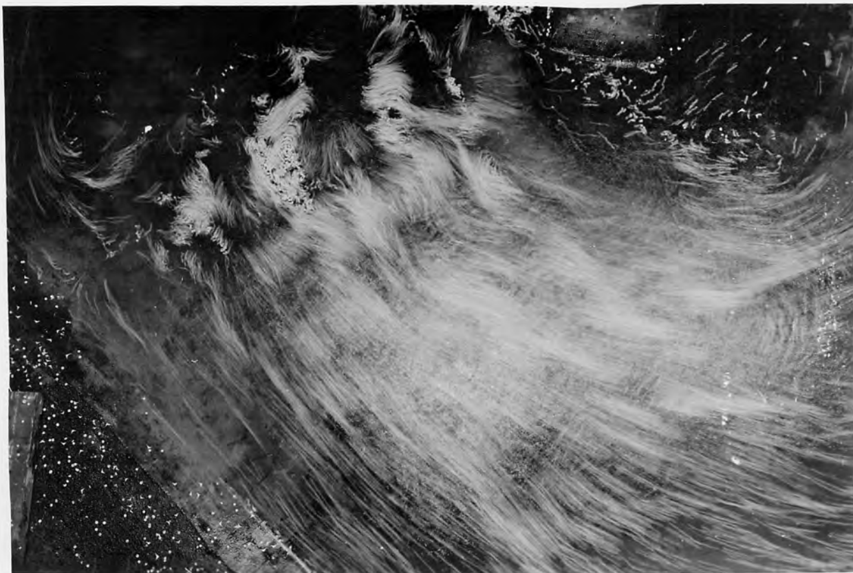
B. FLOW LINES WITH NO WALLS TO RIGHT AND LEFT OF POWERHOUSE.
