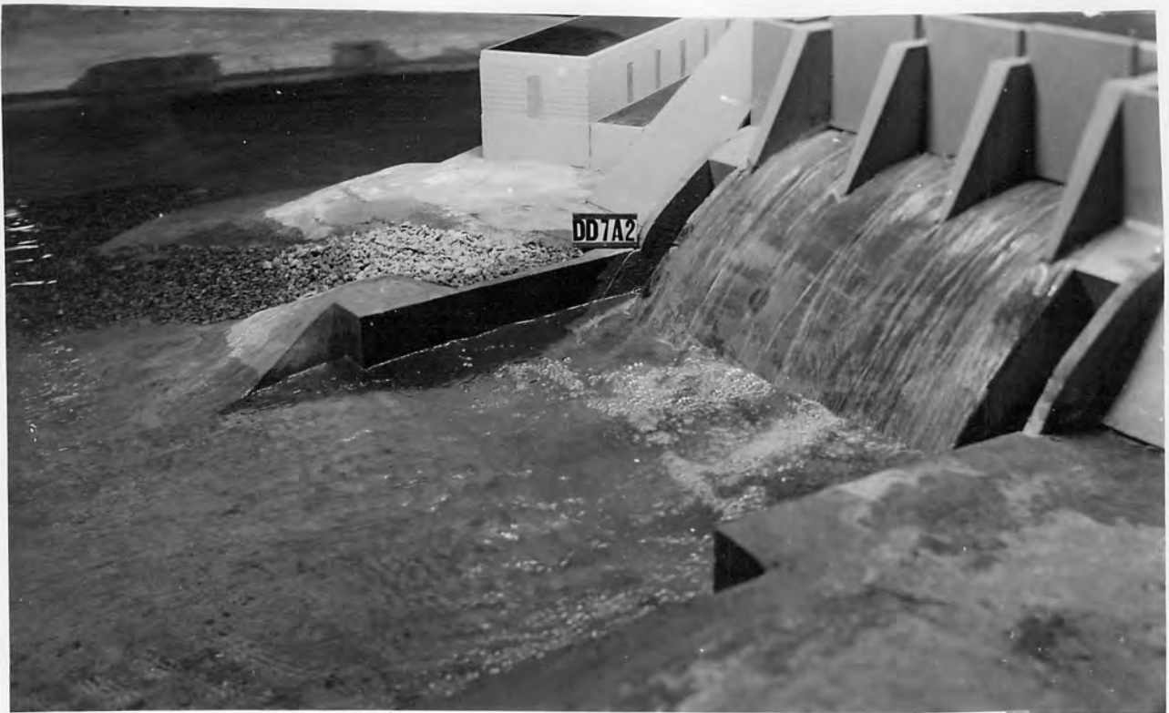
A. POWERHOUSE DISCHARGE 25,000 SECOND-FEET, SPILLWAY DISCHARGE 10,000 SECOND-FEET PRESENT TAILWATER ELEVATION, OUTLET GATES CLOSED.
