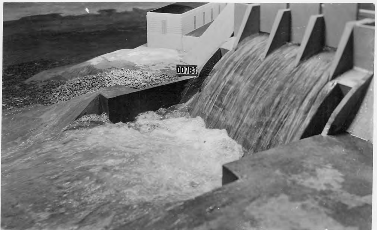
B. POWERHOUSE DISCHARGE 25,000 SECOND-FEET, SPILLWAY DISCHARGE 50,000 SECOND-FEET, ULTIMATE TAILWATER ELEVATION, OUTLET GATES CLOSED.
