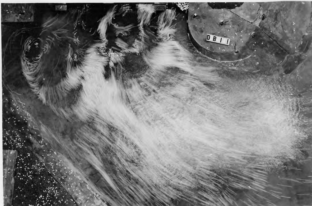
A. FLOW LINES WITH ORIGINAL DESIGN RETAINING WALLS.
