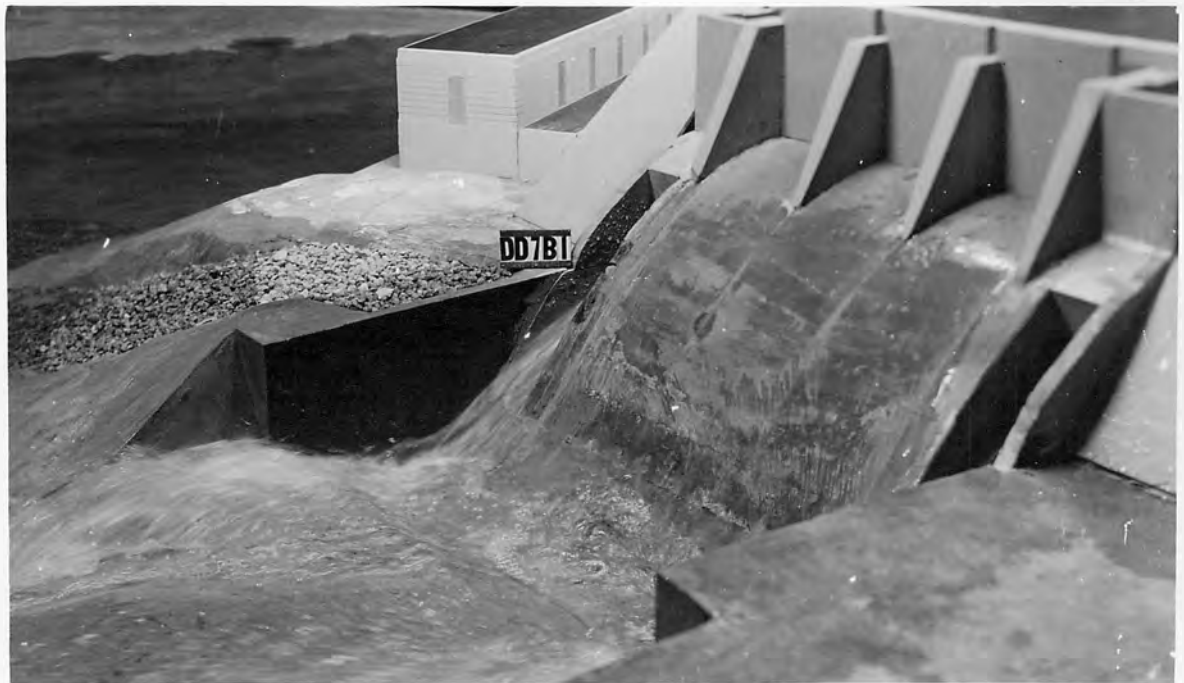
B. POWERHOUSE DISCHARGE 25,000 SECOND-FEET, OUTLET DISCHARGE 10,000 SECOND-FEET EACH, ULTIMATE TAILWATER ELEVATION, SPILLWAY GATES CLOSED.
