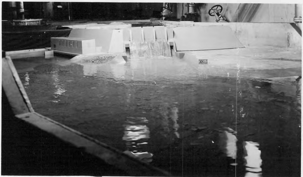
A. POWERHOUSE DISCHARGE 25,000 SECOND-FEET, SPILLWAY DISCHARGE 5,000 SECOND-FEET, PRESENT TAILWATER ELEVATION, OUTLET GATES CLOSED.
