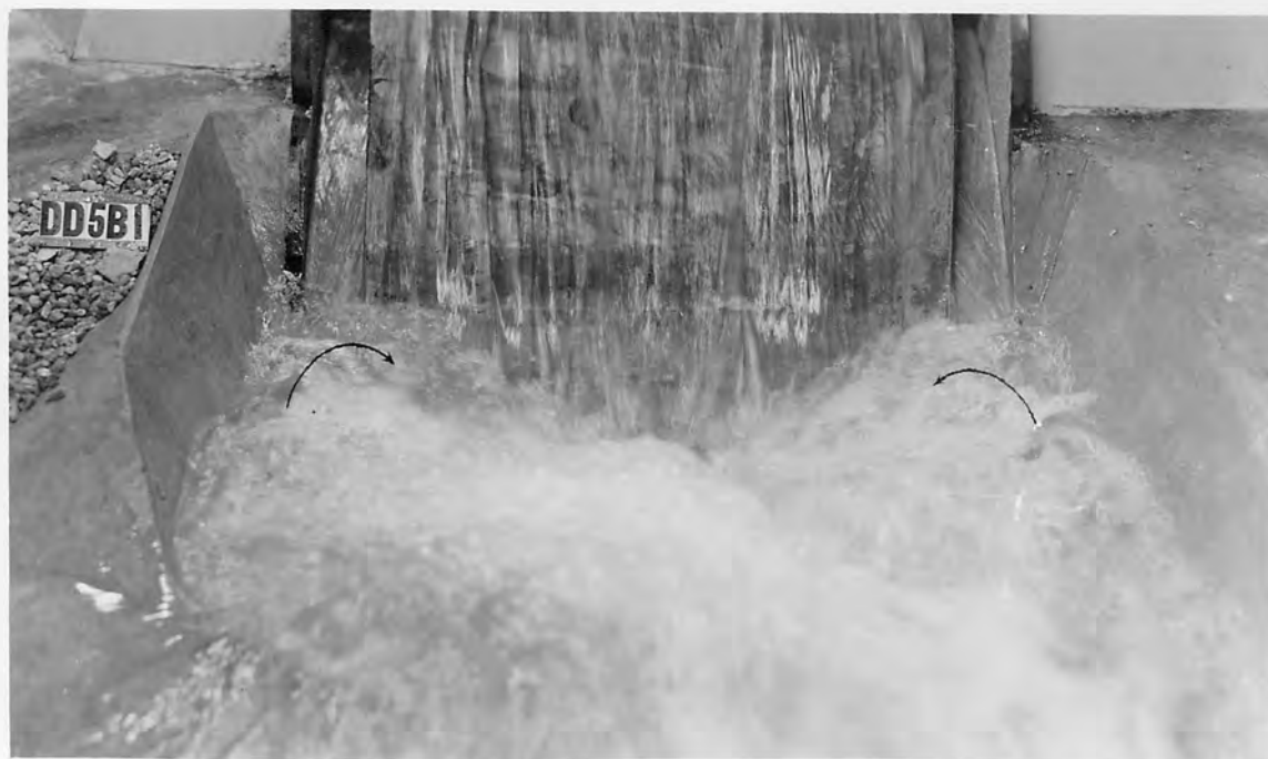
B. FLOW CONDITIONS WITH \frac{1}{2} TO 1 SLOPING RETAINING WALLS AT SIDES OF SPILLWAY BUCKET.
