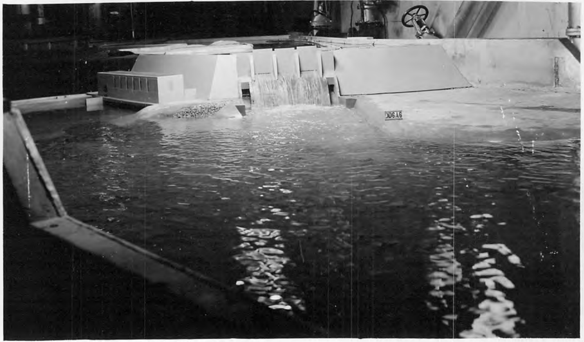
A. POWERHOUSE DISCHARGE 25,000 SECOND-FEET, SPILLWAY DISCHARGE 15,000 SECOND-FEET, PRESENT TAILWATER ELEVATION, OUTLET GATES CLOSED.
