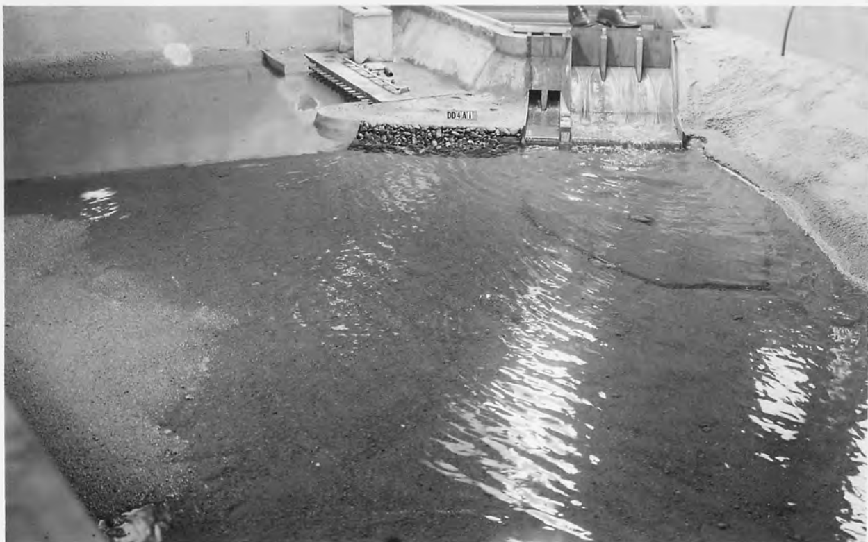
A. FLOW CONDITIONS WITH POWERHOUSE DISCHARGE 25,000 SECOND-FEET, SPILLWAY DISCHARGE 5,000 SECOND-FEET.
