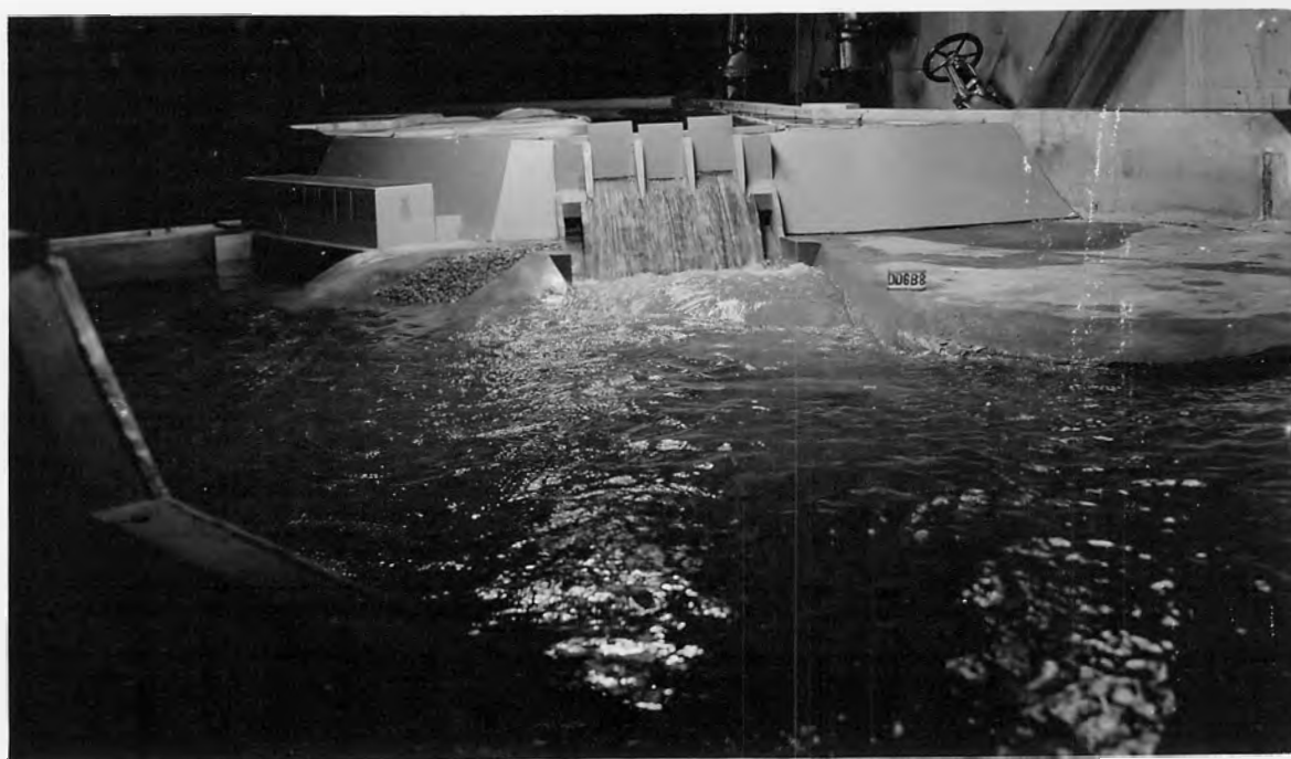
B. POWERHOUSE DISCHARGE 25,000 SECOND-FEET, SPILLWAY DISCHARGE 50,000 SECOND-FEET, ULTIMATE TAILWATER ELEVATION, OUTLET GATES CLOSED.
