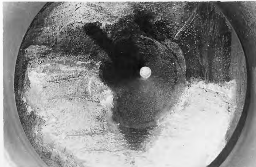
D - Extensive welding on face of needle and leakage through needle - December 17, 1941.
