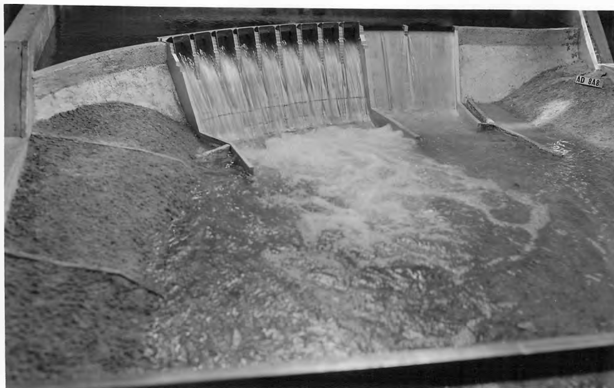
B HORIZONTAL LIP 3 FEET 9 INCHES LONG PLACED AT END OF 4:1 SLOPING APRON.
