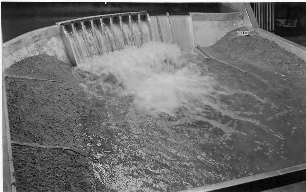
A CONTROLLED SPILLWAY BUCKET EXTENDED UP AT 17 1/2-FOOT RADIUS TO POINT WHERE TANGENT LINE IS 80 DEGREES FROM THE HORIZONTAL.
