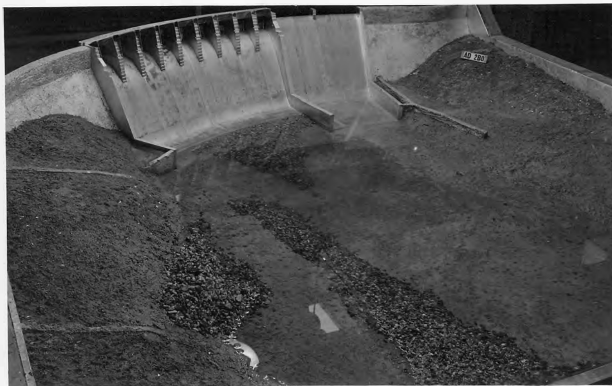
B ROCK JETTY EXTENDED OUT FROM RIGHT BANK, AFTER 3/4 HOUR, 60,000 SECOND- FEET DISCHARGE
