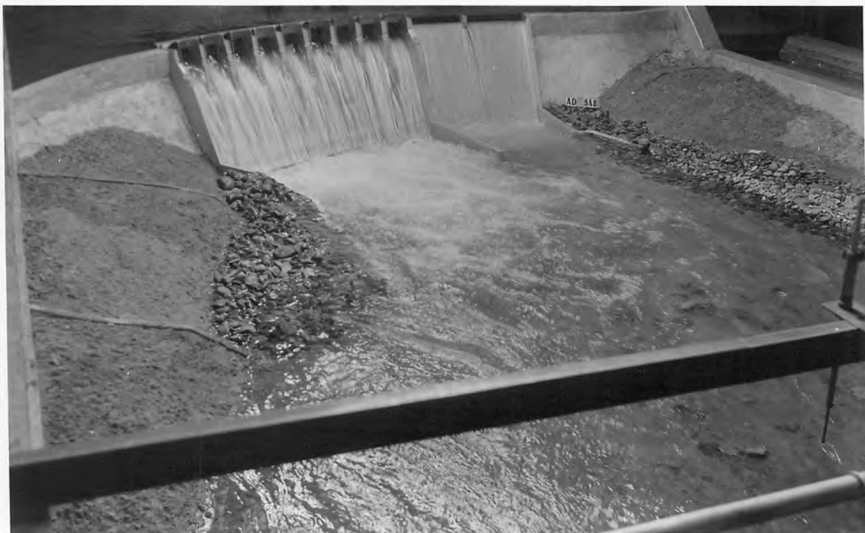
B FLOW CONDITIONS - RESERVOIR ELEVATION 1564.00, DISCHARGES - UNCONTROLLED SPILLWAY 6,000, CONTROLLED SPILLWAY 54,000 SECOND-FEET.
