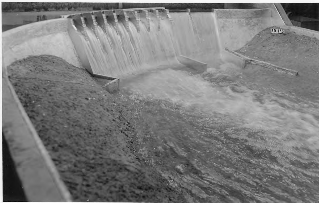
A HYDRAULIC JUMP SWEEPS OFF UNCONTROLLED SPILLWAY APRON WHEN GATES 4 TO 9 ARE OPEN ON CONTROLLED SPILLWAY.
