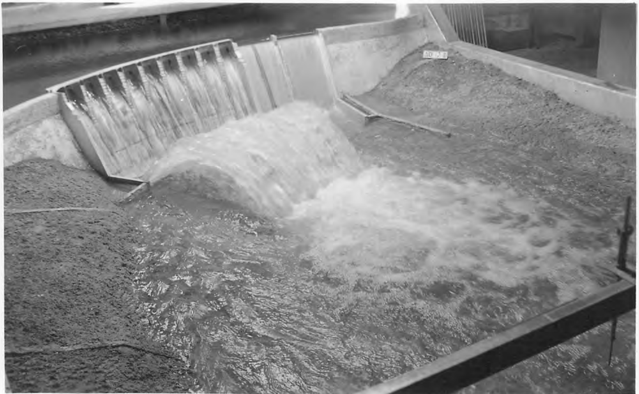
B CONTROLLED SPILLWAY BUCKET EXTENDED UP AT 20-FOOT RADIUS TO POINT WHERE TANGENT LINE IS 60 DEGREES FROM THE HORIZONTAL.
