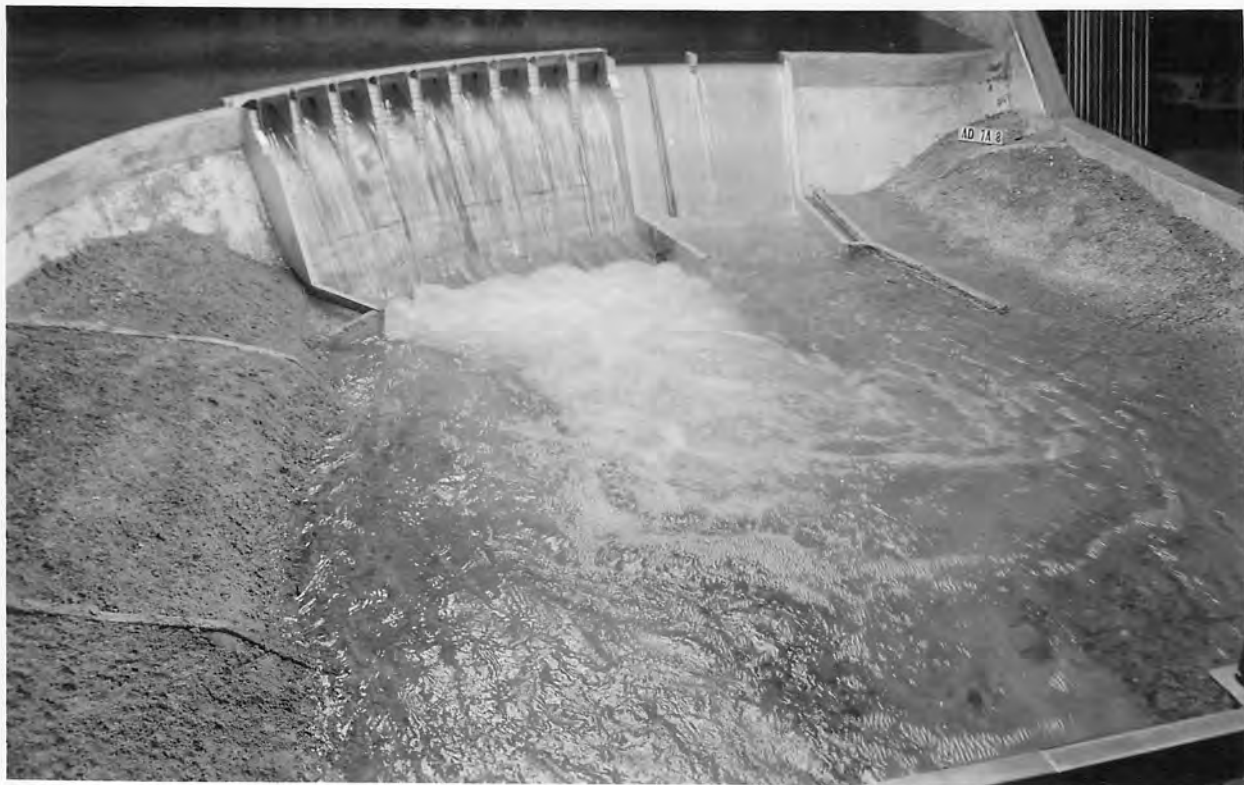
A CONTROLLED SPILLWAY BUCKET REPLACED WITH 4:1 SLOPING APRON TO ELEVATION 1465.26.
