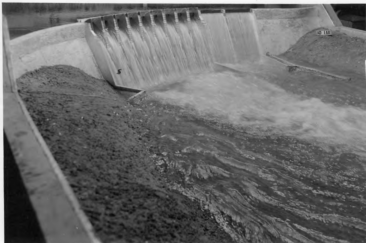
A RESERVOIR ELEVATION 1564.00, DISCHARGES - UNCONTROLLED SPILLWAY 6,000, CONTROLLED SPILLWAY 54.000 SECOND-FEET.
