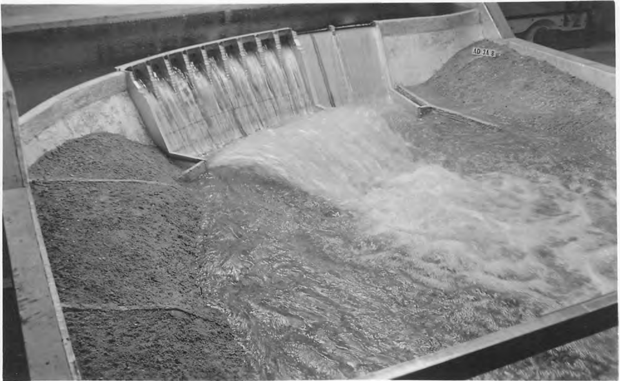
A CONTROLLED SPILLWAY BUCKET EXTENDED UP AT 25-FOOT RADIUS TO POINT WHERE TANGENT LINE IS 45 DEGREES FROM THE HORIZONTAL.
