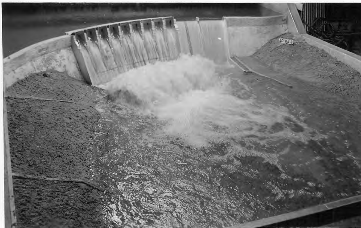
B CONTROLLED SPILLWAY BUCKET EXTENDED UP AT 18 3/4-FOOT RADIUS TO POINT WHERE TANGENT LINE IS 70 DEGREES FROM THE HORIZONTAL.
