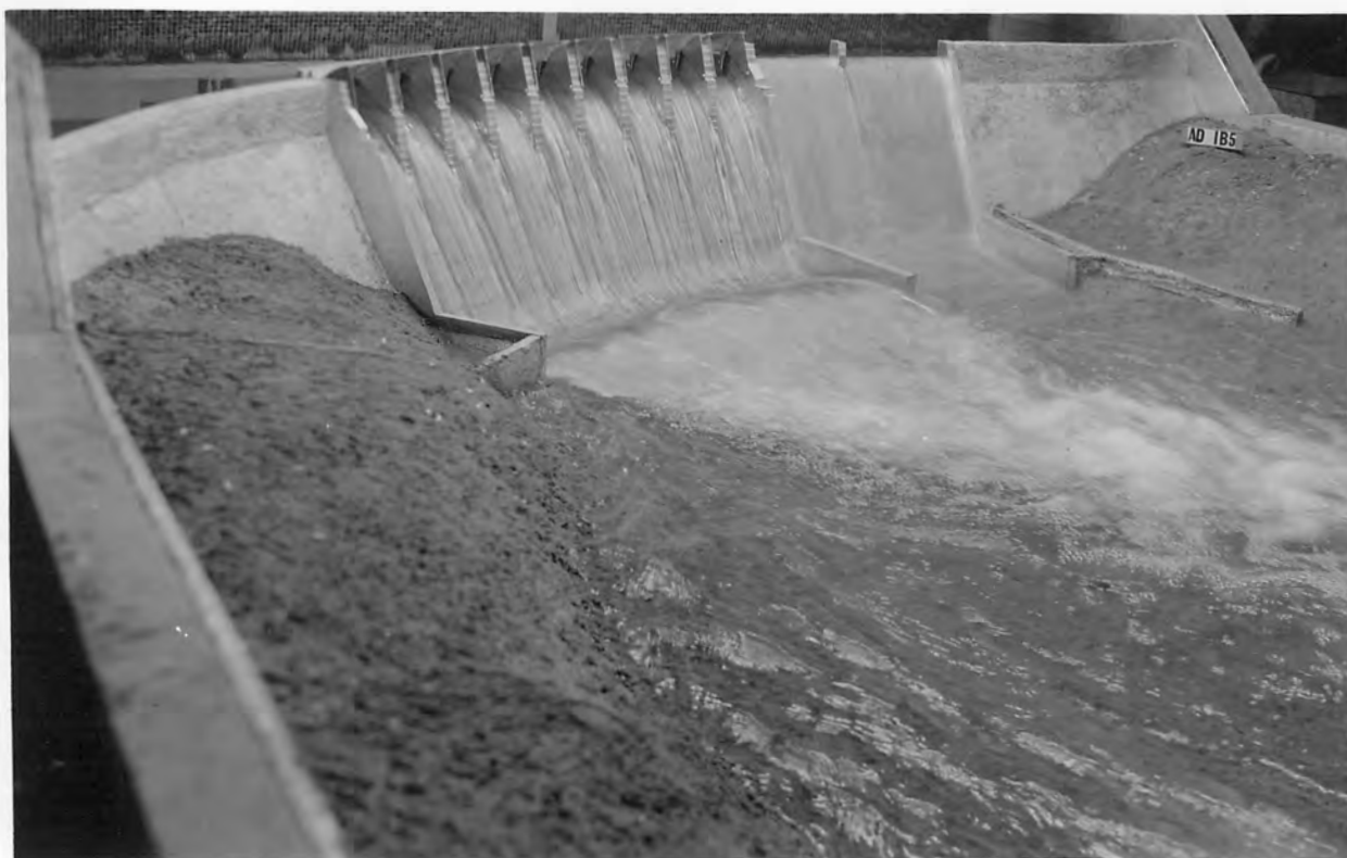
B HYDRAULIC JUMP REMAINS ON UNCONTROLLED SPILLWAY APRON WHEN ALL GATES OF CONTROLLED SPILLWAY ARE OPENED EQUALLY.
