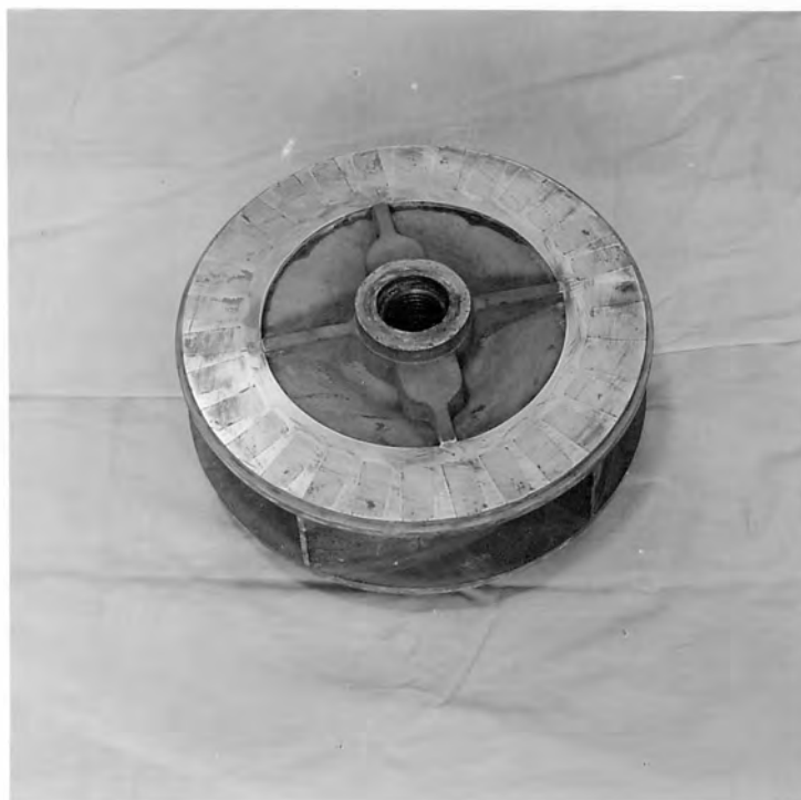
B. PUMP IMPELLER WITH BUCKETS FILLED.
