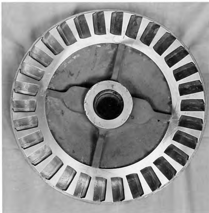
A. TOP OF REMODELED PUMP IMPELLER WITH THIRTY BUCKETS.
