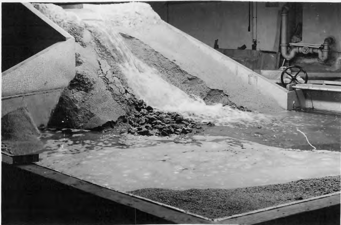
EROSION CAUSED BY MAXIMUM FLOW THROUGH SPILLWAY WHEN GATES ARE OPENED SLOWLY. MAXIMUM FLOW THROUGH OUTLET.
