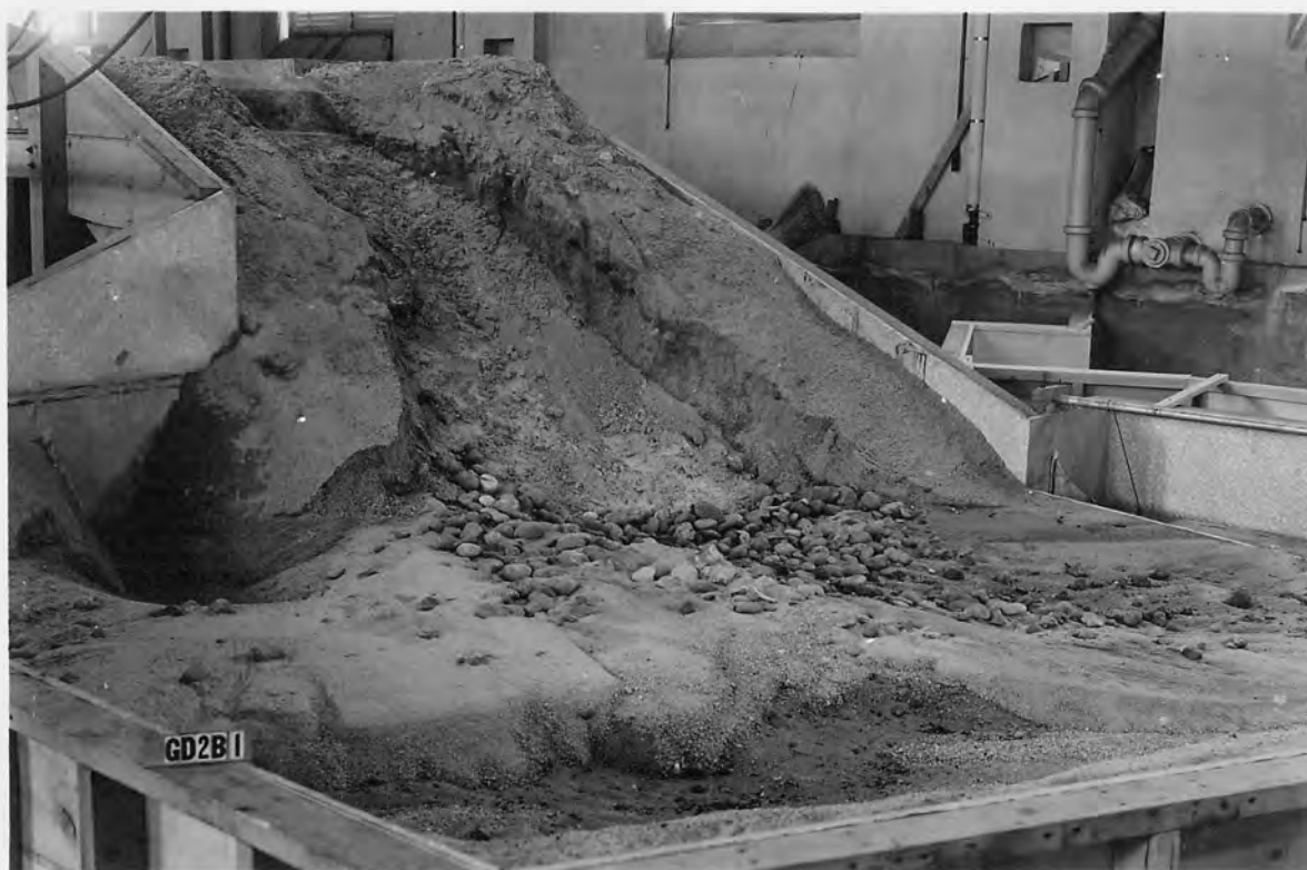
EROSION CAUSED BY MAXIMUM FLOW THROUGH SPILLWAY AND OUTLET.
