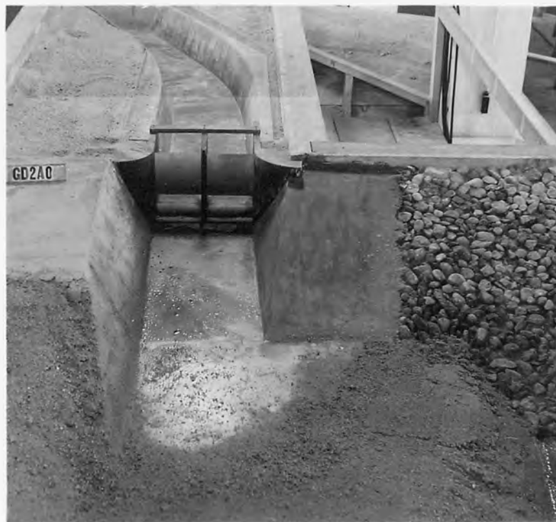
ENTRANCE TO SPILLWAY WITH WARP CHANGED TO SHARP CORNER.
