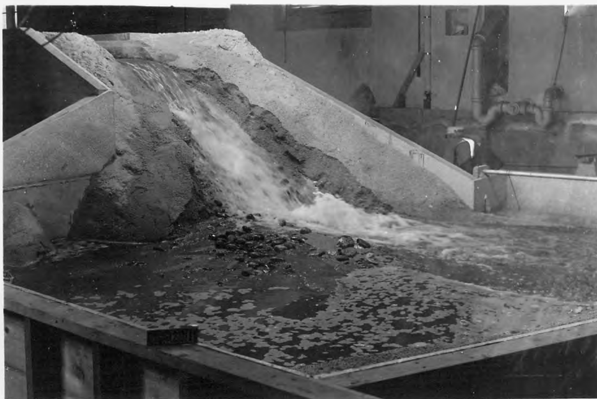
EROSION CAUSED BY MAXIMUM FLOW THROUGH SPILLWAY OF 12,000 SECOND-FEET. MAXIMUM FLOW THROUGH OUTLET.
