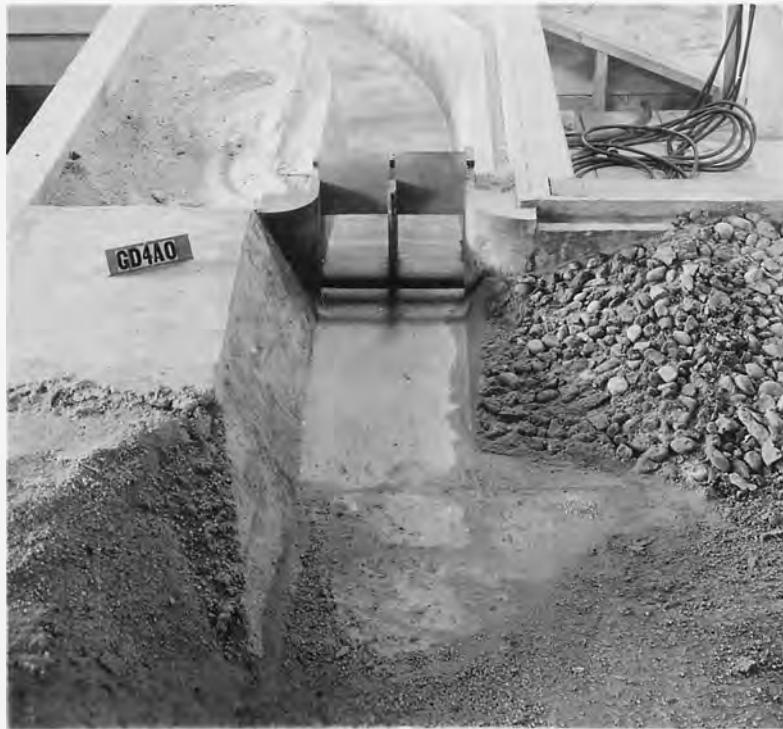
ENTRANCE TO SPILLWAY WITH TWO PLANE SURFACES SUBSTITUTED FOR WARP.
