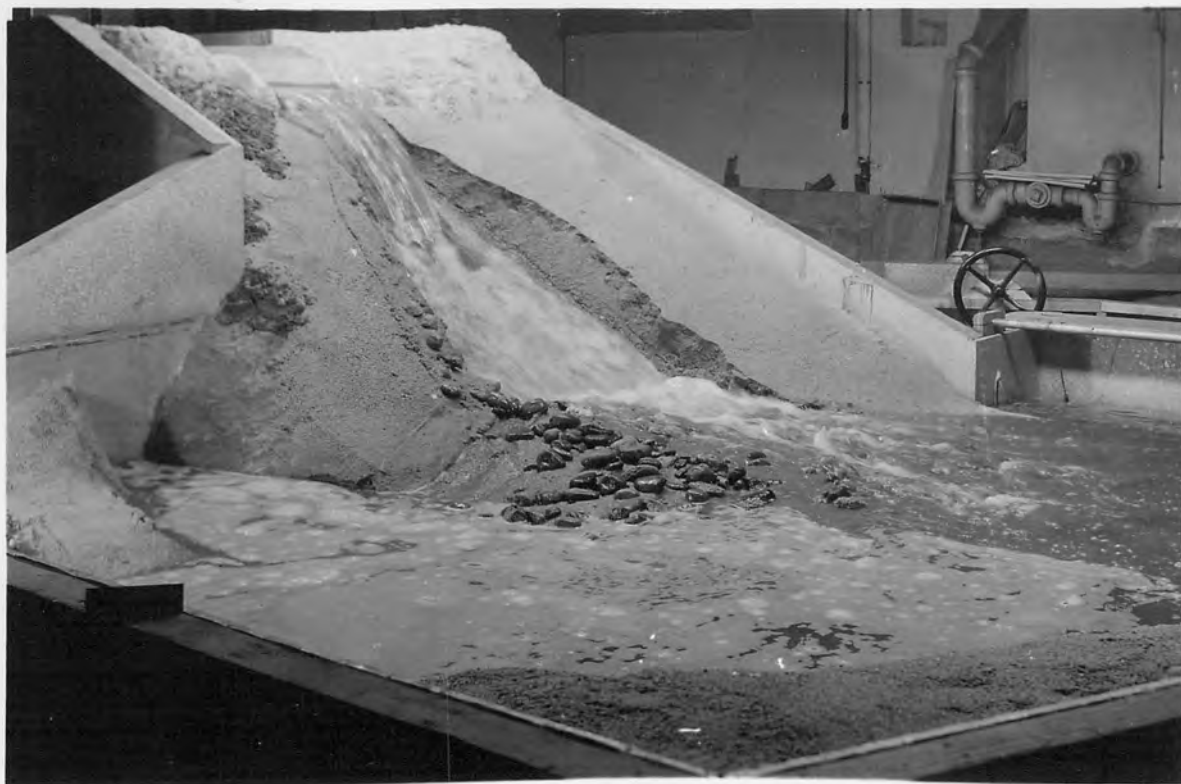
EROSION CAUSED BY MAXIMUM FLOW THROUGH SPILLWAY WHEN GATES ARE OPENED RAPIDLY. MAXIMUM FLOW THROUGH OUTLET.
