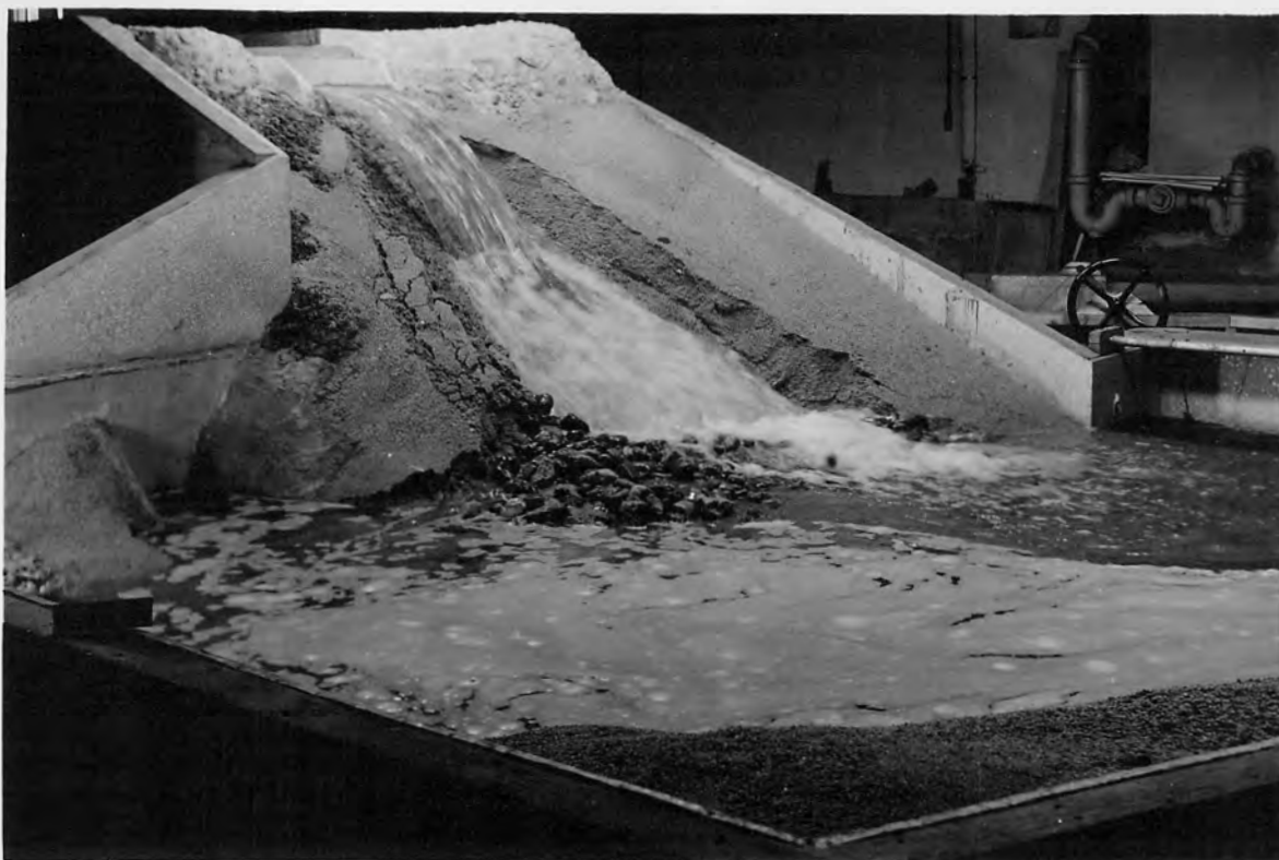
EROSION CAUSED BY MAXIMUM FLOW THROUGH SPILLWAY OF 12,000 SECOND-FOOT. MAXIMUM FLOW THROUGH OUTLET.
