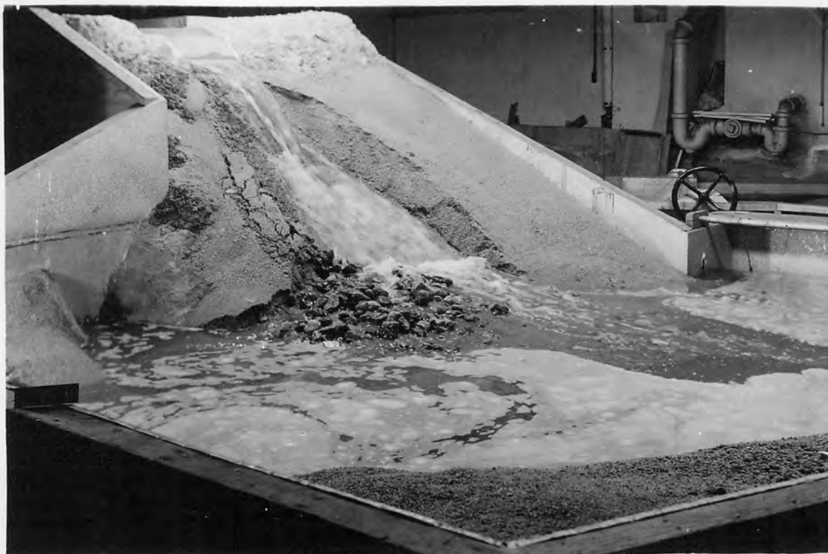
THIRD STEP IN EROSION CAUSED BY GRADUALLY OPENING SPILLWAY GATES. MAXIMUM FLOW THROUGH OUTLET.
