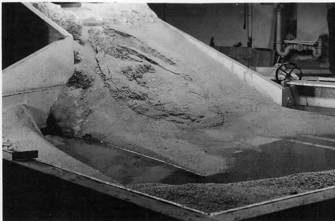
EROSION CAUSED BY MAXIMUM FLOW THROUGH OUTLET AND LEAKAGE THROUGH SPILLWAY GATES.
