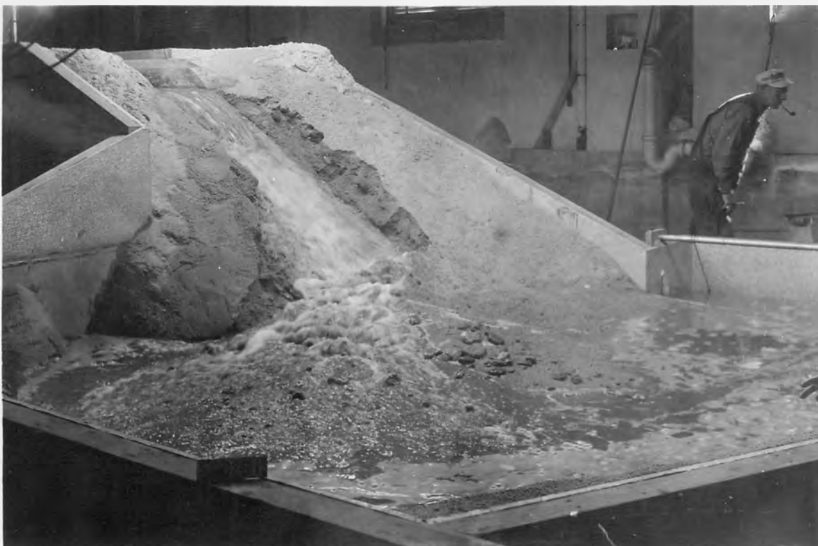
SECOND STEP IN EROSION CAUSED BY GRADUALLY OPENING SPILLWAY GATES. MAXIMUM FLOW THROUGH OUTLET.
