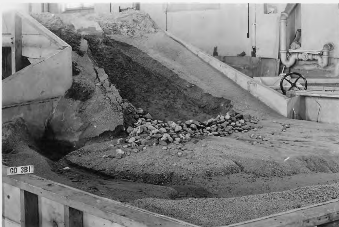
EROSION CAUSED BY GRADUALLY OPENING SPILLWAY GATES TO MAXIMUM DISCHARGE.
