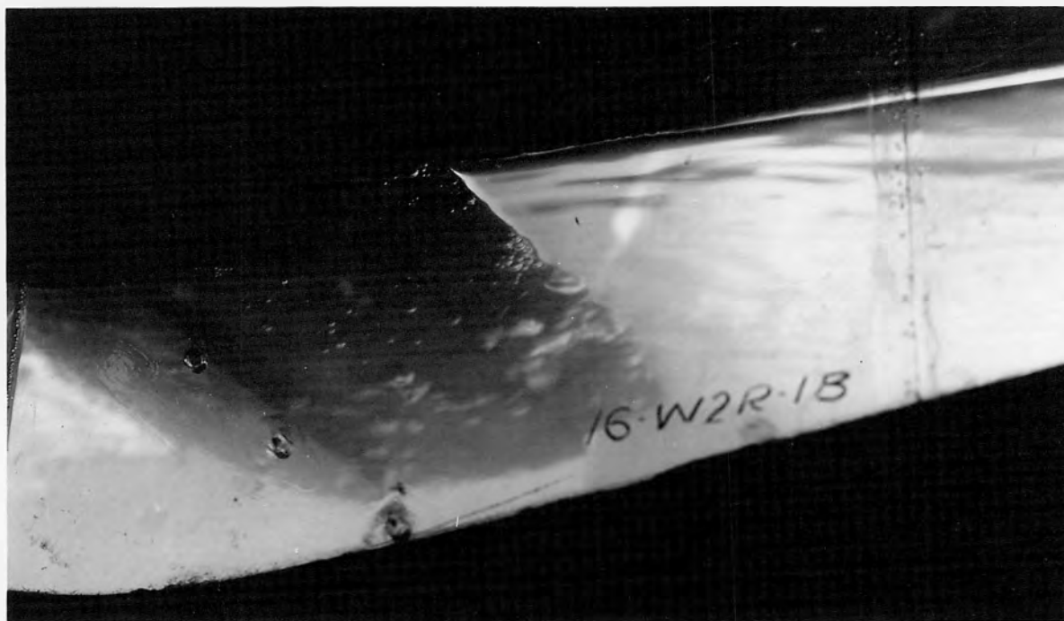
B. AIR ESCAPING FROM END OF VANE PAST CROWN OF LOWER BEND. AT MINIMUM PRIMING HEAD OF 0.15 FOOT.
