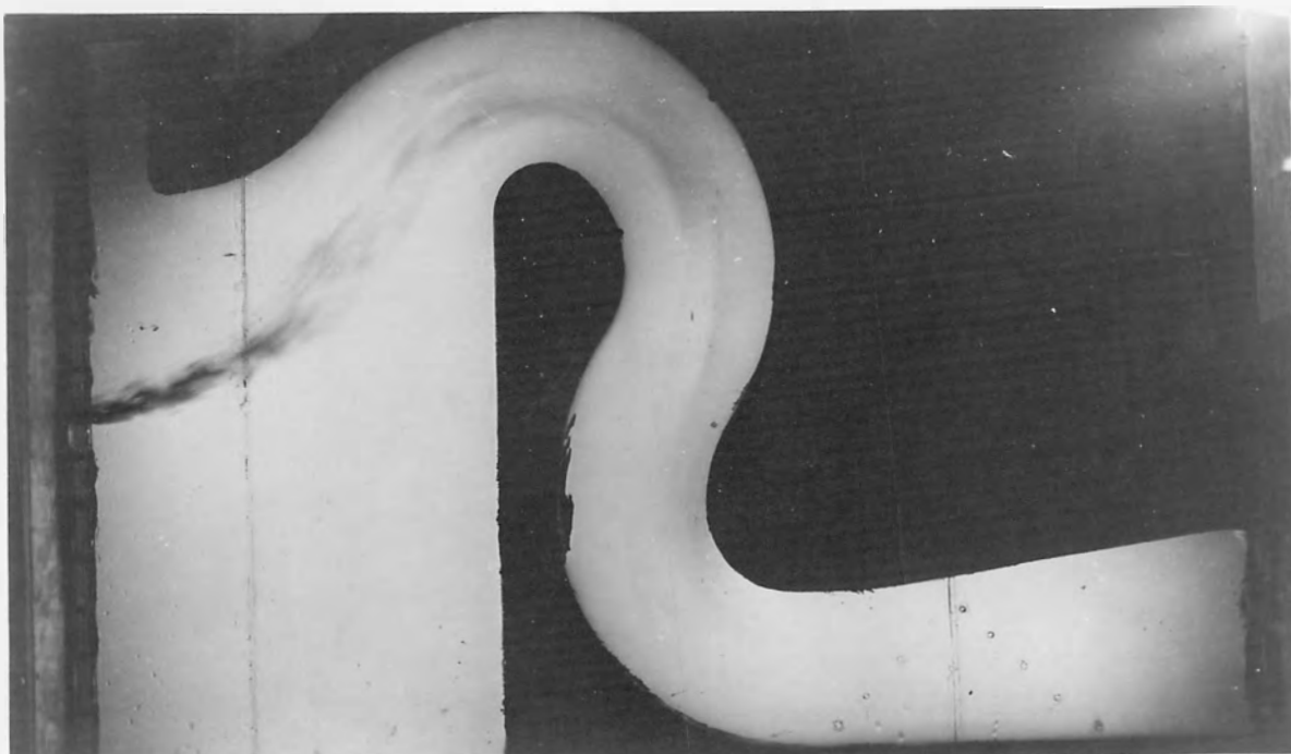
B. DISCHARGE 404 SECOND-FEET WITH HEAD OF 2.50 FEET(PROTOTYPE) TAILWATER TO SEAL EXIT.
