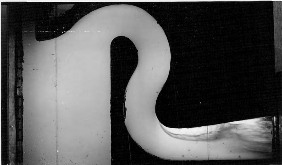
A. DISCHARGE 317 SECOND-FEET WITH HEAD OF 4.10 FEET(PROTOTYPE), NO TAILWATER.
