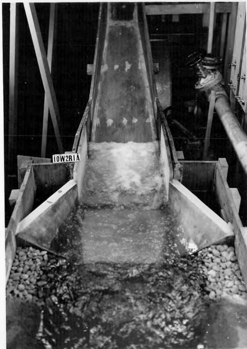
B. DIVERGING CHUTE WITH PARABOLIC WALL DESIGN 4 AND POOL DESIGN 3.
