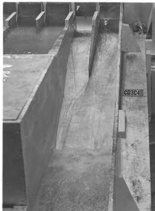
FLOW OF 2200 SECOND-FEET DIVIDED BETWEEN ONE UNIT OF POWERHOUSE AND OPPOSITE SPILLWAY
