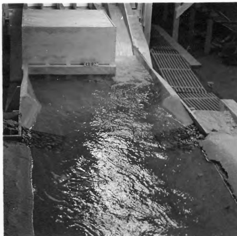
FLOW OF 2200 SECOND-FEET THROUGH SPILLWAY
