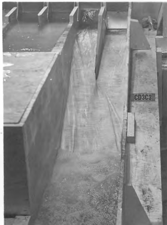
FLOW OF 2200 SECOND-FEET DIVIDED BETWEEN ONE UNIT OF POWERHOUSE AND ADJACENT SPILLWAY
