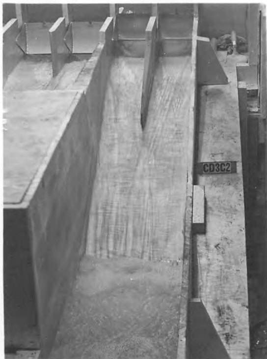
FLOW OF 2200 SECOND-FEET THRU SPILLWAY WITH BOTH GATES OPEN
