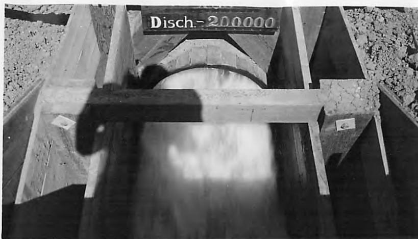
A-OUTLET OF TUNNEL-ORIGINAL DESIGN MODEL M-I TUNNEL FLOWING FULL DURING THUMP
