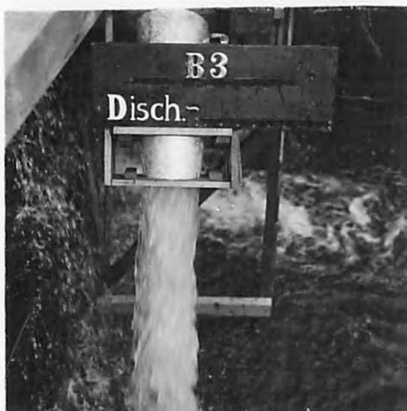
C - SLIGHTLY SPIRAL FLOW AT END OF TRANSITION
