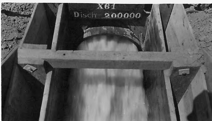
B-OUTLET OF TUNNEL FLOWING PARTLY FULL-MODEL M-I
