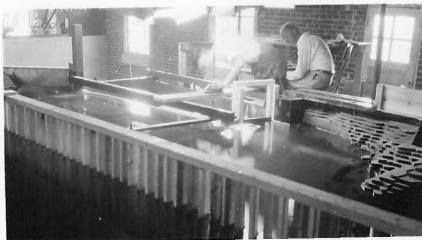
B-OBSERVING WATER SURFACE ELEVATION WITH POINT GAGE
