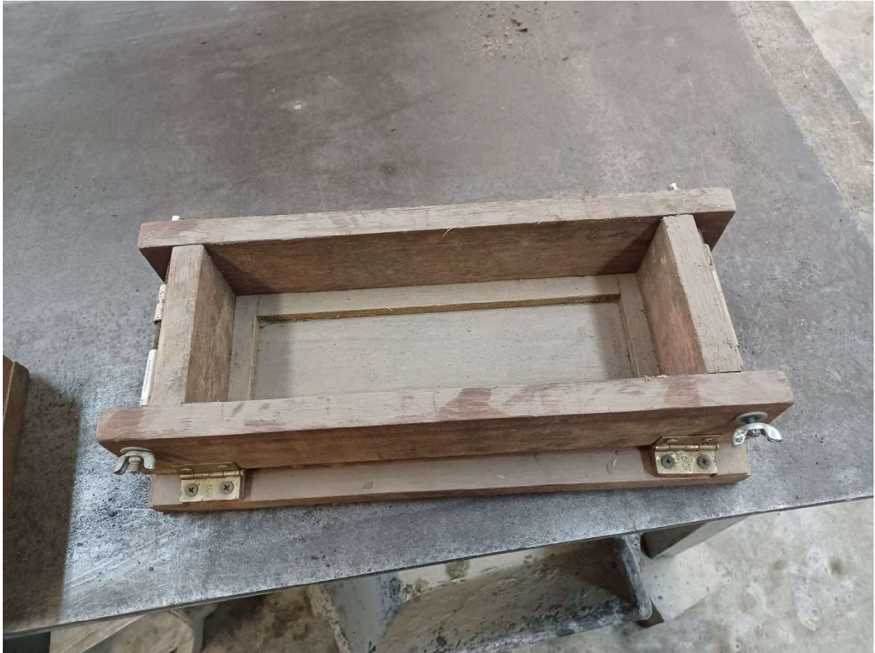
Figure 6. Mold used to form the concrete test samples of the current research in the Concrete and Structural Laboratory at UFRGS.
