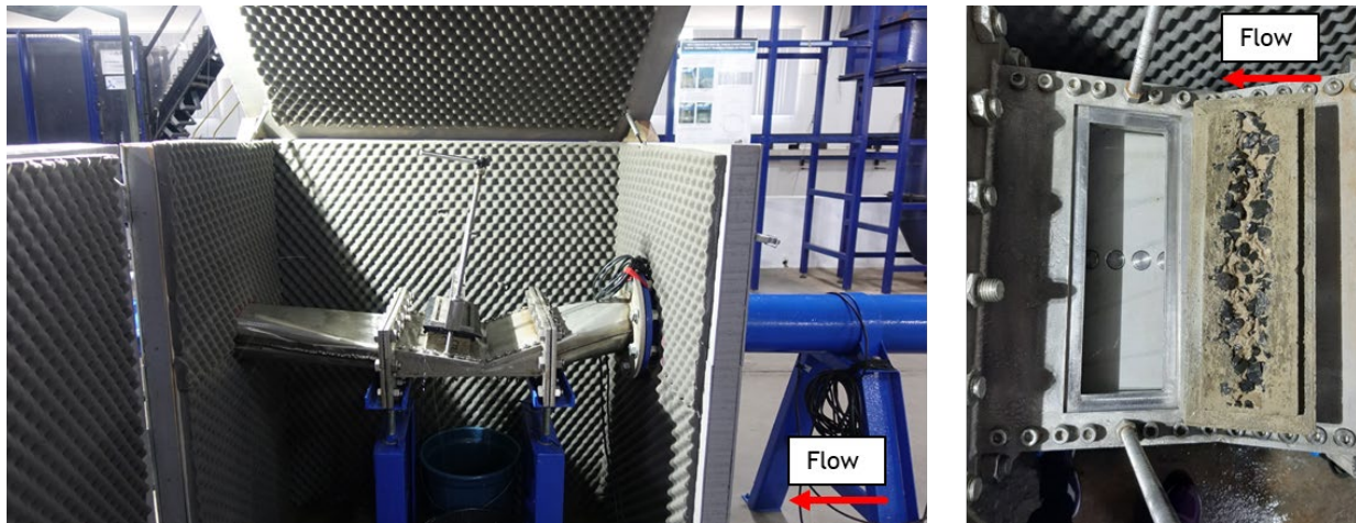
Figure 1. Photograph of the cavitation test machine at UFRGS within the soundproof box (left) and looking from the top where the cavitation sample is installed (right).
