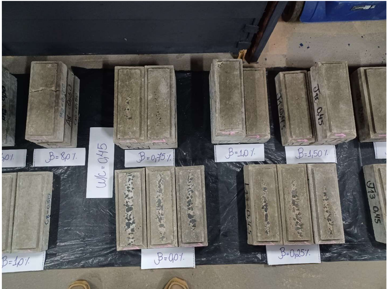
Figure 2. Concrete test samples after cavitation testing at UFRGS.
