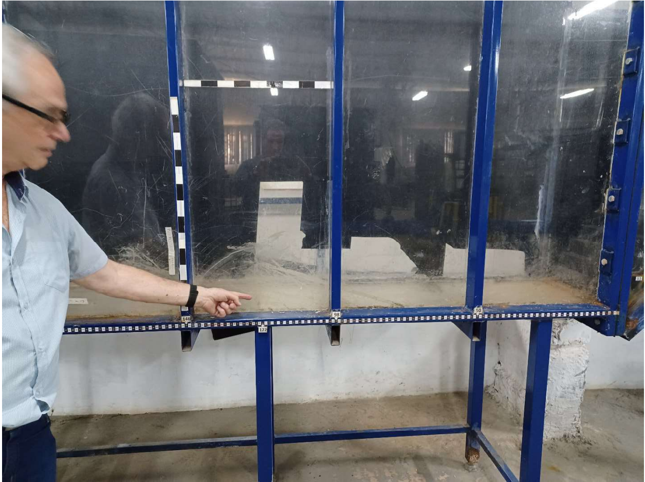
Figure 4. Prof. Marcelo Marques explaining past research of stilling basin design downstream of stepped spillways at UFRGS. Reclamation is at the beginning stages of this same research and the insights and information gained from this trip help boost our study.
