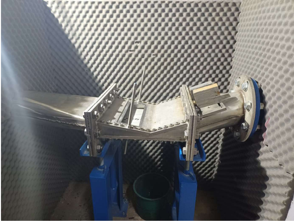
Figure 1. Cavitation machine at UFRGS (similar to Reclamation's) used to test durability of concrete to cavitation.
