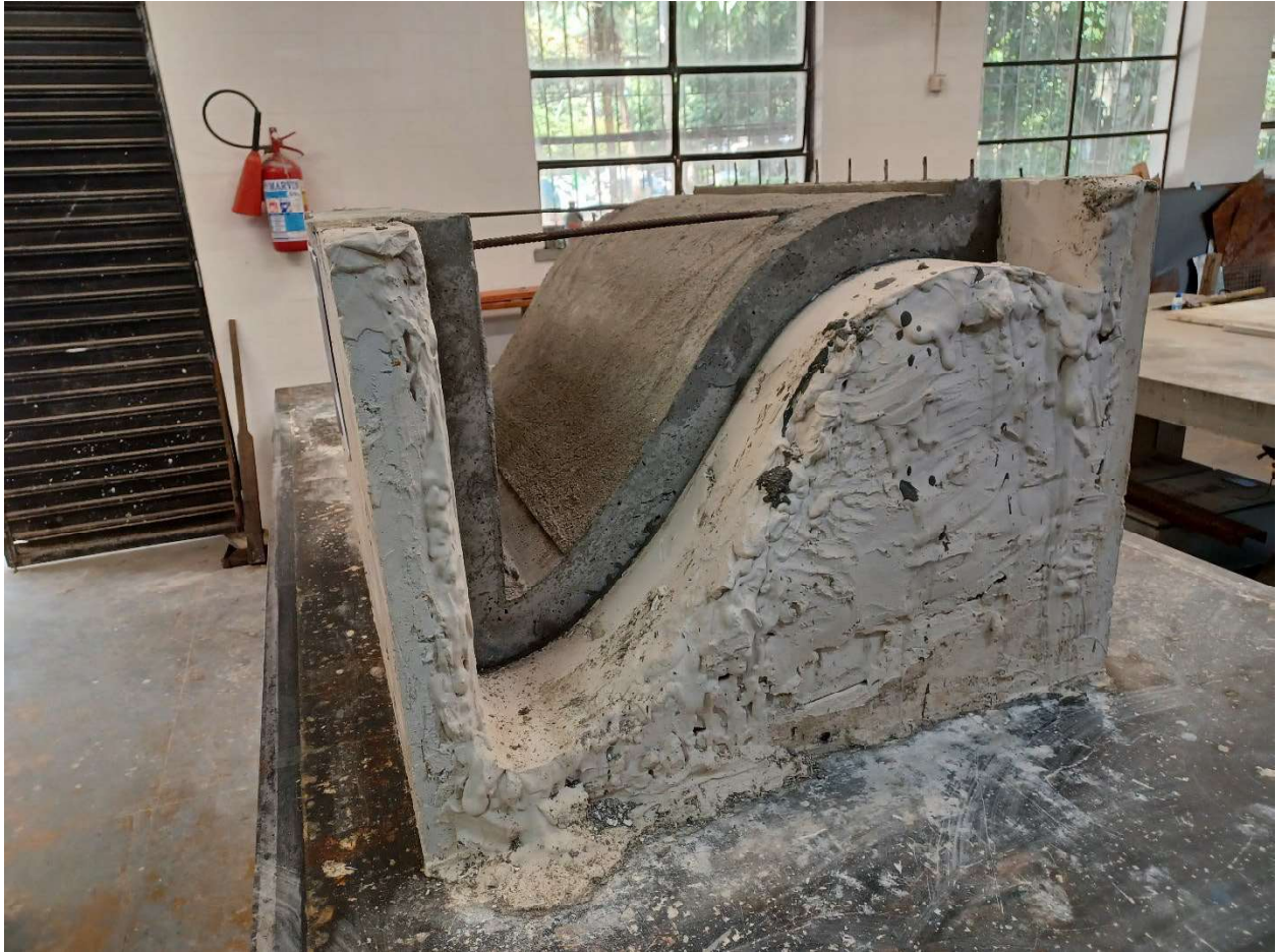
Figure 9. The model fabrication shop at the FURNAS hydraulics lab. This section is part of a spillway model that is made of concrete in a plaster mold. It was beneficial to learn of different model construction techniques used in Brazil compared to our methods in Reclamation.
