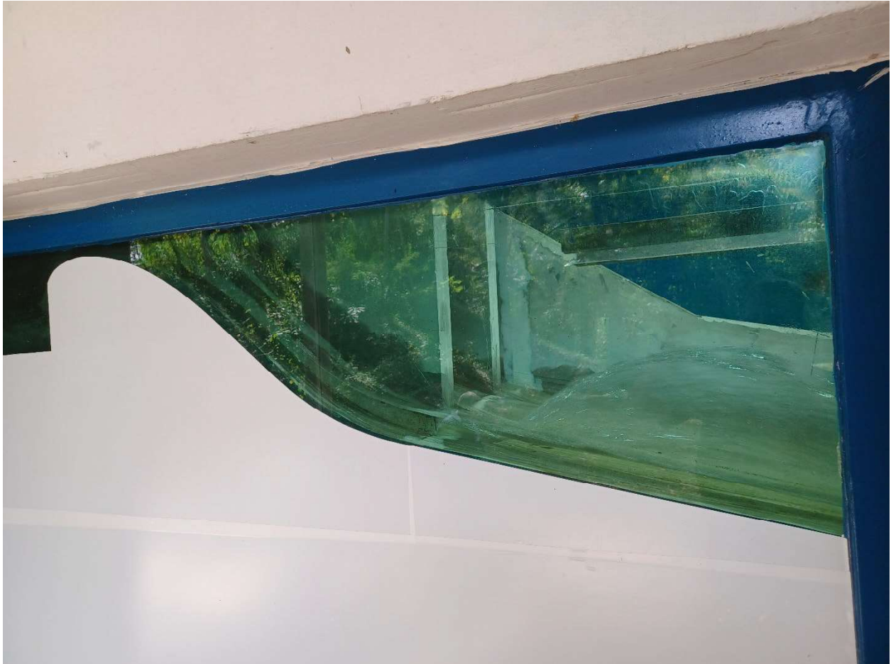
Figure 8. Physical model of the FURNAS facility spillway at the FURNAS hydraulics lab. This spillway has suffered cavitation damage and is an important case study of the current research.
