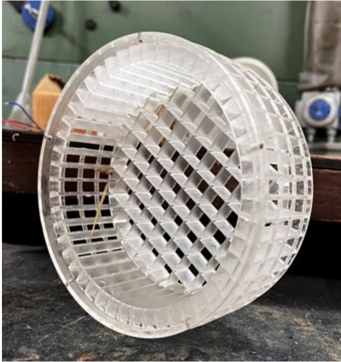
Figure 14. 3D printed flow baskets designed to attach to the bottom of the pump bells.
