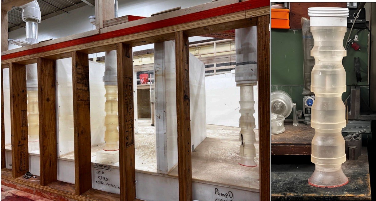
Figure 2. Left, construction methods utilized marine-coated plywood sheeting, clear acrylic paneling and expanded PVC sheeting. Right, clear 3D printed pump bells.
