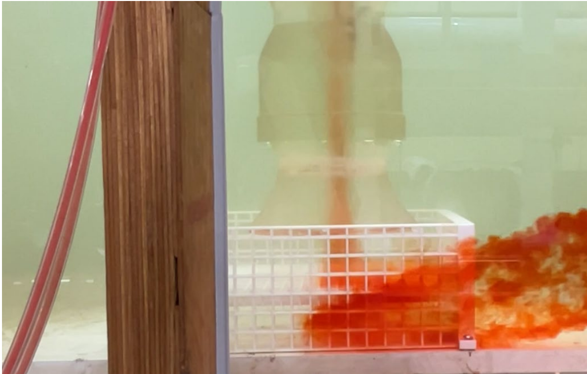
Figure 16. Dye visualization of flow distributed by the rectangular flow straightening basket before entering the pump bell.
