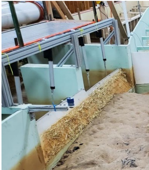
Figure 24. Accumulation of debris on trashrack post-test.
