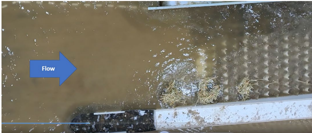
Figure 22. Debris mats accumulated in the 1:24 model at a river flow of 6,000 ft 3 /s. All debris mats were flushed downstream at 12,000 ft 3 /s.
