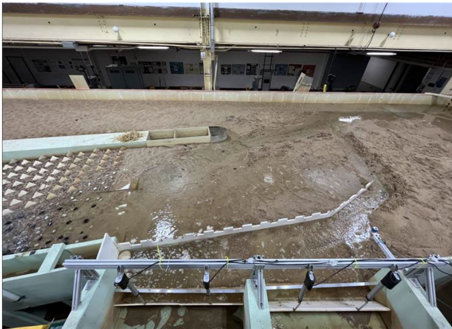
Figure 26. Redirected channel at 250 \text{ ft}^3/\text{s} river flow when the bed was first set.
