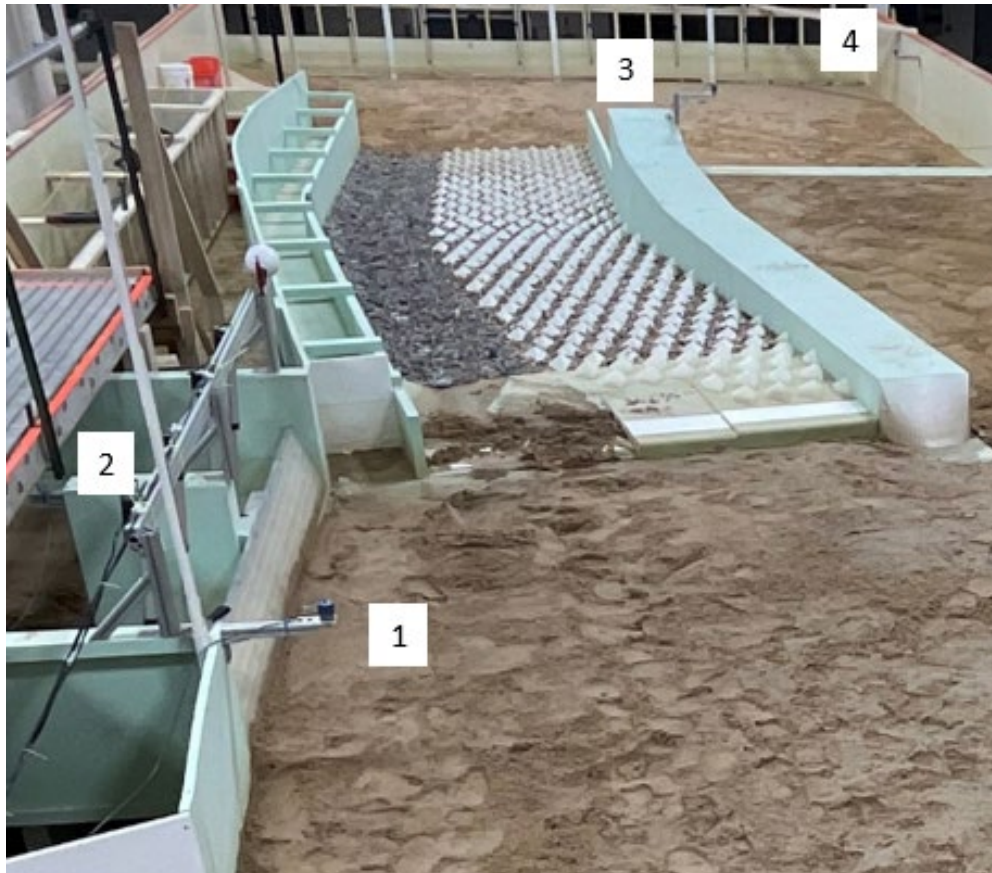
Figure 5. View of water level sensor locations on 1:12 model (looking downstream).
