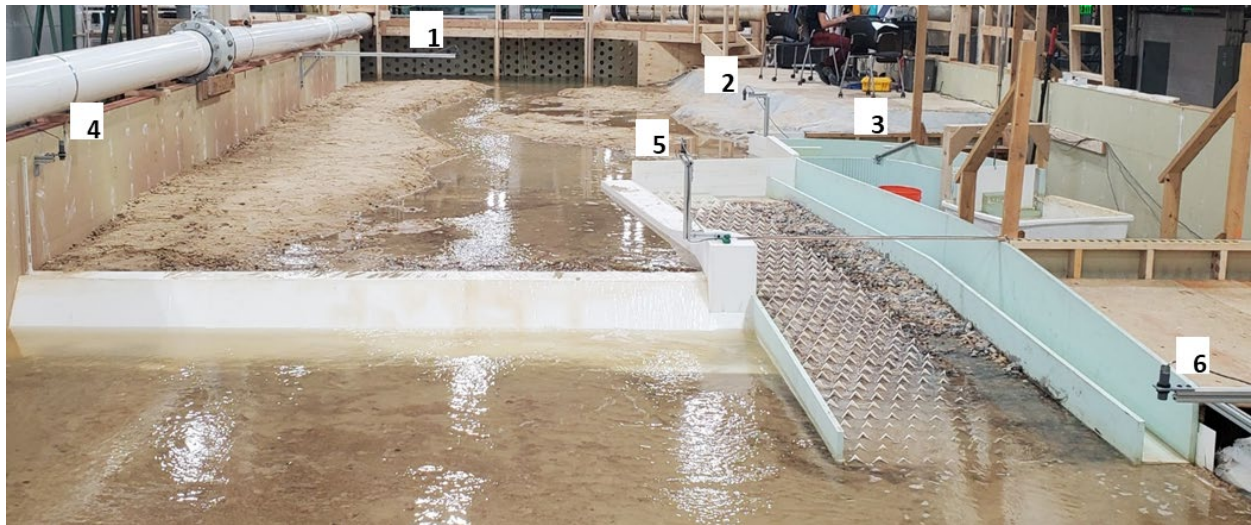
Figure 4. View of water level sensor locations on 1:24 model (looking upstream). Sensors 1 and 4 were removed for this portion of testing.
