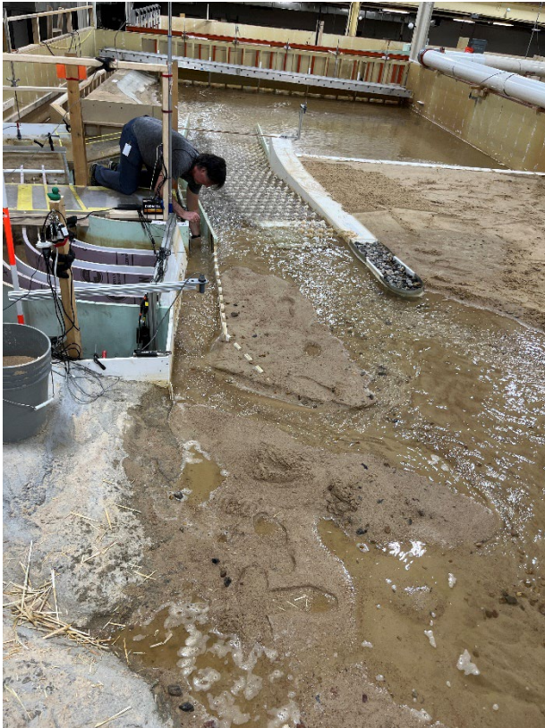
Figure 25. Redirected upstream approach channel in the 1:24 model at 1,500 ft 3 /s.
