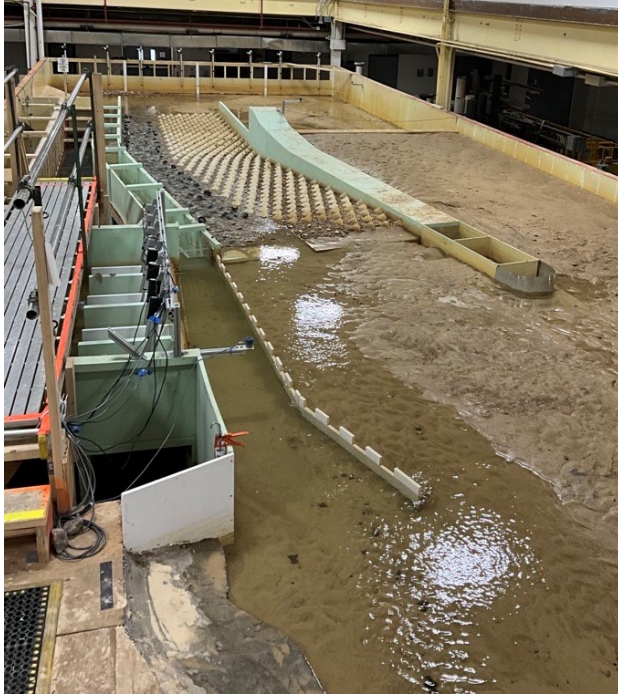
Figure 28. Diversion intake cleared of sediment during testing with a river flow rate of 250 ft 3 /s.
