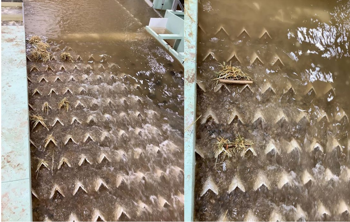
Figure 23. Debris in the 1:12 model showing debris mats (left) and debris mats with woody debris incorporated (right) at a river flow of 6,000 ft 3 /s. Point depths and velocities were measured around the debris mats and between adjacent baffles.
