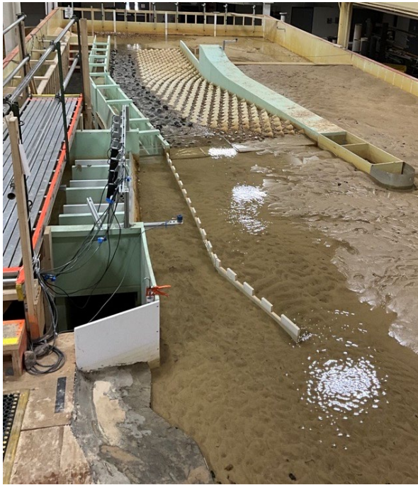
Figure 27. Diversion intake filled with sediment during testing at a river flow of 250 ft 3 /s.
