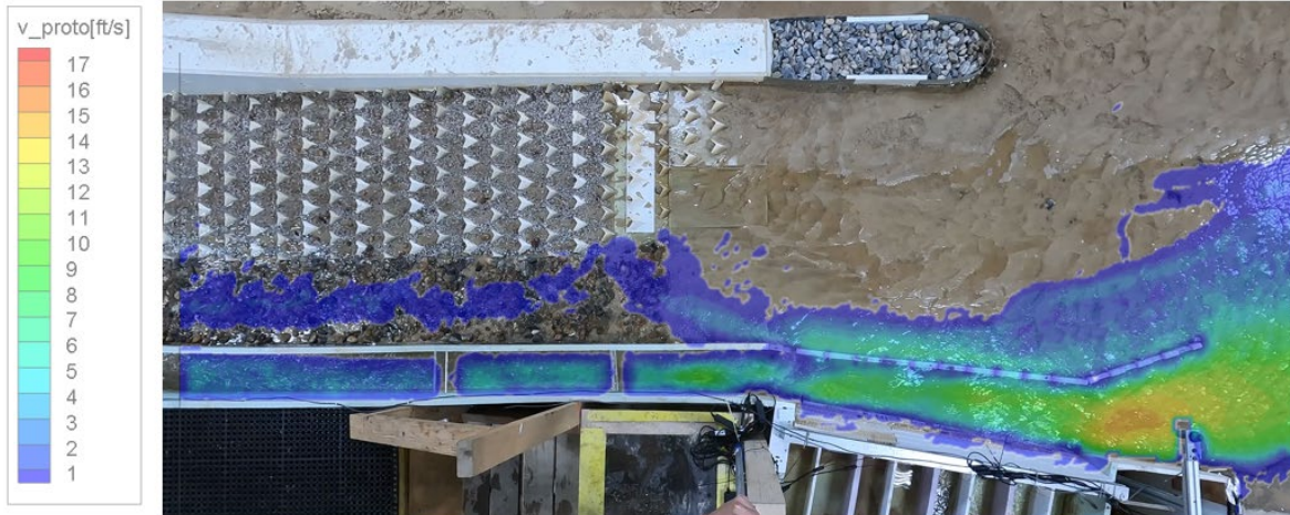
Figure 10. LSPIV data with flushing channel open at a river flow of 1,500 ft 3 /s. Velocities less than 0.1 ft/s have been made transparent.
