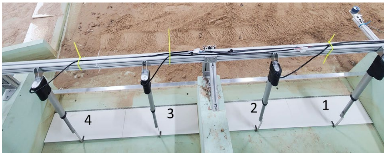
Figure 36. Canal intake gates (looking upstream from intake) with individual actuators to adjust gate settings remotely.
