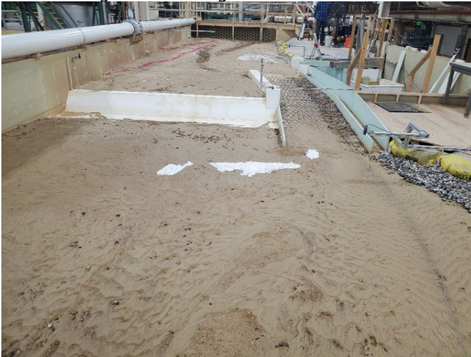
Figure B-10. View looking upstream for MOD-6 design with flushing channel removed after 3,000 ft 3 /s flow rate.
