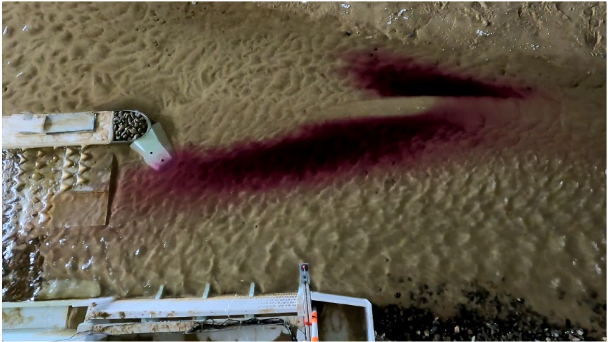
Figure 61. Photograph of dye approaching the hardened ramp without a flushing channel at 3,000 ft 3 /s with added sediment features.
