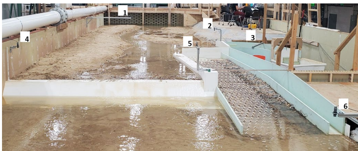
Figure 15. View of water level sensor locations on 1:24 model (looking upstream).
