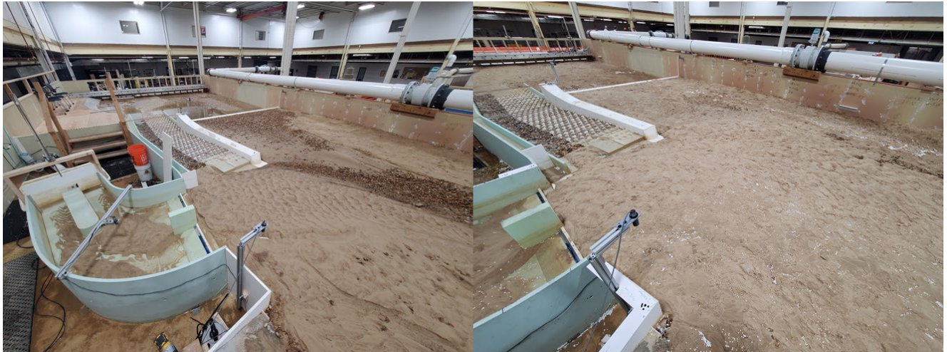
Figure 23. Photographs of the bed material comparisons near the beginning (left) and end (right) of shakedown testing where additional fine materials were added to the top layer for more realistic sediment conditions expected for a flow range of 1,000 to 12,000 ft 3 /s.
