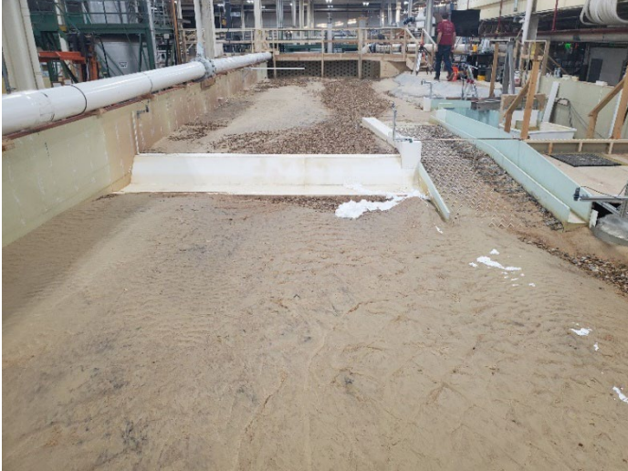
Figure B-96. View looking upstream for MOD-6 design with flushing channel open after 30,000 ft 3 /s flow rate.
