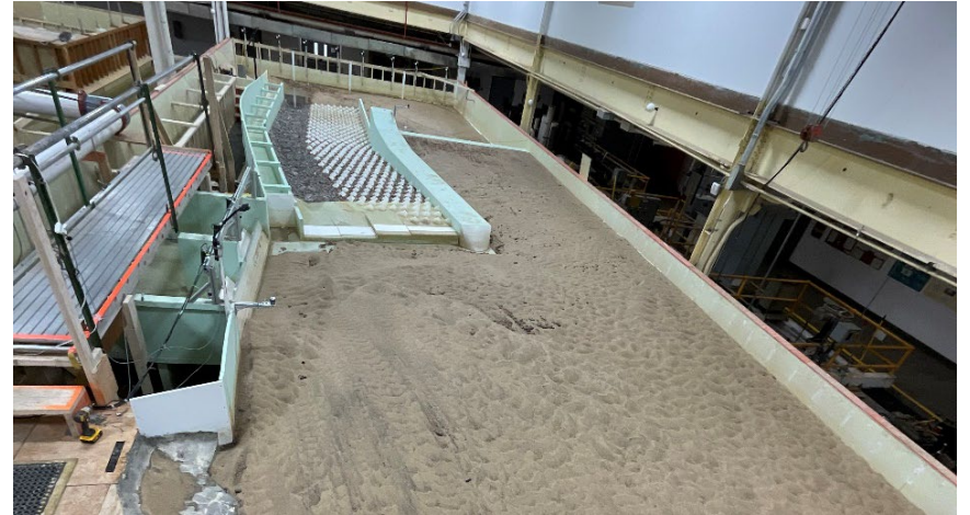
Figure C-43. View looking downstream after dewatering for MOD-9 design with flushing channel open at 1,500 ft 3 /s.
