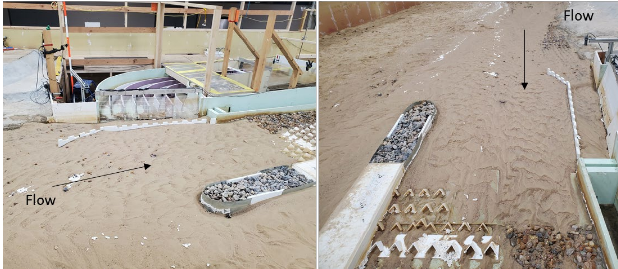
Figure 85. Photographs of the sediment bedforms upstream of hardened ramp with a castle training wall and flushing channel at 1,500 ft 3 /s.
