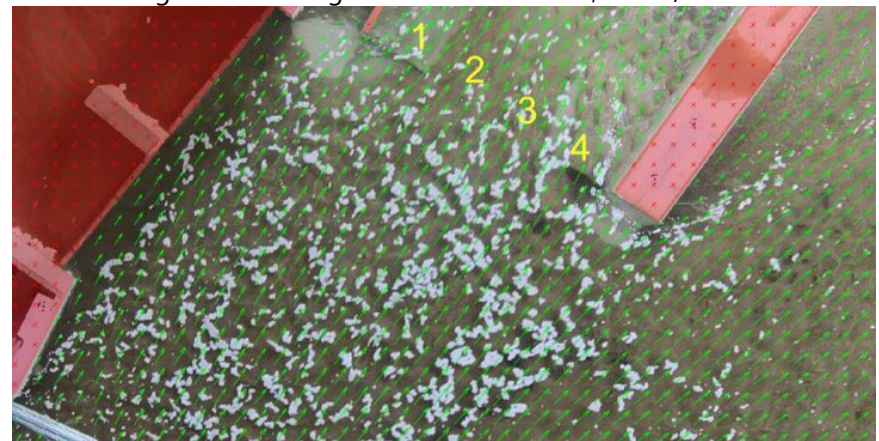
Figure B-76. Surface velocity vector map in area upstream of diversion intake (left) and hardened ramp (right) for MOD-9 design with flushing channel closed at 12,000 ft 3 /s river flow.
