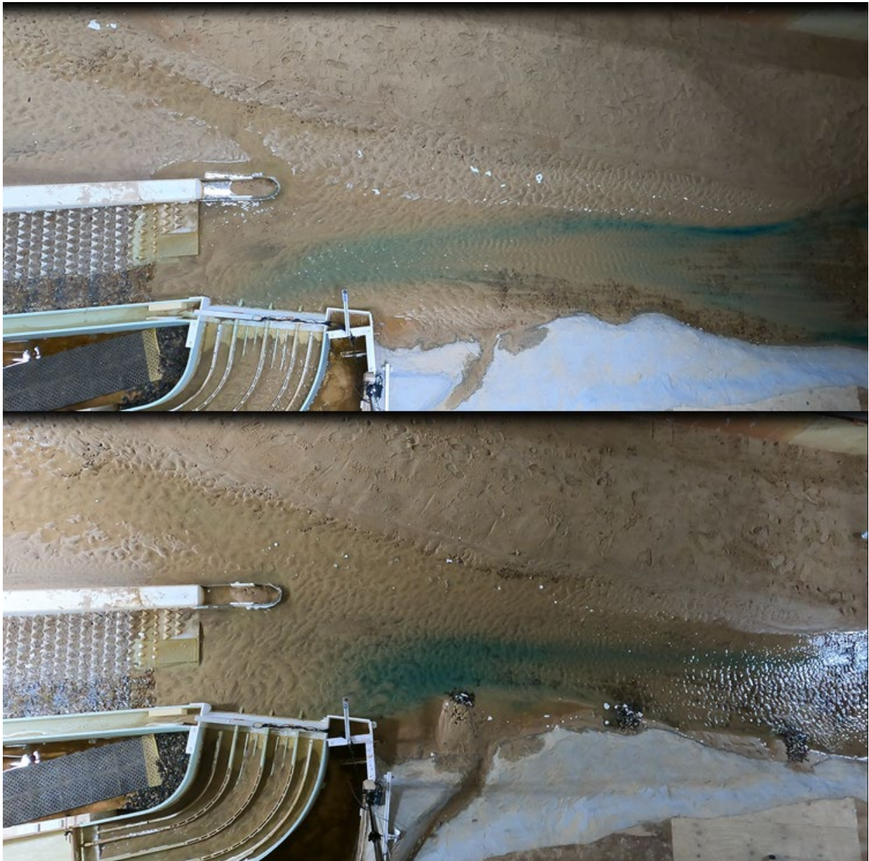
Figure 122. Photographs of flows with dye approaching the hardened ramp without groynes (top) and with groynes (bottom) at 1,500 ft 3 /s.
