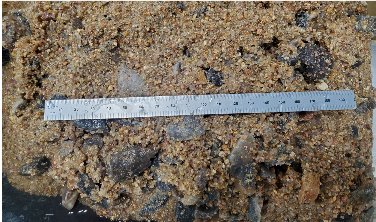
Figure 18. Photograph of ruler and 1:24 scale sediment blend used for visualization of sediment movement.
