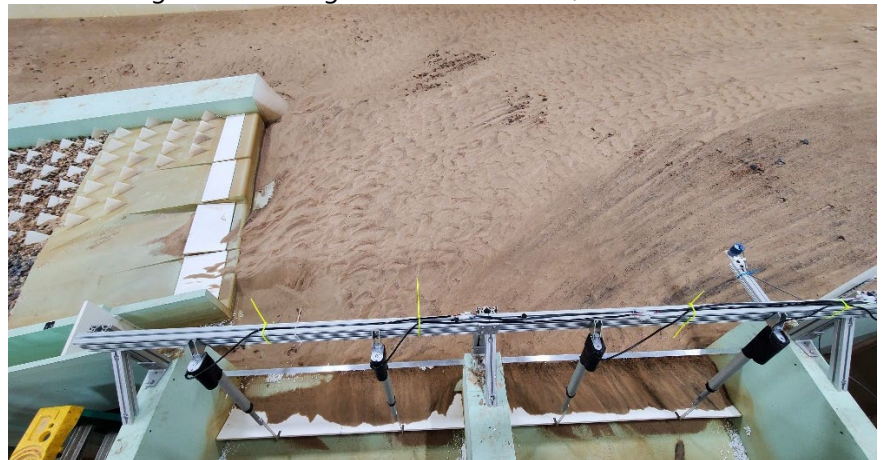
Figure C-47. View looking upstream from diversion canal of area upstream of diversion intake (bottom) and hardened ramp (left) for MOD-9 design with flushing channel closed at 1,500 ft 3 /s river flow.
