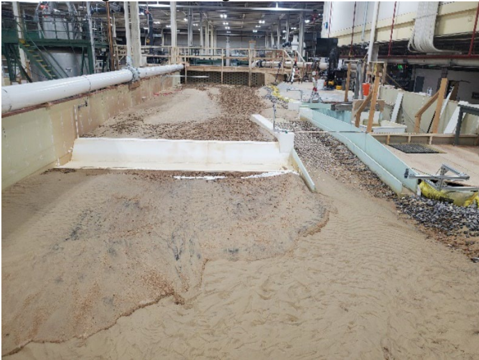
Figure B-100. View looking upstream for MOD-6 design with flushing channel removed after 30,000 ft 3 /s flow rate.
