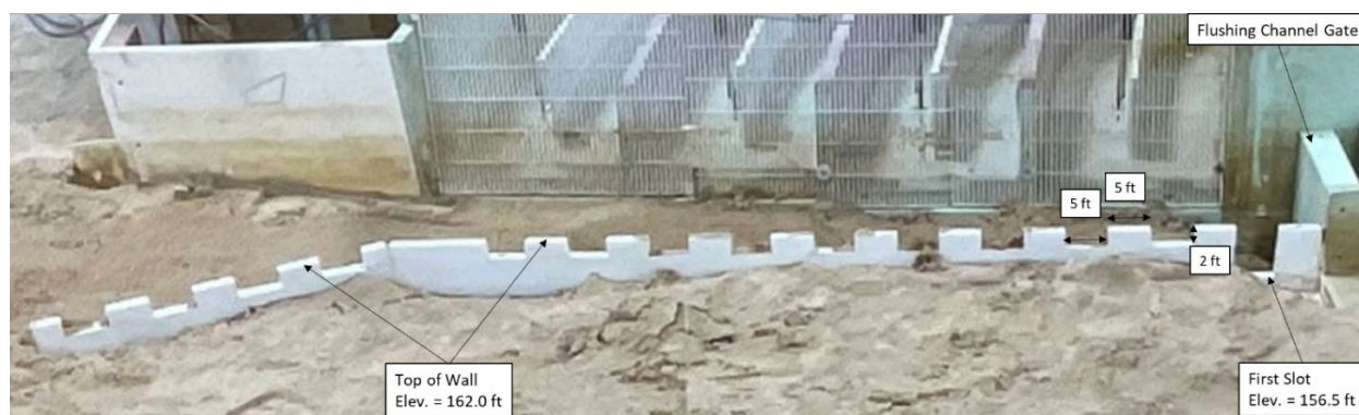
Figure 72. Photograph showing the castle training wall in the 1:24 model.
