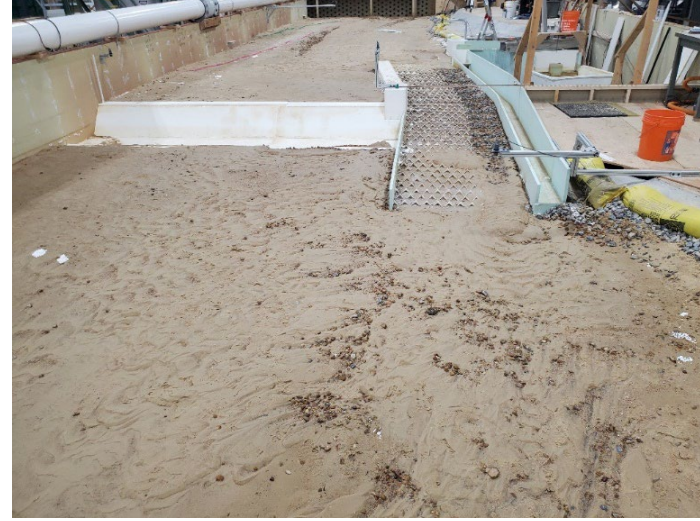
Figure B-12. View looking upstream for MOD-9 design with flushing channel removed after 3,000 ft 3 /s flow rate.
