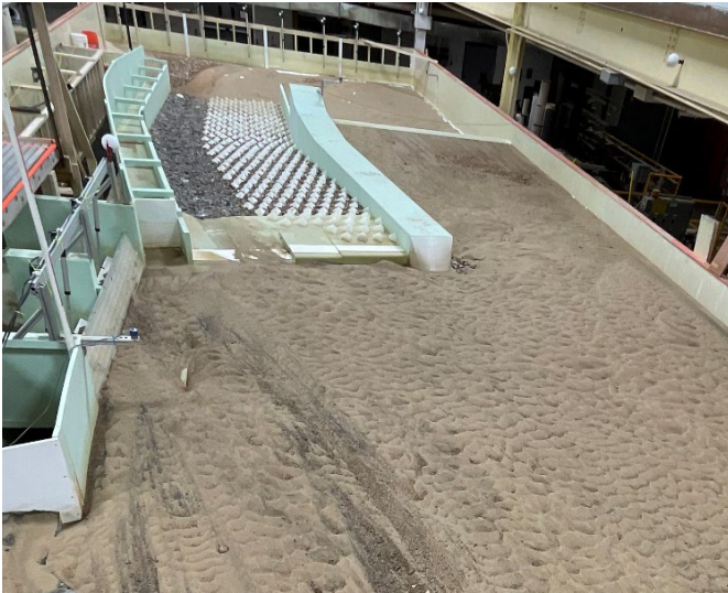
Figure C-17. View looking downstream after dewatering for MOD-6 design with flushing channel closed at 3,000 ft 3 /s.
