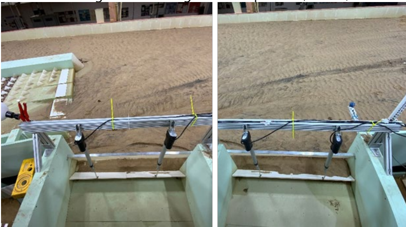
Figure C-14. Views looking upstream from diversion canal of area upstream of diversion intake (bottom) and hardened ramp (left) for MOD-6 design with flushing channel open at 6,000 ft 3 /s.
