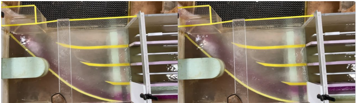
Figure 108. Photographs showing flow patterns with dye exiting the outside (left) and inside (right) channels of Bay 1. Sluicing flow was approximately 200 ft 3 /s.
