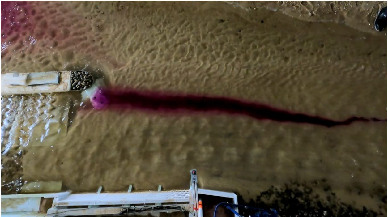
Figure 57. Photograph of dye approaching the hardened ramp without a flushing channel at 6,000 ft 3 /s with added sediment features.
