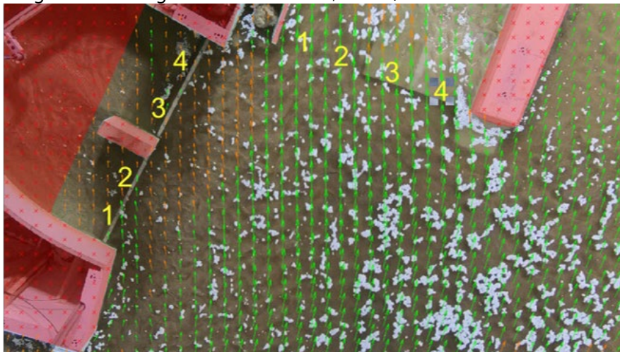
Figure B-44. Surface velocity vector map in area upstream of diversion intake (left) and hardened ramp (right) for MOD-6 design with flushing channel closed at 6,000 ft 3 /s river flow.
