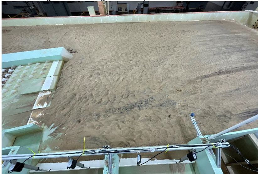
Figure C-30. View looking upstream from diversion canal of area upstream of diversion intake (bottom) and hardened ramp (left) for MOD-6 design with flushing channel open at 3,000 ft 3 /s river flow.
