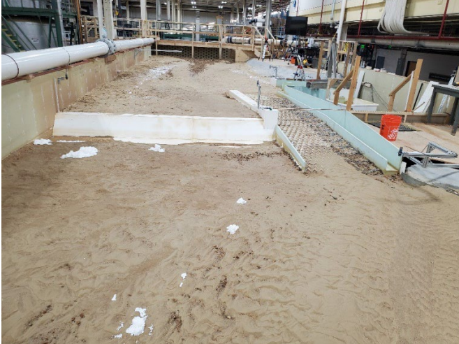
Figure B-6. View looking upstream for MOD-6 design with flushing channel open after 3,000 ft 3 /s flow rate.
