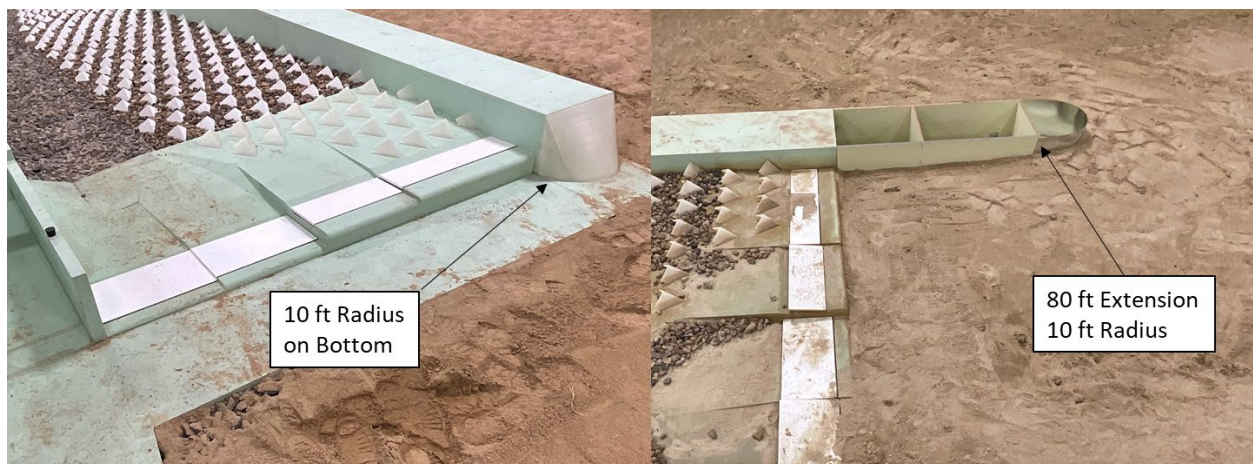
Figure 38. Photographs of the 1:12 physical model comparing the original design of the bullnose for baseline testing (left) with the extension tested in the design development phase (right).
