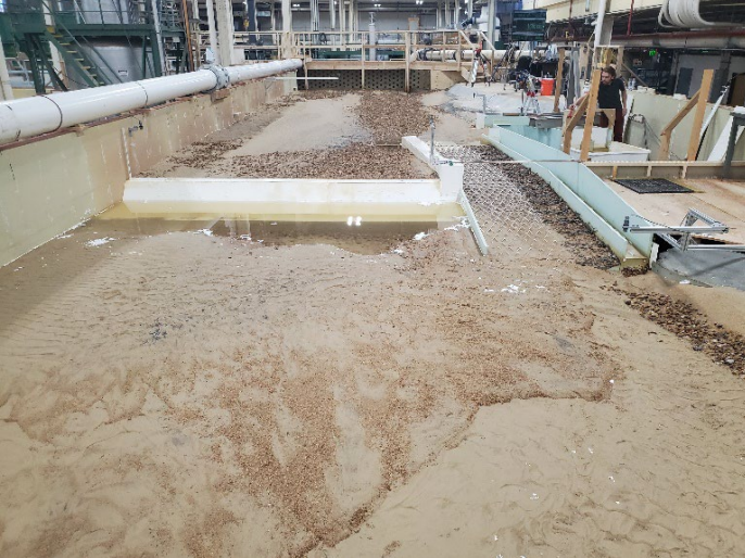
Figure B-92. View looking upstream for MOD-6 design with flushing channel closed after 30,000 ft 3 /s flow rate.
