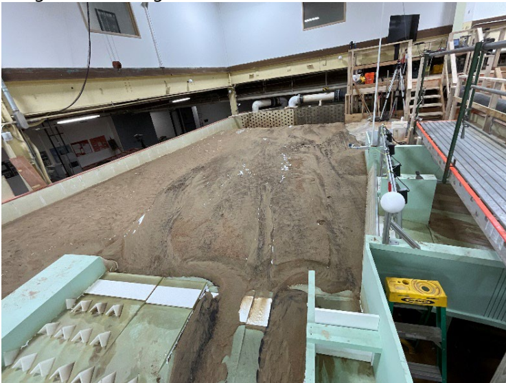
Figure C-56. View looking upstream for MOD-6 design with flushing channel closed after 270 ft 3 /s flow rate.
