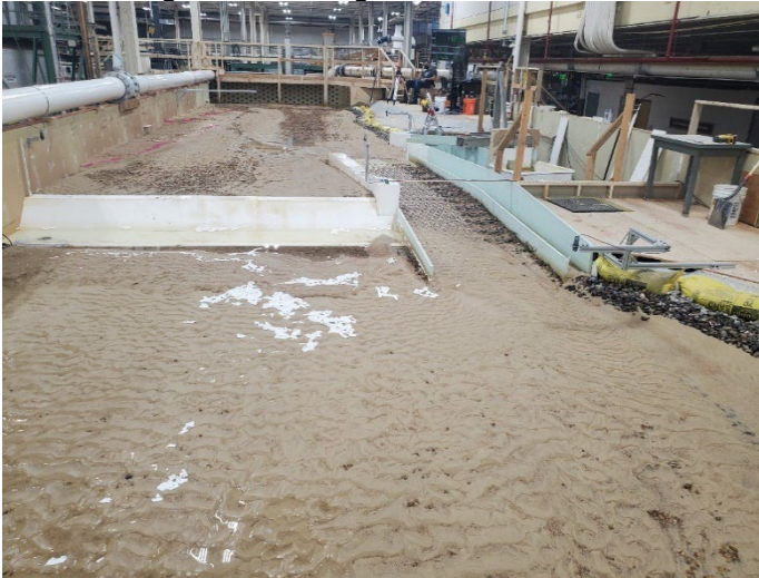
Figure B-70. View looking upstream for MOD-6 design with flushing channel removed after 12,000 ft 3 /s flow rate.
