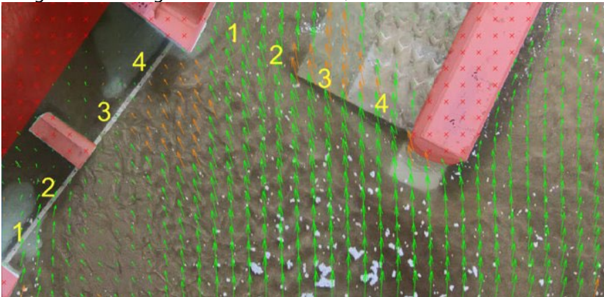
Figure B-52. Surface velocity vector map in area upstream of diversion intake (left) and hardened ramp (right) for MOD-6 design with flushing channel removed at 6,000 ft 3 /s river flow.
