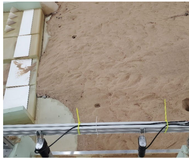
Figure C-4. View of ramp exit looking from left bank for MOD-9 design with flushing channel closed after 6,000 ft 3 /s flow rate.
