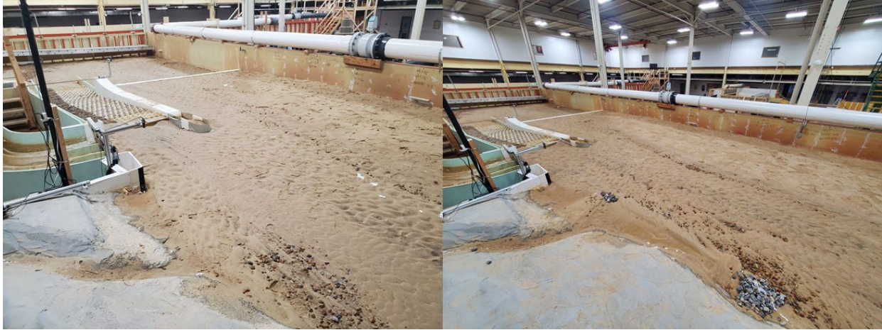
Figure 120. Photographs of sediment bedforms upstream of the hardened ramp without groynes (left) and with groynes (right) at 3,000 ft 3 /s.
