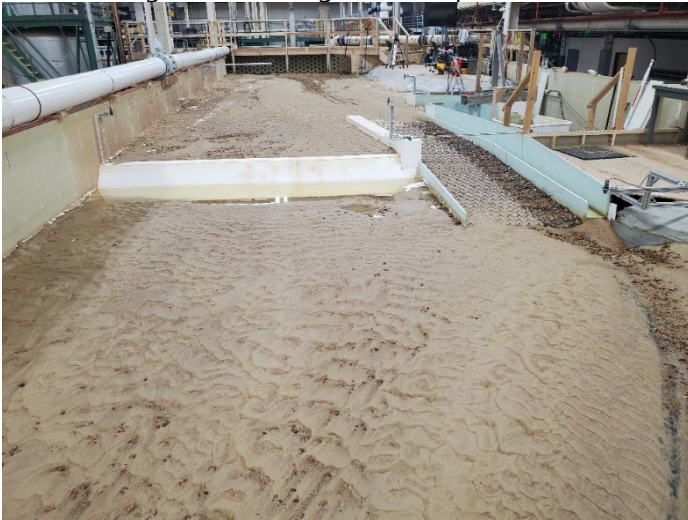
Figure B-36. View looking upstream for MOD-6 design with flushing channel open after 6,000 ft 3 /s flow rate.
