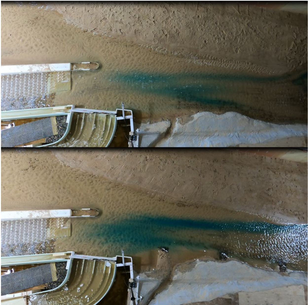
Figure 119. Photographs of flows with dye approaching the hardened ramp without groynes (top) and with groynes (bottom) at 3,000 ft 3 /s.
