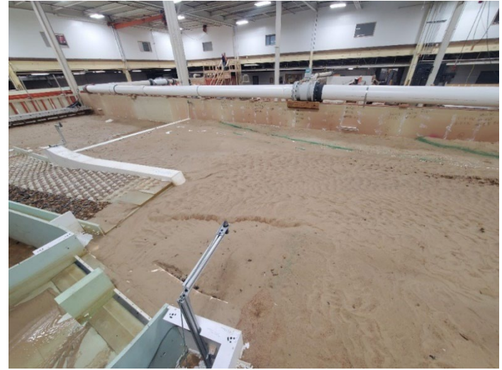
Figure B-3. View looking downstream after dewatering for MOD-9 design with flushing channel closed at 3,000 ft 3 /s.
