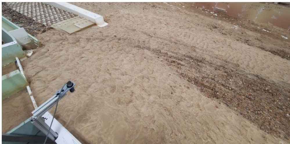
Figure B-121. MOD-6 flushing channel closed at 6,000 ft 3 /s after a 2 hr run duration.
