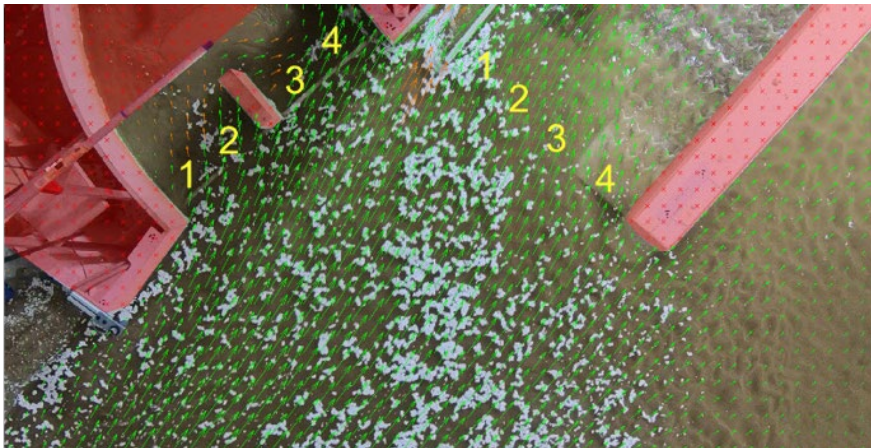
Figure B-48. Surface velocity vector map in area upstream of diversion intake (left) and hardened ramp (right) for MOD-6 design with flushing channel open at 6,000 ft 3 /s river flow.
