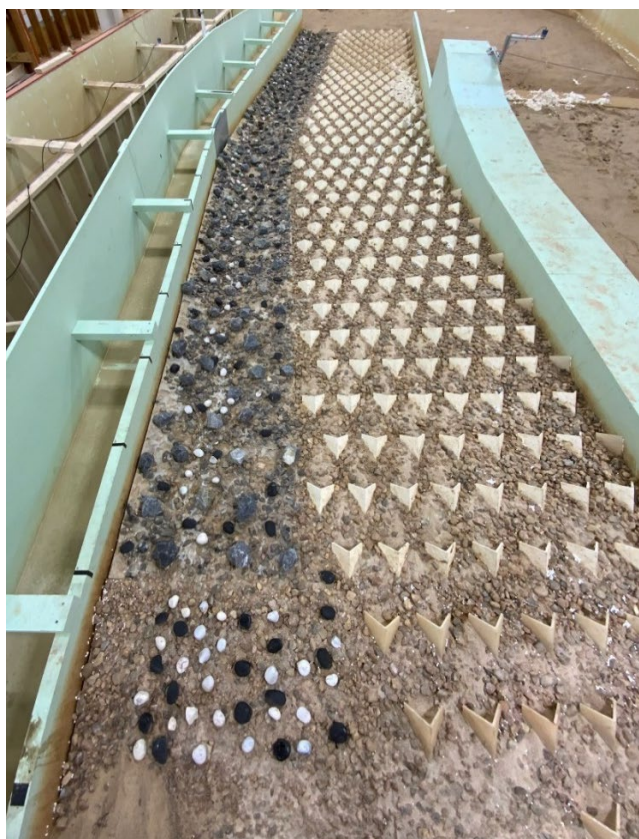
Figure 132. Version 2 of low flow channel rocks shown extending down the hardened ramp.
