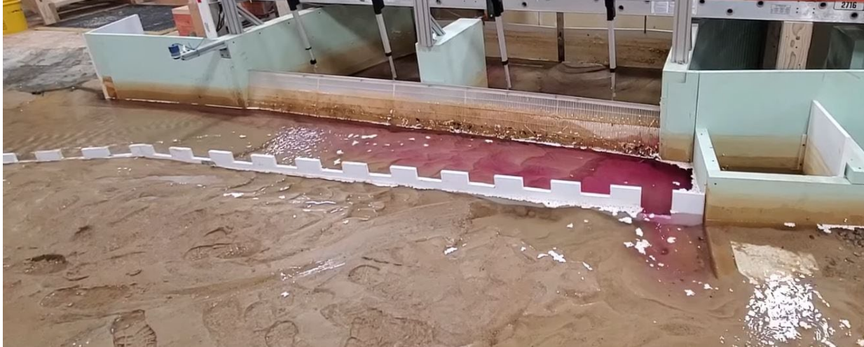
Figure 160. Dye test of the castle training wall structure upstream of intake. River flow was set to 100 \text{ ft}^3/\text{s} , with approximately 50 \text{ ft}^3/\text{s} diverted into the intake.
