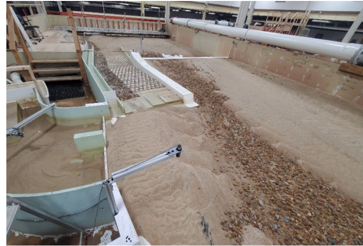
Figure B-97. View looking downstream after dewatering for MOD-9 design with flushing channel open at 30,000 ft 3 /s.
