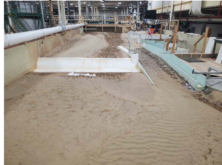
Figure B-98. View looking upstream for MOD-9 design with flushing channel open after 30,000 ft 3 /s flow rate.
