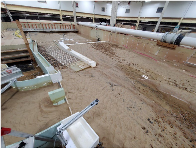
Figure B-69. View looking downstream after dewatering for MOD-6 design with flushing channel removed at 12,000 ft 3 /s.
