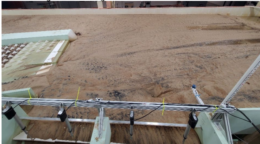
Figure C-10. Views looking upstream from diversion canal of area upstream of diversion intake (bottom) and hardened ramp (left) for MOD-6 design with flushing channel closed at 6,000 ft 3 /s river flow.
