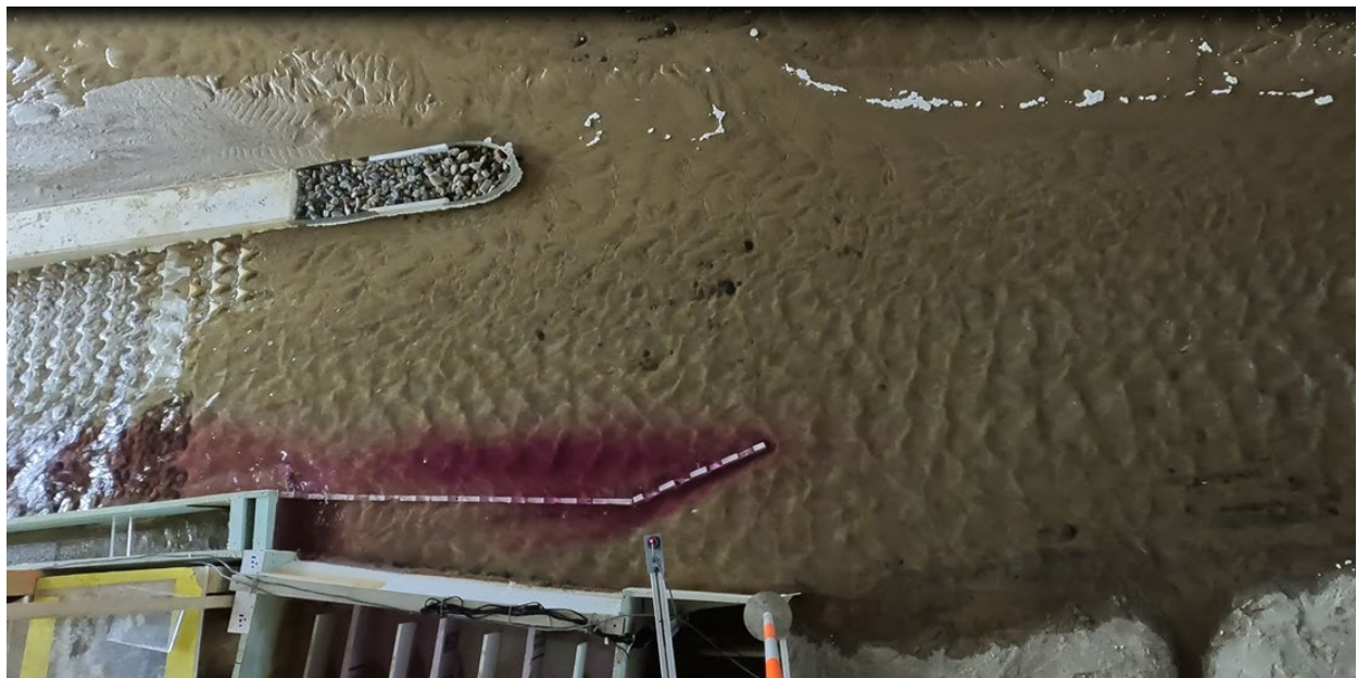
Figure 78. Photograph of dye approaching the hardened ramp with a castle training wall and flushing channel at 3,000 ft 3 /s.
