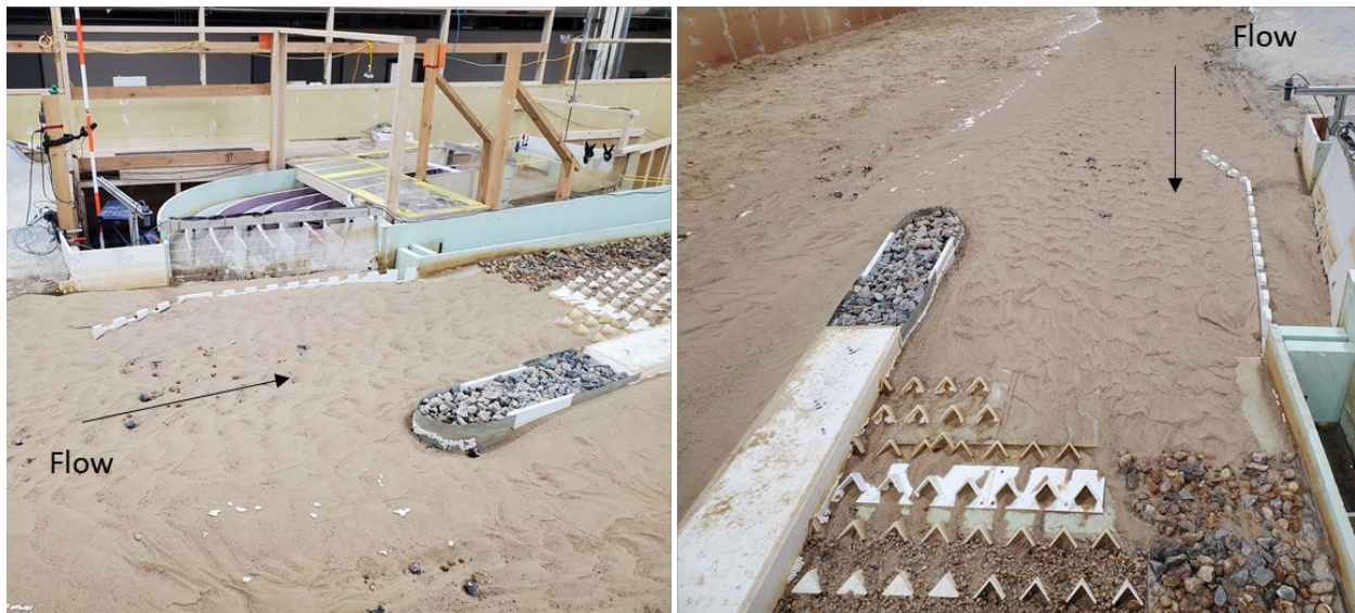
Figure 80. Photographs of the sediment bedforms upstream of hardened ramp with a castle training wall and flushing channel at 3,000 ft 3 /s.
