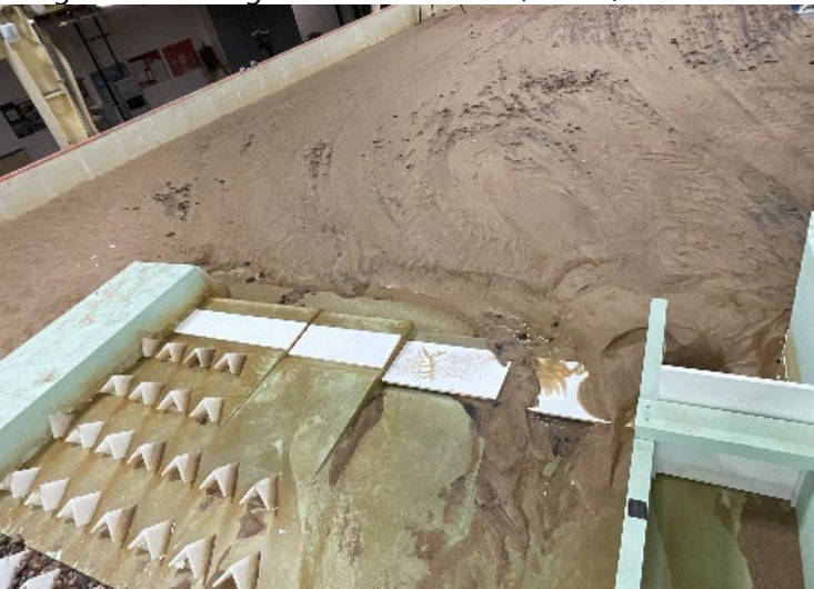
Figure C-38. View of ramp exit looking upstream from left bank for MOD-6 design with flushing channel closed after 1,500 ft 3 /s flow rate.
