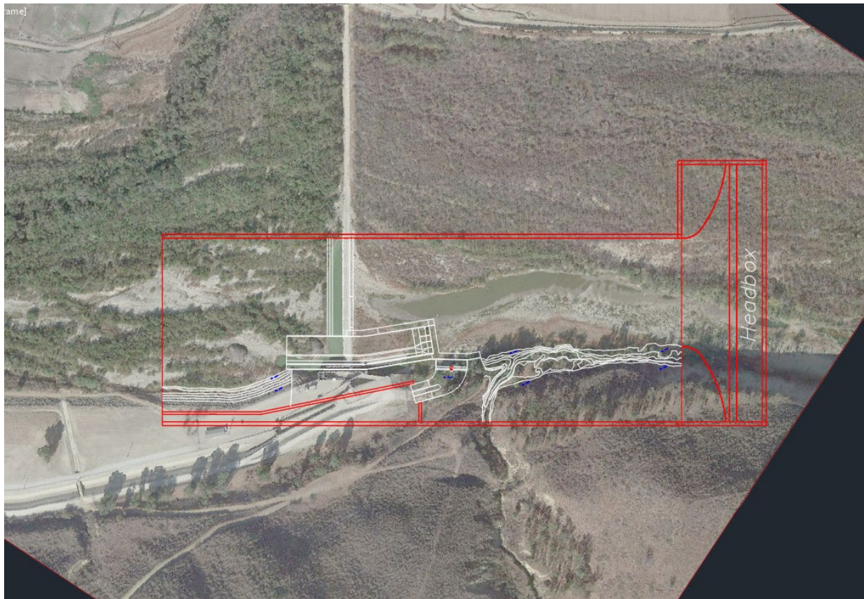
Figure 3. Overlay of 1:24 scale physical model box (red) on aerial photo of site showing model extents.
