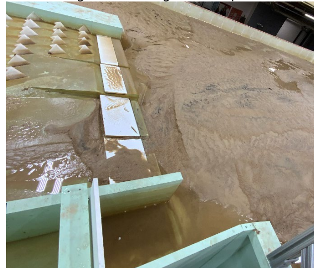
Figure C-8. View of ramp exit looking from left bank for MOD-9 design with flushing channel open after 6,000 ft 3 /s flow rate.
