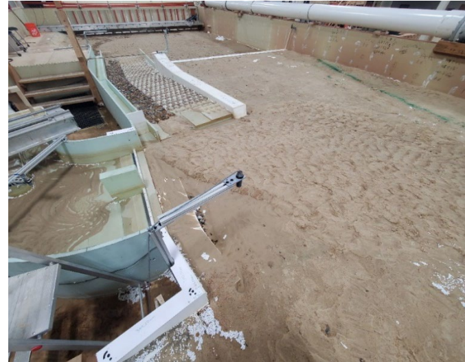
Figure B-7. View looking downstream after dewatering for MOD-9 design with flushing channel open at 3,000 ft 3 /s.
