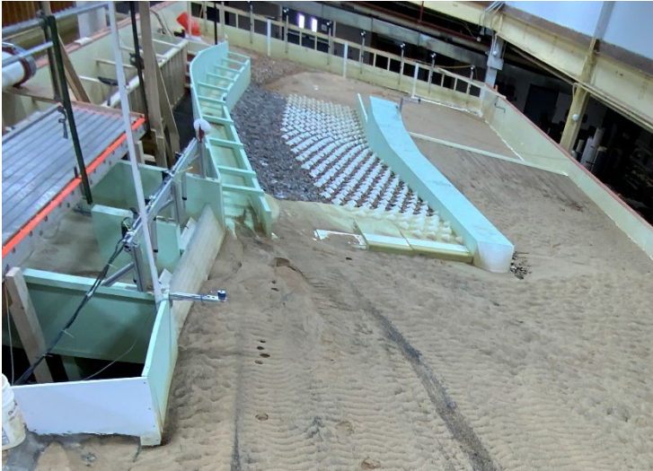
Figure C-5. View looking downstream after dewatering for MOD-6 design with flushing channel open at 6,000 ft 3 /s.
