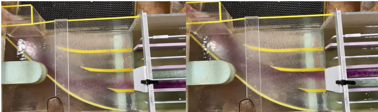
Figure 109. Photographs showing flow patterns with dye exiting the outside (left) and inside (right) channels of Bay 2. Sluicing flow was approximately 200 ft 3 /s.
