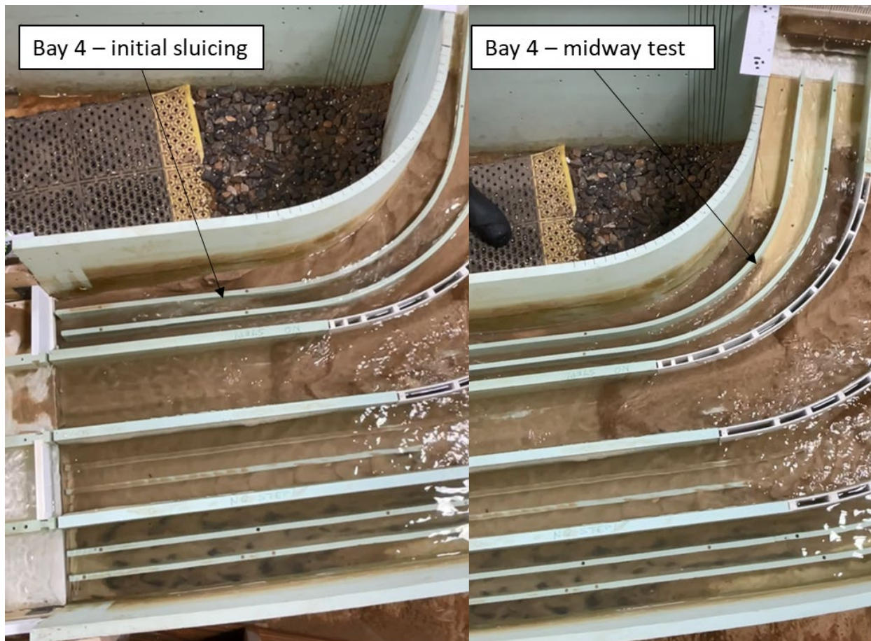
Figure 103. Photographs showing sluicing flows in Bay 4 with dual guide walls.
