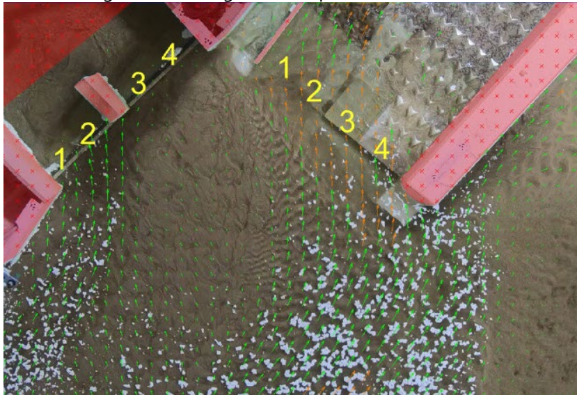
Figure B-18. Surface velocity vector map in area upstream of diversion intake (left) and hardened ramp (right) for MOD-6 design with flushing channel open at 3,000 ft 3 /s river flow.
