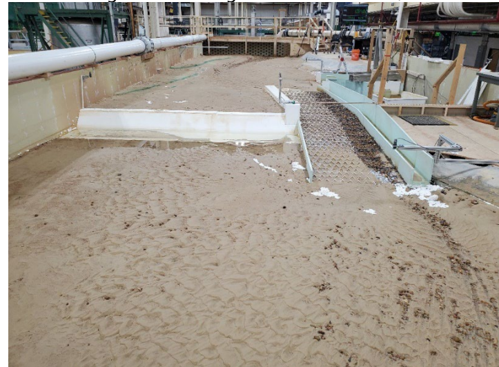
Figure B-4. View looking upstream for MOD-9 design with flushing channel closed after 3,000 ft 3 /s flow rate.
