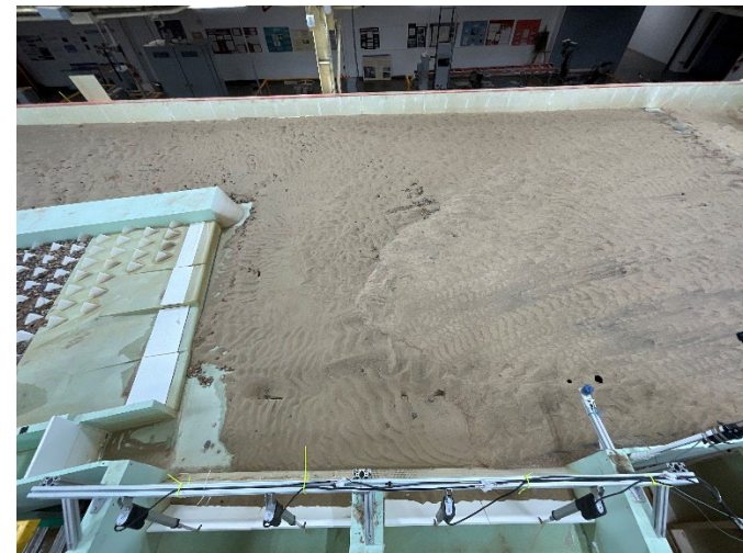
Figure C-50. View looking upstream from diversion canal of area upstream of diversion intake (bottom) and hardened ramp (left) for MOD-9 design with flushing channel open at 1,500 ft 3 /s river flow (PIV data not available).
