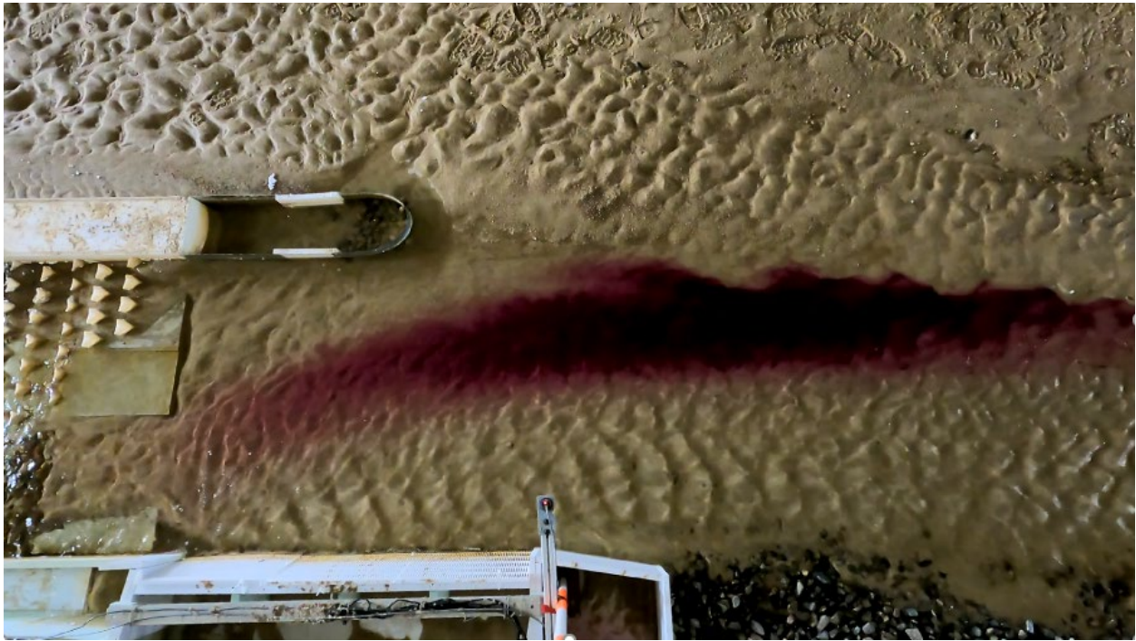
Figure 52. Photograph of dye approaching the hardened ramp without a flushing channel at 1,500 ft 3 /s.
