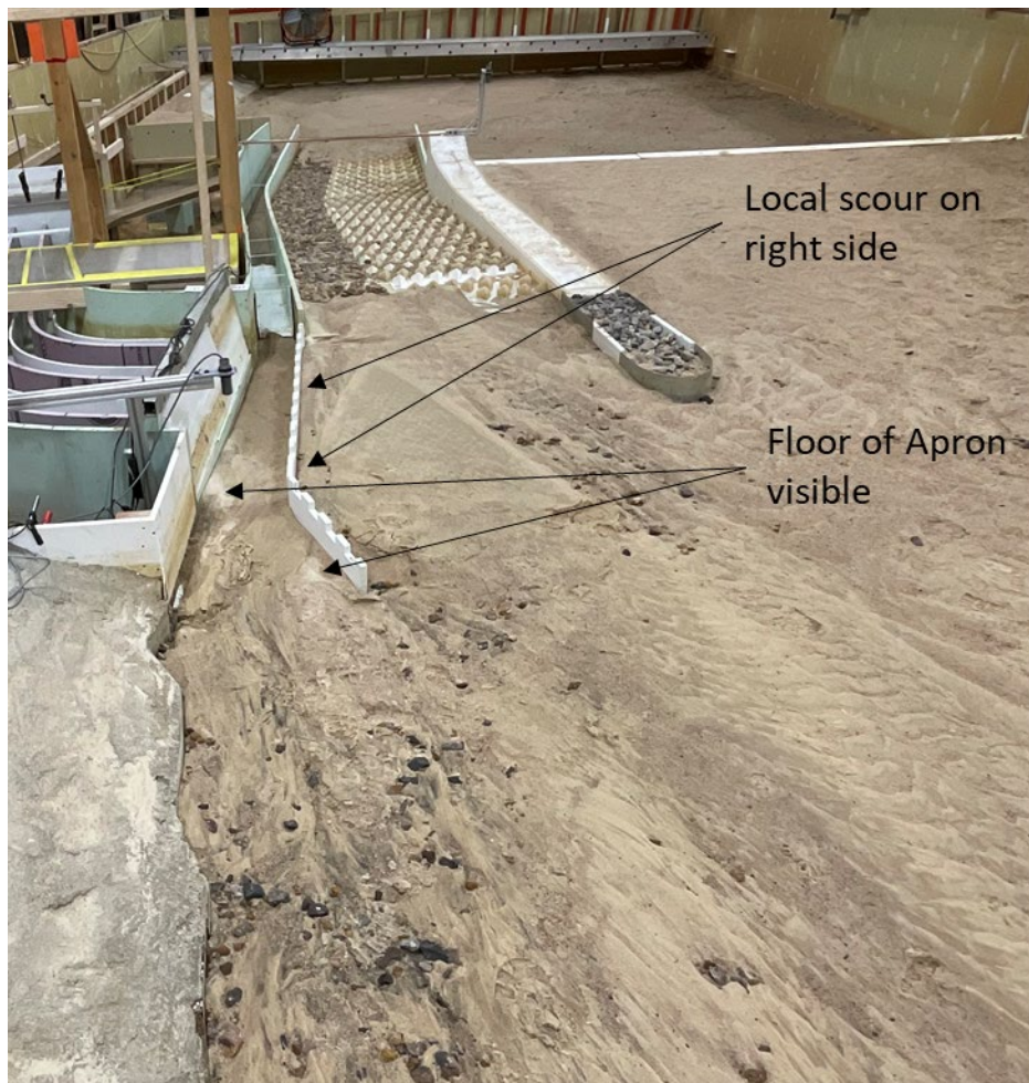
Figure 91. Photograph of bedform upstream of the hardened ramp and canal intake after a flushing operation at 3,000 ft 3 /s.
