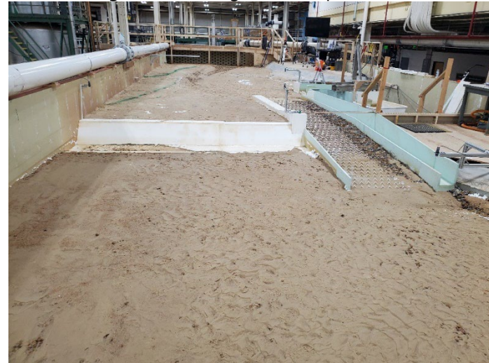
Figure B-8. View looking upstream for MOD-9 design with flushing channel open after 3,000 ft 3 /s flow rate.
