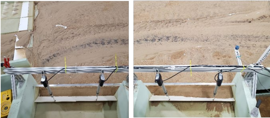
Figure C-64. Views looking upstream from diversion canal of area upstream of diversion intake (bottom) and hardened ramp (left) for MOD-6 design with flushing channel open at 270 ft 3 /s river flow.
