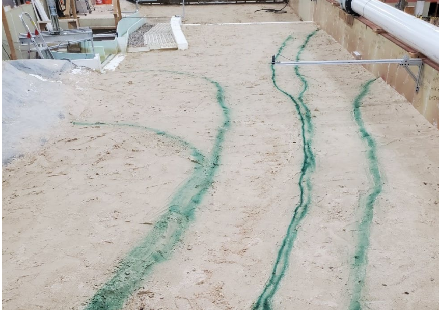
Figure 32. Upstream topography with flushing channel for MOD-6 design configuration.
