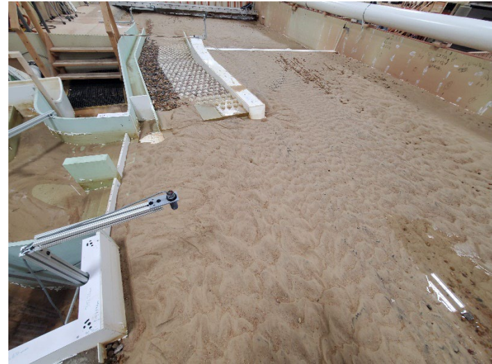
Figure B-63. View looking downstream after dewatering for MOD-9 design with flushing channel closed at 12,000 ft 3 /s.
