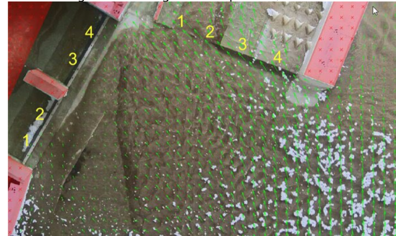
Figure B-20. Surface velocity vector map in area upstream of diversion intake (left) and hardened ramp (right) for MOD-9 design with flushing channel closed at 3,000 ft 3 /s river flow.
