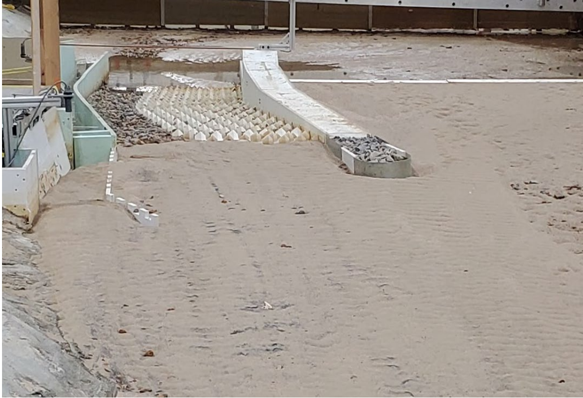
Figure 89. Photograph of bedform upstream of the hardened ramp and canal intake after 6,000 ft 3 /s river flow and 825 ft 3 /s diversion.
