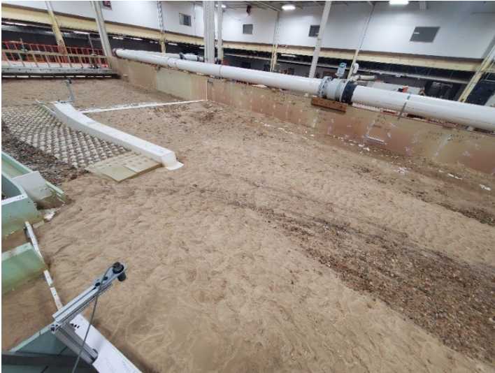
Figure B-31. View looking downstream after dewatering for MOD-6 design with flushing channel closed at 6,000 ft 3 /s.
