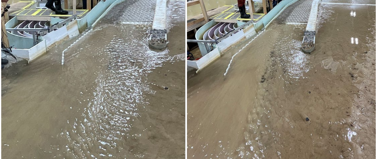
Figure 88. Photographs of a flushing operation at 3,000 ft 3 /s near the beginning of flushing (left) and midway through flushing (right). Looking downstream.
