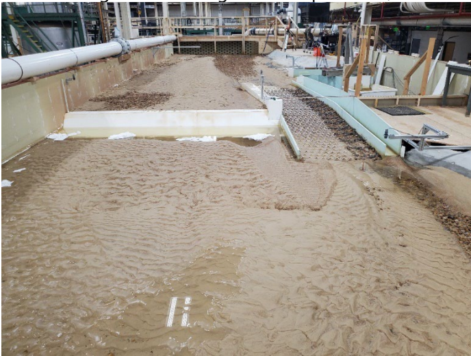
Figure B-66. View looking upstream for MOD-6 design with flushing channel open after 12,000 ft 3 /s flow rate.
