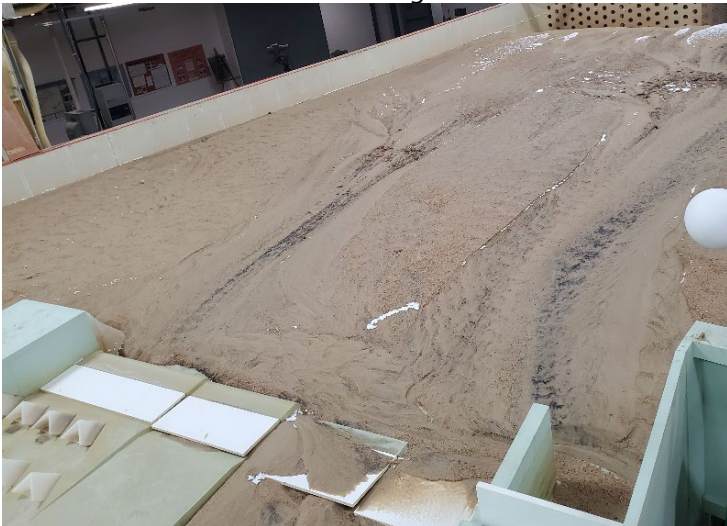
Figure C-58. View looking upstream for MOD-6 design with flushing channel open after 270 ft 3 /s flow rate.
