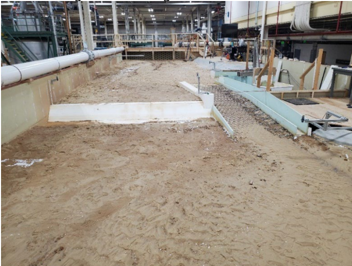
Figure B-2. View looking upstream for MOD-6 design with flushing channel closed after 3,000 ft 3 /s flow rate.
