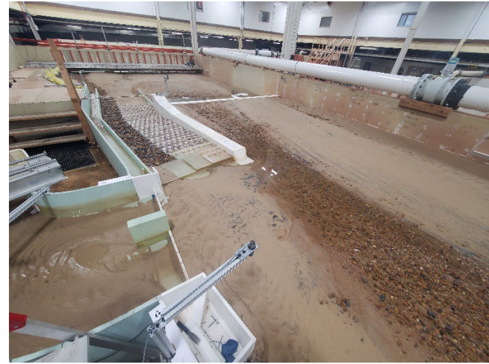
Figure B-101. View looking downstream after dewatering for MOD-9 design with flushing channel removed at 30,000 ft 3 /s.
