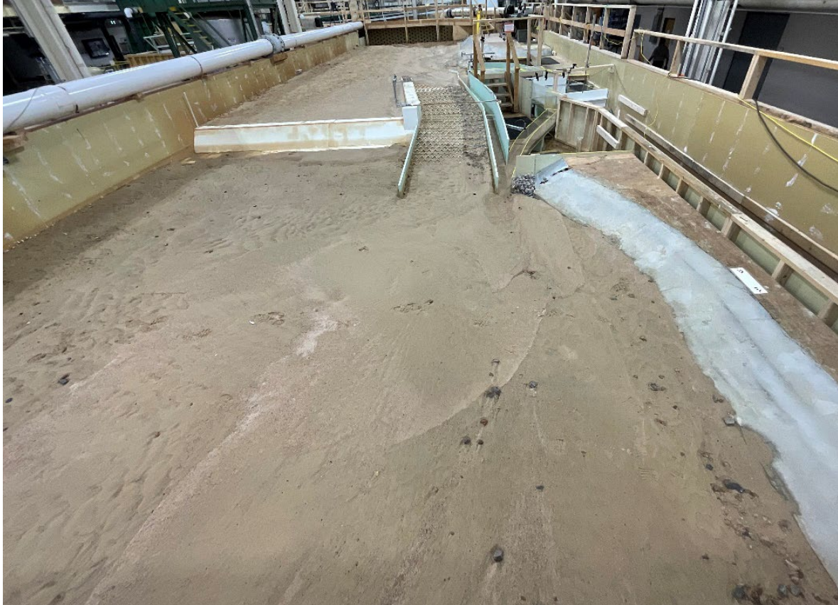
Figure 94. Photograph of bedforms downstream of the hardened ramp following combined flushing and sediment sluicing operations. Looking upstream.
