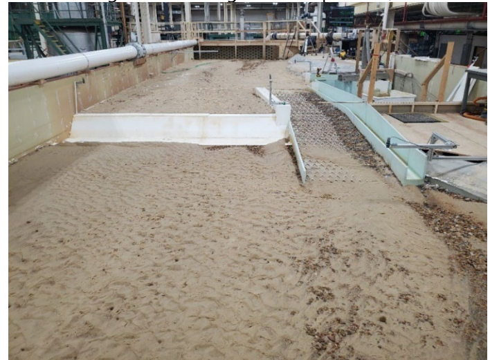
Figure B-38. View looking upstream for MOD-9 design with flushing channel open after 6,000 ft 3 /s flow rate.
