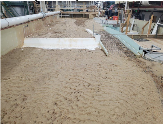
Figure B-32. View looking upstream for MOD-6 design with flushing channel closed after 6,000 ft 3 /s flow rate.
