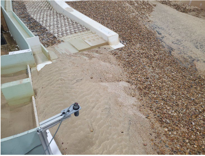
Figure B-95. View looking downstream after dewatering for MOD-6 design with flushing channel open at 30,000 ft 3 /s.
