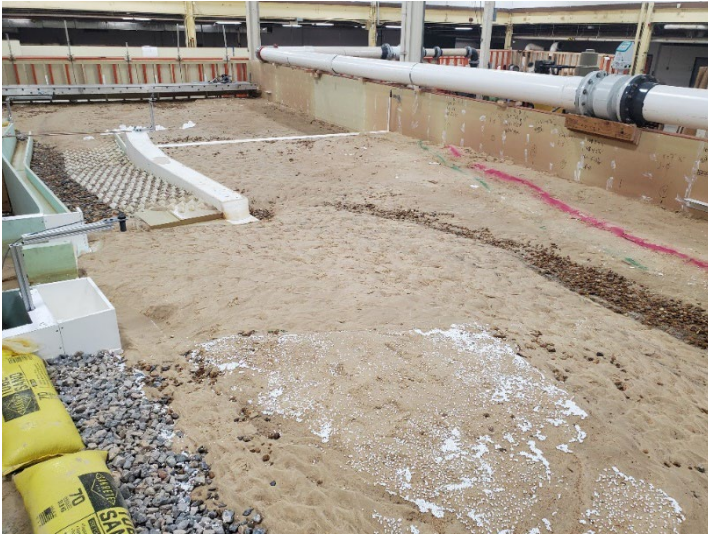
Figure B-9. View looking downstream after dewatering for MOD-6 design with flushing channel removed at 3,000 ft 3 /s.
