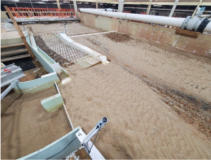
Figure B-61. View looking downstream after dewatering for MOD-6 design with flushing channel closed at 12,000 ft 3 /s.
