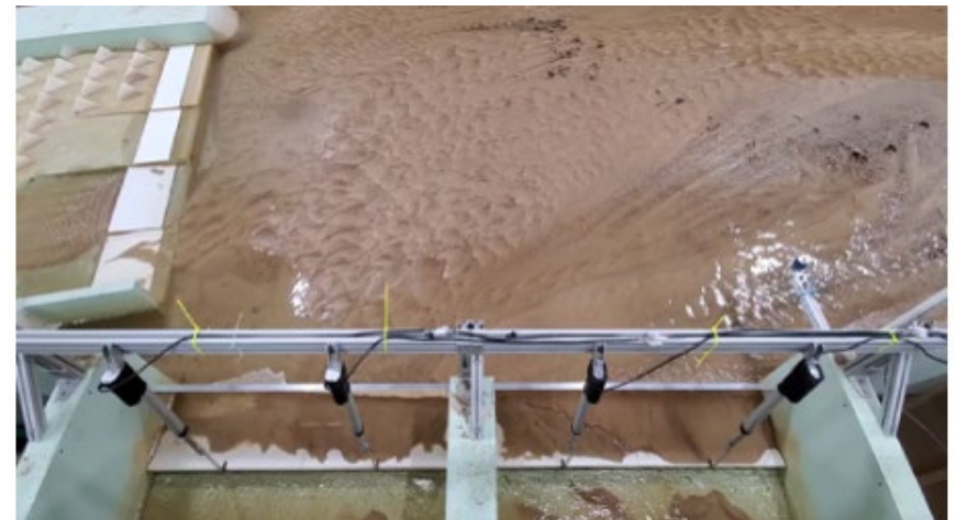
Figure C-62. View looking upstream from diversion canal of area upstream of diversion intake (bottom) and hardened ramp (left) for MOD-9 design with flushing channel closed at 270 ft 3 /s river flow.
