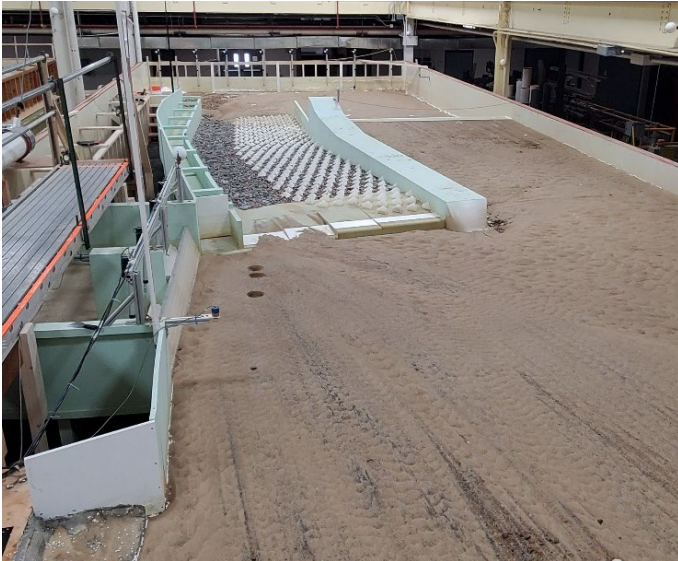
Figure C-41. View looking downstream after dewatering for MOD-6 design with flushing channel open at 1,500 ft 3 /s.
