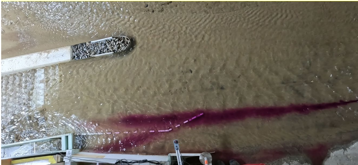
Figure 73. Photograph of dye approaching the hardened ramp with a castle training wall and flushing channel at 6,000 ft 3 /s.
