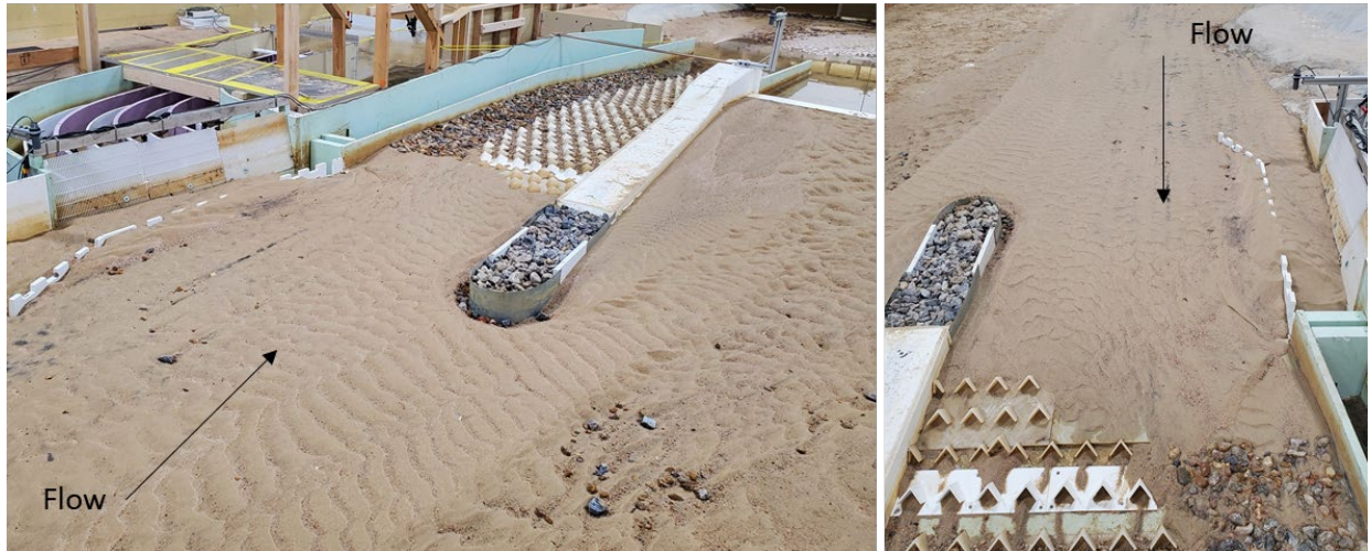
Figure 75. Photographs of the sediment bedforms upstream of hardened ramp with a castle training wall and flushing channel at 6,000 ft 3 /s.
