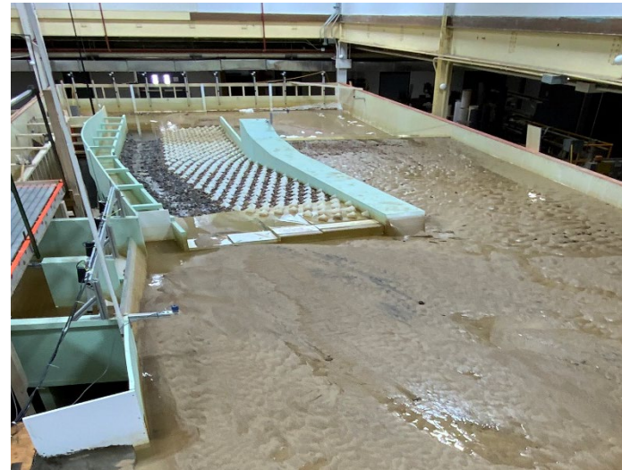
Figure C-7. View looking downstream after dewatering for MOD-9 design with flushing channel open at 6,000 ft 3 /s.
