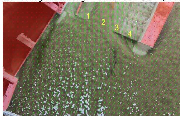
Figure B-80. Surface velocity vector map in area upstream of diversion intake (left) and hardened ramp (right) for MOD-9 design with flushing channel open at 12,000 ft 3 /s river flow.
