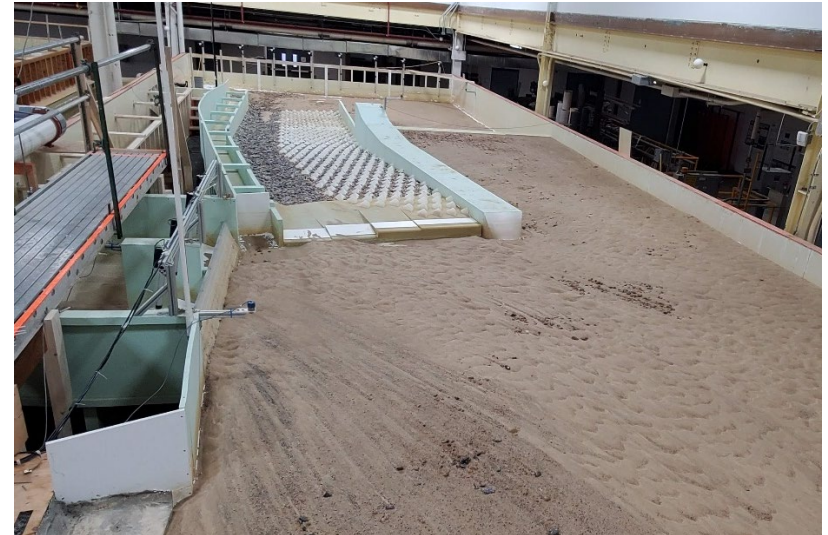
Figure C-39. View looking downstream after dewatering for MOD-9 design with flushing channel closed at 1,500 ft 3 /s.
