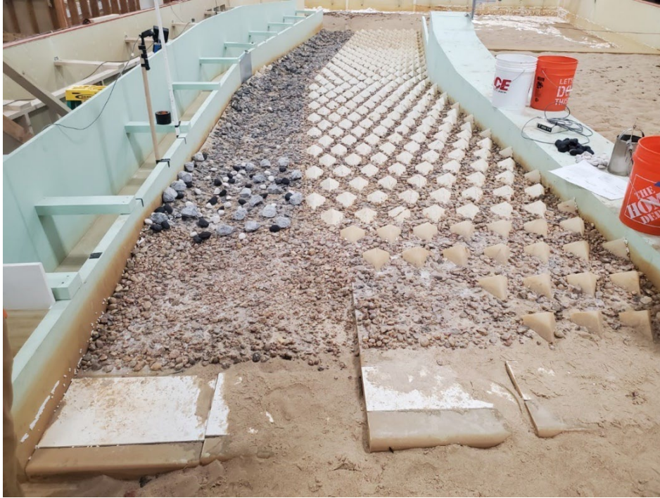
Figure 130. Version 1 of the low flow section of rocks added in for one cycle (40-ft) on the hardened ramp (looking downstream).
