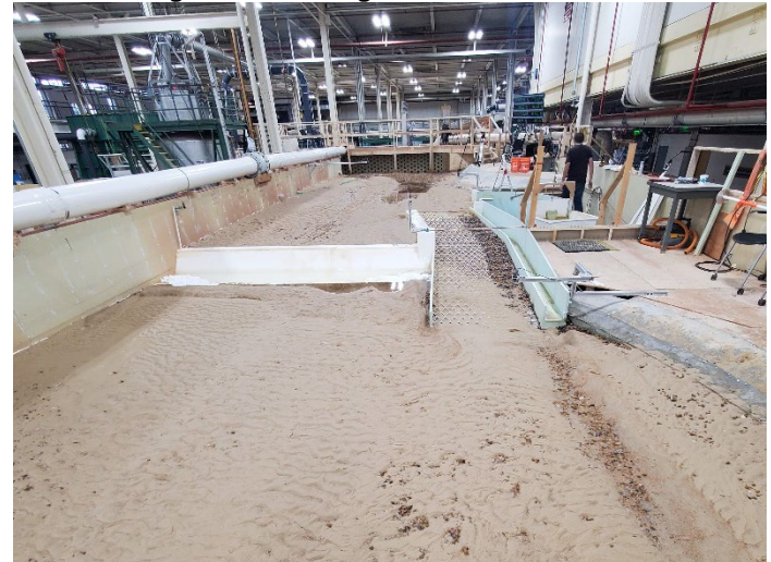
Figure B-64. View looking upstream for MOD-9 design with flushing channel closed after 12,000 ft 3 /s flow rate.
