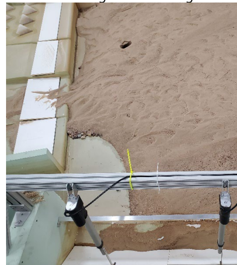
Figure C-20. View of ramp exit looking from left bank for MOD-9 design with flushing channel closed after 3,000 ft 3 /s flow rate.
