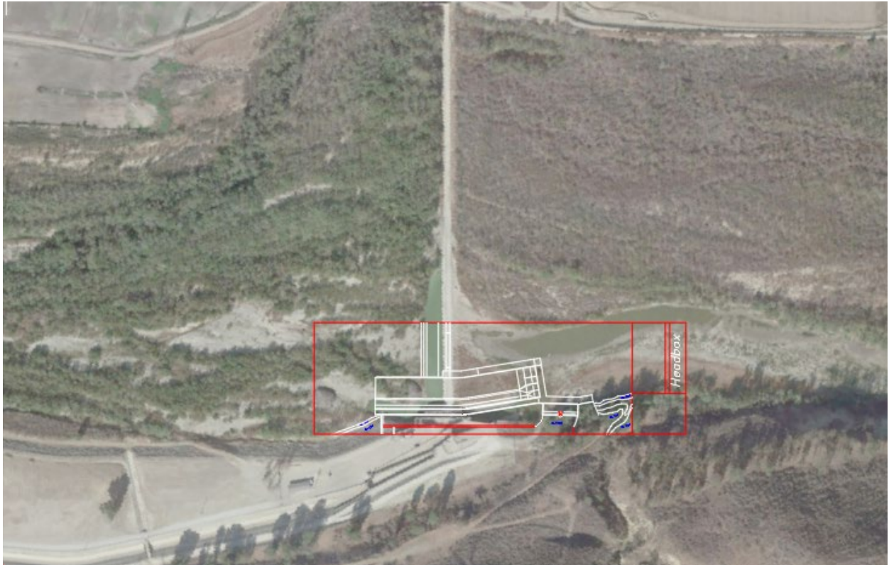
Figure 6. Overlay of 1:12 physical model box (red) on aerial photo of site showing model extents.
