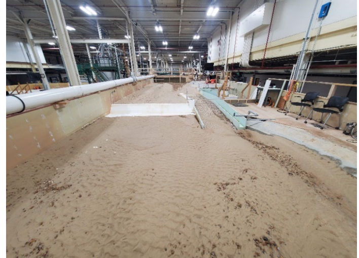
Figure B-68. View looking upstream for MOD-9 design with flushing channel open after 12,000 ft 3 /s flow rate.
