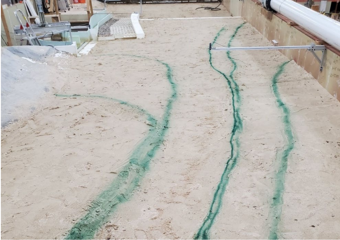
Figure 22. Photograph of upstream topography that was manually set before testing (looking downstream).
