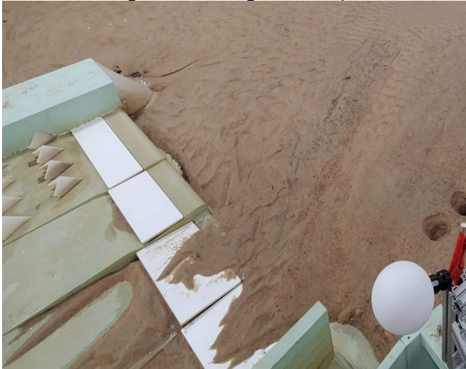
Figure C-42. View of ramp exit looking from left bank for MOD-6 design with flushing channel open after 1,500 ft 3 /s flow rate.
