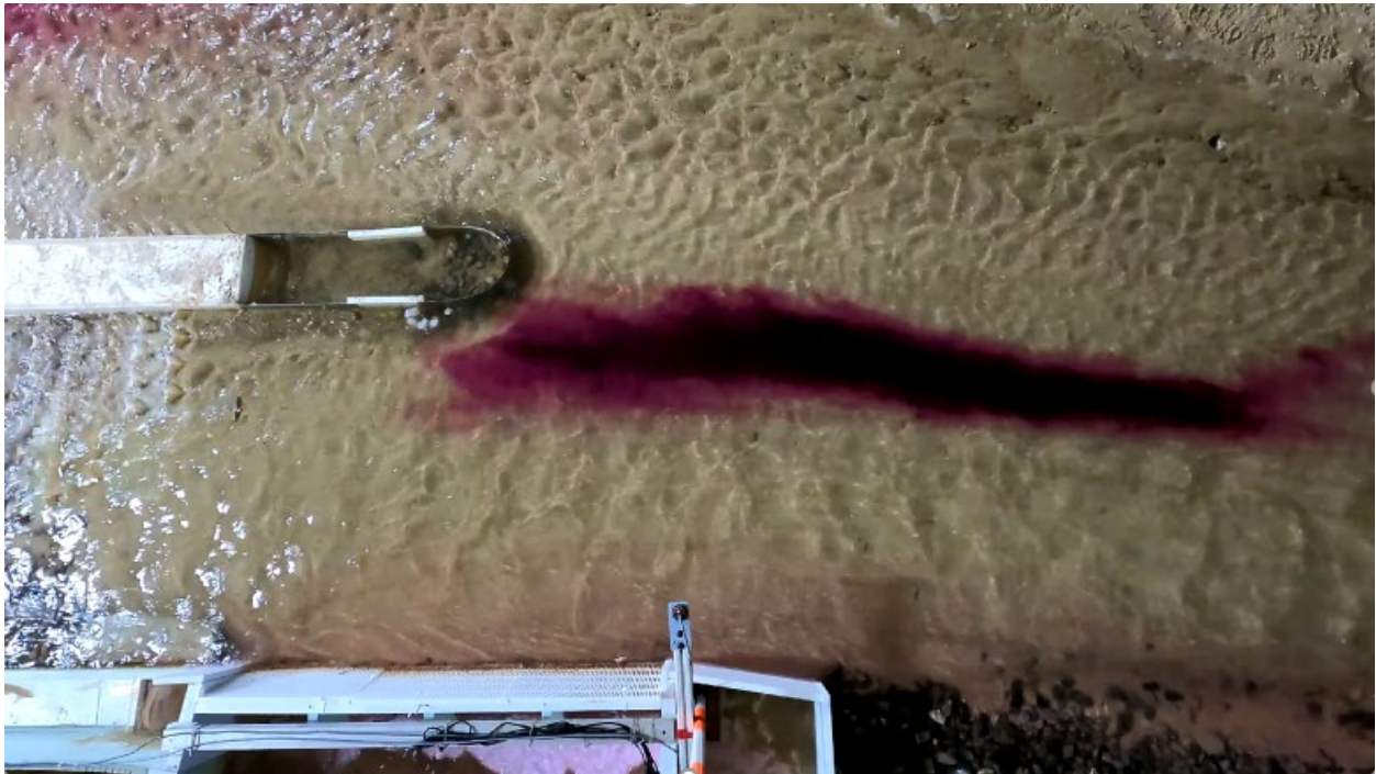
Figure 42. Photograph of dye approaching the hardened ramp without a flushing channel at 6,000 ft 3 /s.
