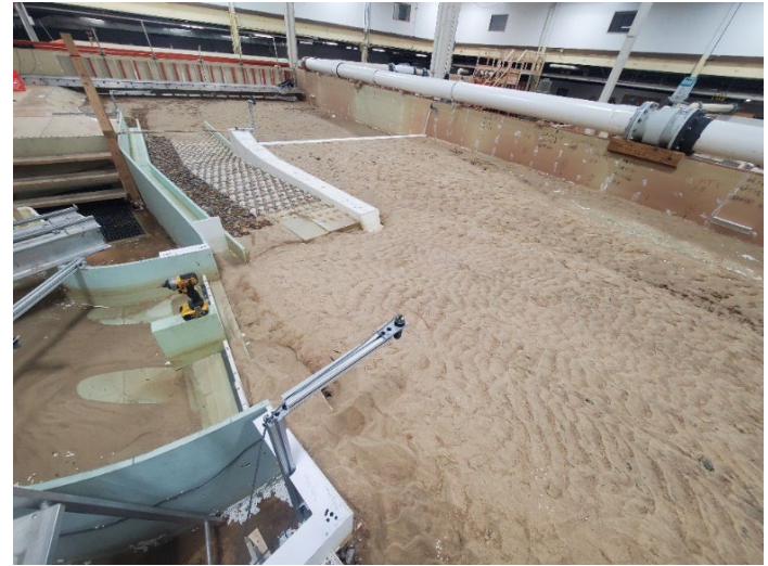
Figure B-37. View looking downstream after dewatering for MOD-9 design with flushing channel open at 6,000 ft 3 /s.
