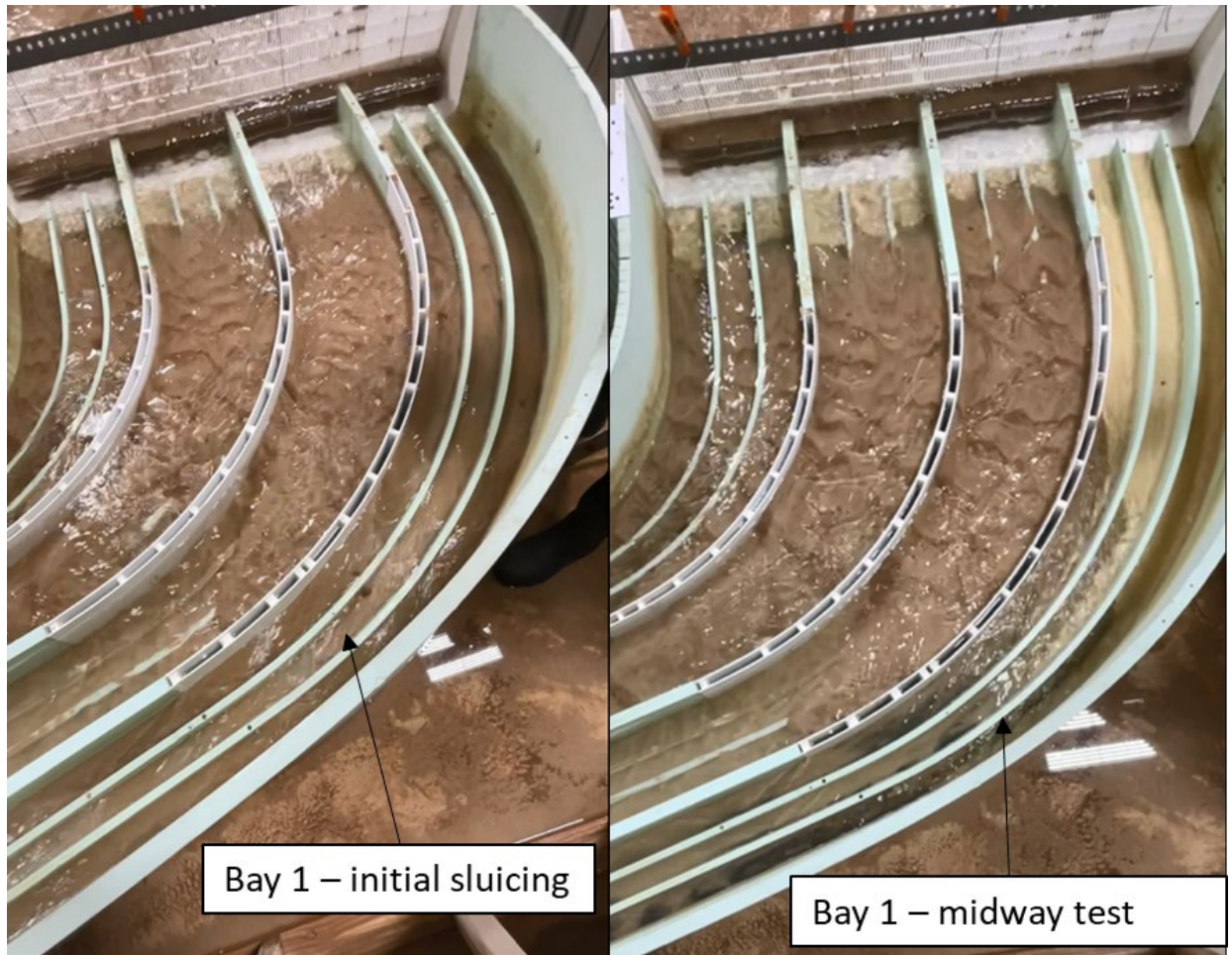
Figure 102. Photographs showing sluicing flows in Bay 1 with dual guide walls.
