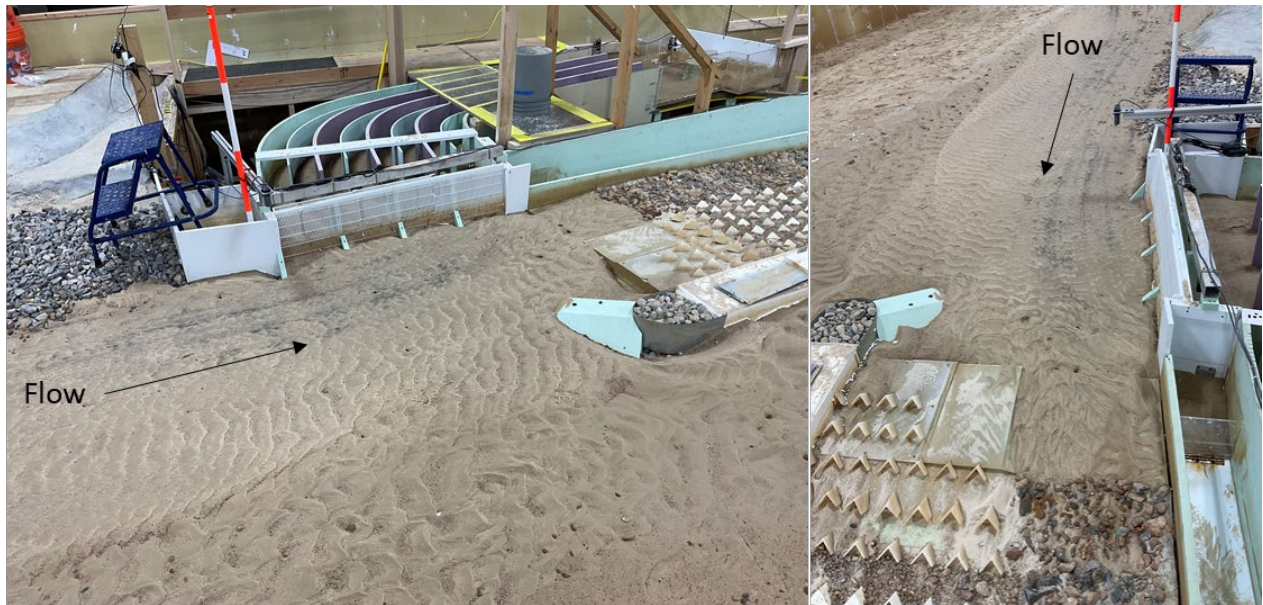
Figure 59. Photographs of the sediment bedforms upstream of hardened ramp without a flushing channel at 6,000 ft 3 /s with added sediment features.
