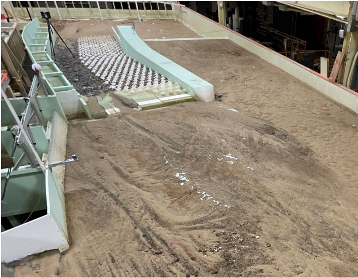
C-55. View looking downstream after dewatering for MOD-6 design with flushing channel closed at 270 ft 3 /s.
