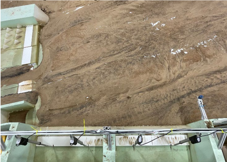
Figure C-60. View looking upstream from diversion canal of area upstream of diversion intake (bottom) and hardened ramp (left) for MOD-6 design with flushing channel closed at 270 ft 3 /s river flow.
