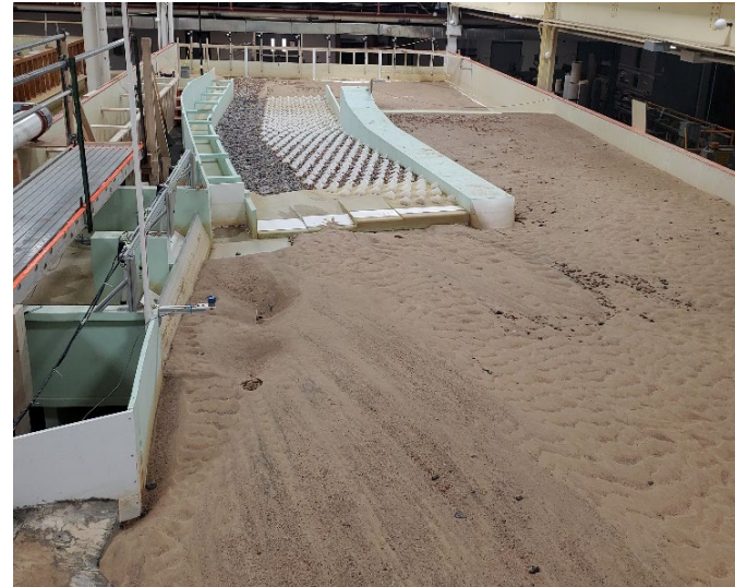
Figure C-19. View looking downstream after dewatering for MOD-9 design with flushing channel closed at 3,000 ft 3 /s.
