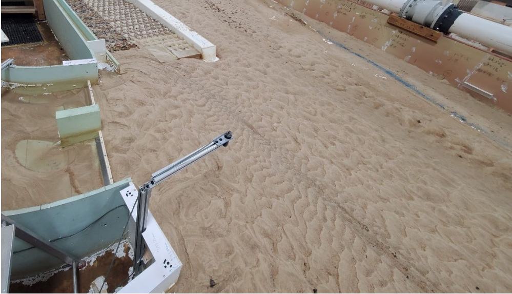
Figure B-123. MOD-9 flushing channel closed at 6,000 ft 3 /s after a 6.5 hr run duration.
