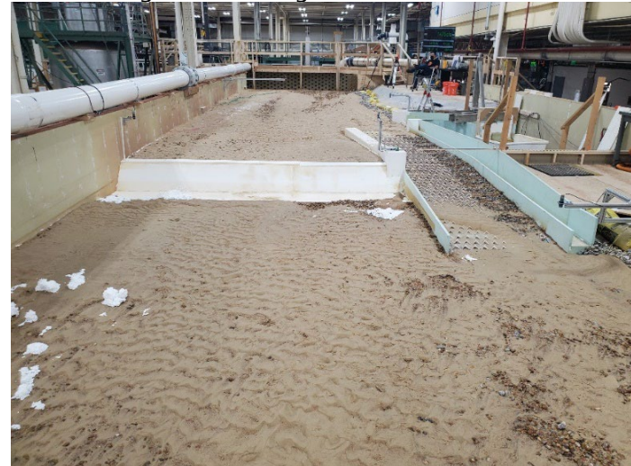
Figure B-42. View looking upstream for MOD-9 design with flushing channel removed after 6,000 ft 3 /s flow rate.
