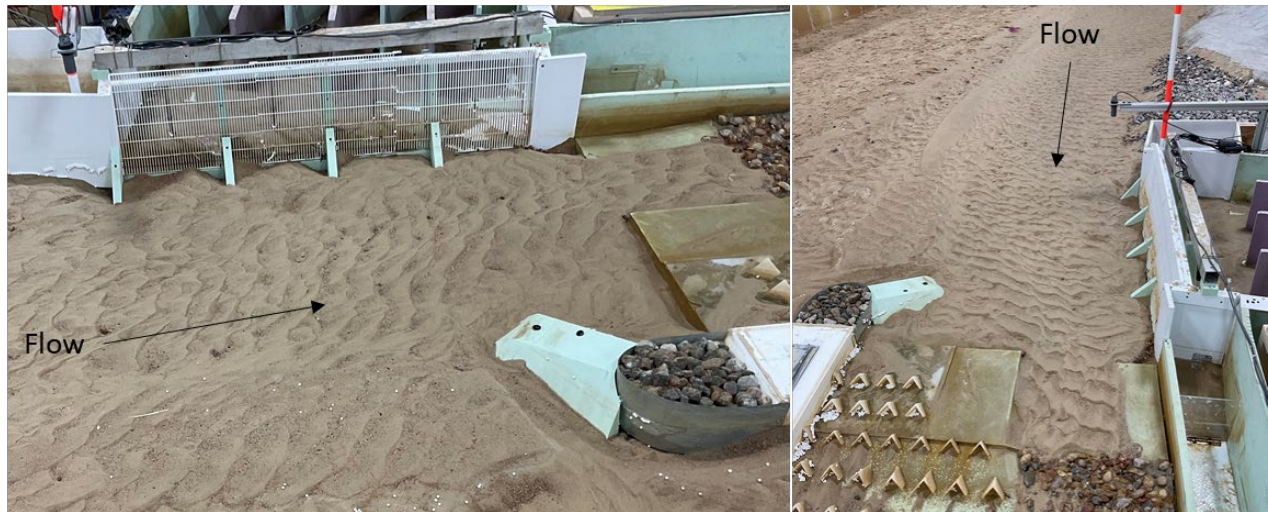
Figure 67. Photographs of the sediment bedforms upstream of hardened ramp without a flushing channel at 1,500 ft 3 /s with added sediment features.
