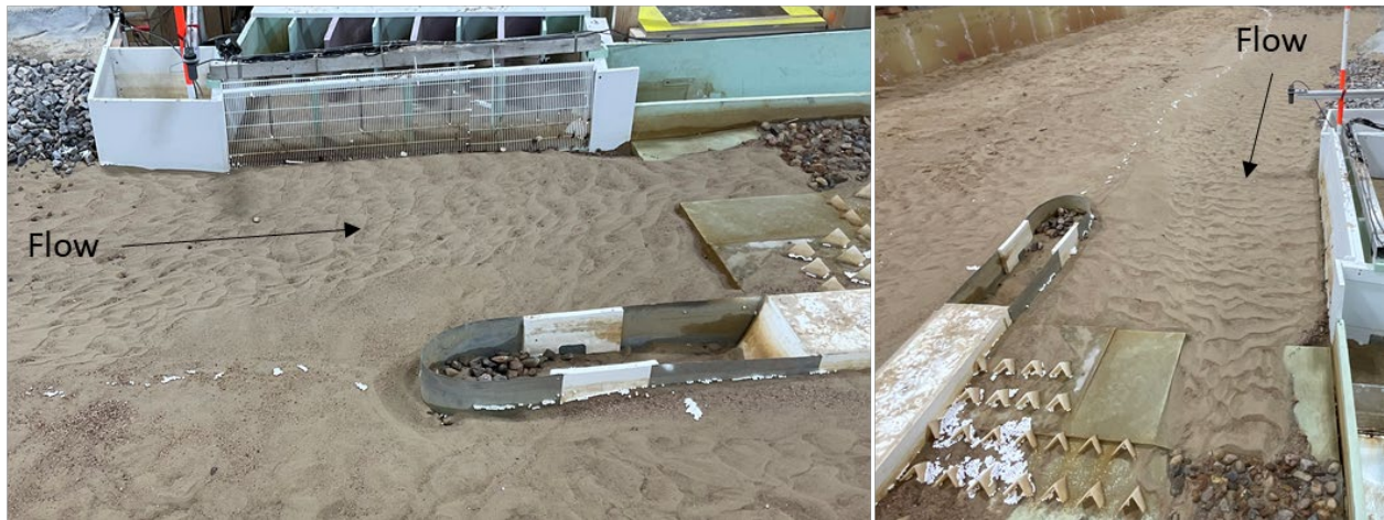
Figure 54. Photographs of the sediment bedforms upstream of hardened ramp without a flushing channel at 1,500 ft 3 /s.
