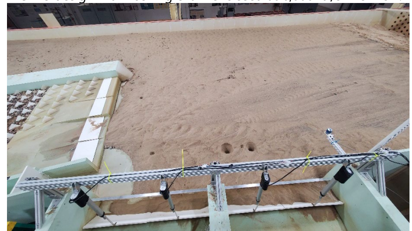
Figure C-12. Views looking upstream from diversion canal of area upstream of diversion intake (bottom) and hardened ramp (left) for MOD-9 design with flushing channel closed at 6,000 ft 3 /s river flow.
