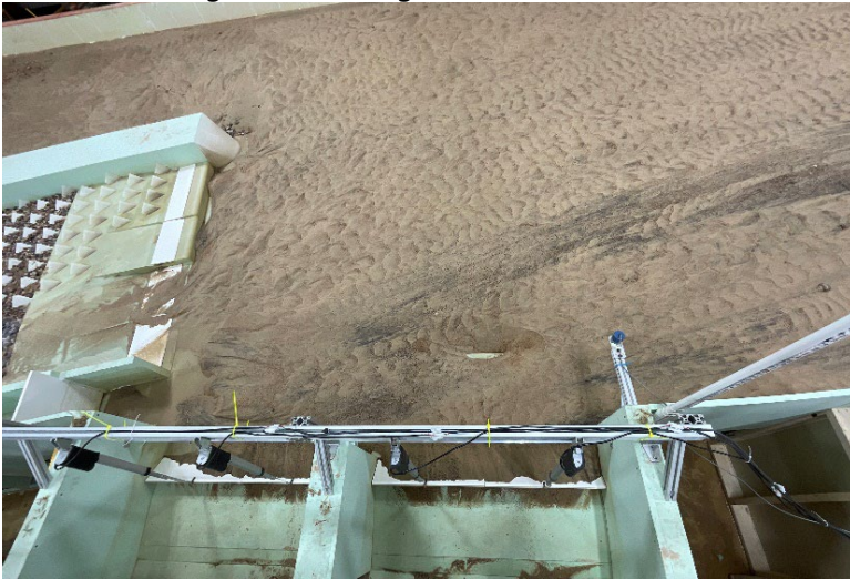
Figure C-26. View looking upstream from diversion canal of area upstream of diversion intake (bottom) and hardened ramp (left) for MOD-6 design with flushing channel closed at 3,000 ft 3 /s river flow.
