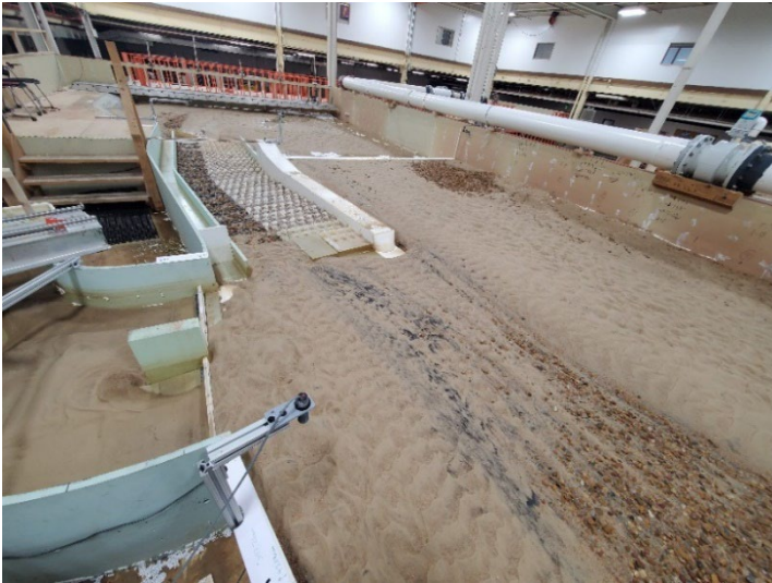
Figure B-65. View looking downstream after dewatering for MOD-6 design with flushing channel open at 12,000 ft 3 /s.
