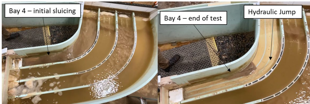
Figure 101. Photographs showing sluicing flows in Bay 4 without guide walls.
