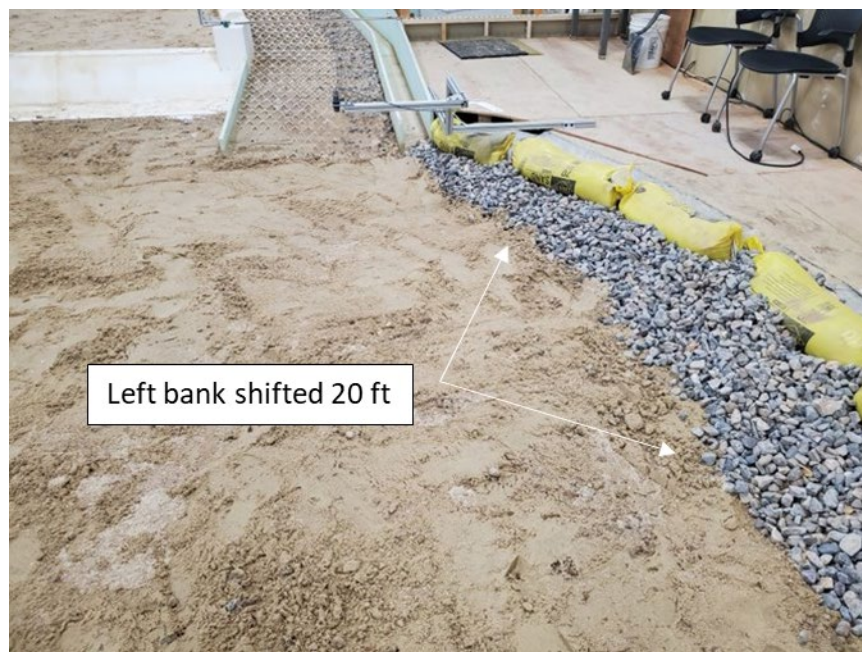
Figure 35. Downstream topography modification with flushing channel removed for MOD-6 design configuration, looking upstream.
