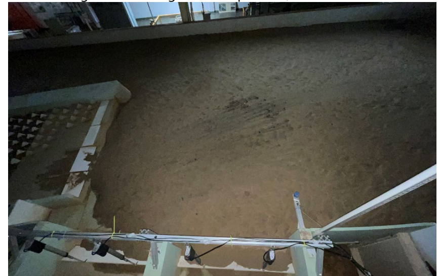
Figure C-32. View looking upstream from diversion canal of area upstream of diversion intake (bottom) and hardened ramp (left) for MOD-9 design with flushing channel open at 3,000 ft 3 /s river flow.
