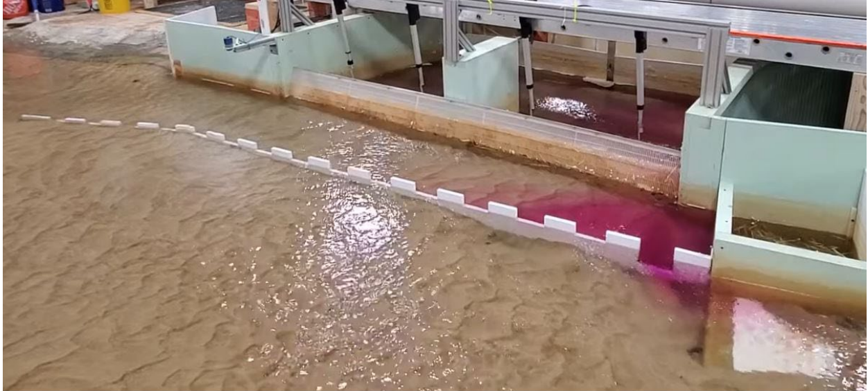
Figure 154. Dye test of the castle training wall structure upstream of intake. River flow was set to 800 ft 3 /s, with approximately 400 ft 3 /s diverted into the intake.
