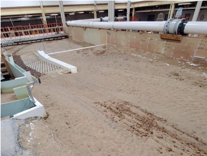
Figure B-35. View looking downstream after dewatering for MOD-6 design with flushing channel open at 6,000 ft 3 /s.
