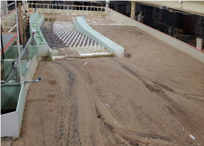
Figure C-57. View looking downstream after dewatering for MOD-6 design with flushing channel open at 270 ft 3 /s. The black features on top of the bedform are iron deposits from the sediment blend and are not larger cobble sized material.
