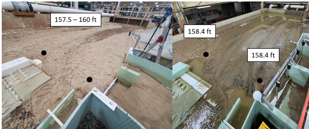
Figure 24. Photographic comparisons of sediment patterns after 6,000 ft 3 /s in the 1:24 model (left) and 1:12 model (right).
