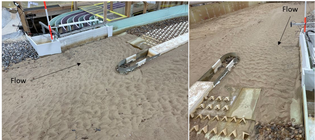
Figure 49. Photographs of the sediment bedforms upstream of hardened ramp without a flushing channel at 3,000 ft³/s.
