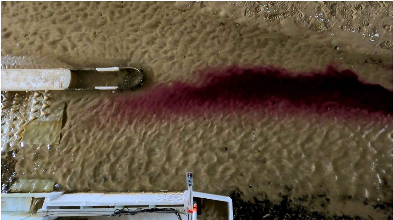
Figure 47. Photograph of dye approaching the hardened ramp without a flushing channel at 3,000 ft 3 /s.
