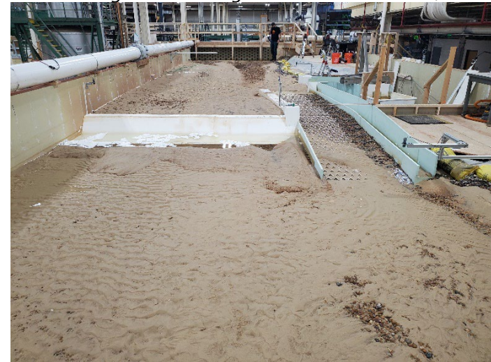
Figure B-72. View looking upstream for MOD-9 design with flushing channel removed after 12,000 ft 3 /s flow rate.
