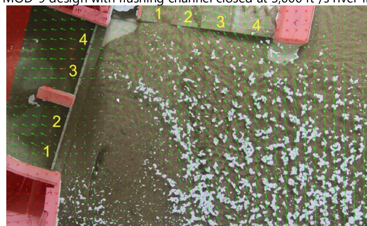
Figure B-16. Surface velocity vector map in area upstream of diversion intake (left) and hardened ramp (right) for MOD-9 design with flushing channel closed at 3,000 ft 3 /s river flow.
