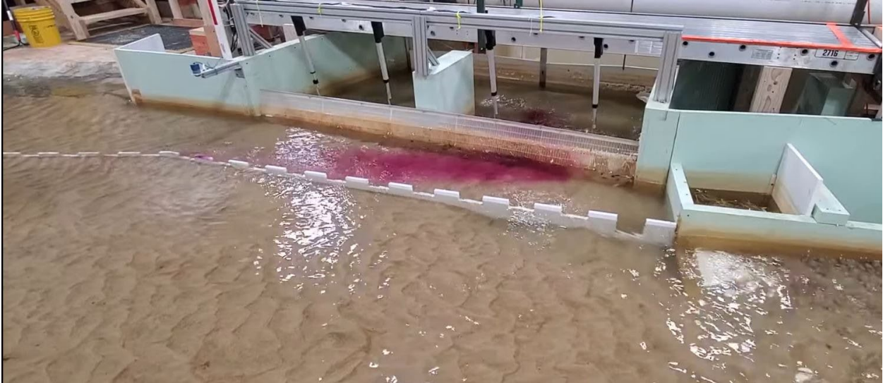
Figure 152. Dye test of the castle training wall structure upstream of intake. River flow was set to 1,500 \text{ft}^3/\text{s} , with approximately 750 \text{ft}^3/\text{s} diverted into the intake. At this flow, all dye was drawn into the intake. This was potentially caused by flow from the hardened ramp going towards the over the lowered notch at the downstream portion of the castle training wall and into the intake.
