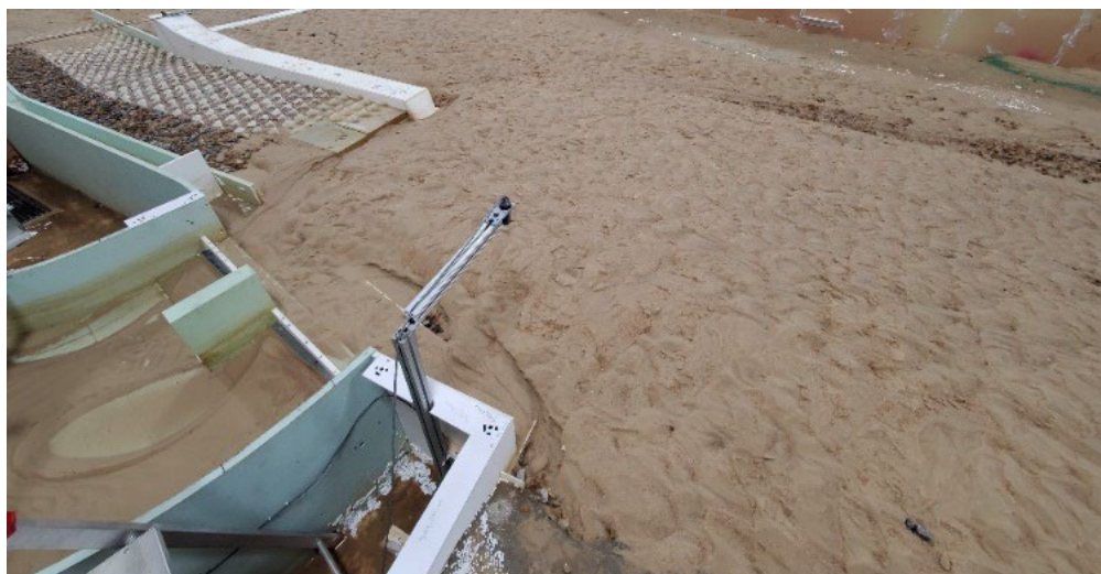
Figure B-122. MOD-9 flushing channel closed at 6,000 ft 3 /s after a 2 hr run duration.
