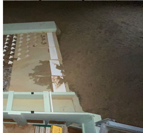
Figure C-24. View of ramp exit looking from left bank for MOD-9 design with flushing channel open after 3,000 ft 3 /s flow rate.
