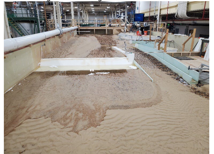
Figure B-94. View looking upstream for MOD-9 design with flushing channel closed after 30,000 ft 3 /s flow rate.
