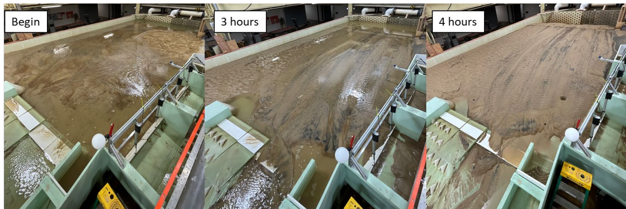
Figure 25. Timelapse photographs of the 1:12 model at 6,000 ft 3 /s to determine run times required for sediment patterns to reach equilibrium.
