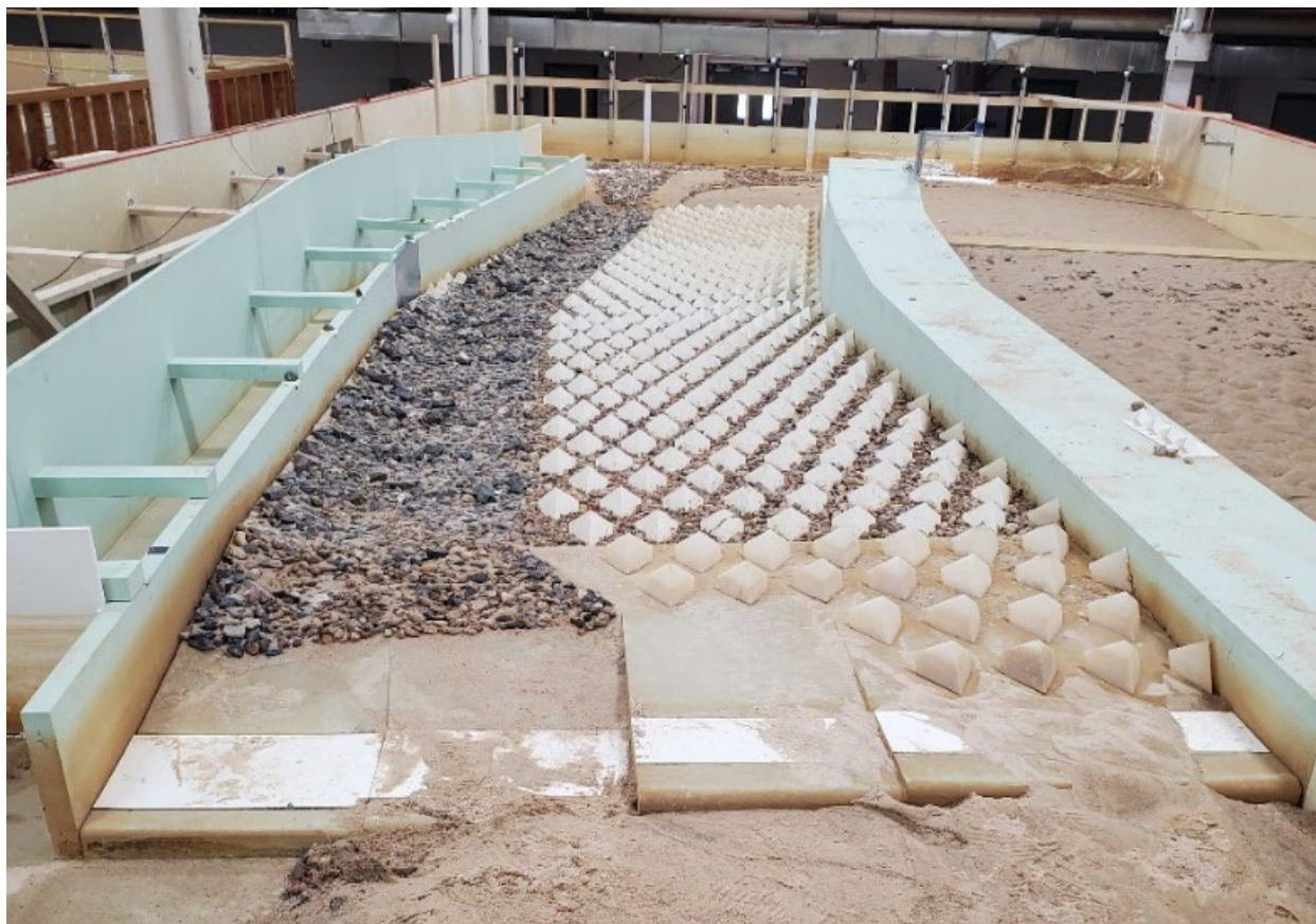
Figure 125. Original hardened ramp roughness configuration.
