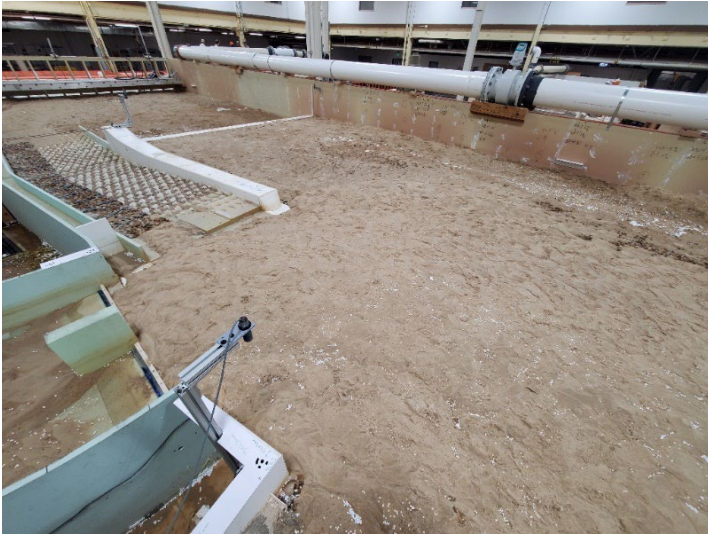
Figure B-1. View looking downstream after dewatering for MOD-6 design with flushing channel closed at 3,000 ft 3 /s.
