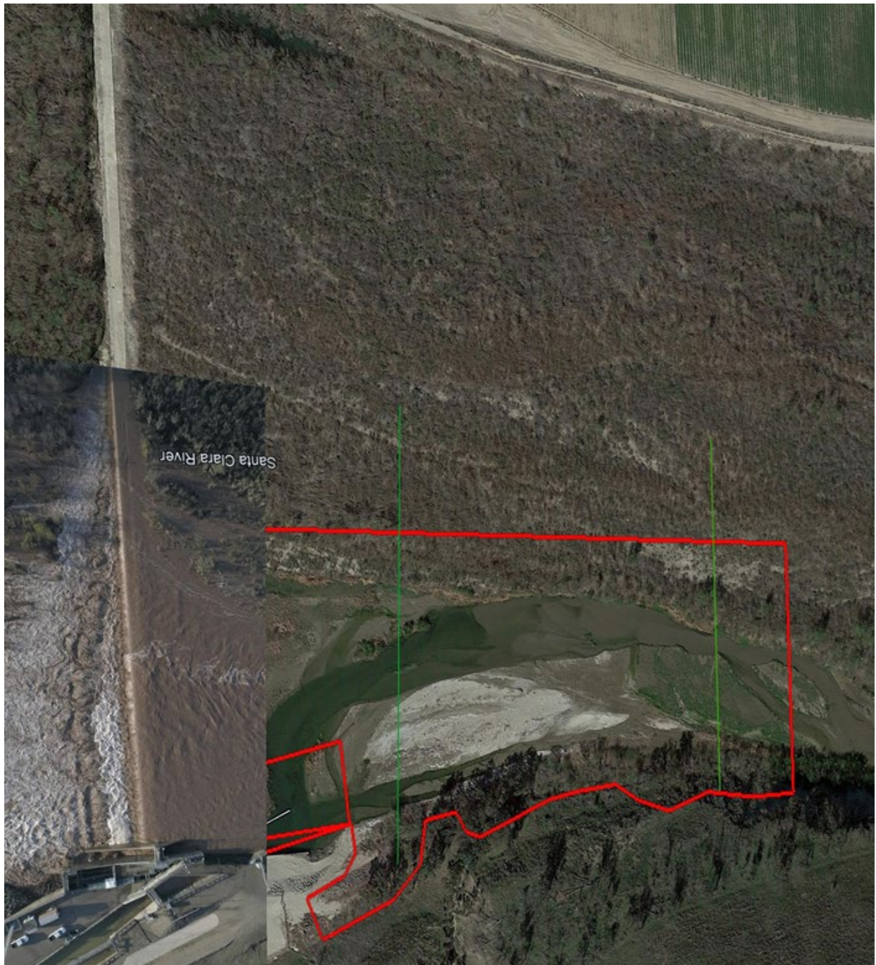
Figure 20. Aerial footage of 23,000 ft 3 /s discharge over the dam crest, overlaid on a lower-flow aerial image and approximate upstream extents of the 1:24 model, outlined in red.
