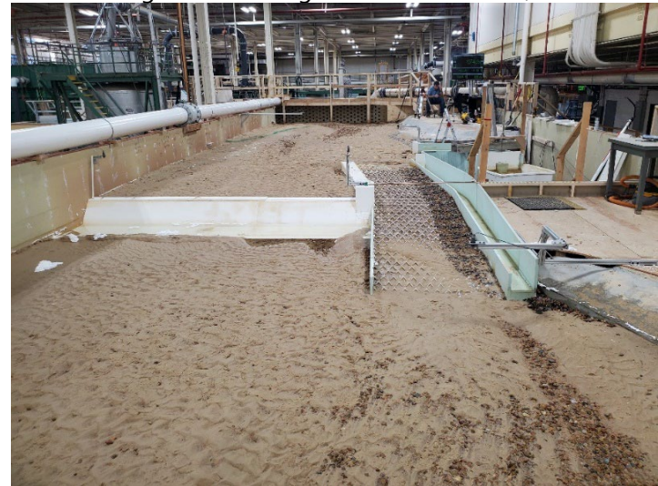
Figure B-34. View looking upstream for MOD-9 design with flushing channel closed after 6,000 ft 3 /s flow rate.
