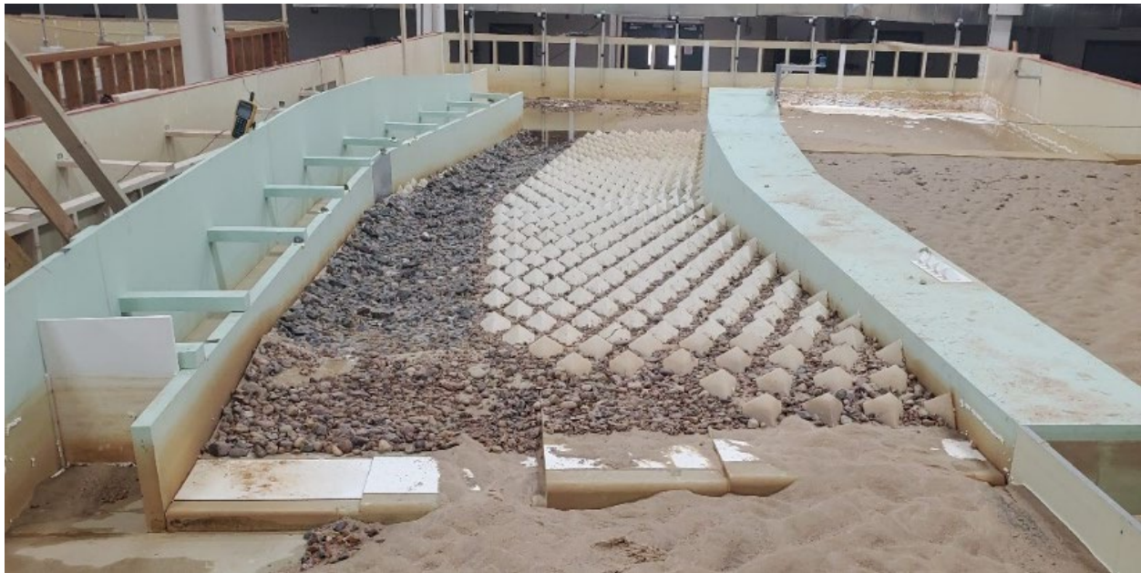
Figure 128. Hardened ramp with 1- to 2-ft-diameter rocks filled in to just downstream of the hardened ramp gates (looking downstream).
