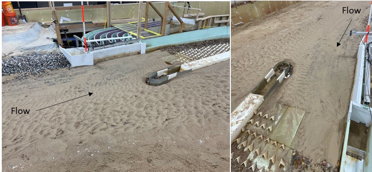
Figure 44. Photographs of the sediment bedforms upstream of hardened ramp without a flushing channel at 6,000 ft 3 /s.
