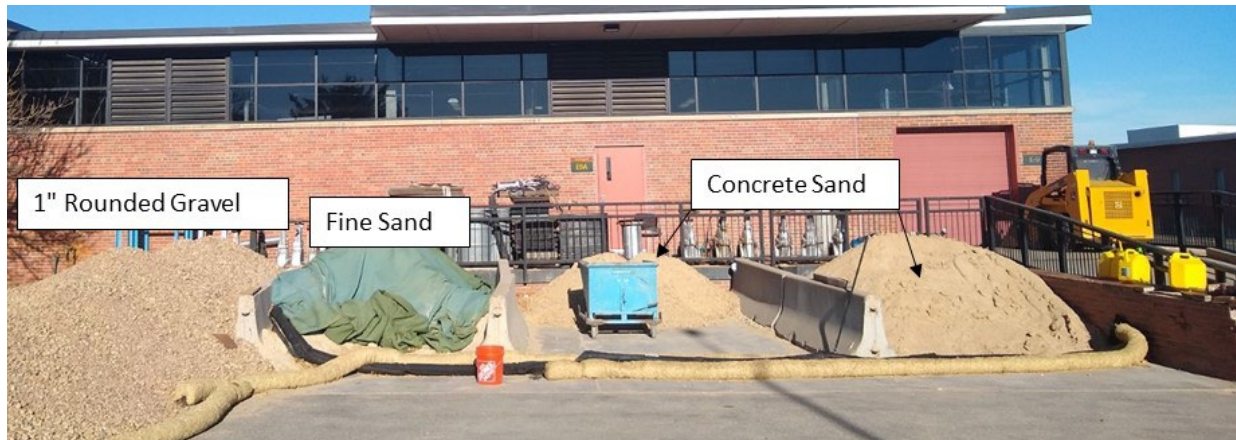
Figure 12. Photograph of materials used for the 1:12 model sediment blend.
