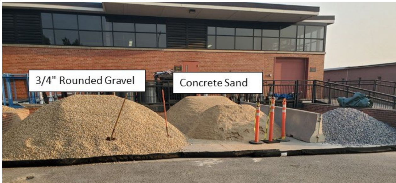
Figure 10. Photograph of materials used for the 1:24 model sediment blend.
