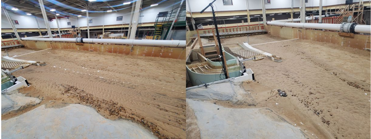
Figure 123. Photographs of sediment bedforms upstream of the hardened ramp without groynes (left) and with groynes (right) at 1,500 ft 3 /s.
