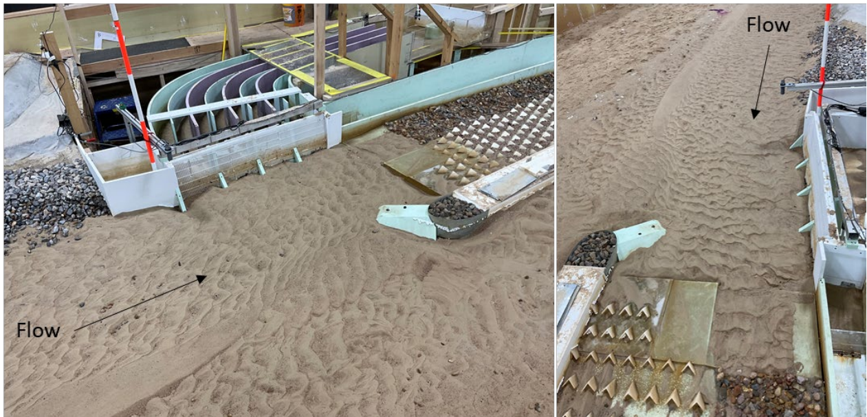
Figure 63. Photographs of the sediment bedforms upstream of hardened ramp without a flushing channel at 3,000 ft 3 /s with added sediment features
