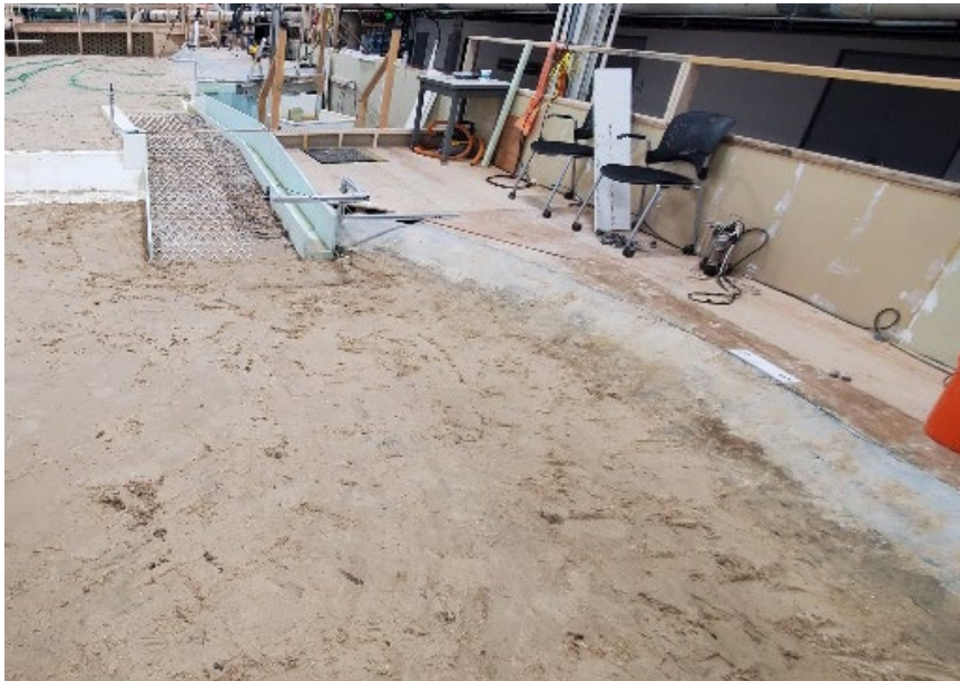
Figure 33. Downstream topography with flushing channel installed for MOD-6 design configuration, looking upstream.
