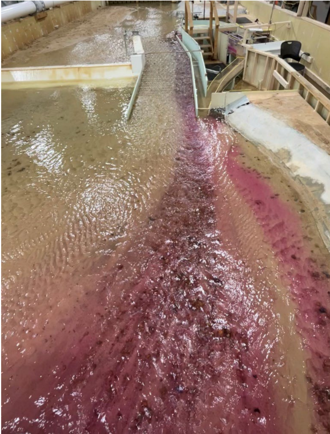
Figure 95. Photograph of flow streamlines on the downstream end of the hardened ramp at 6,000 ft 3 /s following a flushing operation. Looking upstream.
