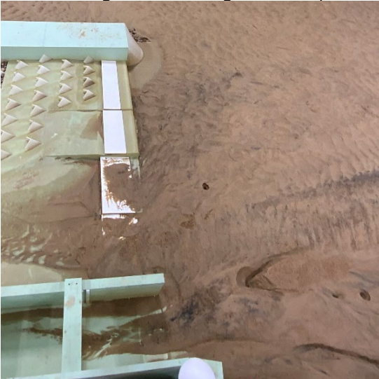
Figure C-6. View of ramp exit looking from left bank for MOD-6 design with flushing channel open after 6,000 ft 3 /s flow rate.
