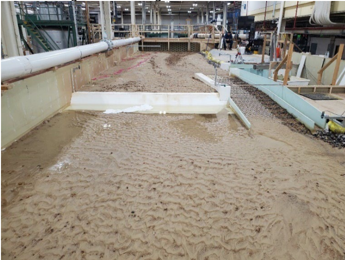
Figure B-40. View looking upstream for MOD-6 design with flushing channel removed after 6,000 ft 3 /s flow rate.
