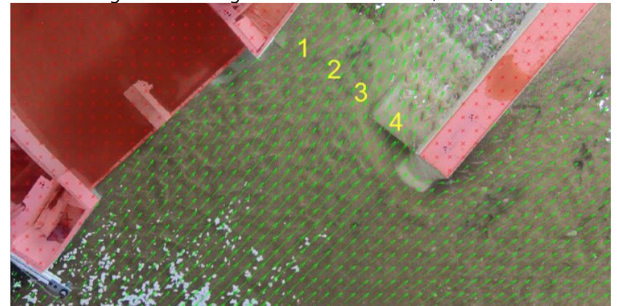
Figure B-84. Surface velocity vector map in area upstream of diversion intake (left) and hardened ramp (right) for MOD-9 design with flushing channel removed at 12,000 ft 3 /s river flow.
