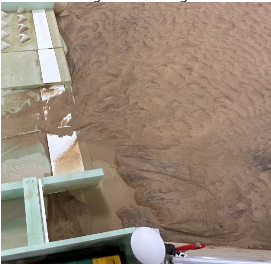
Figure C-18. View of ramp exit looking from left bank for MOD-6 design with flushing channel closed after 3,000 ft 3 /s flow rate.
