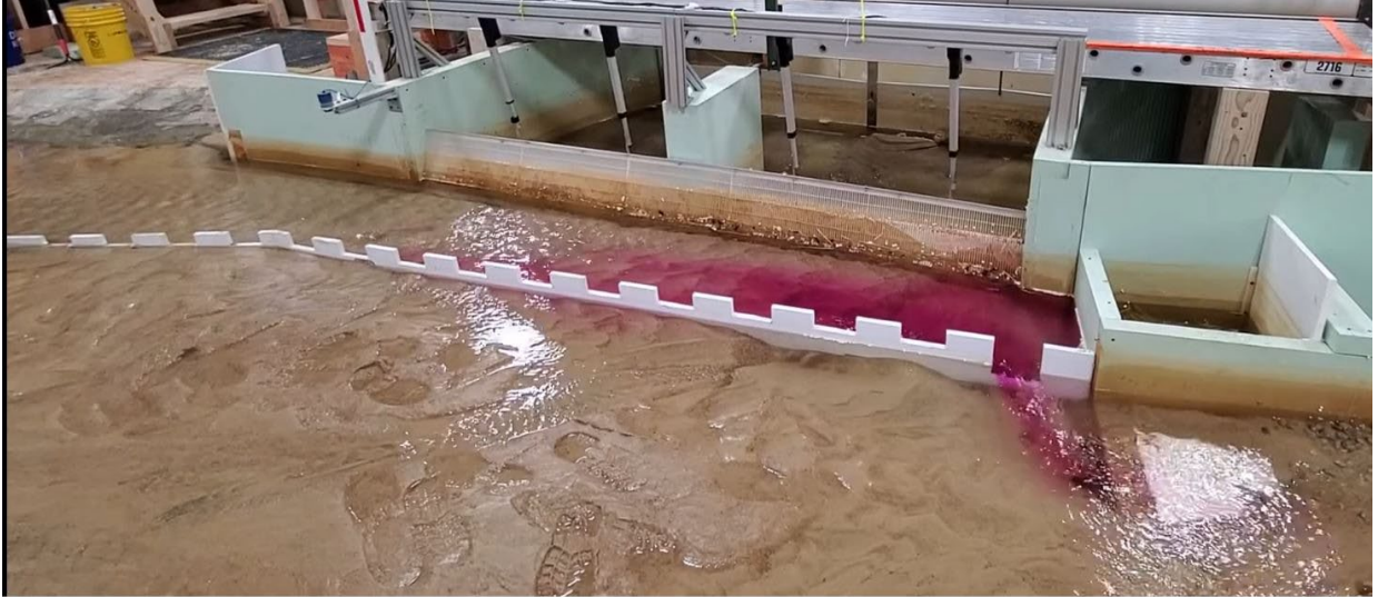
Figure 158. Dye test of the castle training wall structure upstream of intake. River flow was set to 200 ft 3 /s, with approximately 100 ft 3 /s diverted into the intake.
