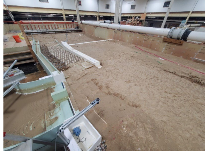
Figure B-11. View looking downstream after dewatering for MOD-9 design with flushing channel removed at 3,000 ft 3 /s.
