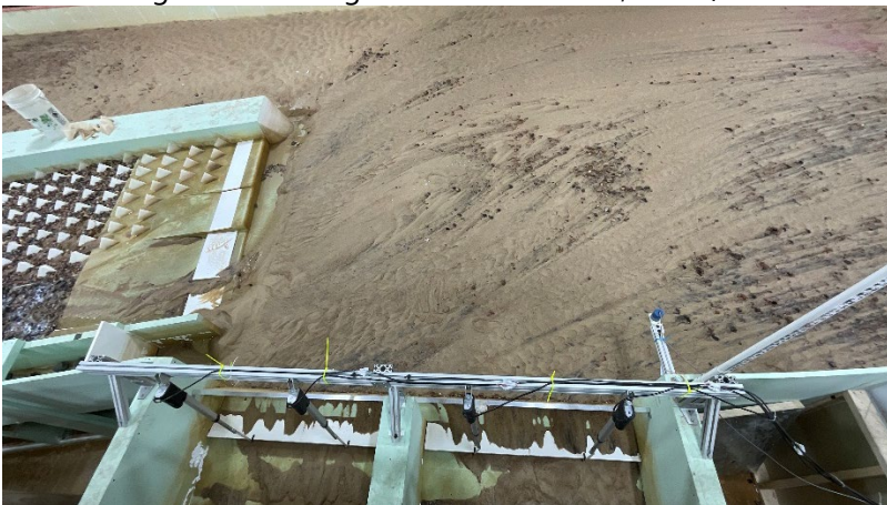
Figure C-45. View looking upstream from diversion canal of area upstream of diversion intake (bottom) and hardened ramp (left) for MOD-6 design with flushing channel closed at 1,500 ft 3 /s river flow.
