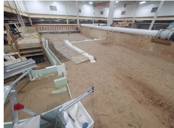
Figure B-71. View looking downstream after dewatering for MOD-9 design with flushing channel removed at 12,000 ft 3 /s.
