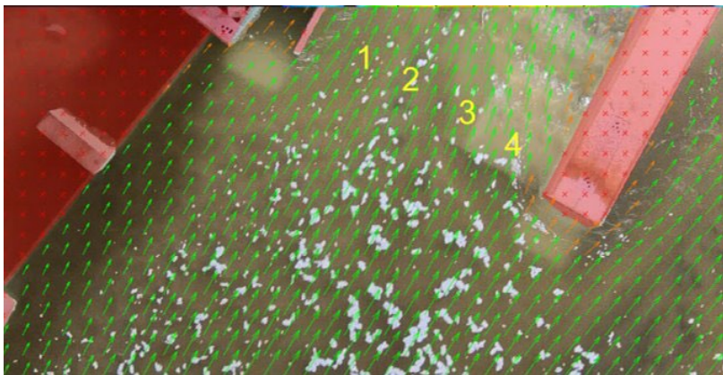
Figure B-74. Surface velocity vector map in area upstream of diversion intake (left) and hardened ramp (right) for MOD-6 design with flushing channel closed at 12,000 ft 3 /s river flow.
