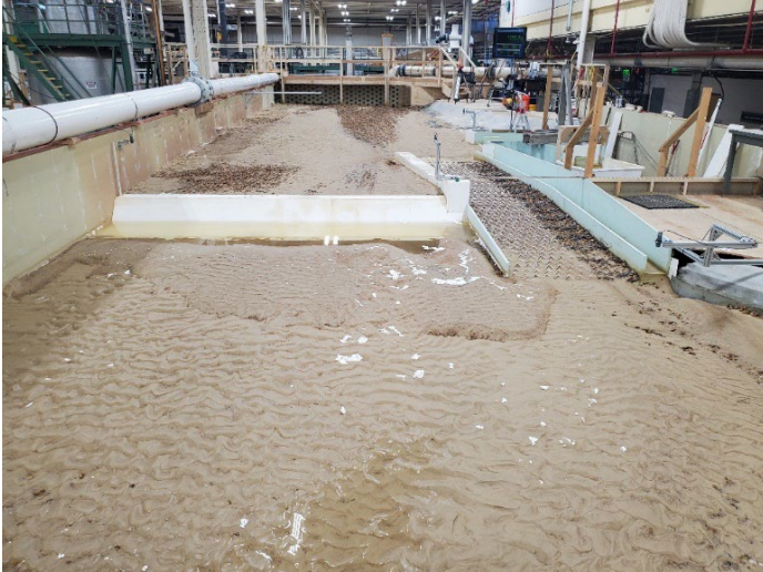
Figure B-62. View looking upstream for MOD-6 design with flushing channel closed after 12,000 ft 3 /s flow rate.
