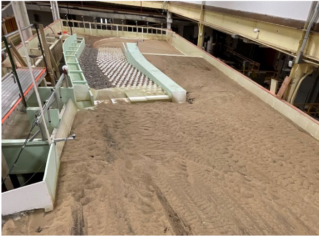
Figure C-21. View looking downstream after dewatering for MOD-6 design with flushing channel open at 3,000 ft 3 /s.
