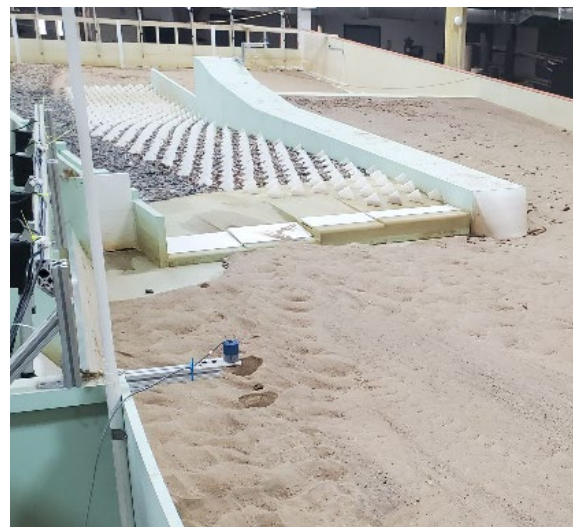
Figure C-3. View looking downstream after dewatering for MOD-9 design with flushing channel closed at 6,000 ft 3 /s.
