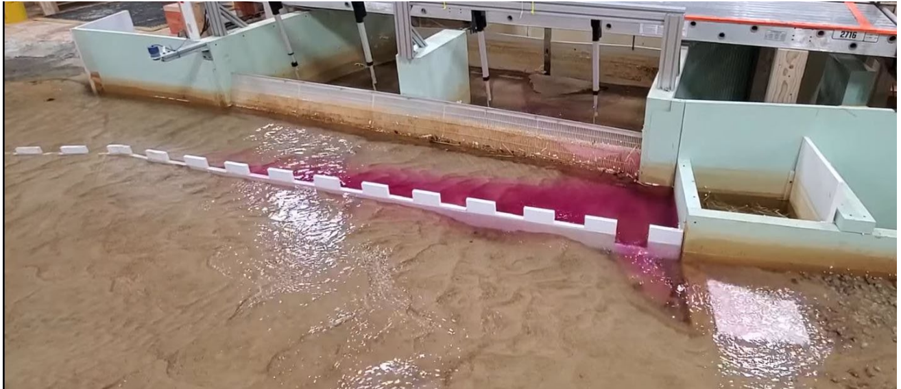
Figure 156. Dye test of the castle training wall structure upstream of intake. River flow was set to 400 ft 3 /s, with approximately 200 ft 3 /s diverted into the intake.
