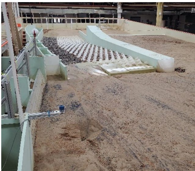
Figure C-1. View looking downstream after dewatering for MOD-6 design with flushing channel closed at 6,000 ft 3 /s.
