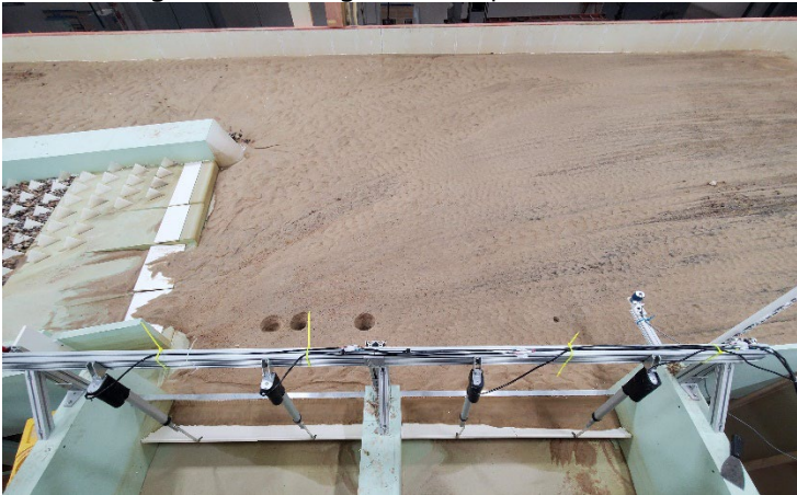
Figure C-49. View looking upstream from diversion canal of area upstream of diversion intake (bottom) and hardened ramp (left) for MOD-6 design with flushing channel open at 1,500 ft 3 /s river flow.
