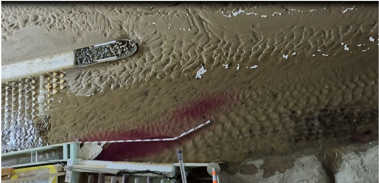
Figure 83. Photograph of dye approaching the hardened ramp with a castle training wall and flushing channel at 1,500 ft 3 /s.
