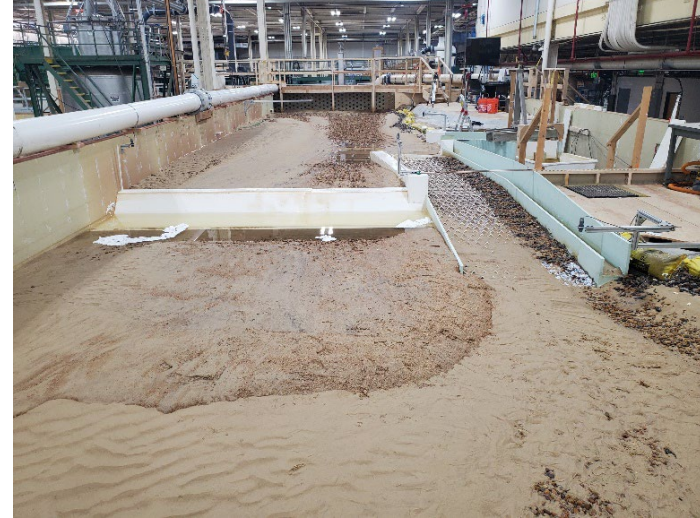
Figure B-102. View looking upstream for MOD-9 design with flushing channel removed after 30,000 ft 3 /s flow rate.
