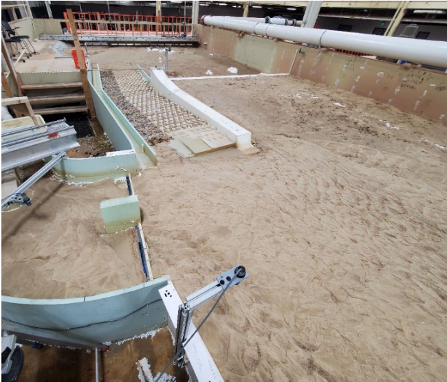
Figure B-5. View looking downstream after dewatering for MOD-6 design with flushing channel open at 3,000 ft 3 /s.
