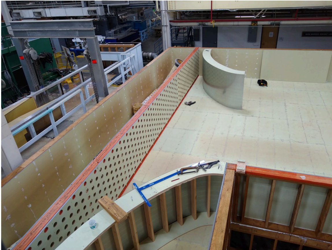
Figure 5. Baffle wall in 1:24 model with 3-inch hole “honey-comb” pattern for flow conditioning and sediment passage as well as curved baffle walls to direct flow into the upstream extents of the model.
