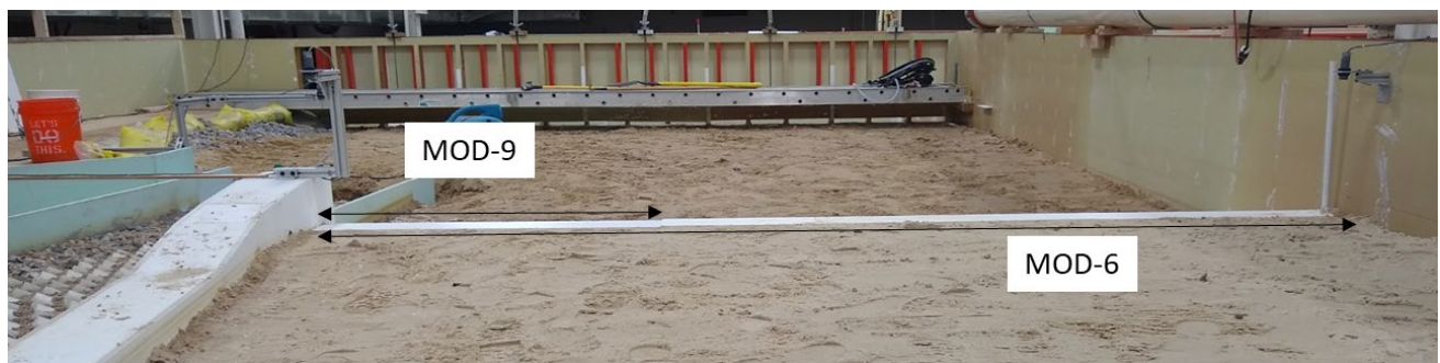
Figure 26. Dam crest configuration comparing MOD-6 (400 ft notch) to MOD-9 (100 ft notch) design configurations in 1:24 model.
