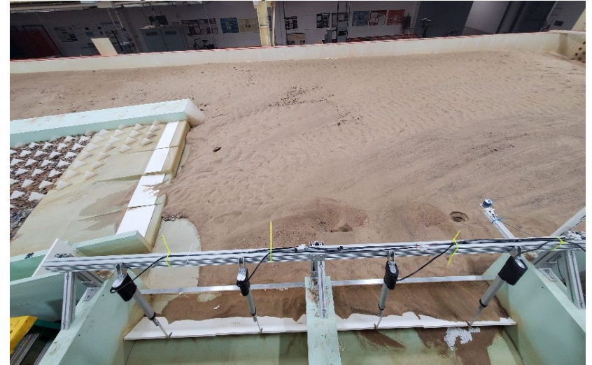
Figure C-28. View looking upstream from diversion canal of area upstream of diversion intake (bottom) and hardened ramp (left) for MOD-9 design with flushing channel closed at 3,000 ft 3 /s river flow.
