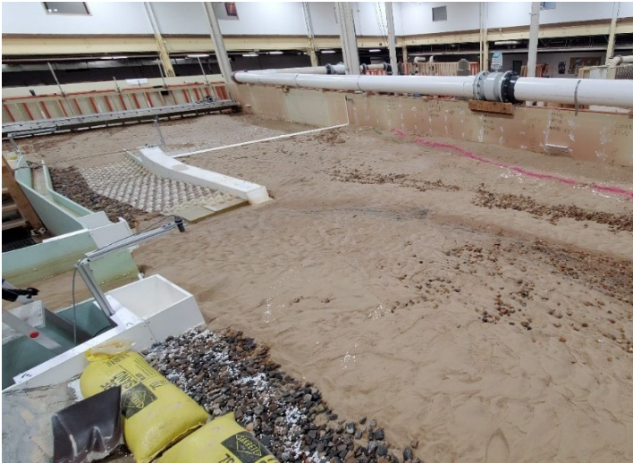
Figure B-39. View looking downstream after dewatering for MOD-6 design with flushing channel removed at 6,000 ft 3 /s.
