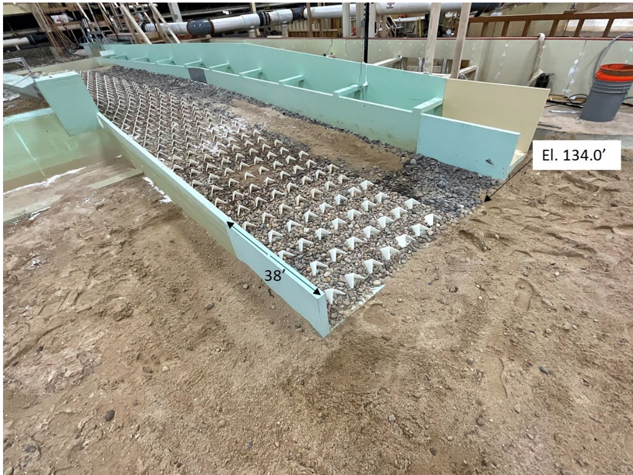
Figure 28. Photograph showing the 38-ft downstream extension of the hardened ramp in the 1:12 scale model for the MOD-9 design configuration.
