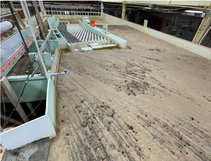
C-37. View looking downstream after dewatering for MOD-6 design with flushing channel closed at 1,500 ft 3 /s.
