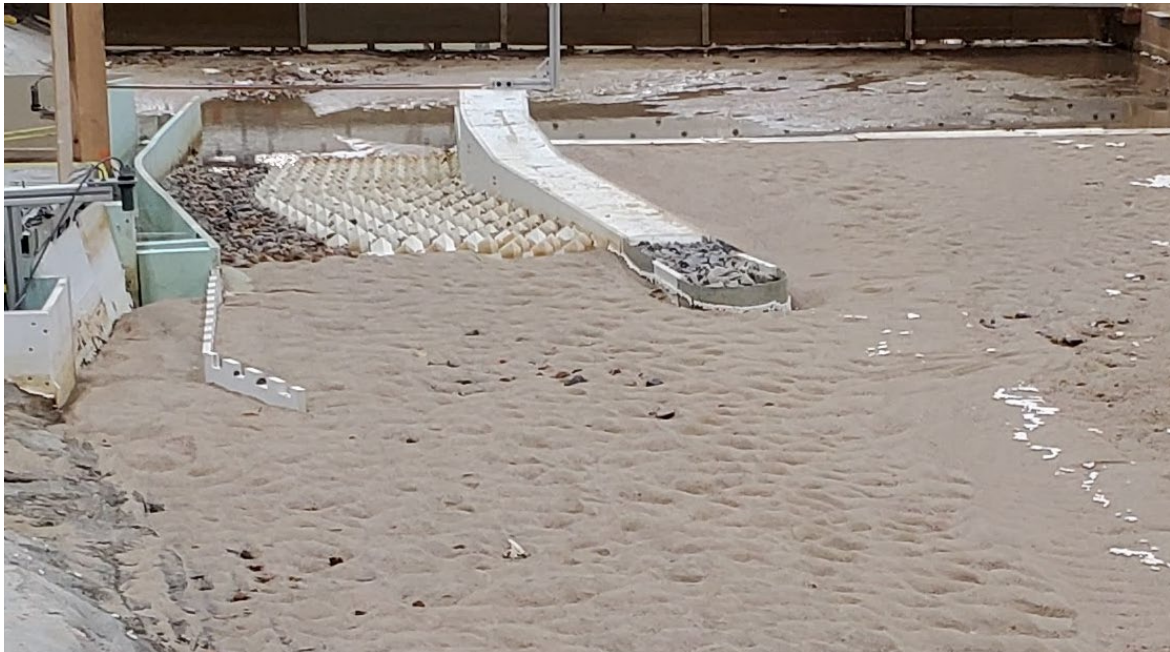
Figure 90. Photograph of bedform upstream of the hardened ramp and canal intake after 3,000 ft 3 /s river flow and 825 ft 3 /s diversion before flushing operations.
