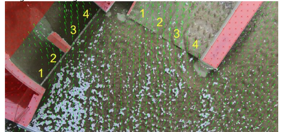
Figure B-46. Surface velocity vector map in area upstream of diversion intake (left) and hardened ramp (right) for MOD-9 design with flushing channel closed at 6,000 ft 3 /s river flow.
