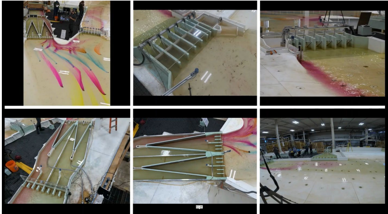
Figure 33. Mosaic image of dye testing on the 1:24 scale physical model for Scenario 1:24 – 18.
