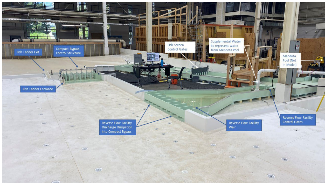
Figure 15. Reverse flow facility viewed from the downstream right bank of the Compact Bypass channel.
