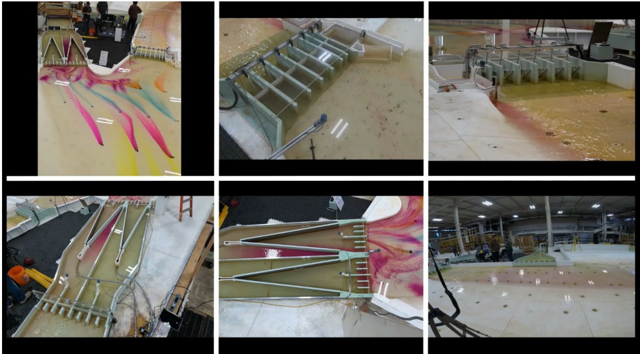
Figure 32. Mosaic image of dye testing on the 1:24 scale physical model for Scenario 1:24 – 11.
