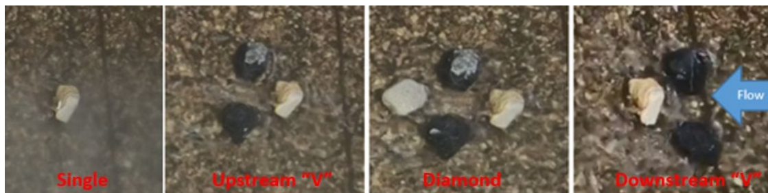
Figure 6. Single, upstream "V", diamond, and downstream "V" configurations, respectively for the large boulder tests. For the small boulder tests only the single, upstream "V", and downstream "V" configurations were tested.
