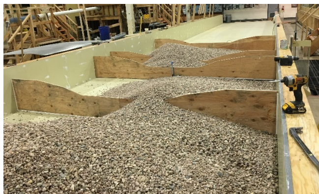
Figure 1. Template system used in model construction.
