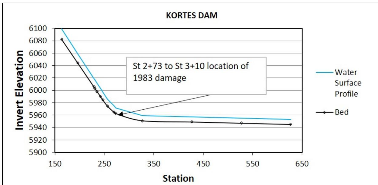
Figure 28 Water surface profile plot from Spillway Pro and location of cavitation damage observed at Kortés Dam.
