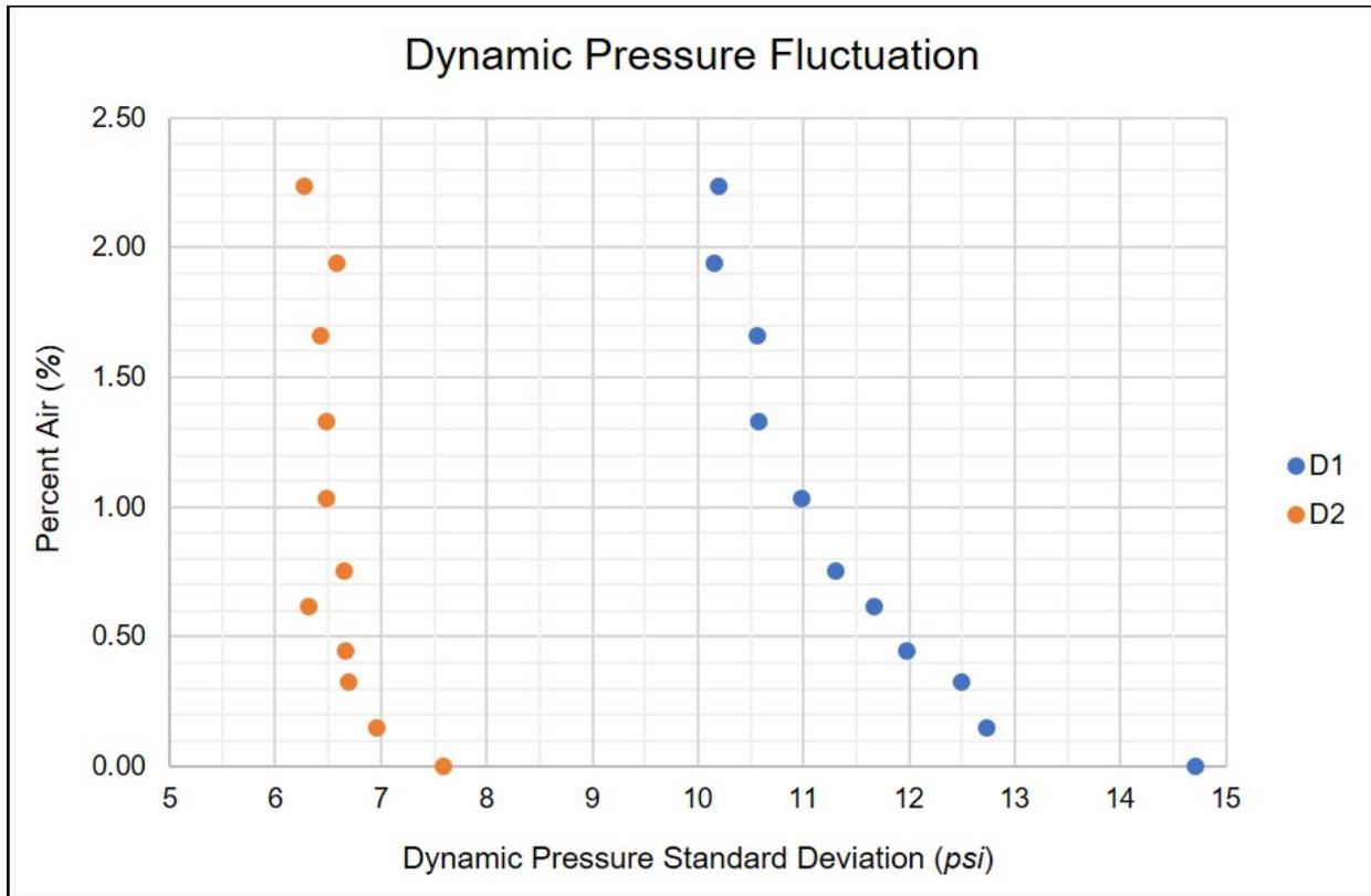
Figure 16 Plot showing effect of air percentage on hydrodynamic pressure fluctuations (standard deviation) on the test surface.
