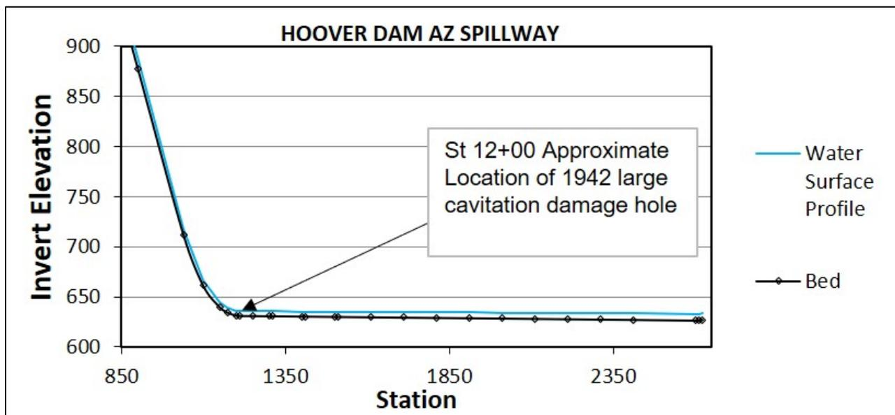
Figure 27 Water surface profile plot from Spillway Pro and location of cavitation damage observed at Hoover Dam.
