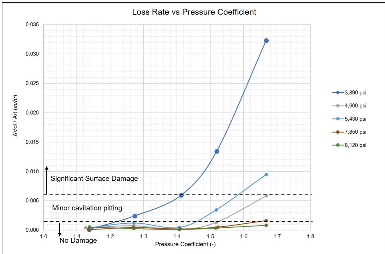
Figure 23 Plot showing preliminary method from current laboratory data to compare the degree of cavitation damage with localized hydraulic conditions at the surface and concrete strength.
