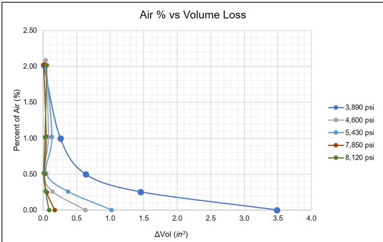
Figure 18 Plot showing effect of air percentage in the flow of water on cavitation damage during a 4 hour test period to concrete test blocks (volume loss) for the range of concrete strengths.
