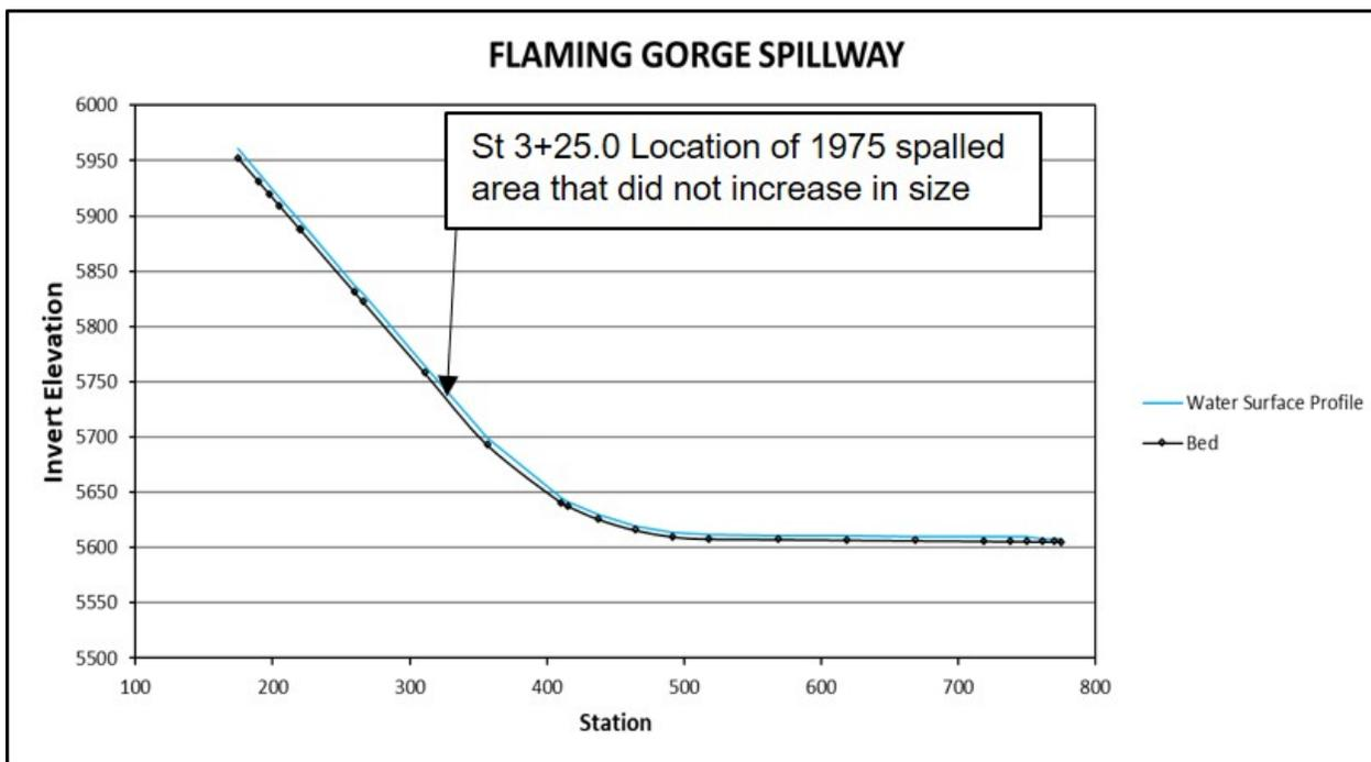
Figure 25 Water surface profile plot from Spillway Pro and location of cavitation damage observed at Flaming Gorge Dam.
