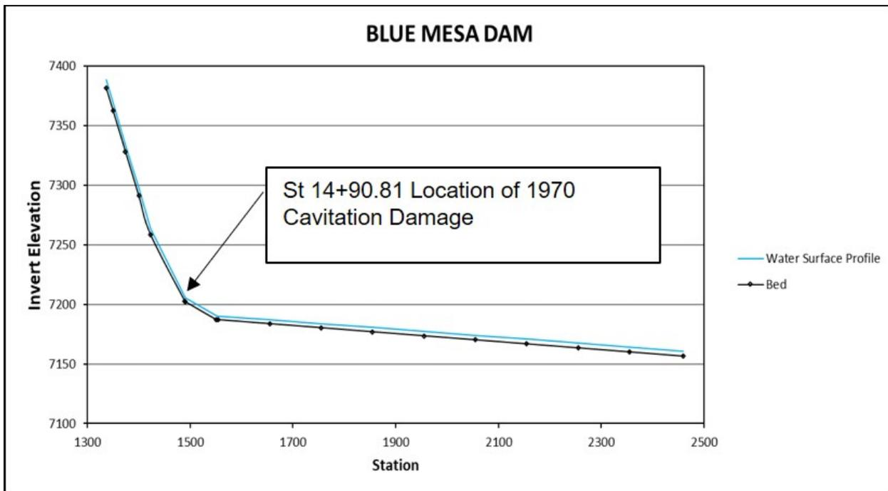
Figure 24 Water surface profile plot from Spillway Pro and location of cavitation damage observed at Blue Mesa Dam.
