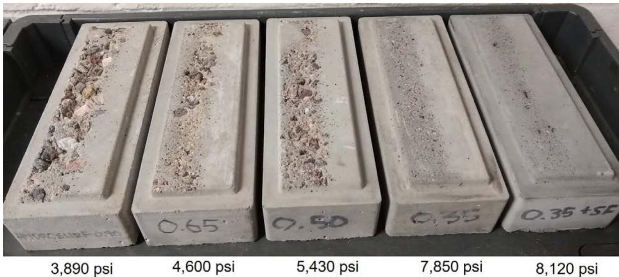
Figure 21 Photographs showing extent of cavitation damage with concrete strength to concrete test blocks with no air injection.
