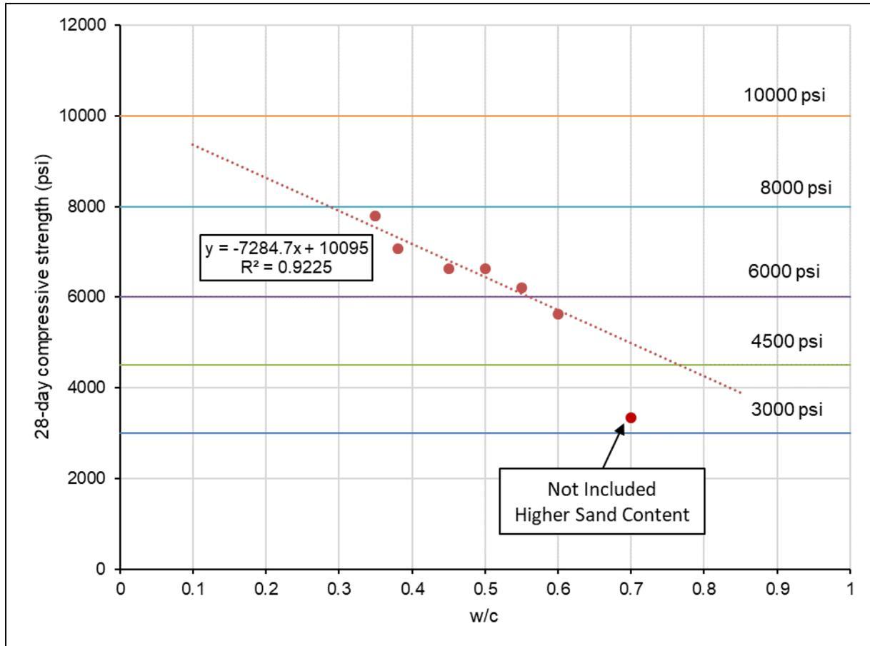
Figure 7. Trial batch strength results to determine proportions for final specimens.
