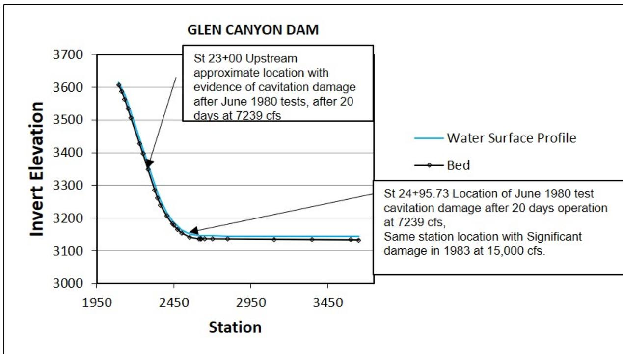
Figure 26 Water surface profile plot from Spillway Pro and location of cavitation damage observed at Glen Canyon Dam.
