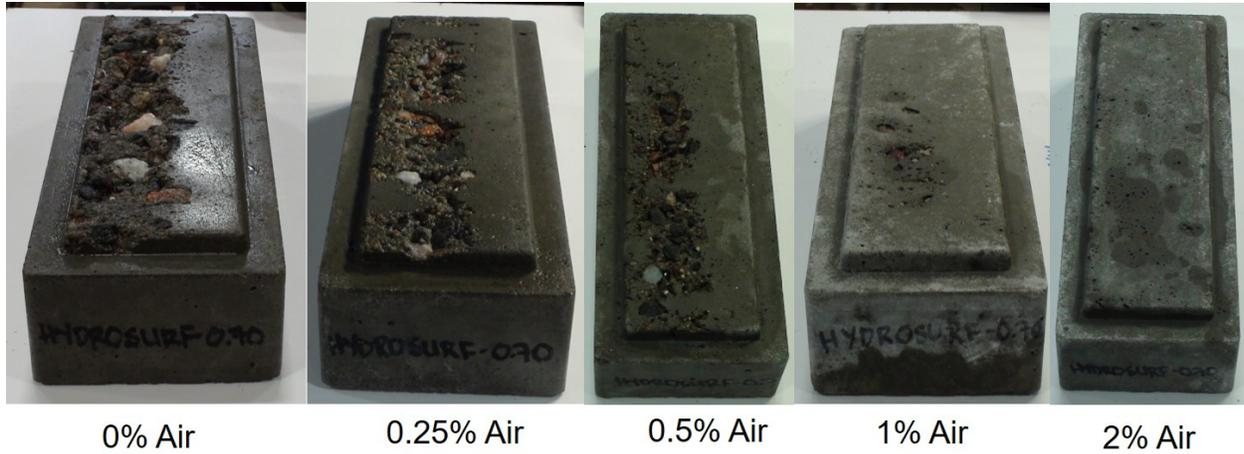
Figure 20 Photographs showing extent of cavitation damage with air percentage (in flow of water) to concrete test blocks with the lowest strength (average of 3,890 psi).
