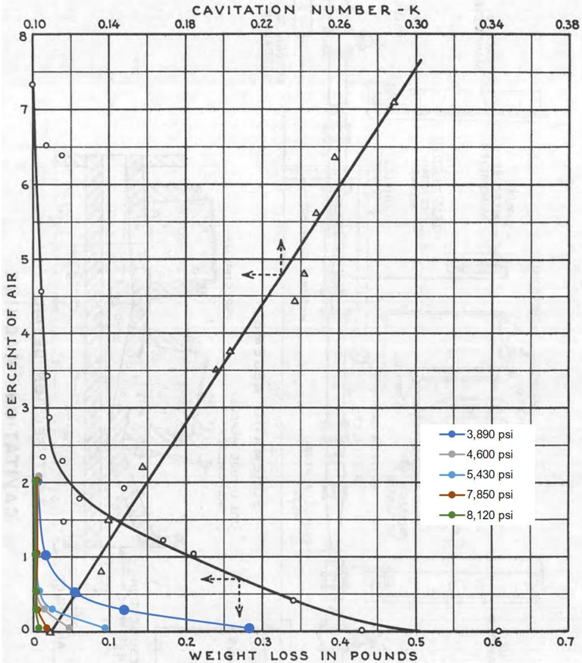
Figure 19 Plot comparing concrete damage results of current study to that of Peterka in 1953. Percent of air pertains to air in flow of water. The present tests used a 4-hour exposure time. Peterka's tests used a 2-hour exposure time and concrete samples of unmeasured strength (and no coarse aggregate) cured for only 7 days.
