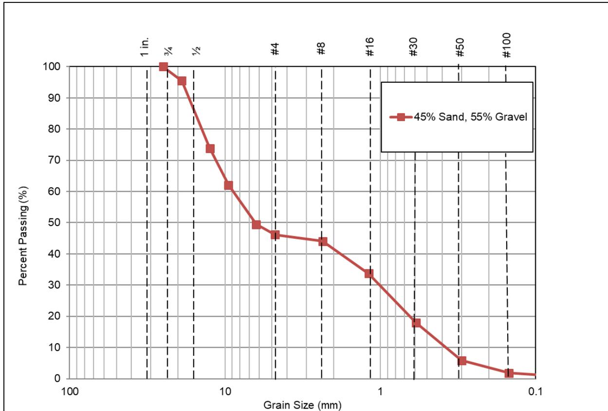
Figure 5. Combined fine and coarse aggregate gradation
