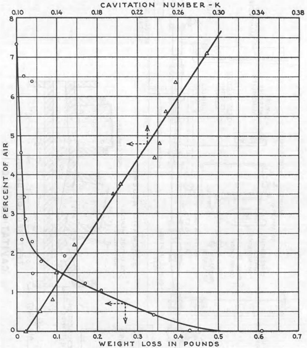
Figure 2 Test data from Peterka's 1953 laboratory study showing significant decrease in concrete damage from cavitation with percentage of air in the flow of water.
