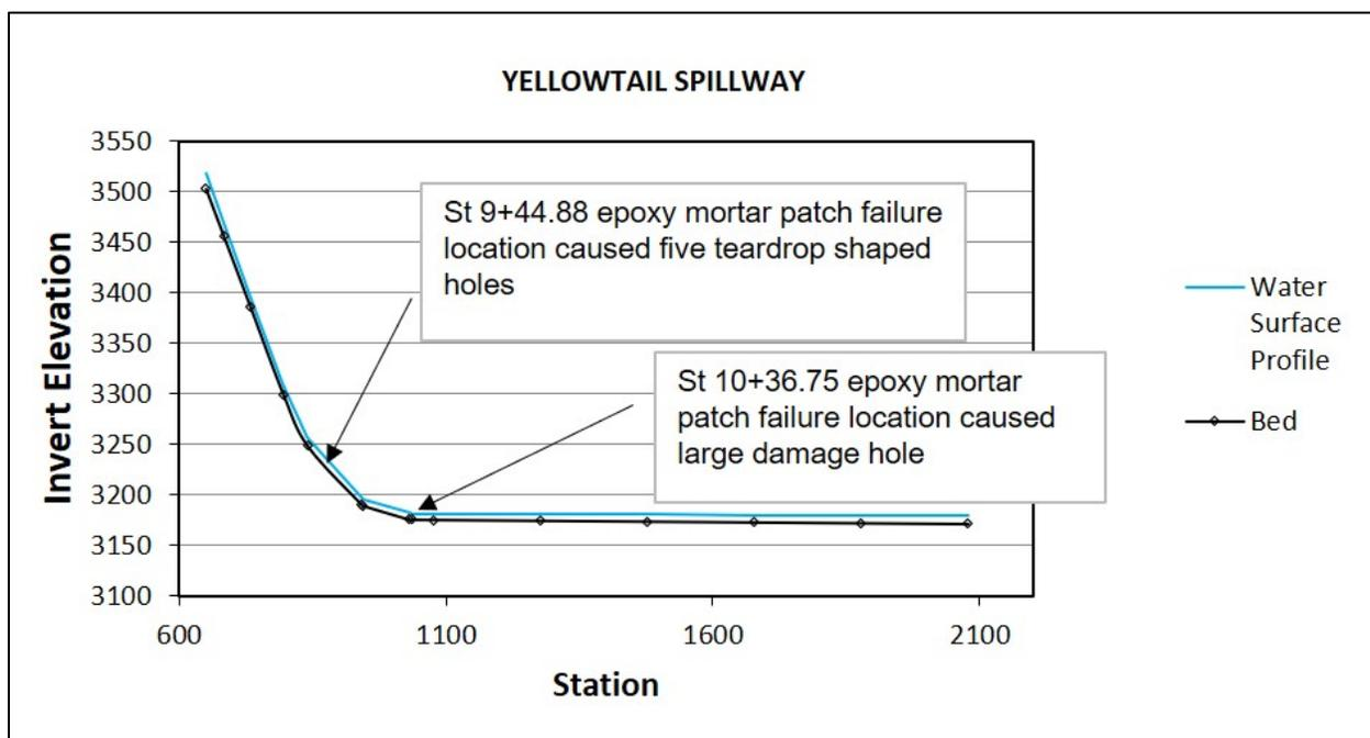
Figure 29 Water surface profile plot from Spillway Pro and location of cavitation damage observed at Yellowtail Dam.
