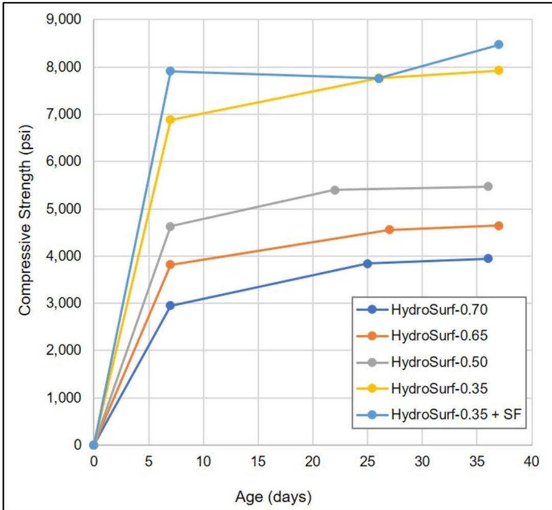
Figure 13 Compression strength results over time for concrete samples used for cavitation damage testing.
