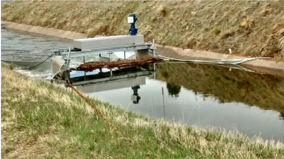
Figure 19 Debris clogged in the HK rotors. Tarp transitions were cut to relieve upstream water levels. Looking downstream.
