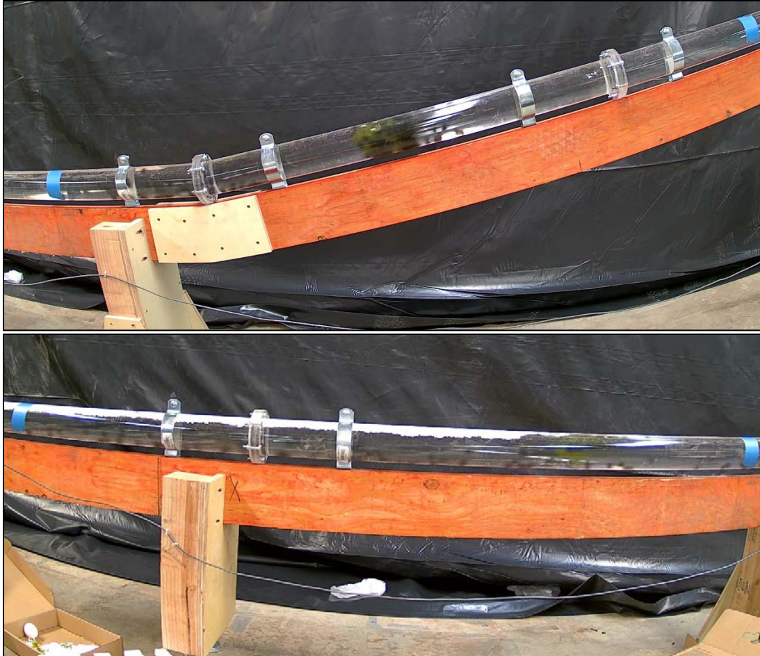
Figure 12. (Top) The black neutrally buoyant particles moving rapidly through the pipe at the bend. (Bottom) The neutrally buoyant particles moving under the stable Extreme Debris Load slug floating at the crown of the pipe (discharge is from right to left in both images).
