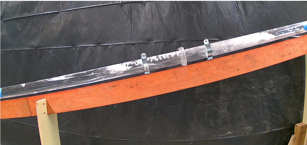
Figure 9. A hydraulic jump forming during the beginning of the pre-flushing phase
