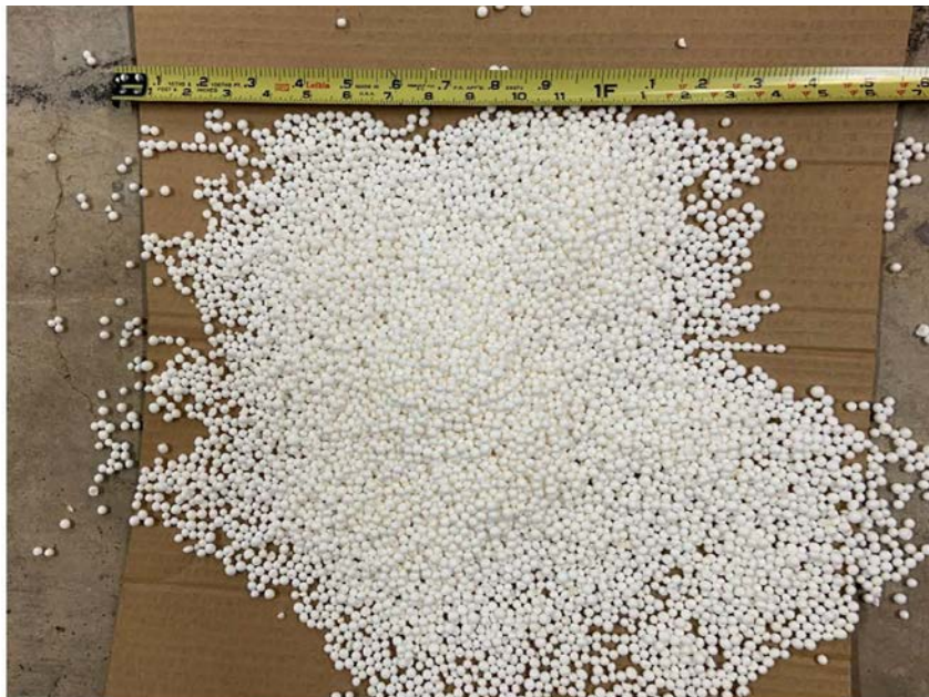
Figure 8. Extreme worst-case debris load, the smaller debris particles took longer to clear from the release pipe during shakedown testing of the model and were selected for a worst-case debris load.
