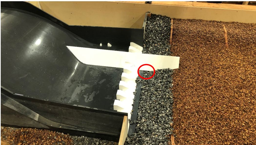
Figure 29. Photograph of gravity wall post-test viewed from river right, red circle indicates location of scour that should be mitigated with a shallow cutoff wall.
