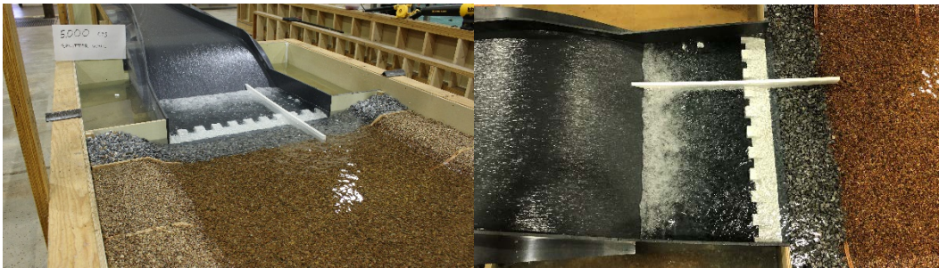
Figure 15. Photograph of splitter wall configuration for 5,000 ft 3 /sec, the left image is looking from the downstream river right, and the right image is looking at a plan view with flow from left to right.
