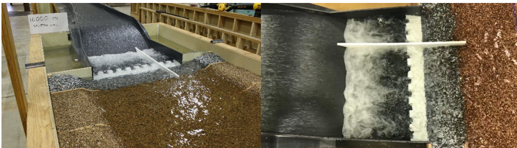
Figure 16. Photograph of splitter wall configuration for 10,000 ft 3 /sec, the left image is looking from the downstream river right, and the right image is looking at a plan view with flow from left to right.
