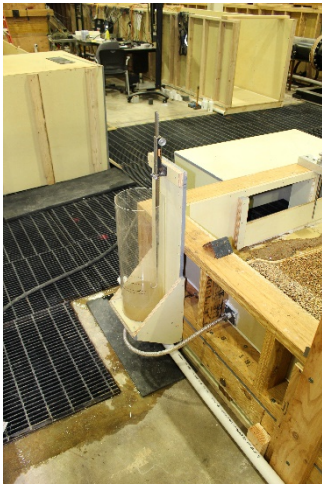
Figure 5. Photograph of stilling well attached to piezometer tap in the center of the downstream river channel.
