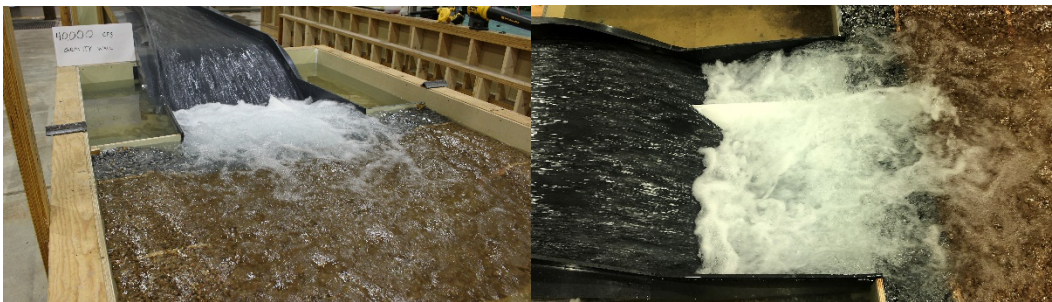
Figure 27. Photograph of gravity wall configuration for 40,000 ft 3 /sec, the left image is looking from the downstream river right, and the right image is looking at a plan view with flow from left to right.
