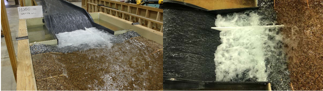
Figure 17. Photograph of splitter wall configuration for 25,000 ft 3 /sec, the left image is looking from the downstream river right, and the right image is looking at a plan view with flow from left to right.
