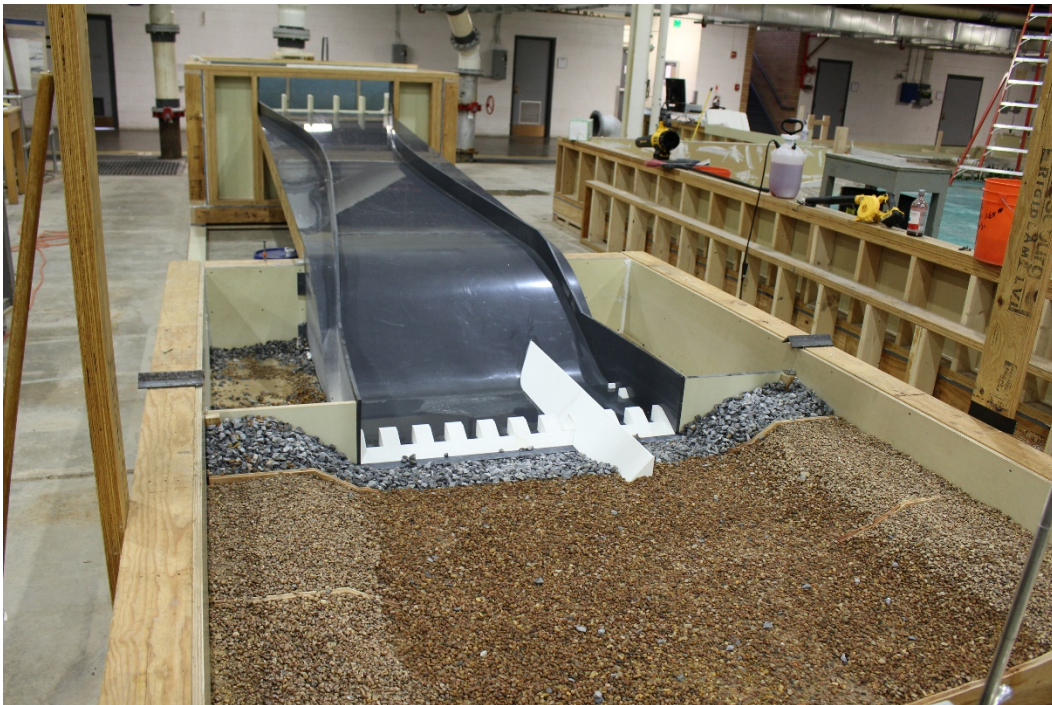
Figure 4. Photograph of spillway, energy dissipation basin with baffle blocks and gravity wall installed and downstream river channel.
