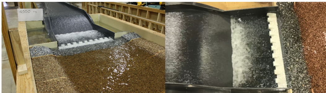
Figure 7. Photographs of as built configuration for 5,000 ft 3 /sec the left image is looking from the downstream river right, and the right image is looking at a plan view with flow from left to right.
