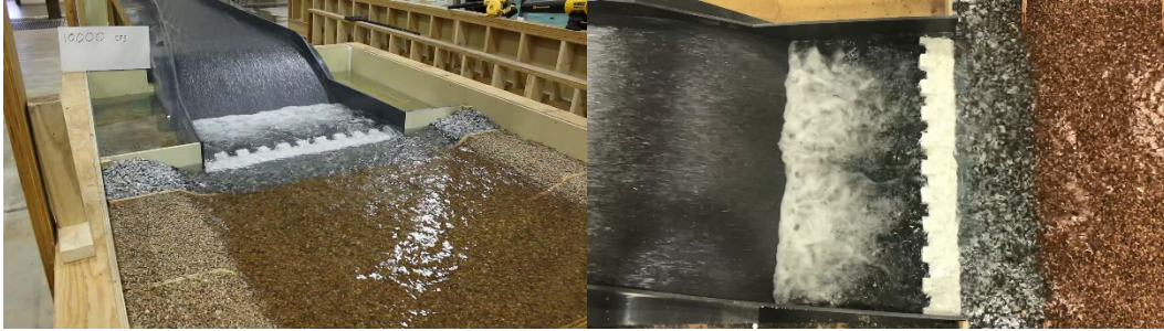
Figure 8. Photograph of as built configuration for 10,000 ft 3 /sec, the left image is looking from the downstream river right, and the right image is looking at a plan view with flow from left to right.
