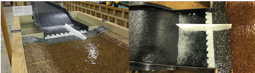
Figure 24. Photograph of gravity wall configuration for 5,000 ft³/sec, the left image is looking from the downstream river right, and the right image is looking at a plan view with flow from left to right.
