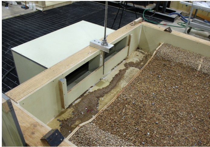
Figure 6. Photograph of downstream overflow weir used to set the tailwater depth of the model.
