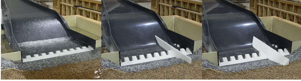
Figure 1. The three energy dissipation basin configurations tested in the physical model, as built (left), splitter wall (center), gravity wall (right).
