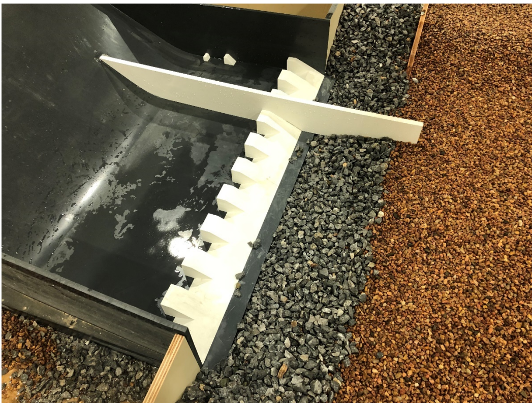
Figure 21. Photograph of splitter wall post-test downstream bed showing that a few rocks moved upstream onto the apron that extends beyond the energy dissipation blocks in the basin.
