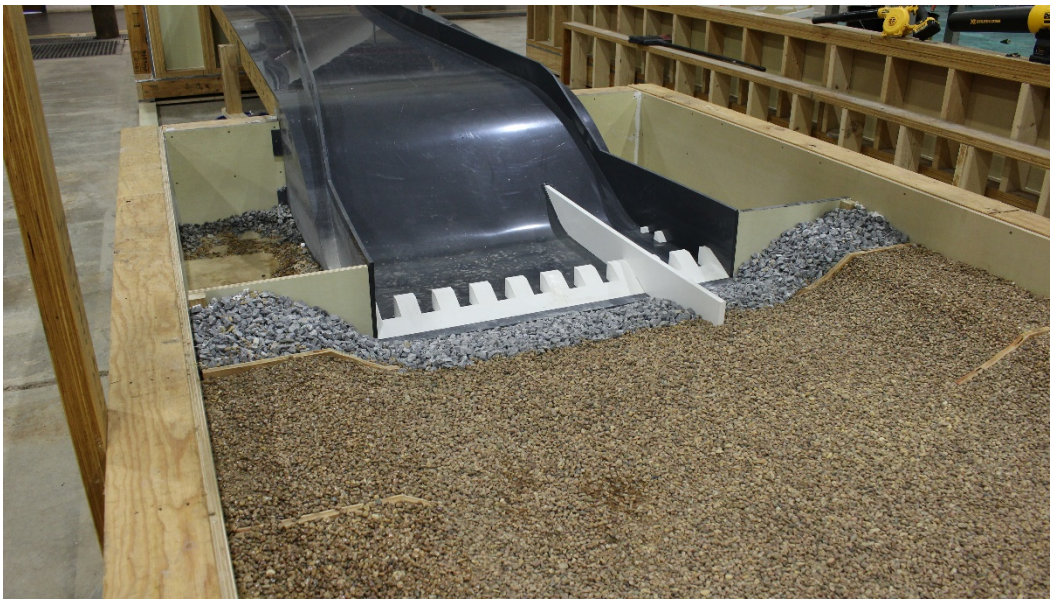
Figure 13. Photograph of splitter wall pre-test image looking from the downstream river right.
