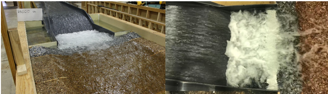
Figure 9. Photograph of as built configuration for 25,000 ft 3 /sec, the left image is looking from the downstream river right, and the right image is looking at a plan view with flow from left to right.
