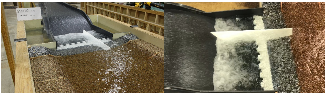
Figure 25. Photograph of gravity wall configuration for 10,000 ft³/sec, the left image is looking from the downstream river right, and the right image is looking at a plan view with flow from left to right.
