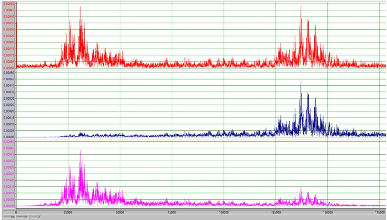
Figure 10 Example frequency spectrum of the raw broadband AE signal (red), HF signal (blue), and LF signal (pink).
