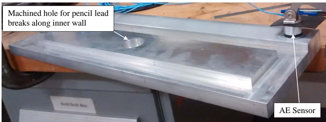
Figure 1 Aluminum plate used for bench testing of pencil lead breaks to produce acoustic waves on the surface and deeper into the material.
