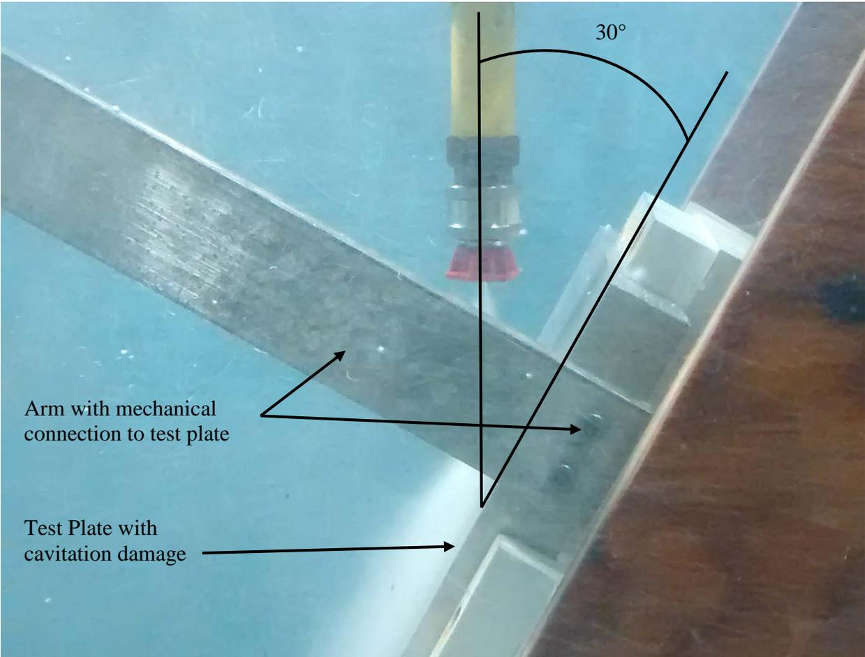
Figure 7 Test setup for inducing cavitation damage on an aluminum plate with a submerged jet.
