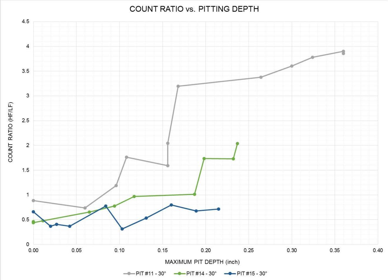
Figure 14 HF/LF ratio of counts over a determined threshold vs. max pitting depth for test runs where the test setup was not disturbed between tests.
