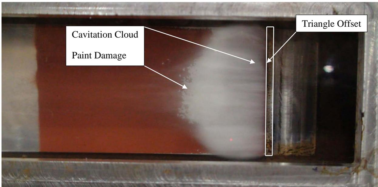
Figure 6 Top view of triangle offset and downstream test plate with visible paint removal after 30 hours of operation. However, depth of cavitation pitting was not significant. Flow is from right to left.
