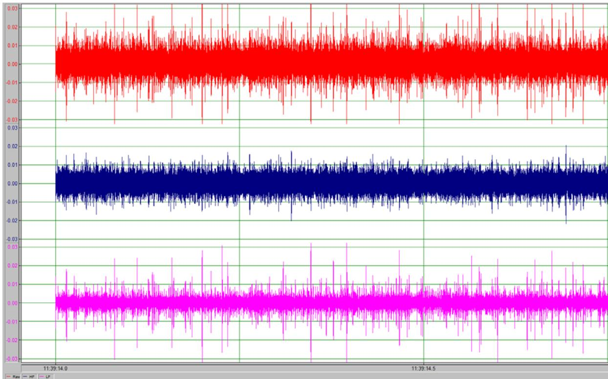
Figure 9 Example time series of the raw broadband AE signal (red), HF signal (blue), and LF signal (pink).
