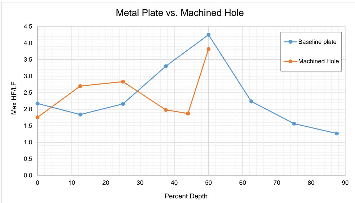
Figure 12 Comparison of pencil lead break results from the baseline plate to one with a machined hole.
