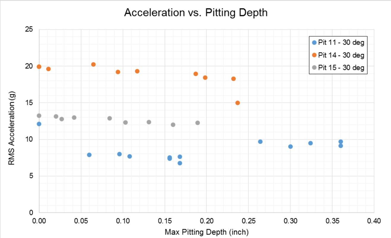
Figure 17 RMS vibration data vs. maximum pit depth for test runs where the test setup was not disturbed between tests.
