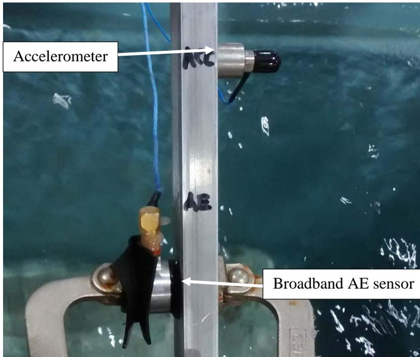
Figure 8 AE and accelerometer sensors mounted out of the water on a metal arm that is mechanically connected to the test plate.
