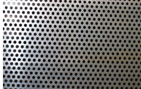
Figure 35. Perforated plate with 3/32-inch holes at 5/32-inch spacing (33% porosity).
