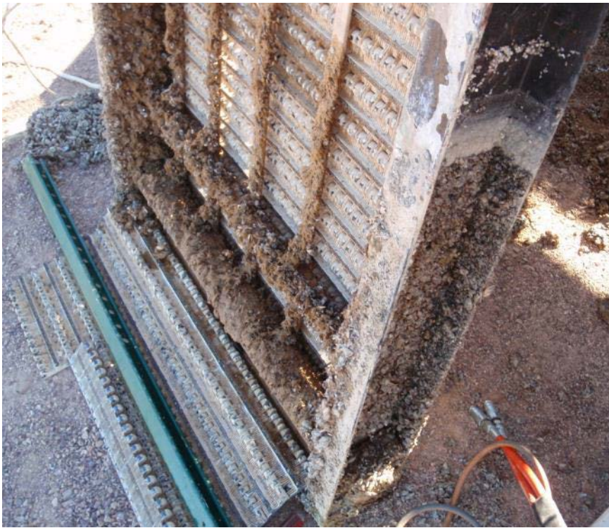
Figure 36 Mussel settlement on Hydrolox frame and interior supports following testing (inside of Hydrolox screen).
