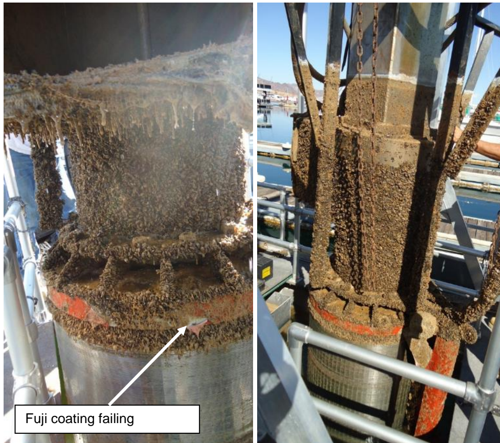
Figure 39 Mussel settlement on ISI frame and screen edges. Mussels did not attach on areas coated with the Fuji Silicone coating. Mussels did attach to areas where the Fuji coating had peeled off.
