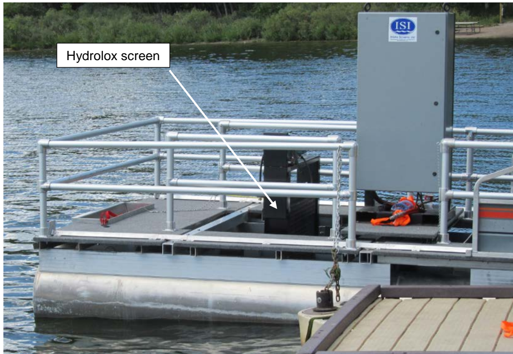
Figure 11 Hydrolox screen mounted in the downstream test channel near the rear of the pontoon boat (flow is right to left through test channel which is not visible in the photo).
