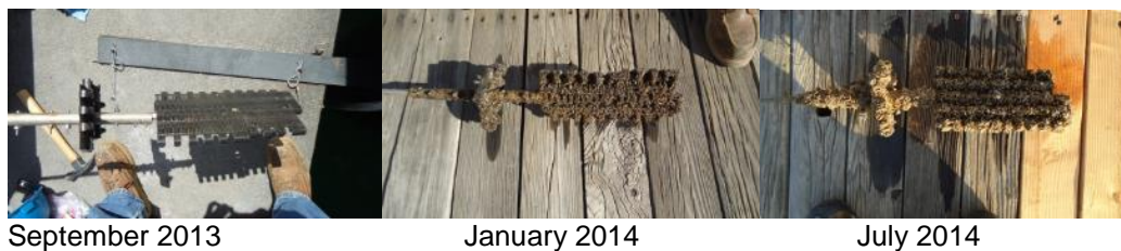
Figure 19 Hydrolox sample sections that were mounted below the water surface and rotated at approximately the same speed as the main Hydrolox screen. Despite continuous motion, mussels attached to the samples.
