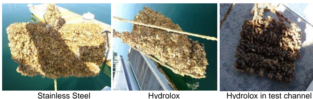
Figure 15 Heavy mussel attachment on static screen samples that were submerged about 12 ft below the surface and a control Hydrolox sample submerged about 2 ½ ft below the surface in the test channel (Summer 2013).
