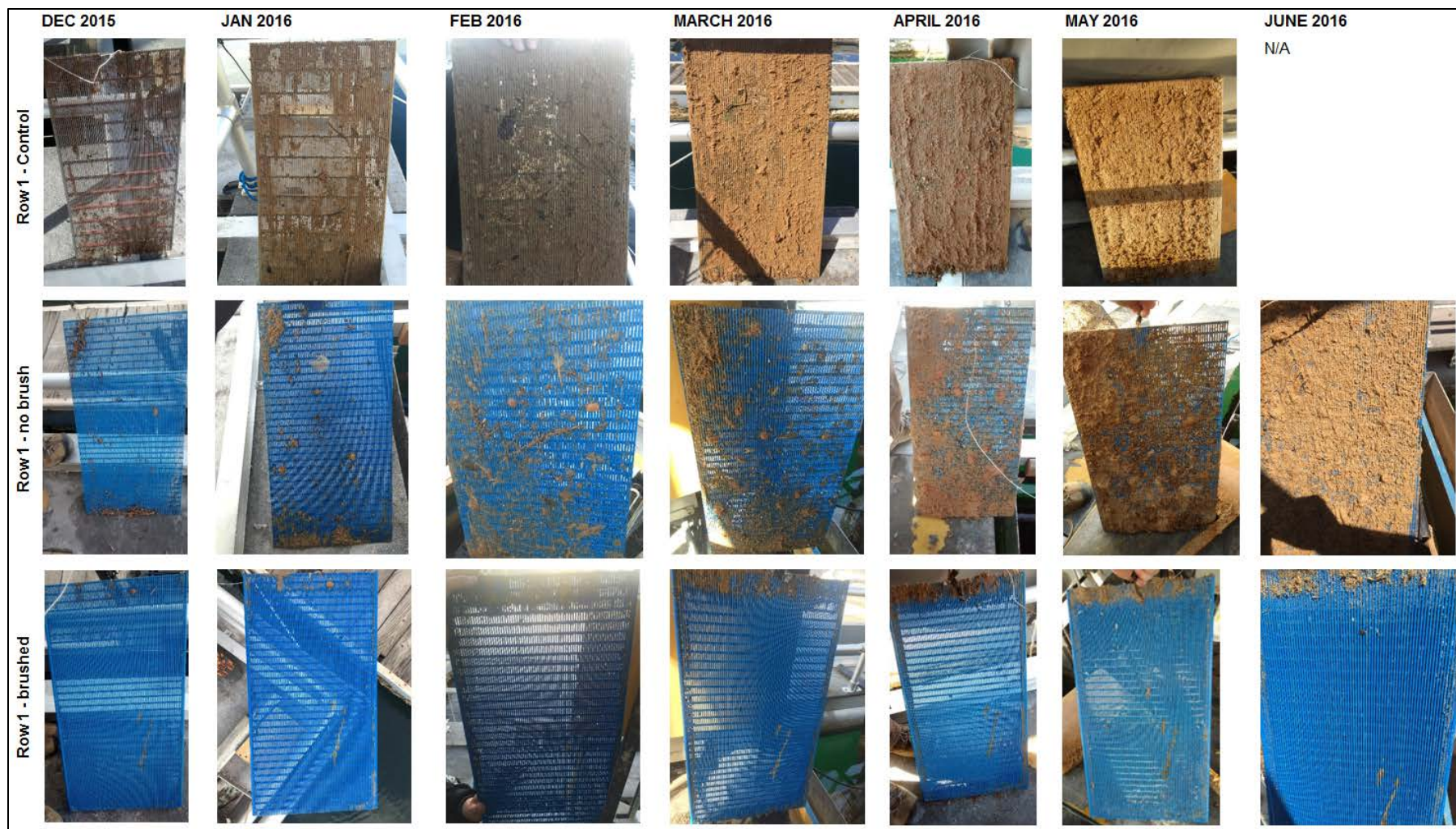
Figure 27 Time lapse photo comparison from Dec. 2015 through June 2016 of the first row of flat plate test screens (vertical wedgewire).
