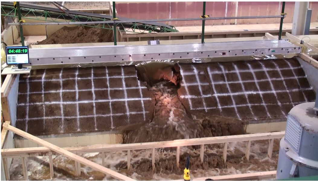
Figure 8. — Breach moving into canal during a laboratory test (Wahl and Lentz 2011).
