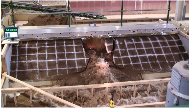
Figure 2. — Headcut erosion is advancing through the embankment crest, enlarging the breach at the point of hydraulic control.
