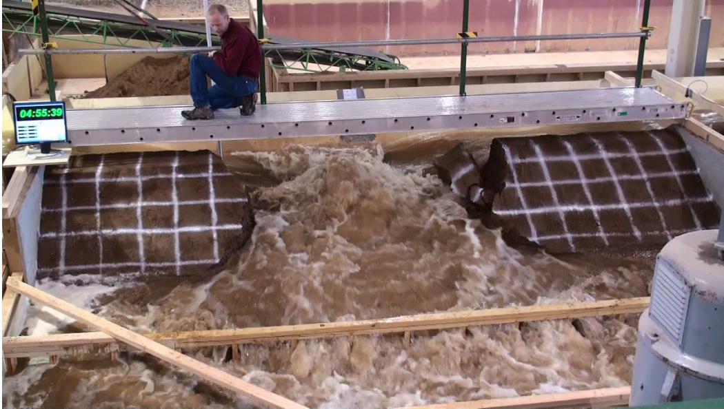
Figure 3. — Canal embankment breach test during late stages of breach widening. Initial flow in the canal behind the embankment was from right to left. Flow in both canal legs leading to the breach opening is passing through critical depth, as indicated by the hydraulic jump where the flows converge. Flow out of the breach is limited by the canal capacity at this point.
