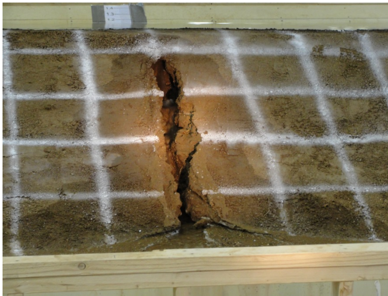
Figure 1. — Laboratory test of a canal breach due to internal erosion. Flow through a hole located just below the embankment crest has led to formation of a narrow headcut gully in the downstream slope that is advancing upstream, through the embankment.
