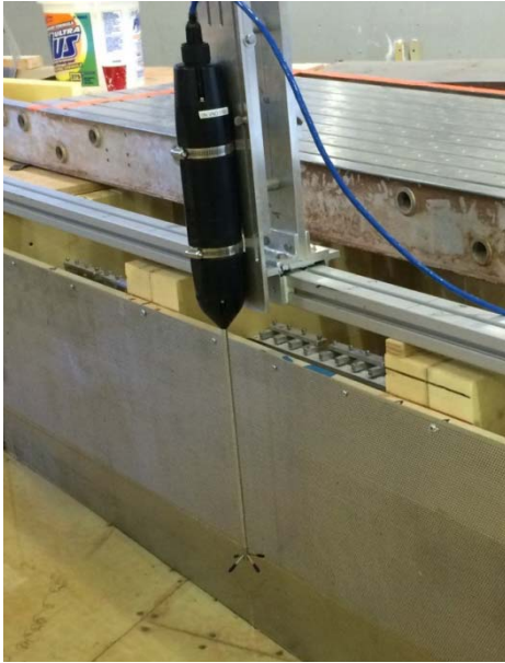
Figure 11. Nortek Vectrino+ 3D velocimeter mounted in the model at 0.75 depth.
