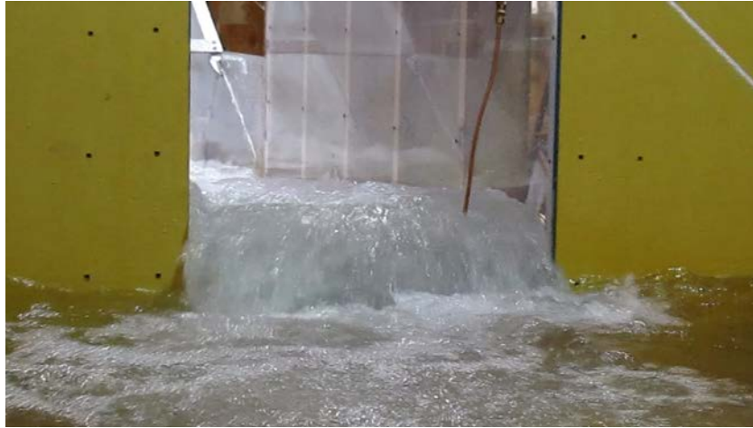
Figure A-12. — Flow over the top of a single deflector at design flow ( 956 \text{ ft}^3/\text{s} ), with deflector bottom lip located 6.2 ft above basin floor.
