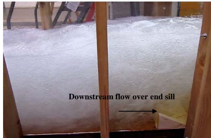
Figure A-4. — At design flow ( 956 \text{ ft}^3/\text{s} ) the jet typically stays low and near the bottom, preventing upstream currents from carrying materials into the stilling basin.
