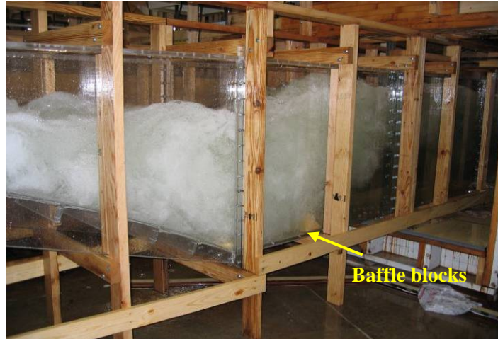
Figure 30. — Baffle blocks help lift jet above basin floor.
