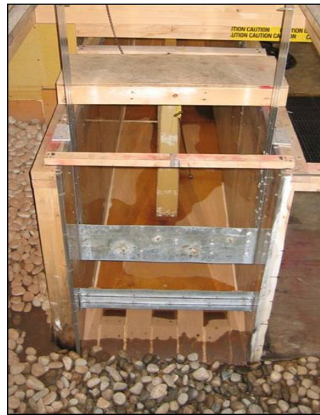
Figure 26. — Mason Dam stilling basin staggered deflector configuration
