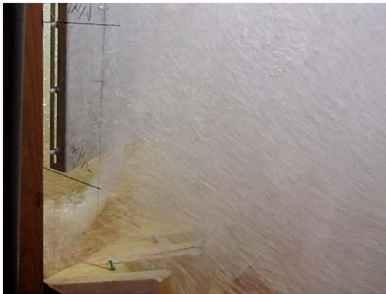
Figure A-11. — Single deflector at design flow (956 ft 3 /s) with deflector bottom edge located 5.1 ft above basin floor.
