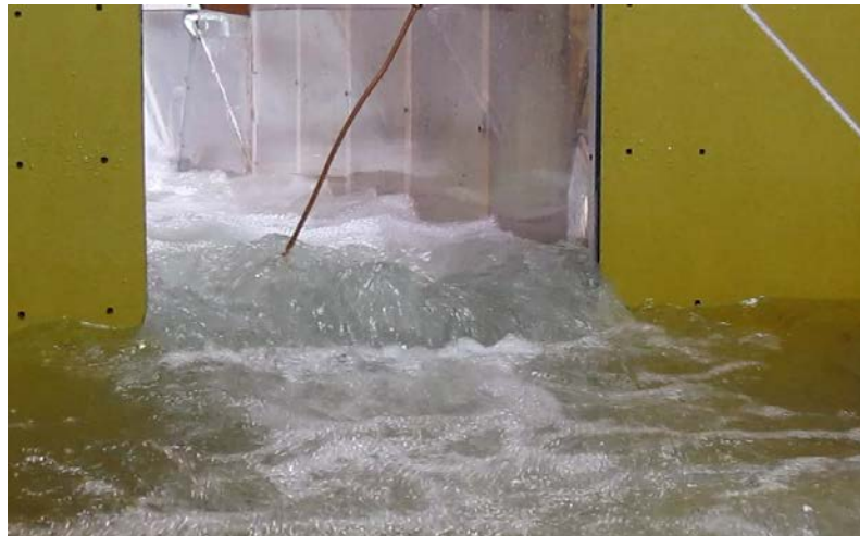
Figure A-13. — Flow over the top of staggered deflectors at design flow ( 956 \text{ ft}^3/\text{s} ) with the lowest deflector bottom edge located 6.2 ft above basin floor.
