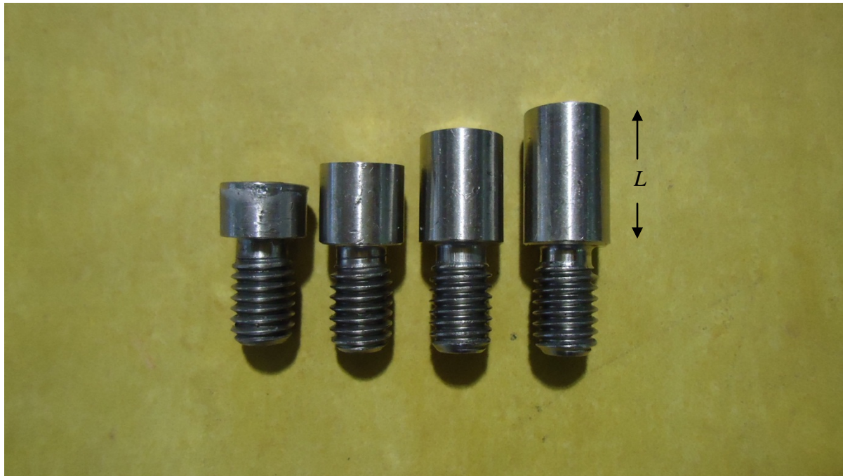
Figure 5 Model scale gate catcher pin lengths that were used in the hydraulic model testing ( L = 3.5, 5.5, 7.5 , and 9.5 prototype inches).
