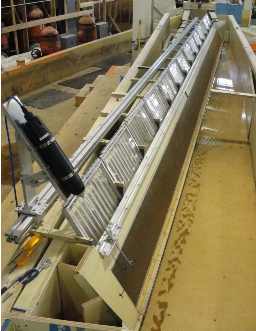
Figure 4. Fish screen looking downstream. Notice the louver panels, Nortek velocity meter and meter guide rail.
