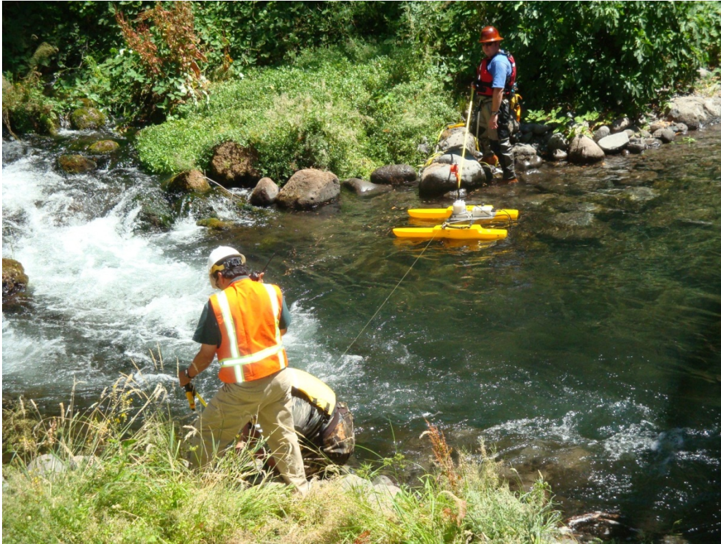
Figure 7. August 2012 field visit. DWR shown collecting velocity profiles upstream of the dam.
