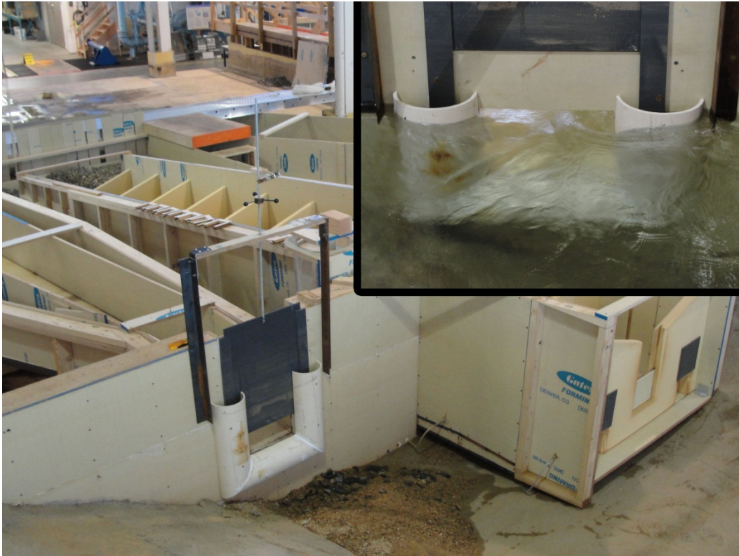
Figure 20. One-foot-radius half pipe bullnose around the entrance to the diversion. In the inset picture the flow can be seen curving around the bullnose into the diversion channel.
