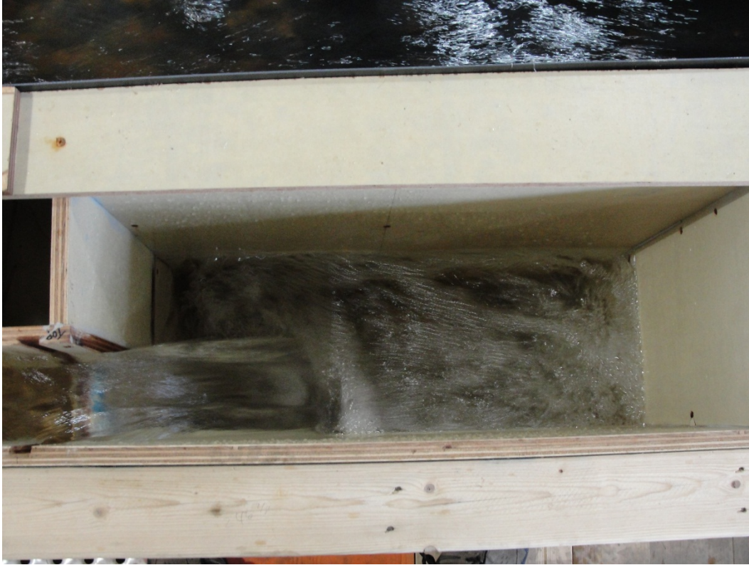
Figure 26. Bypass downwell chamber passing 7.5 ft 3 /s.
