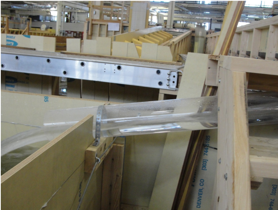
Figure 25. Bypass pipe passing 7.5 \text{ ft}^3/\text{s} .
