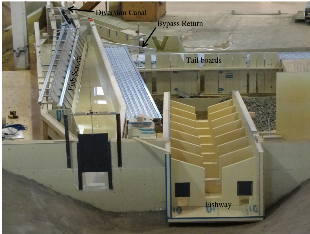
Figure 3. NBCF physical model showing the original fish ladder and fish screen
