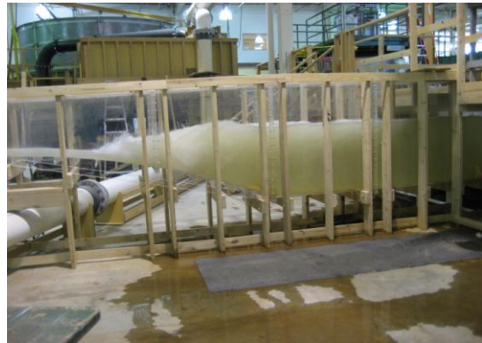
Figure 11. Choke Canyon 1:6 scale model stilling basin.
