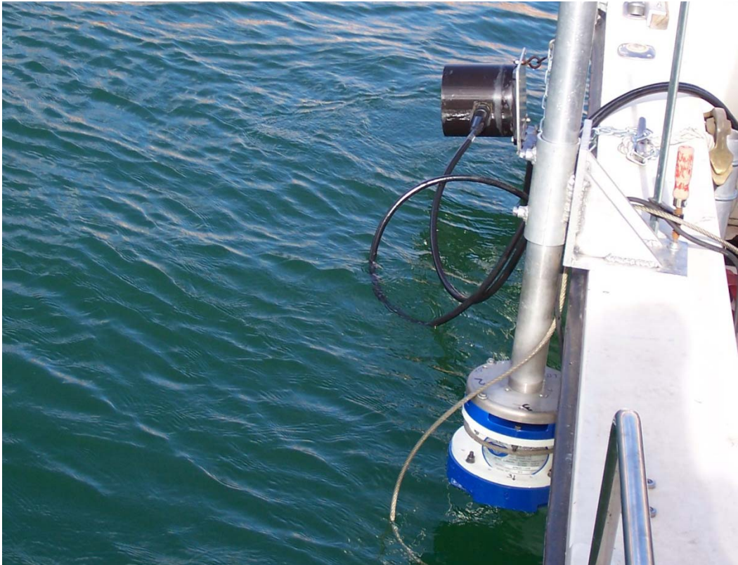
Figure 4. Photograph of ADCP mounted to the gunwhale (foreground). The black transducer (background) was used to survey fish distribution in the forebay.
