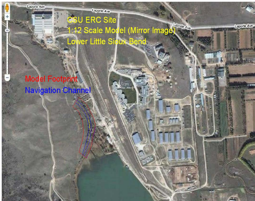
Figure 20 - 1:12 Lower Little Sioux Bend Mirror Image Overlay at Colorado State University Engineering Research Center Site
