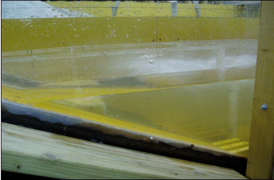
Figure 25. Side view with a 12.5-ft-long deflector installed at 3071.5 ft and existing stilling basin geometry. At a discharge of 700 \text{ ft}^3/\text{s} , mild undular flow was observed.
