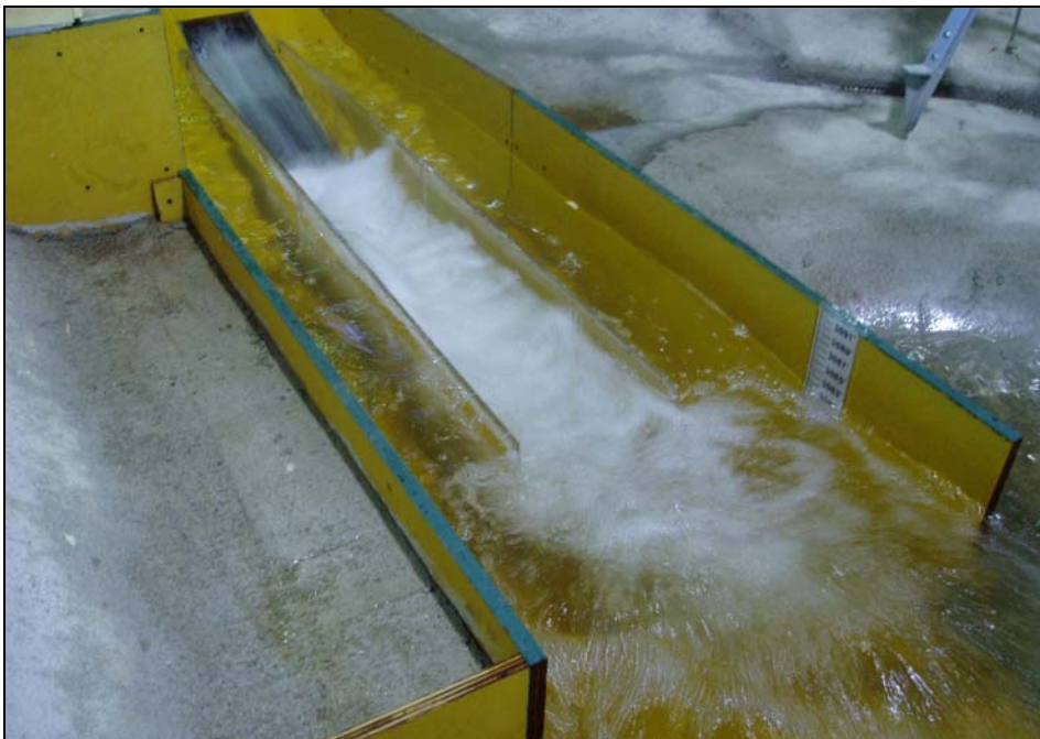
Figure 20. Surface view with no deflector installed and existing stilling basin geometry. At a discharge of 3,000 \text{ ft}^3/\text{s} , plunging flow was observed.
