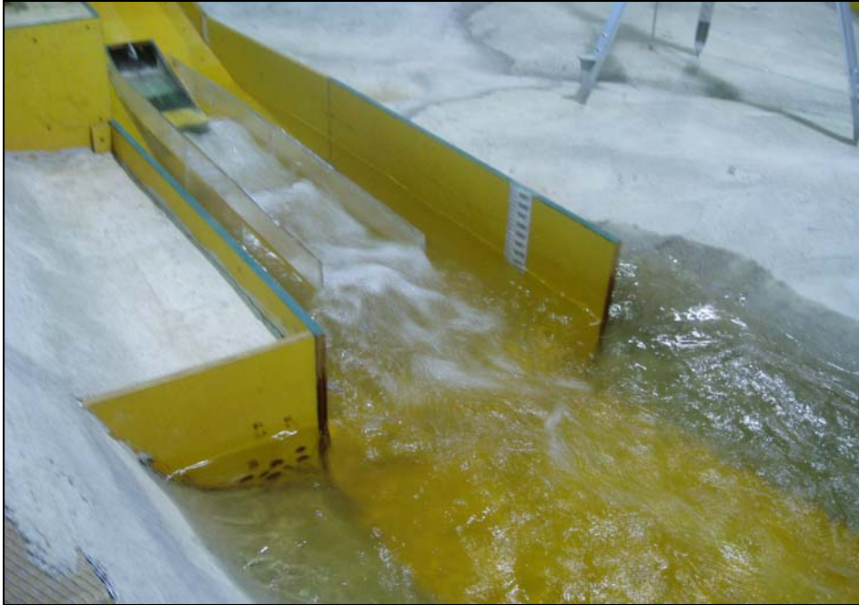
Figure 32. Surface view with a 20-ft-long deflector installed at 3070.3 ft and existing stilling basin geometry. At a discharge of 1,000 \text{ ft}^3/\text{s} , undular flow was observed.
