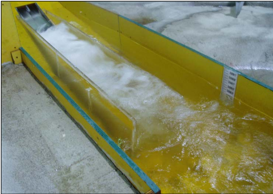
Figure 18. Surface view with no deflector installed and existing stilling basin geometry. At a discharge of 2,000 ft 3 /s, plunging flow was observed.
