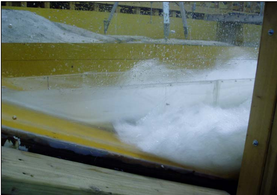
Figure 54. Condition 2: Side view with deflector installed and existing stilling basin geometry (deflector elevation 3071.5 ft). Release flow was 8,120 ft 3 /s.
