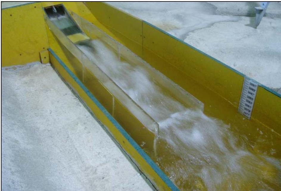
Figure 28. Surface view with a 12.5-ft-long deflector installed at 3071.5 ft and existing stilling basin geometry. At a discharge of 1,000 ft 3 /s, mild undular flow was observed.
