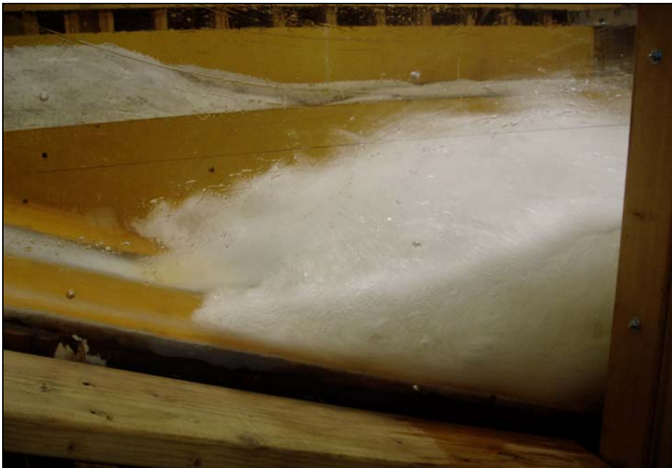
Figure 51. Condition 3: Side view with deflector installed and splitter walls completely removed (deflector elevation 3073.3 ft). Release flow was 4,000 ft 3 /s.
