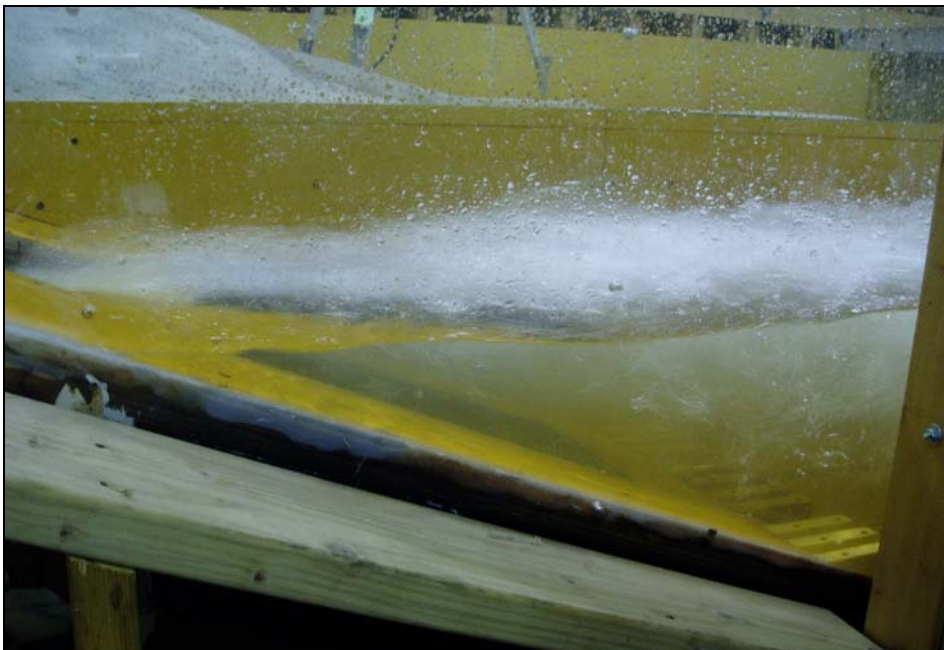
Figure 38. Deflector installed at 3075.3 ft with splitter walls fully removed. At a discharge of 2,000 ft 3 /s, some plunging bubbles were observed.
