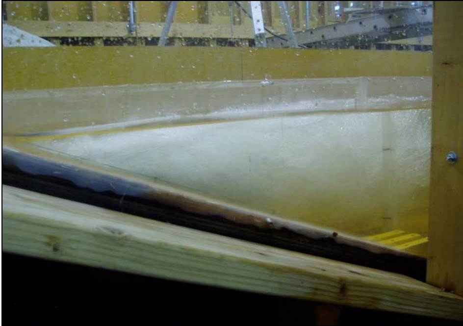
Figure 15. Side view with no deflector installed and existing stilling basin geometry. At a discharge of 1,000 \text{ ft}^3/\text{s} , plunging flow was observed.
