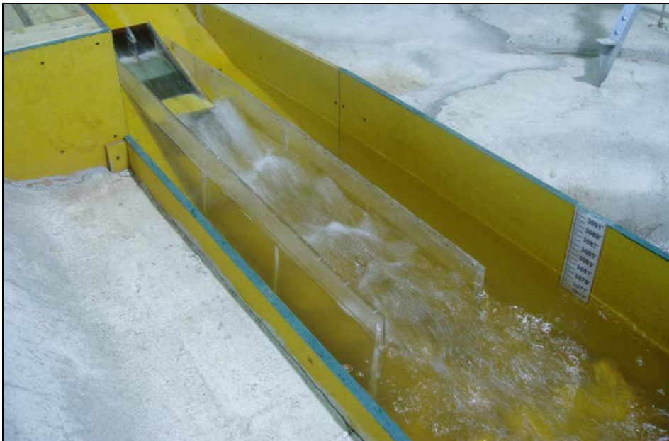
Figure 26. Surface view with a 12.5-ft-long deflector installed at 3071.5 ft and existing stilling basin geometry. At a discharge of 700 \text{ ft}^3/\text{s} , mild undular flow was observed.
