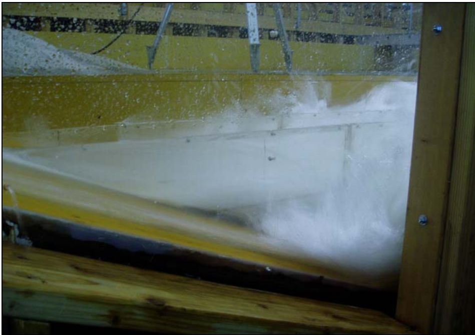
Figure 59. Condition 2: Side view with deflector installed and existing stilling basin geometry (deflector elevation 3071.5 ft). Release flow was 14,965 ft 3 /s.
