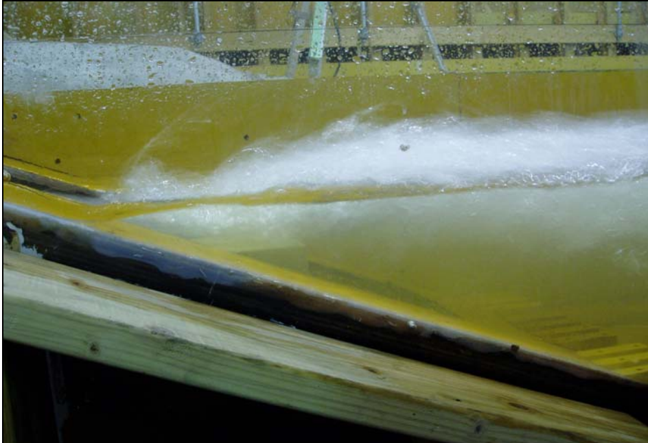
Figure 37. Deflector installed at 3071.5 ft with splitter walls fully removed. At a discharge of 2,000 ft 3 /s, undular flow was observed.
