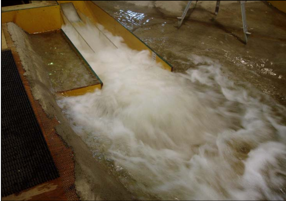
Figure 60. Condition 2: Surface view with deflector installed and existing stilling basin geometry (deflector elevation 3071.5 ft). Release flow was 14,965 ft 3 /s.
