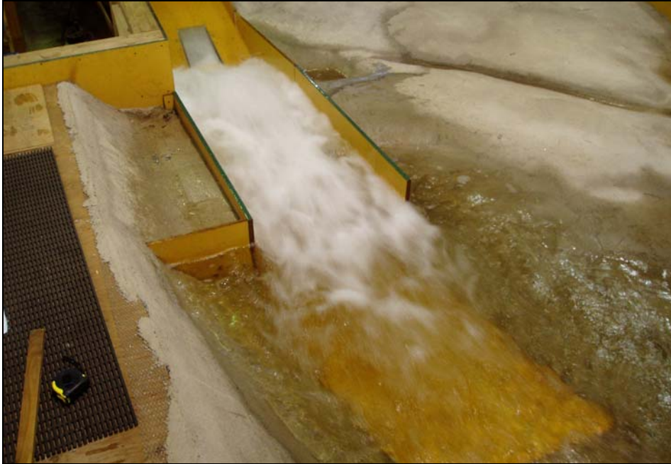
Figure 52. Condition 3: Surface view with deflector installed and splitter walls completely removed (deflector elevation 3073.3 ft). Release flow was 4,000 ft 3 /s.
