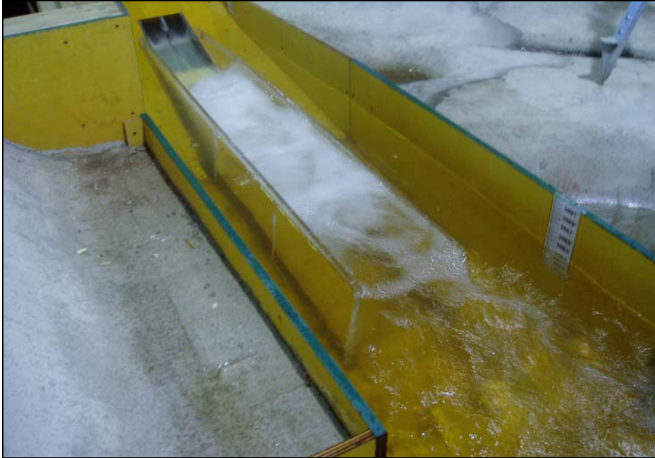
Figure 24. Surface view with a 12.5-ft-long deflector installed at 3073.3 ft and existing stilling basin geometry. At a discharge of 2,000 ft 3 /s, plunging flow was observed.
