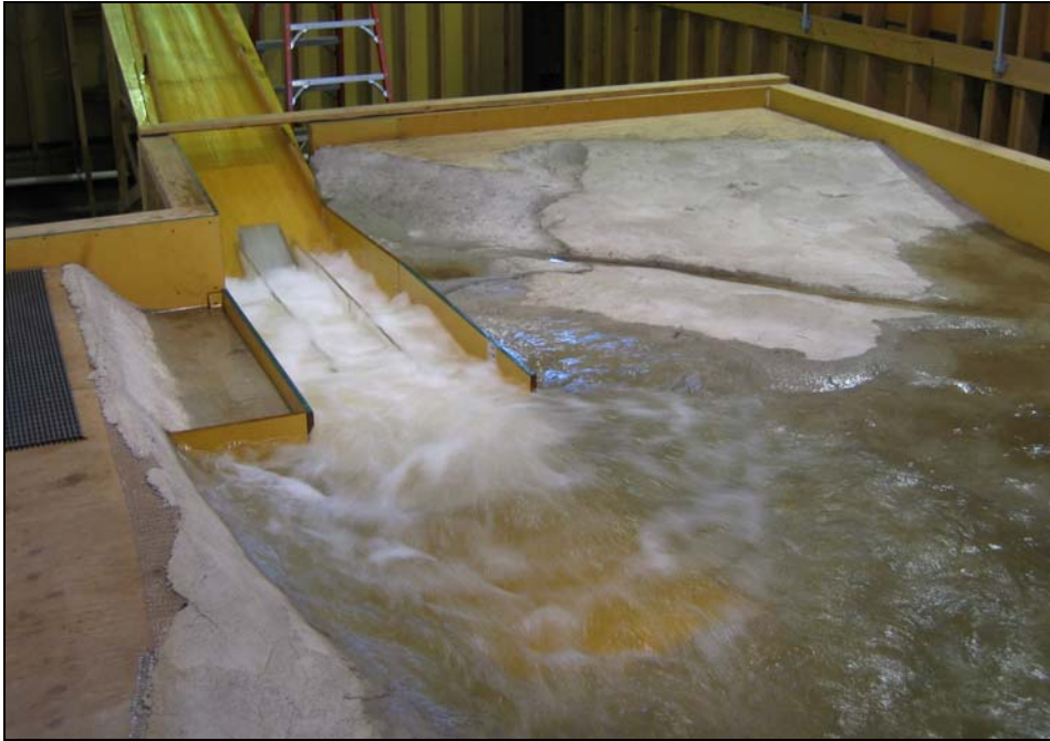
Figure 53. Condition 1: Surface view with no deflector and existing stilling basin geometry at a discharge of 8,120 ft 3 /s.
