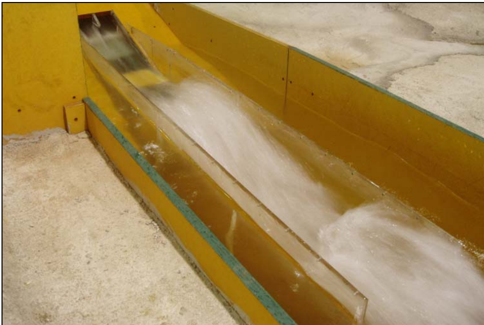
Figure 30. Surface view with a 12.5-ft-long deflector installed at 3071.5 ft and existing stilling basin geometry. At a discharge of 2,000 ft 3 /s, undular flow was observed.
