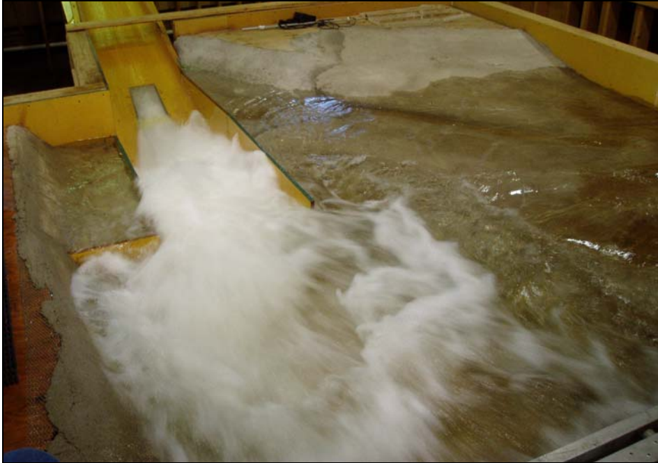
Figure 62. Condition 3: Surface view with deflector installed and splitter walls completely removed (deflector elevation 3073.3 ft). Release flow was 14,965 ft 3 /s. Note the uneven flow distribution in the stilling basin. Flow moves over right stilling basin wall and up the right bankline.
