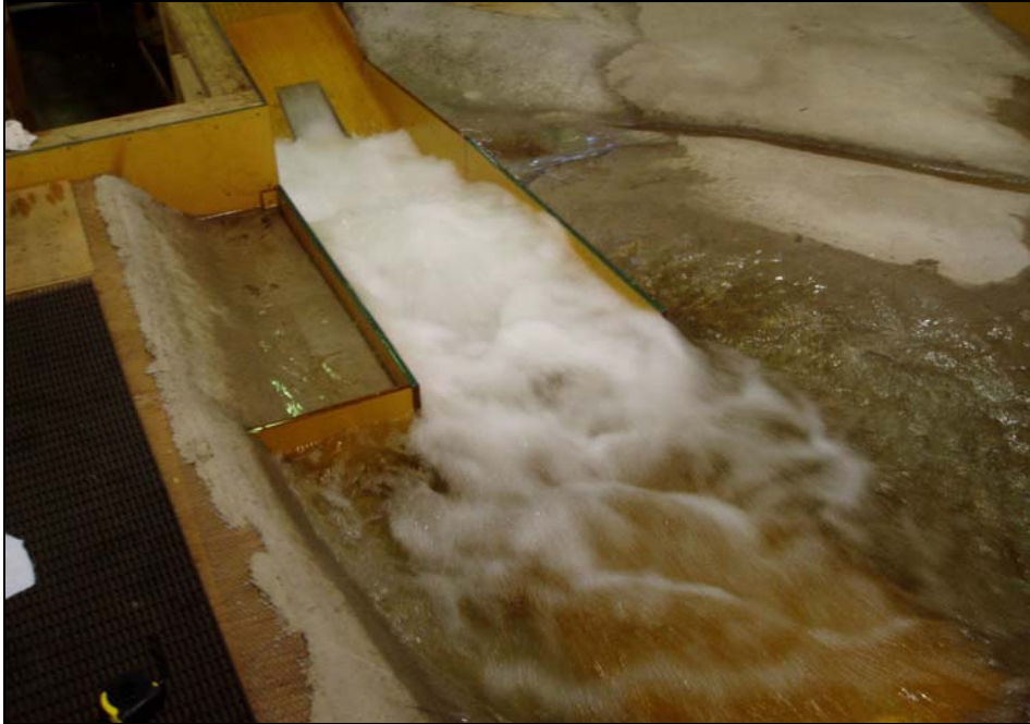
Figure 57. Condition 3: Surface view with deflector installed and splitter walls completely removed (deflector elevation 3073.3 ft). Release flow was 8,120 ft 3 /s.
