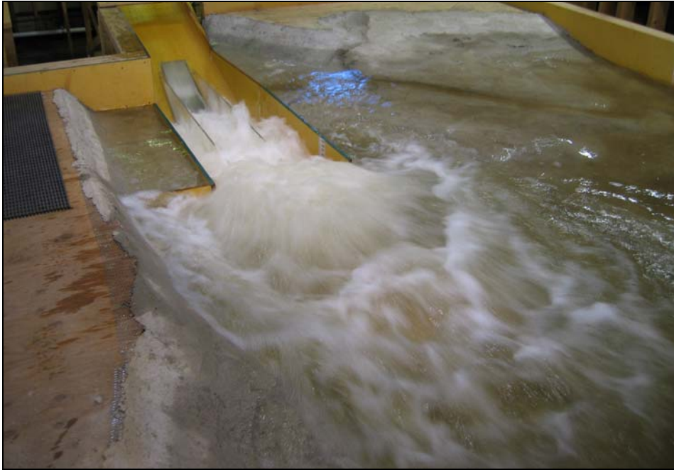
Figure 58. Condition 1: Surface view with no deflector and existing stilling basin geometry at a discharge of 14,965 ft 3 /s.
