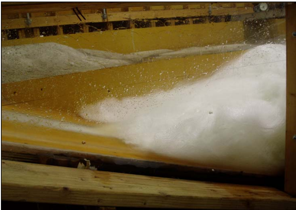
Figure 56. Condition 3: Side view with deflector installed and splitter walls completely removed (deflector elevation 3073.3 ft). Release flow was 8,120 ft 3 /s.
