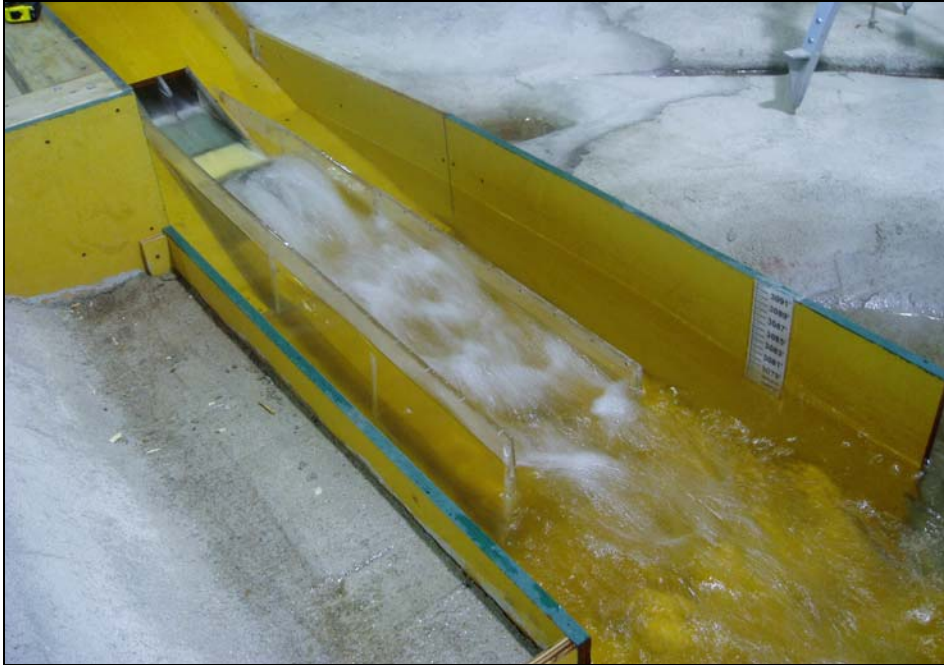
Figure 22. Surface view with a 12.5-ft-long deflector installed at 3073.3 ft and existing stilling basin geometry. At a discharge of 1,000 \text{ ft}^3/\text{s} , undular flow was observed.
