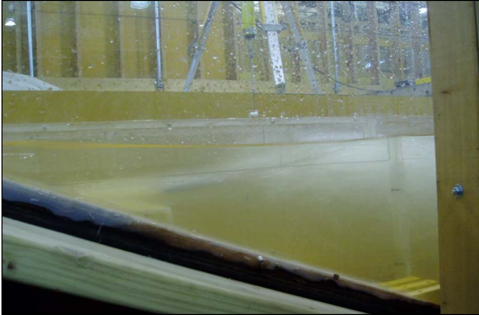
Figure 29. Side view with a 12.5-ft-long deflector installed at 3071.5 ft and existing stilling basin geometry. At a discharge of 2,000 ft 3 /s, undular flow was observed.
