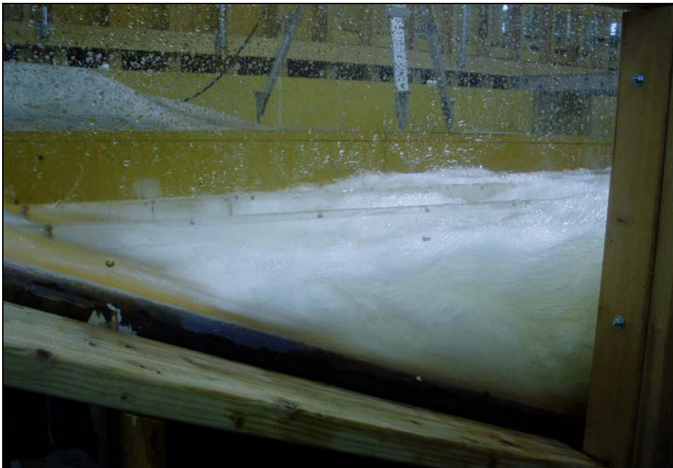
Figure 47. Condition 1: Side view with no deflector and existing stilling basin geometry at a discharge of 4,000 ft 3 /s.
