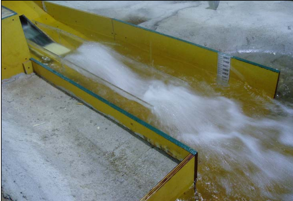
Figure 34. Surface view with a 20-ft-long deflector installed at 3070.3 ft and existing stilling basin geometry. At a discharge of 2,000 \text{ ft}^3/\text{s} , strong undular flow was observed.
