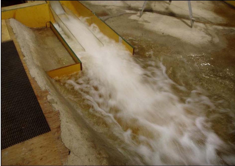
Figure 55. Condition 2: Surface view with deflector installed and existing stilling basin geometry (deflector elevation 3071.5 ft). Release flow was 8,120 ft 3 /s.
