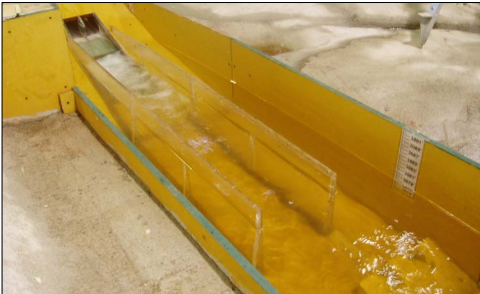
Figure 14. Surface view with no deflector installed and existing stilling basin geometry. At a discharge of 700 ft 3 /s, plunging flow was observed.
