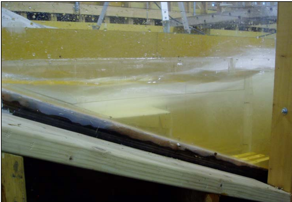
Figure 35. Unstable undular flow at 3,000 \text{ ft}^3/\text{s} with a 20-ft-long deflector installed at elevation 3070.3 ft. Existing stilling basin geometry.
