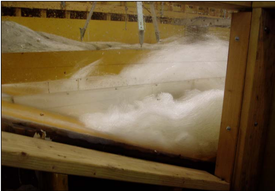
Figure 49. Condition 2: Side view with deflector installed and existing stilling basin geometry (deflector elevation 3071.5 \text{ ft} ). Release flow was 4,000 \text{ ft}^3/\text{s} .
