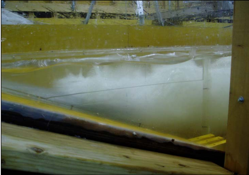
Figure 19. Side view with no deflector installed and existing stilling basin geometry. At a discharge of 3,000 \text{ ft}^3/\text{s} , plunging flow was observed.
