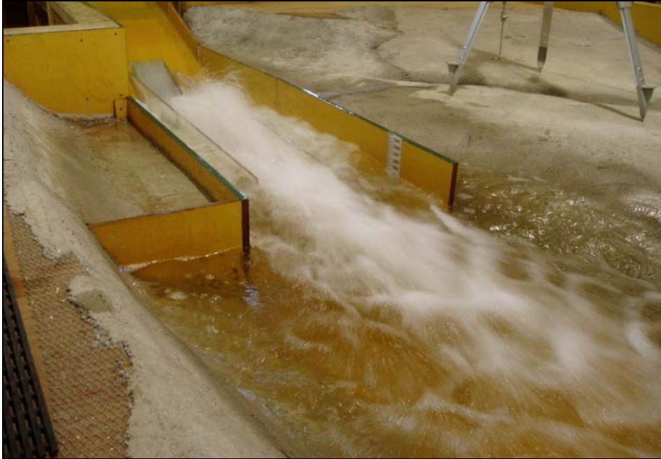
Figure 50. Condition 2: Surface view with deflector installed and existing stilling basin geometry (deflector elevation 3071.5 ft). Release flow was 4,000 ft 3 /s.
