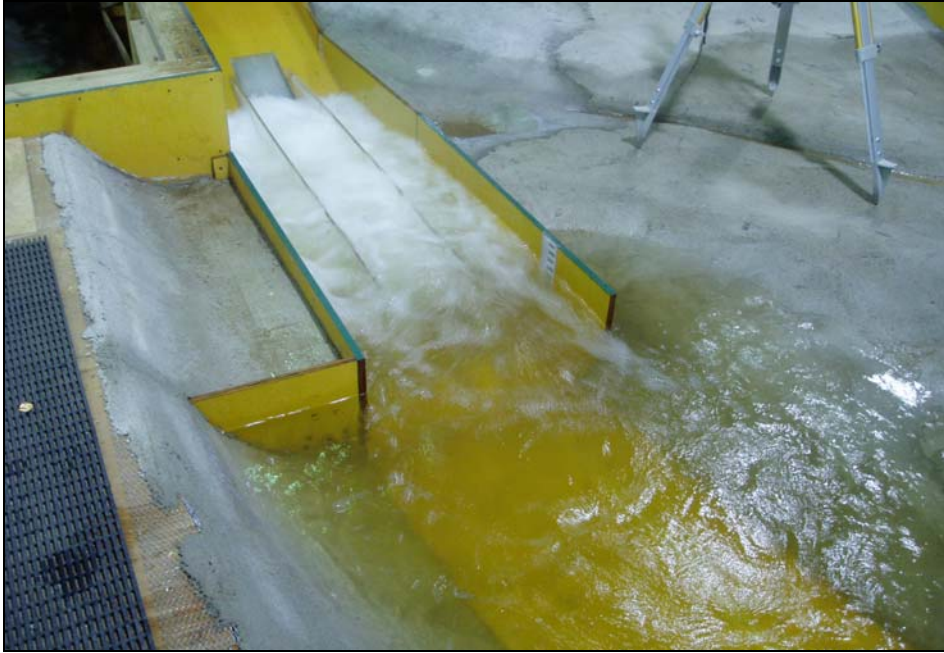
Figure 48. Condition 1: Surface view with no deflector and existing stilling basin geometry at a discharge of 4,000 \text{ ft}^3/\text{s} .
