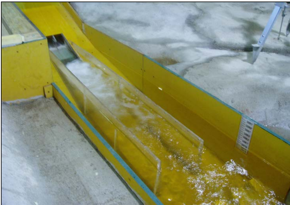
Figure 16. Surface view with no deflector installed and existing stilling basin geometry. At a discharge of 1,000 \text{ ft}^3/\text{s} , plunging flow was observed.
