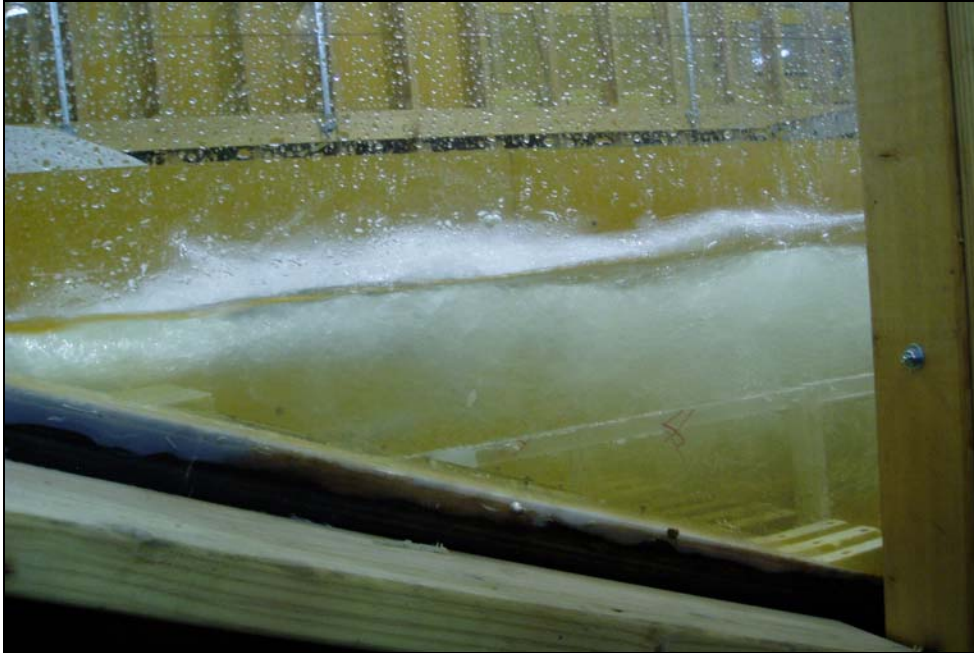
Figure 45. Deflector installed at 3073.3 ft with splitter walls reduced by 15 ft. At a discharge of 2,000 ft 3 /s, skimming flow occurred on the surface, but some bubbles were observed deep in the basin.
