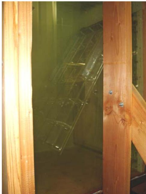
Figure 10: Model gate in operation, fully submerged.
